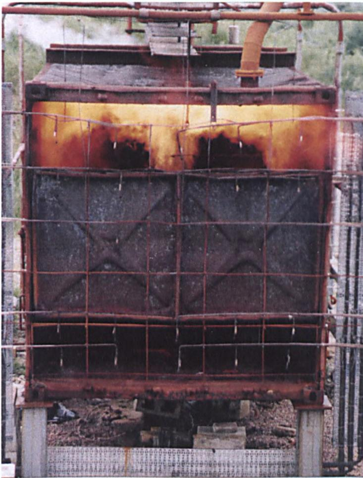
*Plate 6: Experimental fire-rig with 0.1kg/s combustion of Propane*
