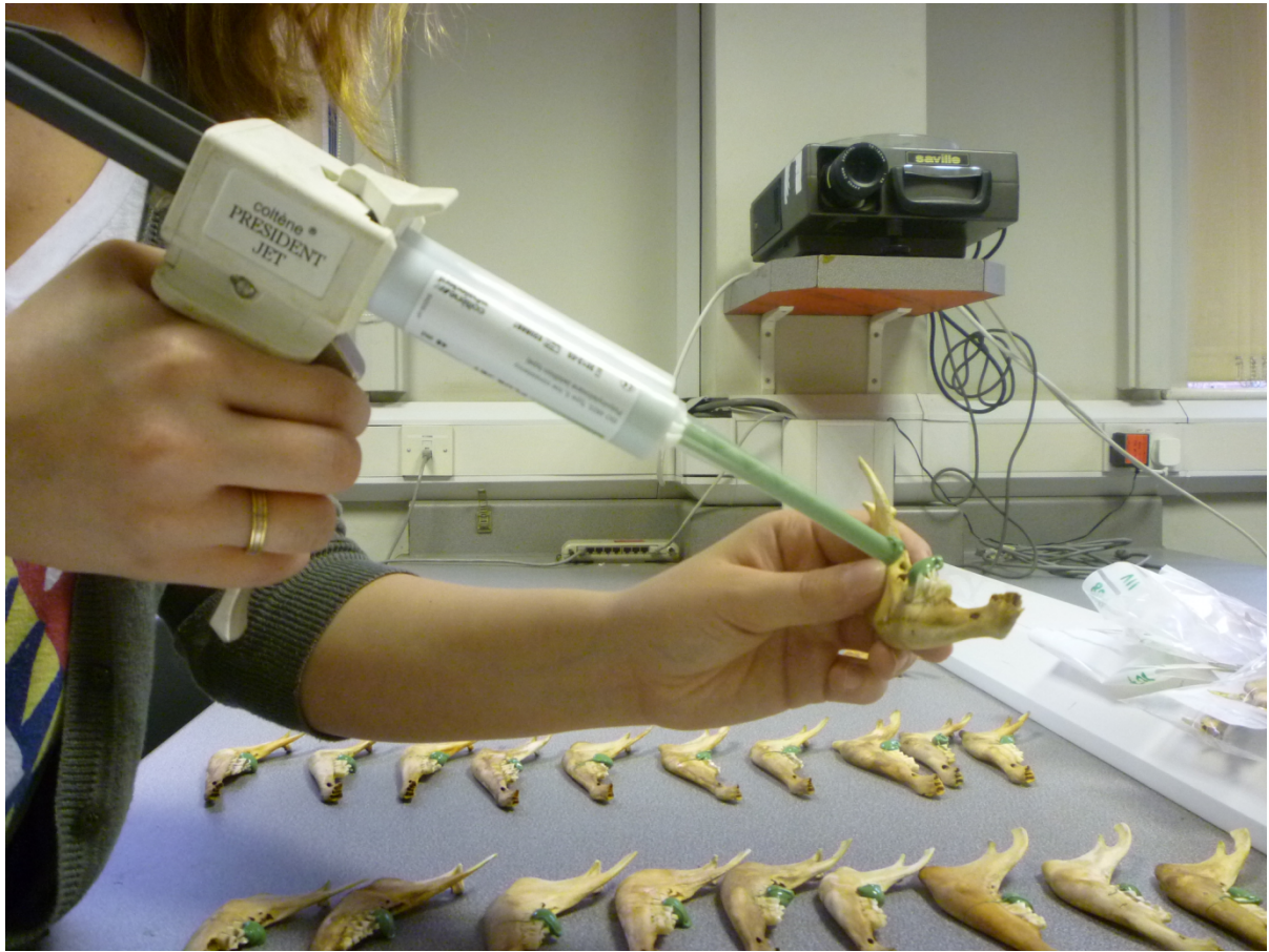
Figure 3.3: Photograph demonstrating the method for creating negative impressions of teeth using silicone material (Lawrence 2013).
