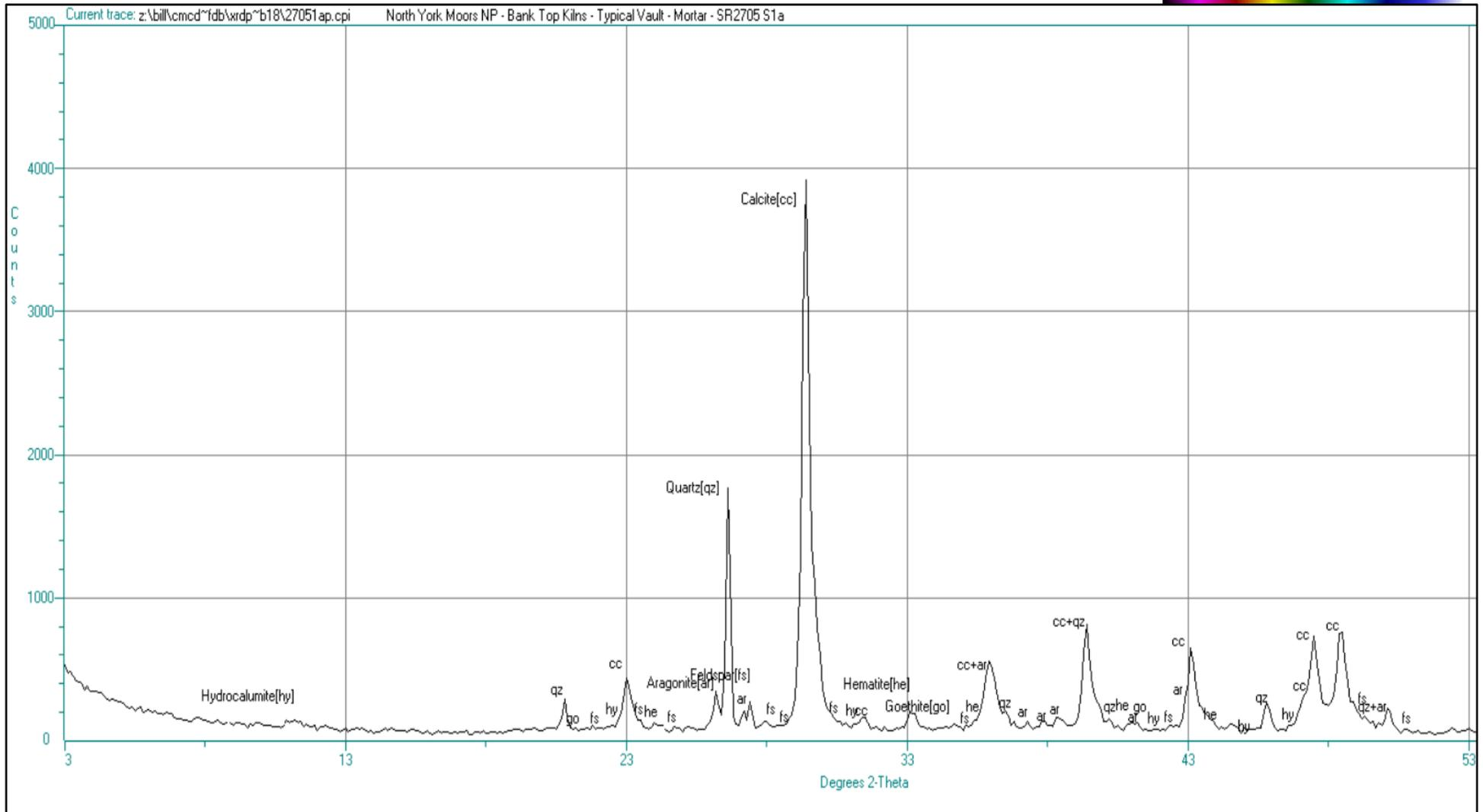
Figure No. 5: SR2705-S1A (BTK1A) Mortar Typical Vault Stonework, Bank Top Kilns.
