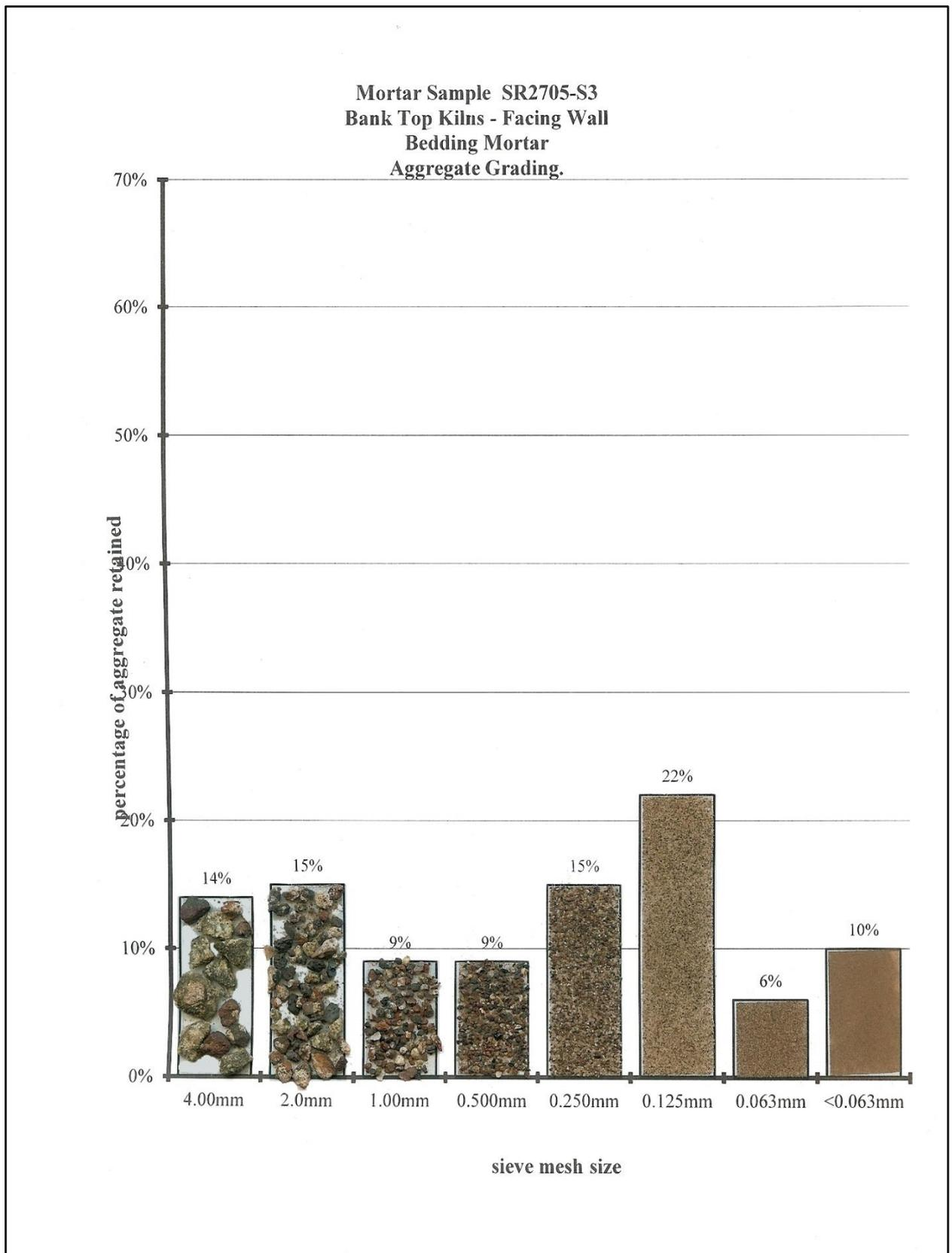
**Figure No. 4** – Aggregate Grading on Aggregate recovered from sample BTK3.
