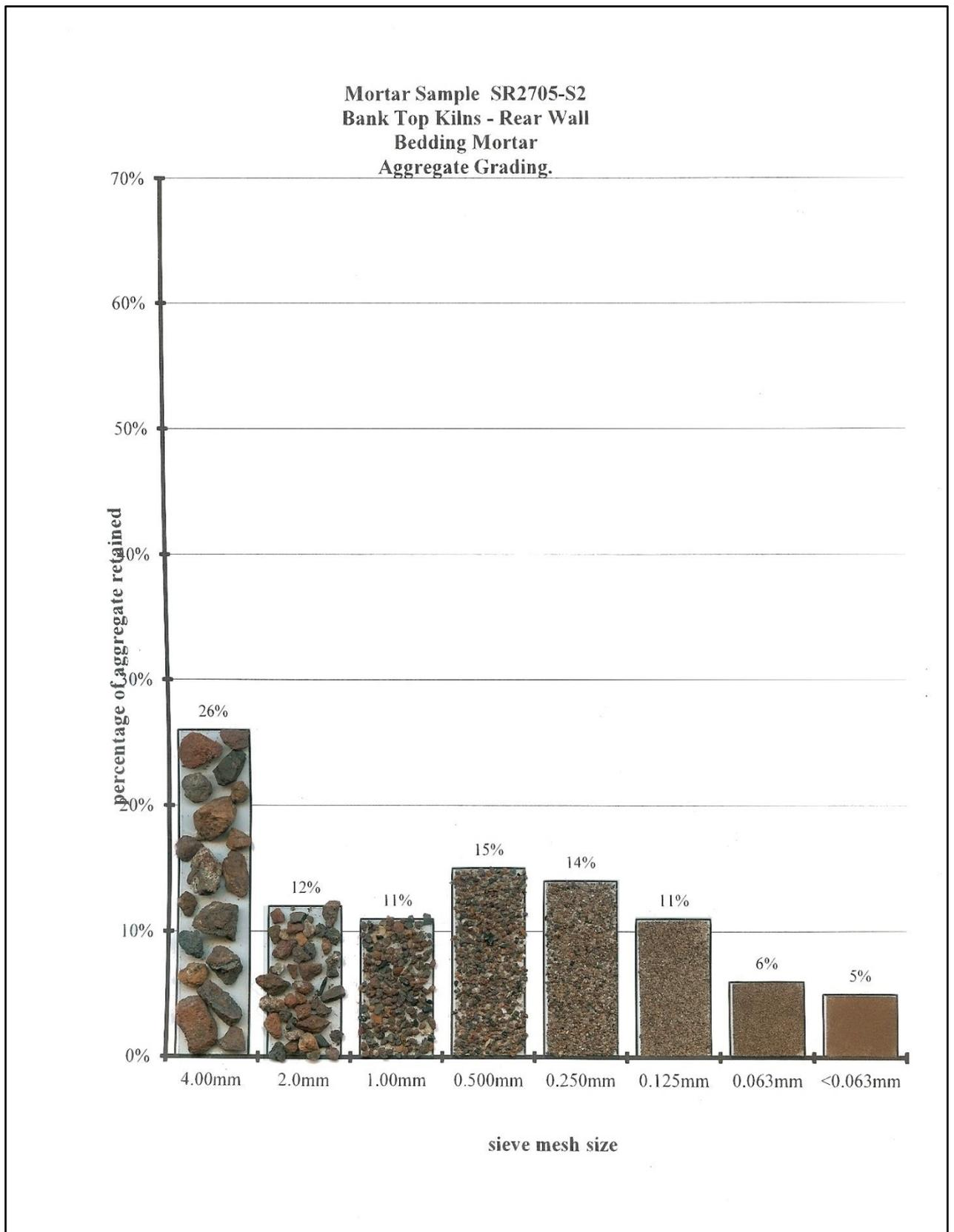
Figure No. 3 – Aggregate Grading on Aggregate recovered from sample BTK2.
