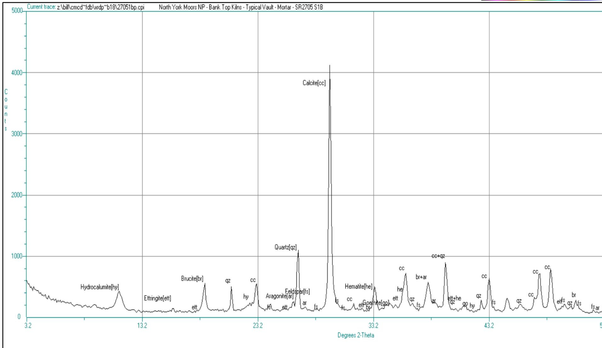
Figure No. 6: SR2705-S1B (BTK1B) Mortar Typical Vault Brickwork, Bank Top Kilns.
