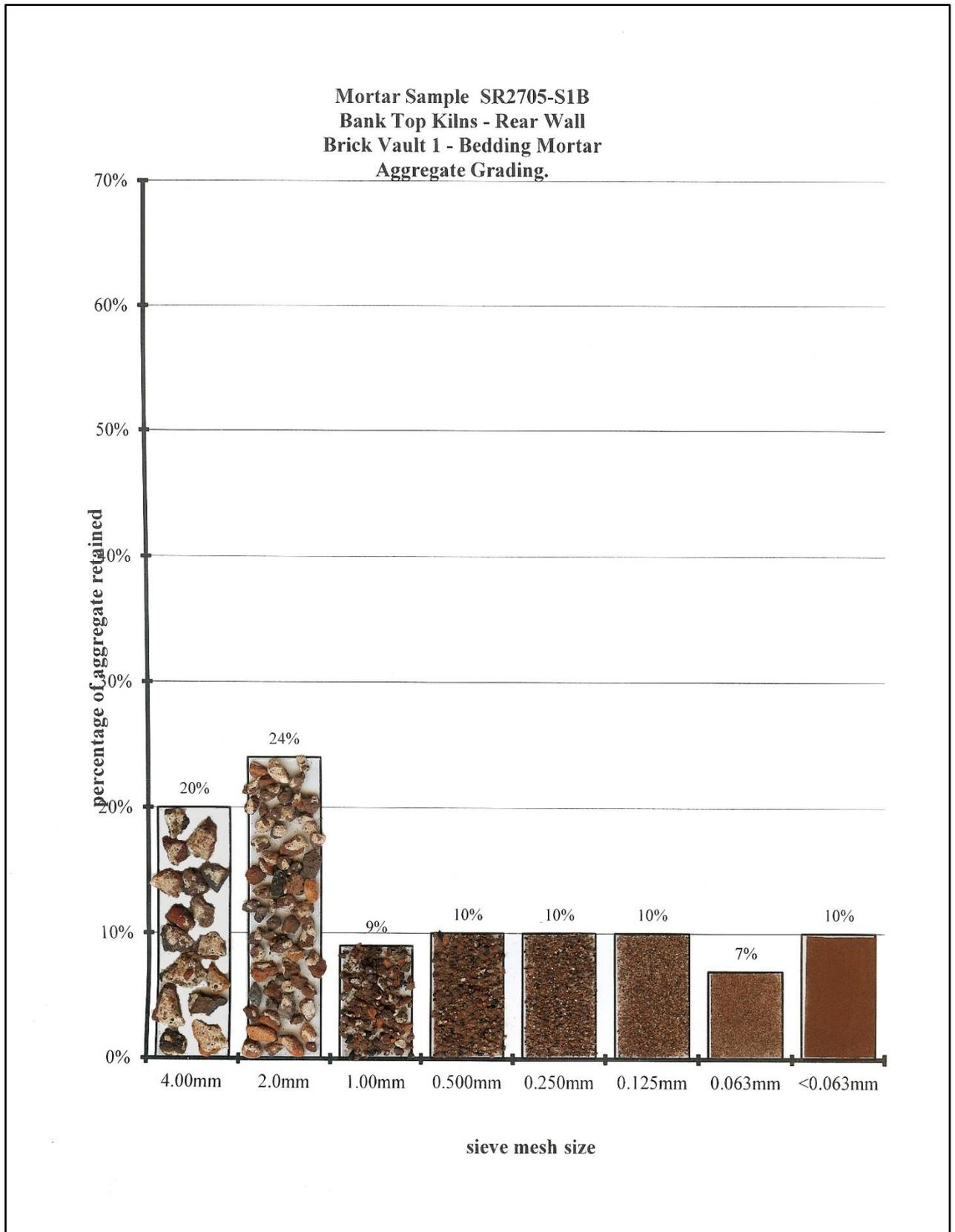
**Figure No. 2:** Aggregate Grading on Aggregate recovered from sample BTK1B.
