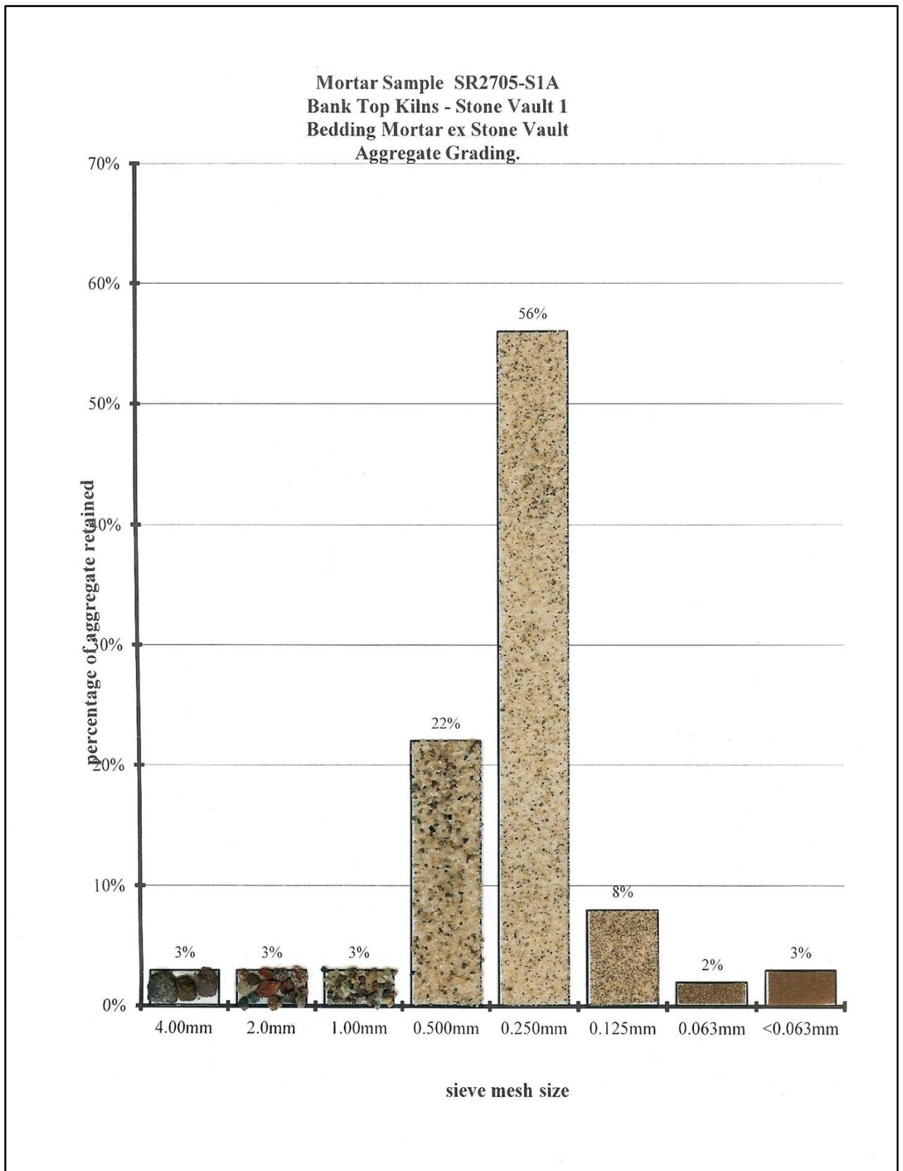
**Figure No. 1:** Aggregate Grading on Aggregate recovered from sample BTK1A.
