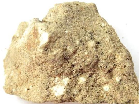
**Plates No. 5 & 6:** The plates above show the condition of the mortar in sample “D”. The left plate is the sample, as received, with the right plate showing a fractured surface through one of the larger pieces. Note the abundance of sub-angular to rounded lime inclusions.
