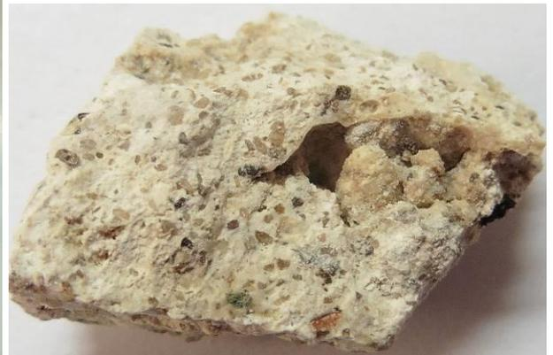
**Plates No. 15 & 16:** View of the sample as received, left plate, and a magnified view of a fractured surface through the thickness of the pointing mortar.
