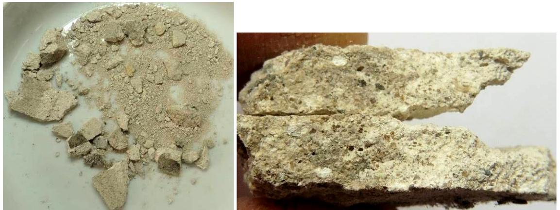
**Plates No. 1 & 2:** The above left plate shows the sample as received, with a few intact pieces along with a quantity of fines. The right plate shows a freshly fractured surface through the thickness of the mortar. The piece in the image had been treated with a phenolphthalein indicator solution to check for carbonation. The mortar was found to be fully carbonated.
