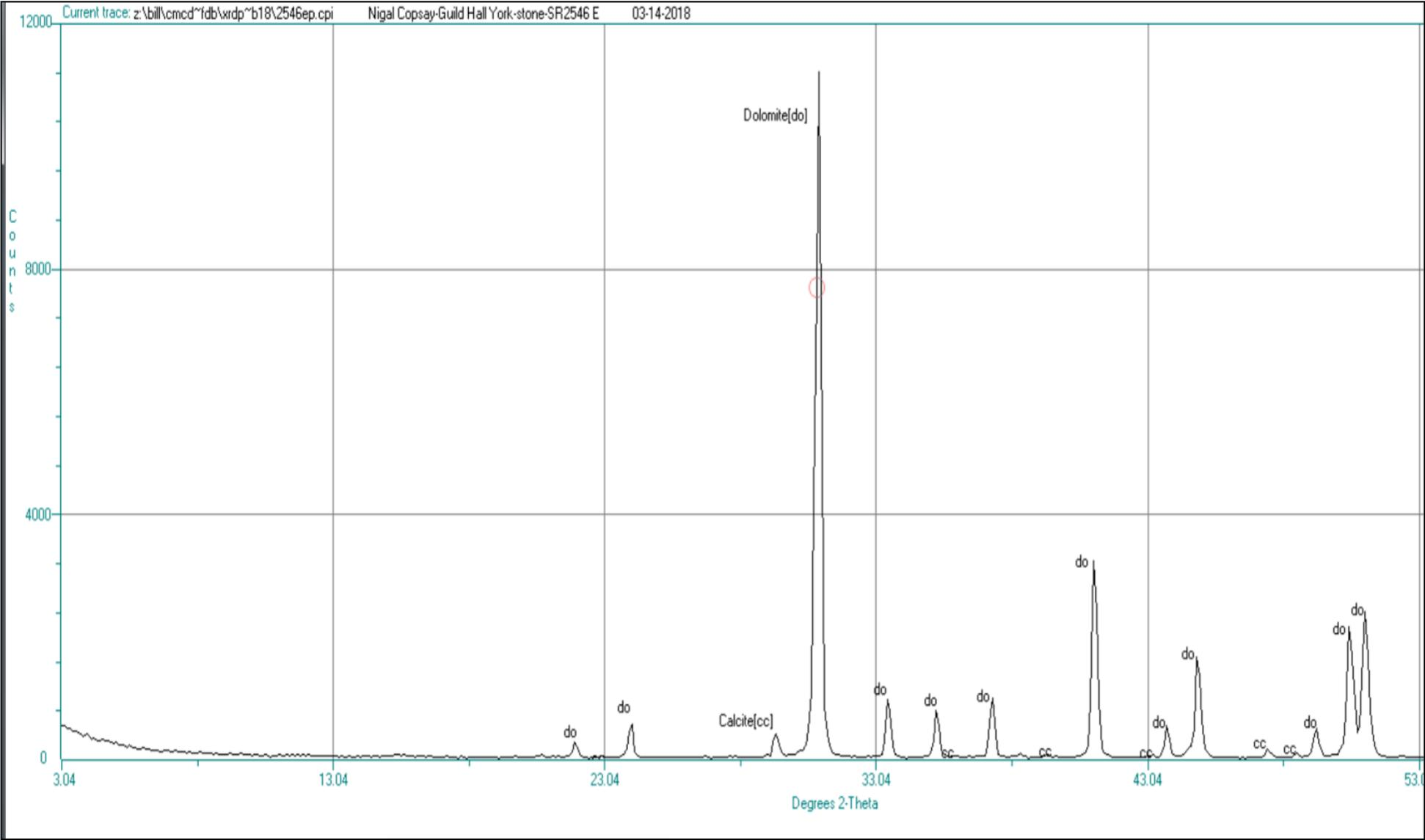
Figure No. 8 – SR2546-S4 – “E” Stone Masonry sample, to check for Dolomite.
