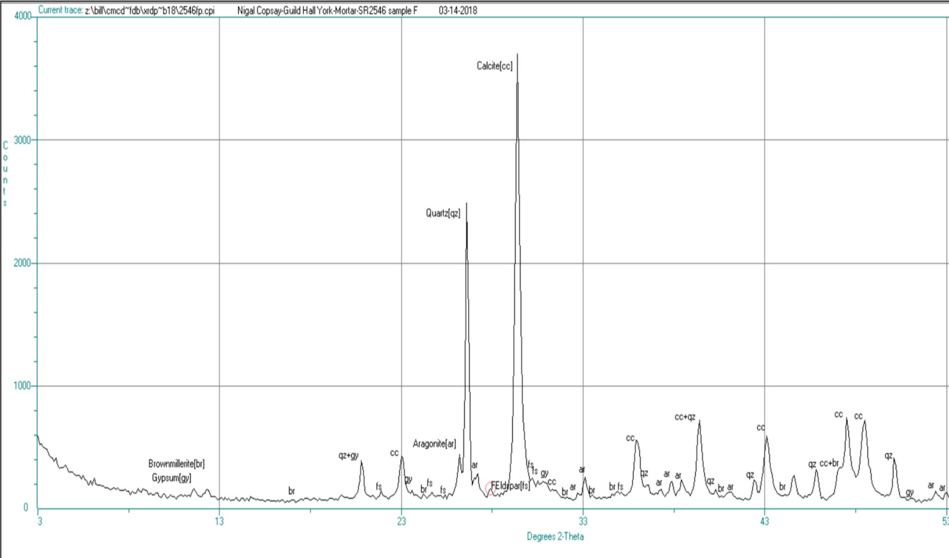
Figure No. 9 – SR2546-S5 – “F” Binder ex Pointing from Sand Lime Brick on Lean-to in Lane.
