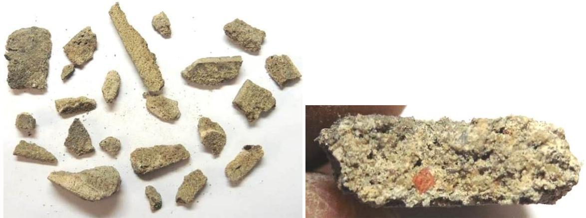
**Plates No. 17 & 18:** The left plate shows the intact ribbons of pointing mortar from which the sample was composed. The right plate shows a fresh fracture through the thickness of one of the intact pieces, displaying a well compacted mortar.
