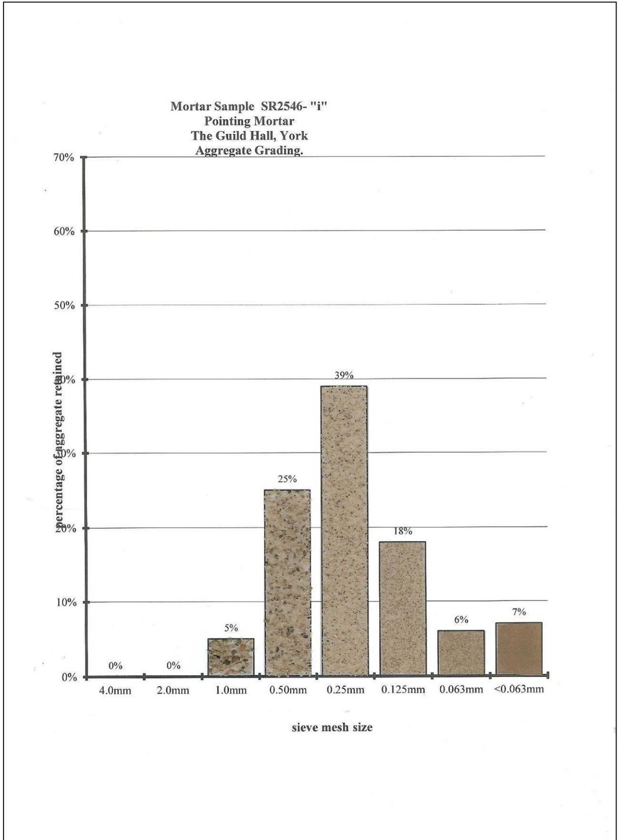
**Figure No. 4:** Grading of Aggregate from sample SR2546-S8 "i"
