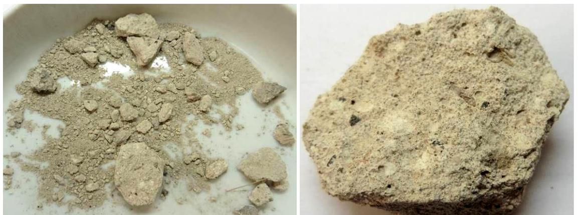
**Plates No. 13 & 14:** The left plate shows the sample as received, with the right plate showing a close-up of the largest fragment, which contains an abundance of lime inclusions.
