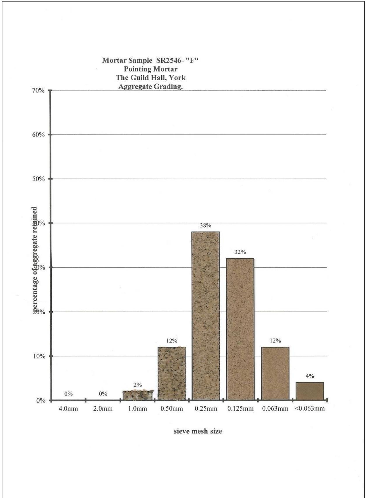
**Figure No. 2:** Grading of Aggregate from sample SR2546-S5 "F"
