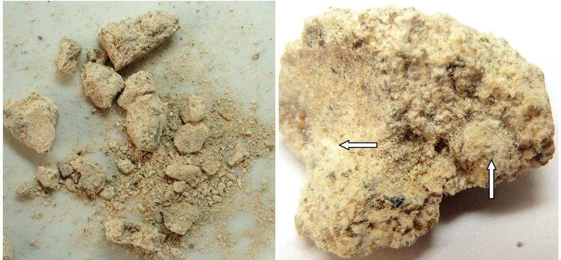
**Plates No. 11 & 12:** The left plate shows the sample as received, with the right plate showing a magnified view of one intact piece, where the dense fabric can be seen along with line inclusions, these are arrowed in plate.
