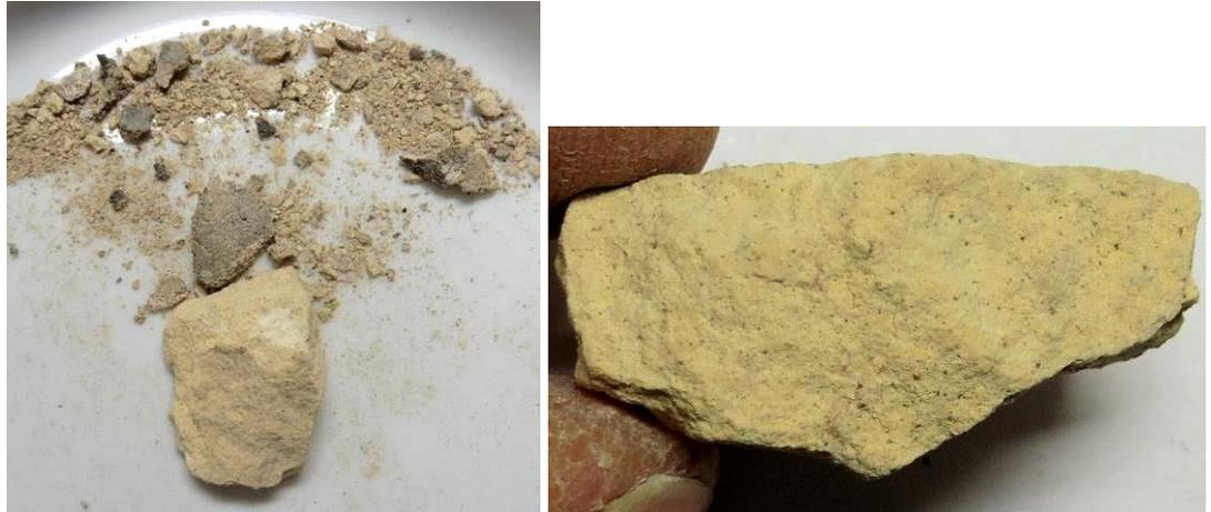
**Plates No. 7 & 8:** The left plate shows a view of the sample as received. The right plate shows a close-up of a freshly fractured surface through the stone fragment.
