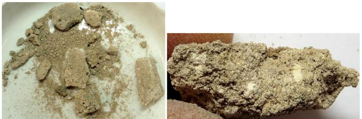
**Plates No. 9 & 10:** The left plate shows the sample as received with the right showing a fractured surface through an intact piece of the mortar, where lime inclusions can be seen.
