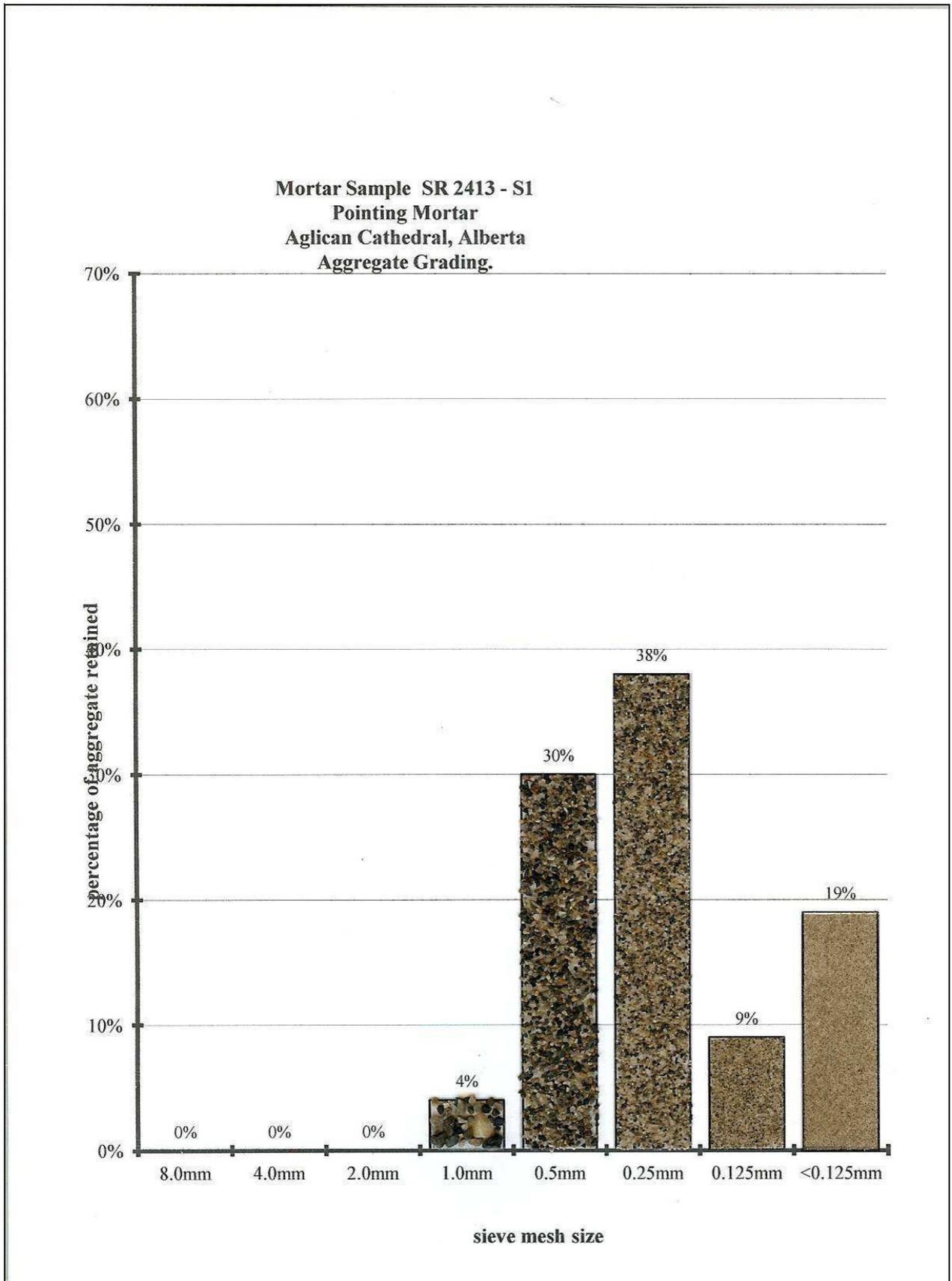
**Figure No. 3:** Aggregate grading – Sample SR2413-S1 – Pointing Mortar
