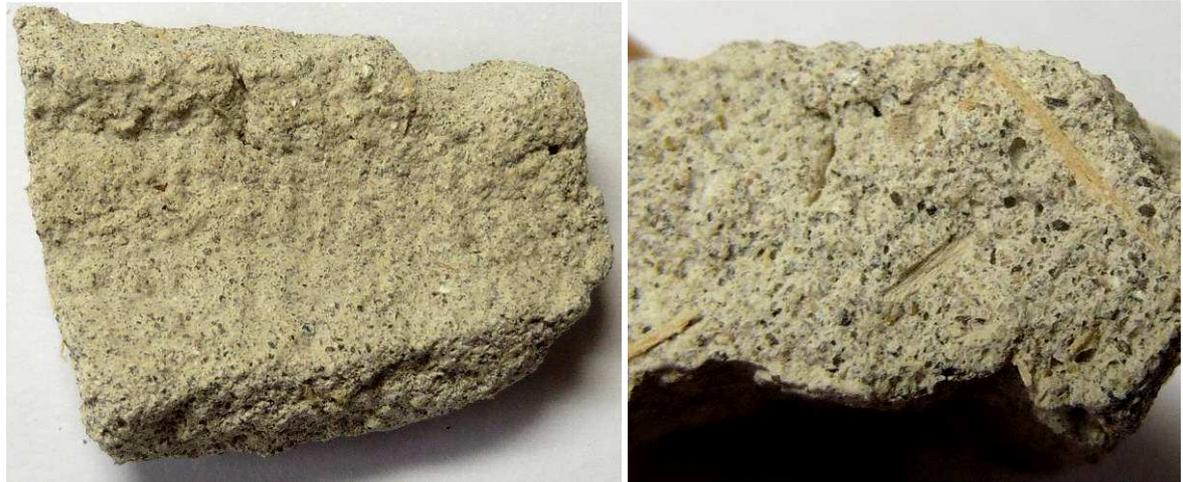
**Plates No. 6 & 7:** The left plate shows the condition of sample S2 as-received, with the right plate showing a magnified view of a freshly fractured surface through the thickness of the plate, where it was noted that the mortar contained an abundance of fine wood fibres, which given its distribution may infer that had been added purposefully to the plaster.
