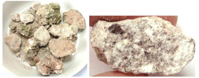
**Plates No. 5 & 6**: The left plate shows the sample, as received. The right plate shows a close-up of a freshly fractured surface, where the dense condition of the fabric can be seen along with abundance of angular white lime inclusions, grey and white limestone fragments, dark coal fragments, with patches of grey ash.
