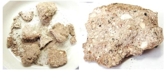
**Plates No. 3 & 4**: The left plate shows the sample as-received. The right plate shows a freshly fractured surface through the thickness of a large fragment, in which an abundance of lime inclusions and limestone fragments were apparent, with small dark coal fragments and red brick fragments distributed throughout.
