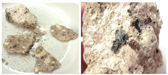
**Plates No. 7 & 8**: The left plate shows the four intact mortar fragments in the sample as received. The right plate shows a close-up of a fractured surface, through the largest intact piece. This shows a dense fabric, along with an abundance of lime inclusions and limestone fragments.
