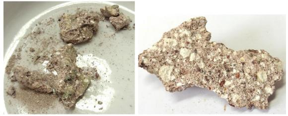
**Plates No. 1 & 2**: The left plate shows the intact pieces in this part of the mortar sample. With the right plate showing a magnified image of a freshly fractured surface through the thickness of the sample. Note the abundance of lime inclusions, and possible limestone, observed randomly distributed throughout.
