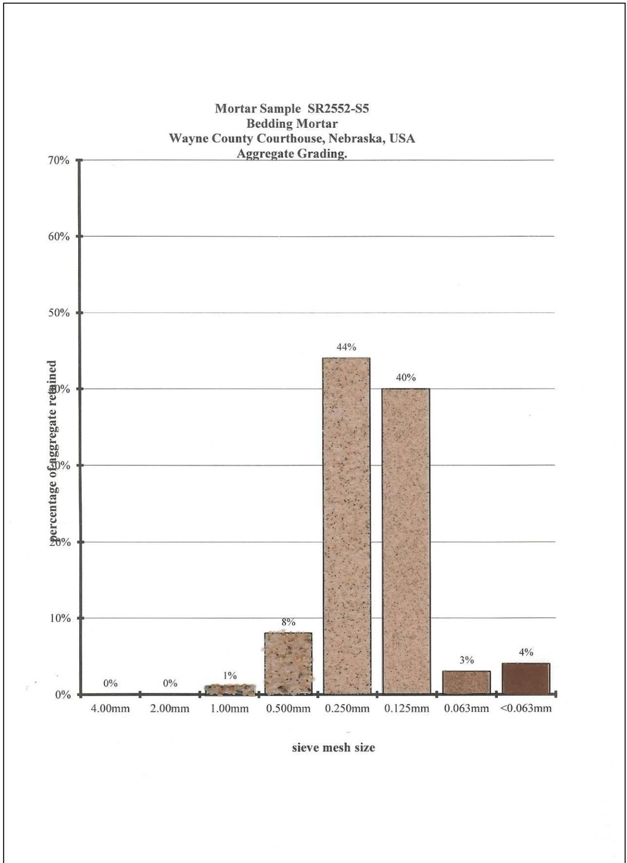
**Figure No. 3:** Grading of Aggregate from sample SR2552-S5
