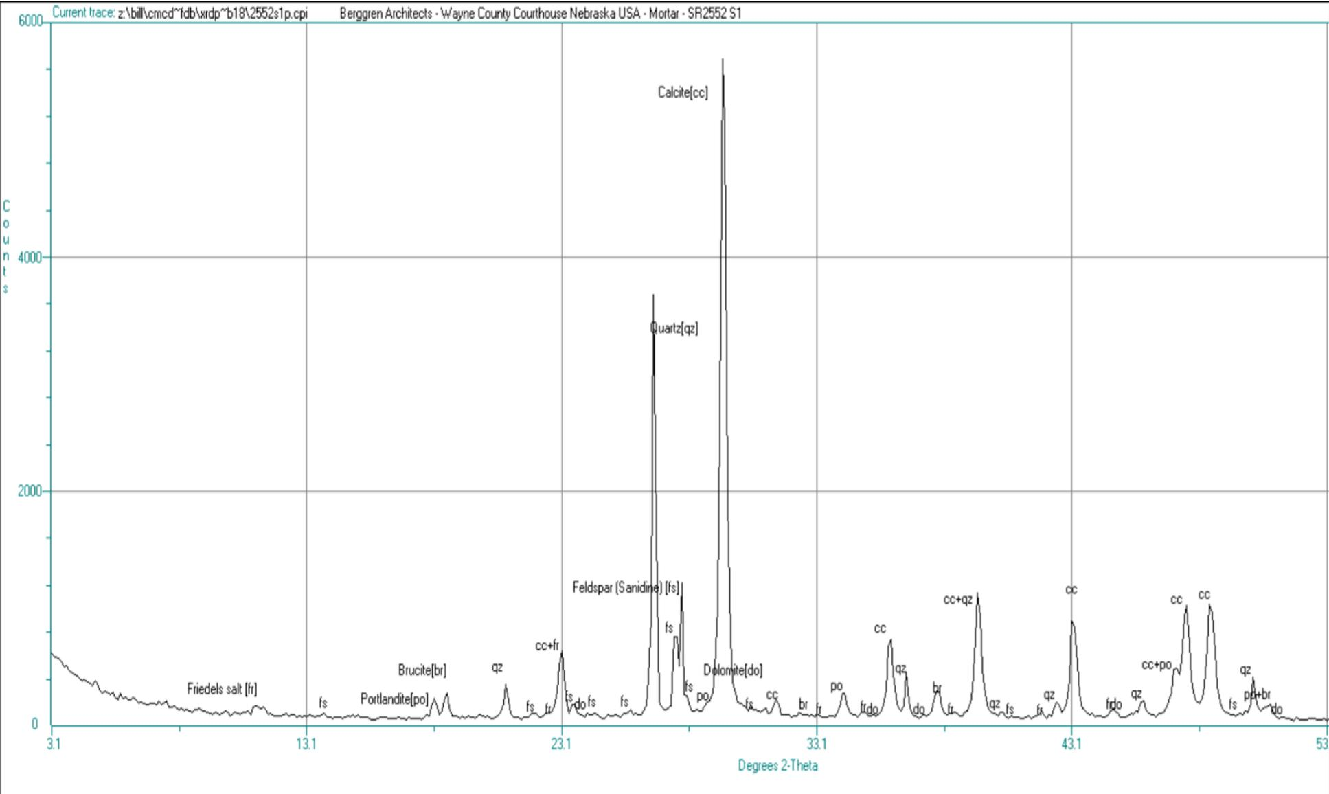
Figure No. 4 – SR2552-S1 – “Original” Grey bedding mortar, adhering to brick from Attic.
