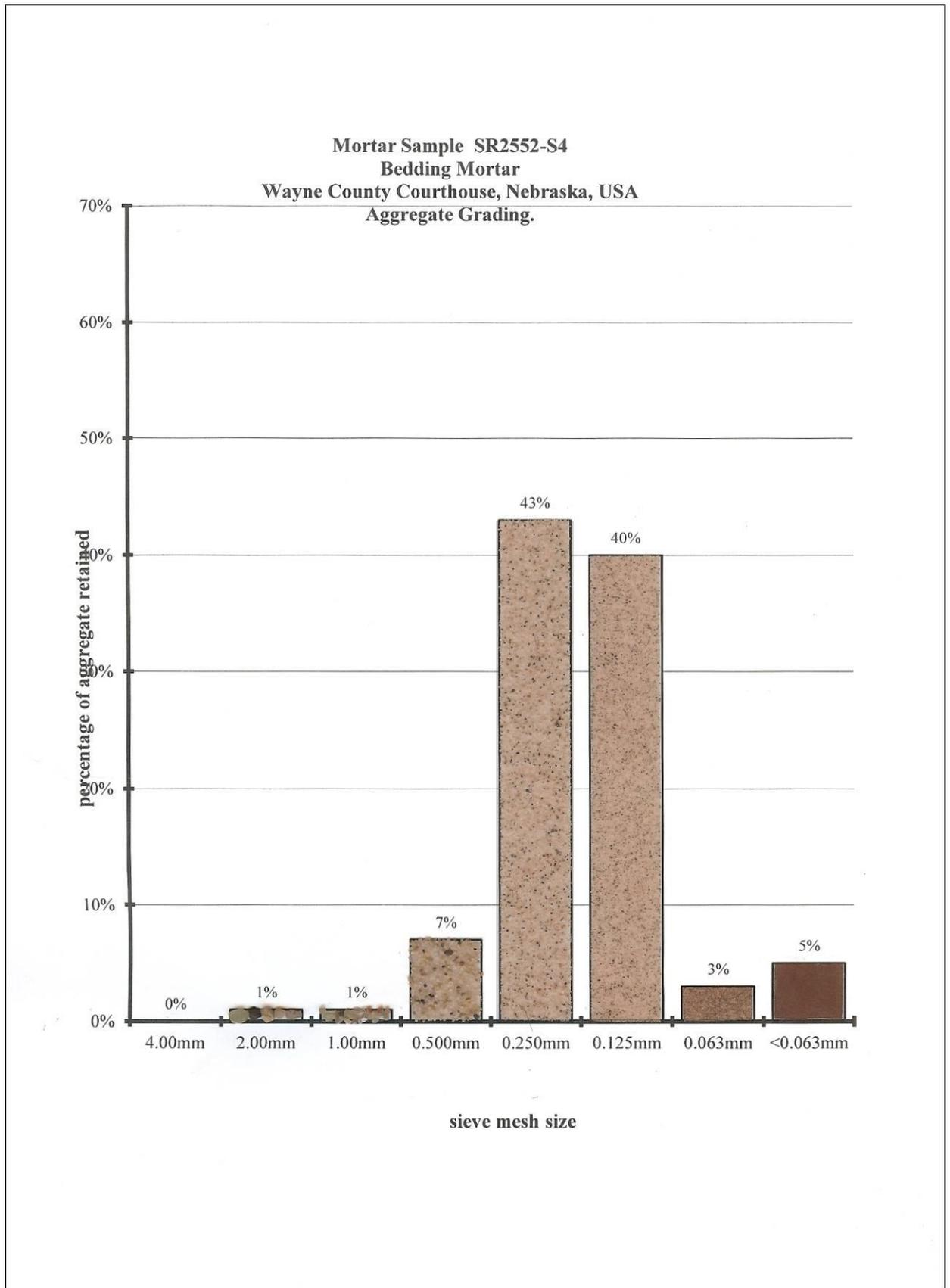
**Figure No. 2:** Grading of Aggregate from sample SR2552-S4
