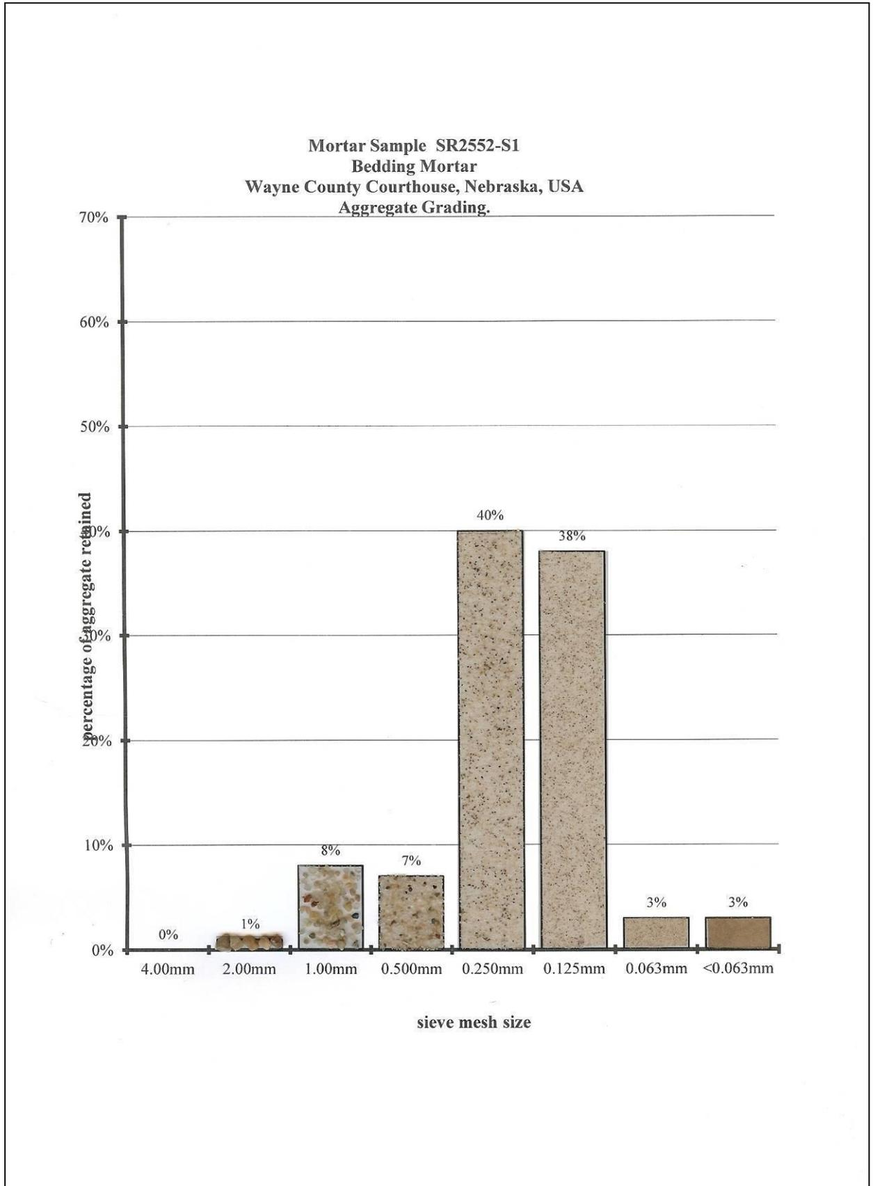
**Figure No. 1:** Grading of Aggregate from sample SR2552-S1
