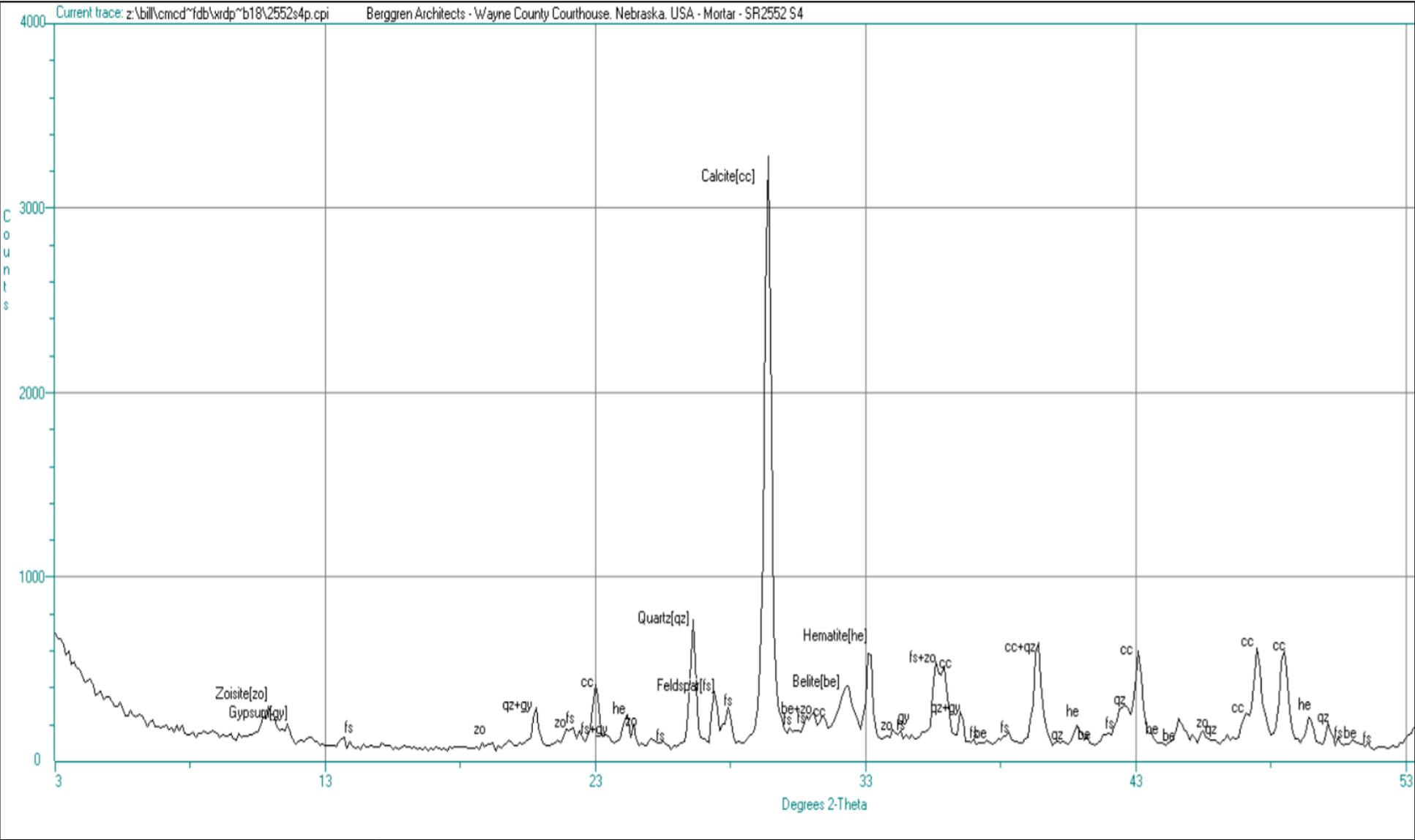
Figure No. 7 – SR2552-S4 – “Pink” Brick bedding mortar from inside column, on Tower.
