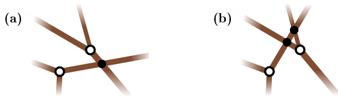
Figure 6.15: Detail of a layout, showing the importance of converting crossover joints to full joints between the MILP and GO stages when imposing a limit on the total number of joints. (a) Before geometry optimization, containing 3 joints in this region. (b) After geometry optimization, containing 4 joints in this region.
