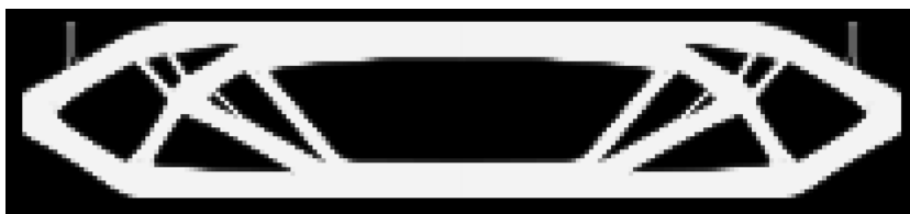
FIGURE 5: Basement transfer truss: continuum topology optimisation solution
