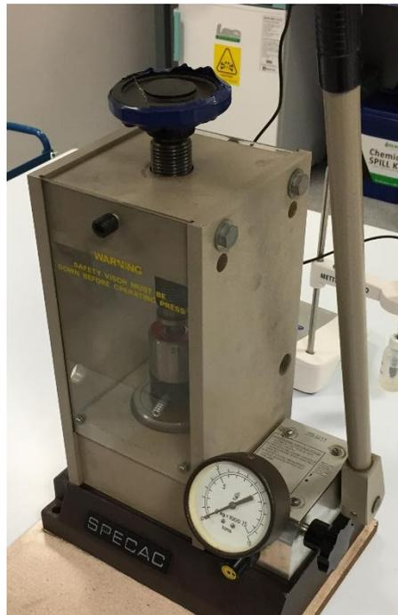
**Figure 8.4 SPECAC 15.011 laboratory manual hydraulic press**
