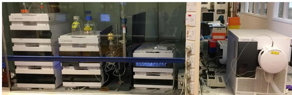
**Figure 8.20 Agilent 1260 Mass Directed Preparative HPLC**
