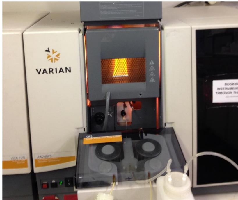
**Figure 8.6 Varian AA240FS atomic absorption spectrophotometer**
