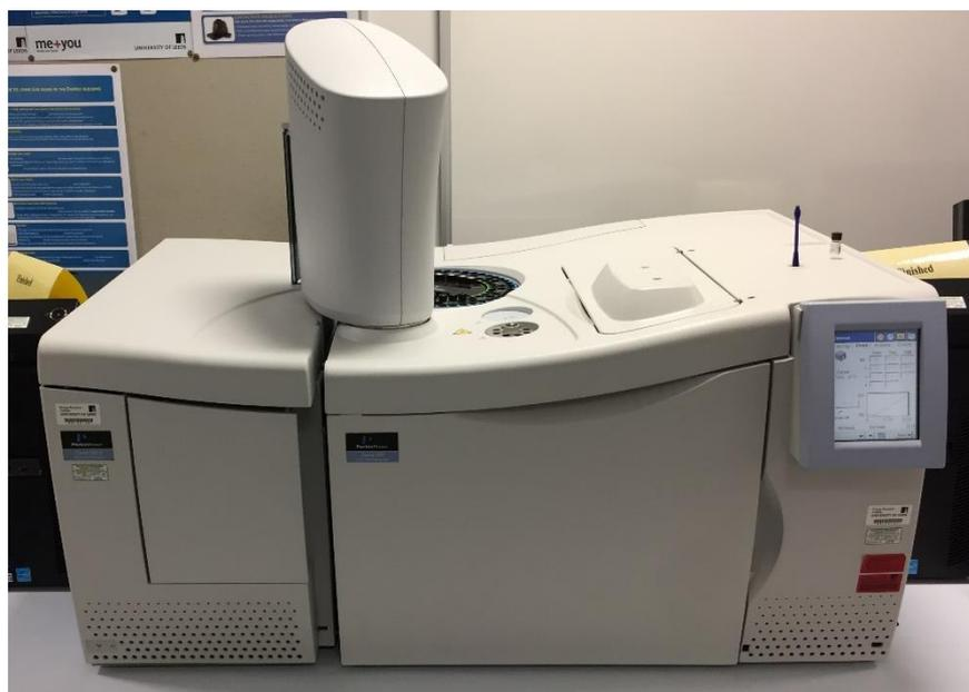
**Figure 8.12 Perkin Elmer Clarus GC-MS with autosampler**
