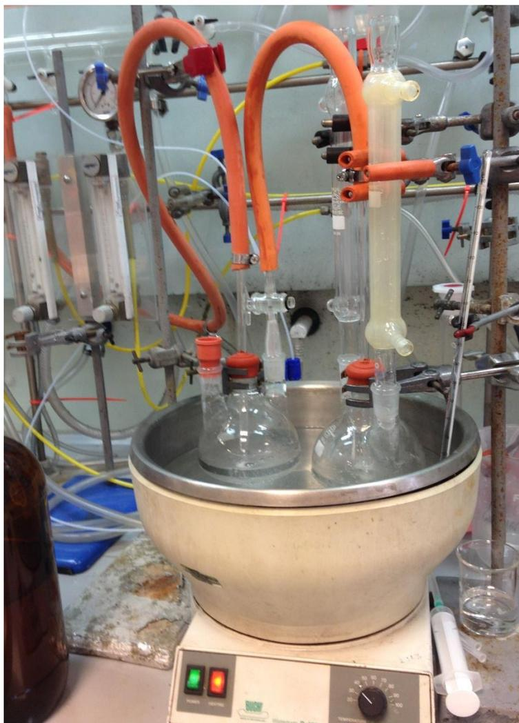
**Figure 8.18 Oxidative degradation apparatus set-up**
