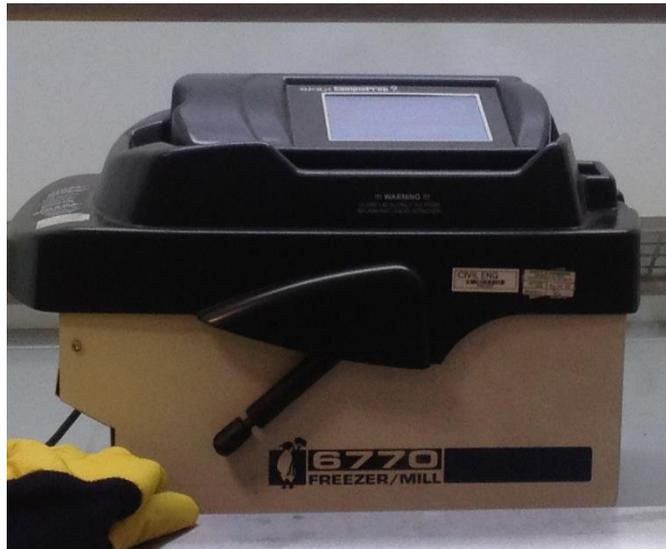
**Figure 8.3 SPEX 6770 freezer mill**
