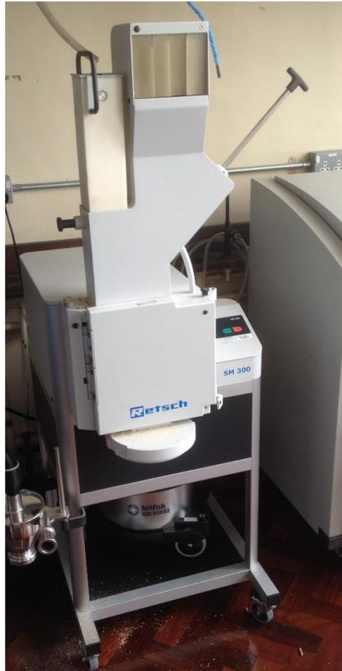
**Figure 8.2 Retsch SM300 Cutting Mill**
