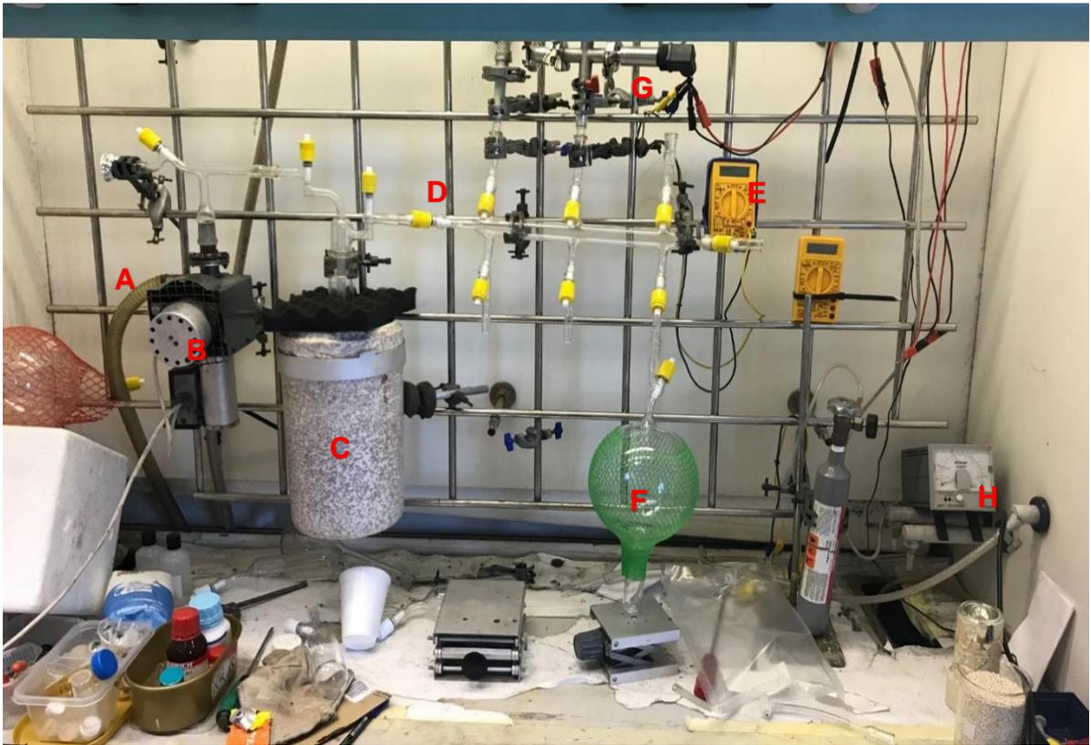
**Figure 4.20.** Photo of the gas handling line. (A) roughing pump bypass tap, (B) vacuum pump for low pressure ( $1 \times 10^{-3}$  mbar), (C) trap of liquid nitrogen, (D) the Schlenk line, (E) pressure gauge for higher pressures, (F) the glass balloon to be filled with sample, (G) a Pirani gauge and (H) Pirani gauge read-out unit for low pressures.
