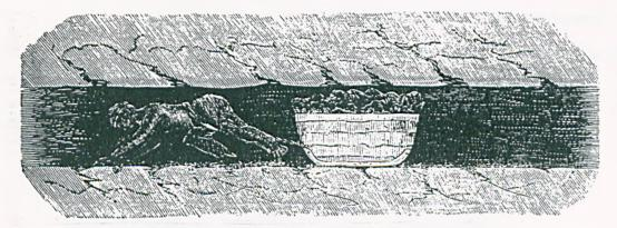
Drawing coal in a thin seam using a sledge (P.P. 1842, XVII, p. 475).
