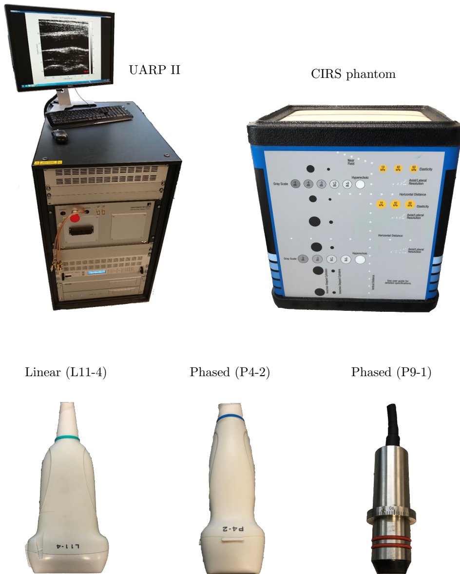
Figure 5.2: Images of the UARP II system, CIRS tissue-mimicking test phantom, and the three transducer probes used in this study: linear (L11-4), phased (P4-2), and waterproof-phased (P9-1).
