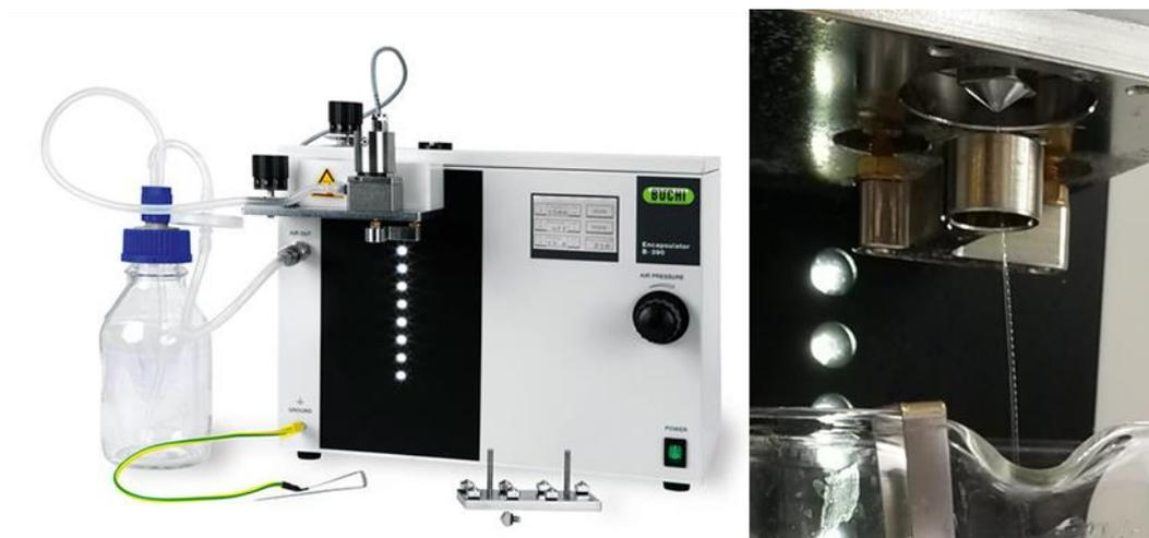
**Figure 3.5. Buchi Encapsulator<sup>®</sup> set-up (left) and dropping mechanism of the NaA solution into a water bath with Ca<sup>2+</sup> ions (right).**
