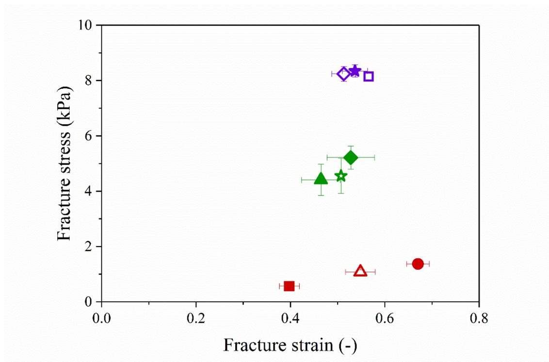
**Figure 3.7.** Mean ( $\pm$  SD) fracture stress and fracture strain of puncture tests with Volodkevitch probe of mixed  $\kappa$ C and LBG hydrogels, with concentrations 0.7 $\kappa$ C0.3LBG (●), 0.8 $\kappa$ C0.2LBG (△), 0.9 $\kappa$ C0.1LBG (■), 1.5 $\kappa$ C0.5LBG (☆), 1.67 $\kappa$ C0.33LBG (◆), 1.8 $\kappa$ C0.2LBG (▲), 2.25 $\kappa$ C0.75LBG (□), 2.5 $\kappa$ C0.5LBG (★) and 2.7 $\kappa$ C0.3LBG (◇).
