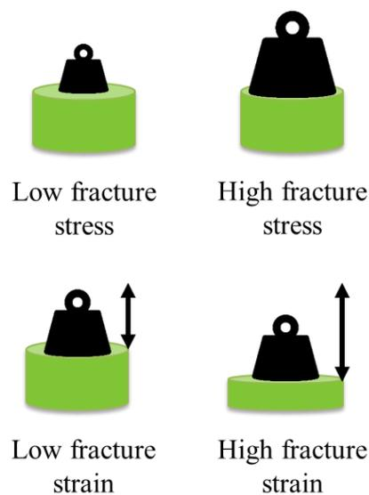
**Figure 1.2. Schematic representation of fracture stress and fracture strain.**
