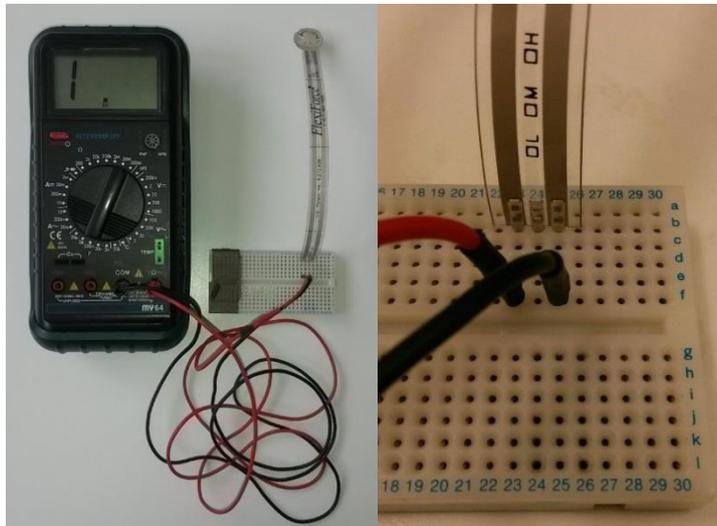
**Figure 1.11. Multi-meter and flexisensor with silicon disc for bite force measurements, connected through a bread board.**
