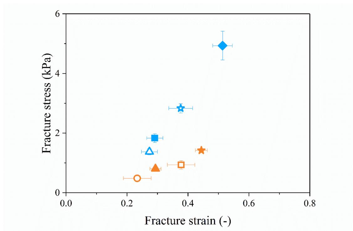
**Figure 3.8. Mean ( $\pm$  SD) fracture stress and fracture strain curve of puncture tests with Volodkevitch probe of mixed  $\kappa$ C and NaA hydrogels, with concentrations 1 $\kappa$ C1NaA ( $\circ$ ), 1.4 $\kappa$ C0.6NaA ( $\blacktriangle$ ), 1.5 $\kappa$ C0.5NaA ( $\square$ ), 1.8 $\kappa$ C0.2NaA ( $\star$ ), 1.5 $\kappa$ C1.5NaA ( $\triangle$ ), 1.8 $\kappa$ C1.2NaA ( $\blacksquare$ ), 2.25 $\kappa$ C0.75NaA ( $\star$ ) and 2.7 $\kappa$ C0.3NaA ( $\blacklozenge$ ).**
