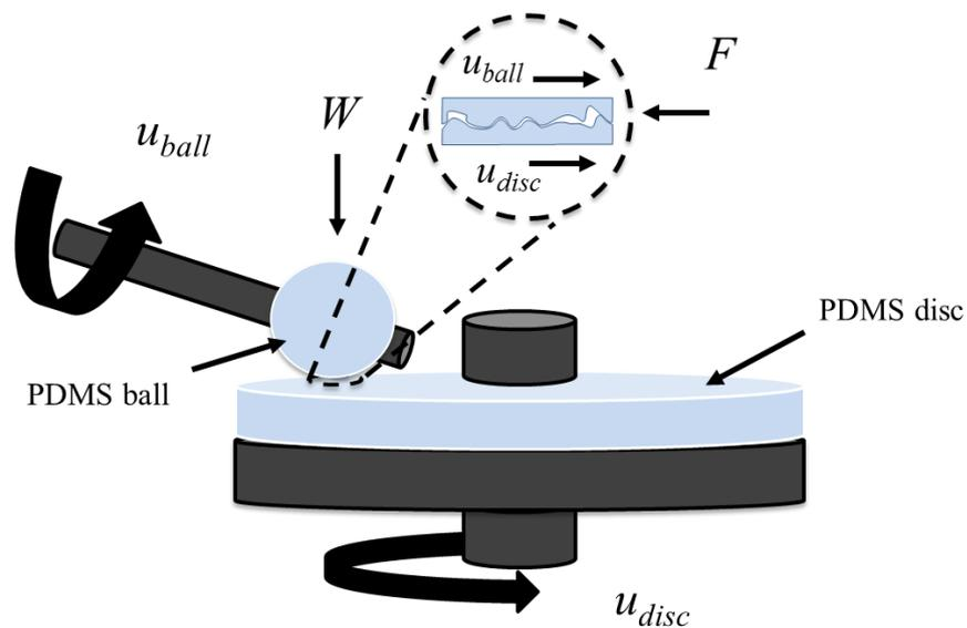
**Figure 1.6.** Schematic representation of a tribometer set-up, with  $W$  the applied contact load,  $u_{ball}$  and  $u_{disc}$  the ball and disc speed, respectively, and  $F$  the friction force.
