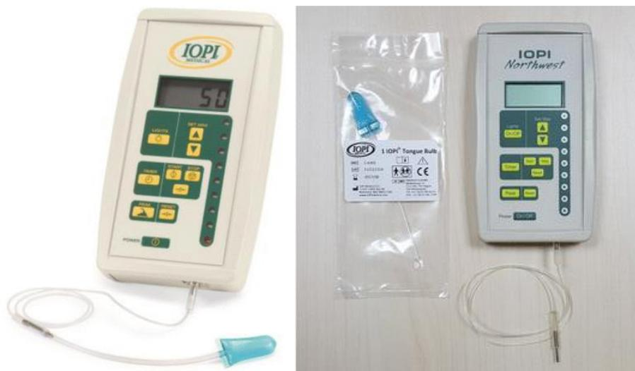
**Figure 1.12. The Iowa Oral Performance Instrument (IOPI) and tongue bulb used for tongue pressure measurements.**
