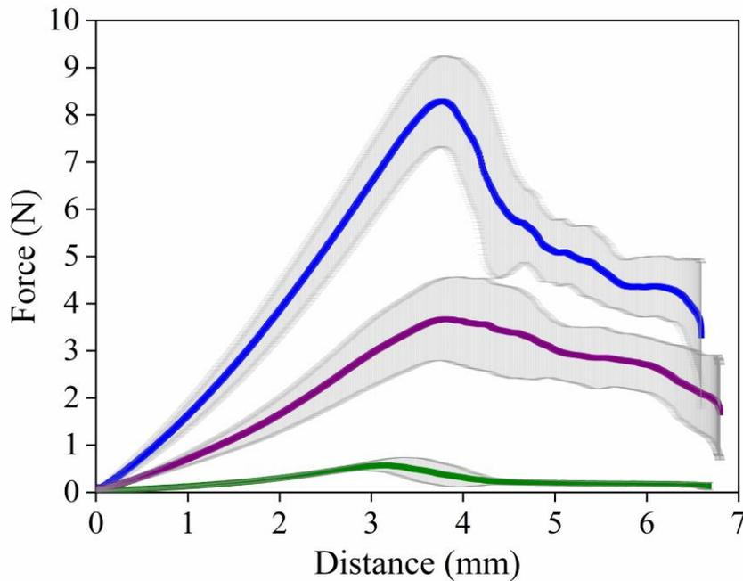
**Figure 5.1.** Mean ( $\pm$  SD) force over distance curve of the hydrogels obtained from puncture tests with a Volodkevitch probe (first bite), with 3 $\kappa$ C ( $\blacktriangle$ ), 1.5 $\kappa$ C0.5NaA ( $\blacklozenge$ ) and 2.4 $\kappa$ C0.2CaA<sub>300</sub> ( $\circ$ ).
