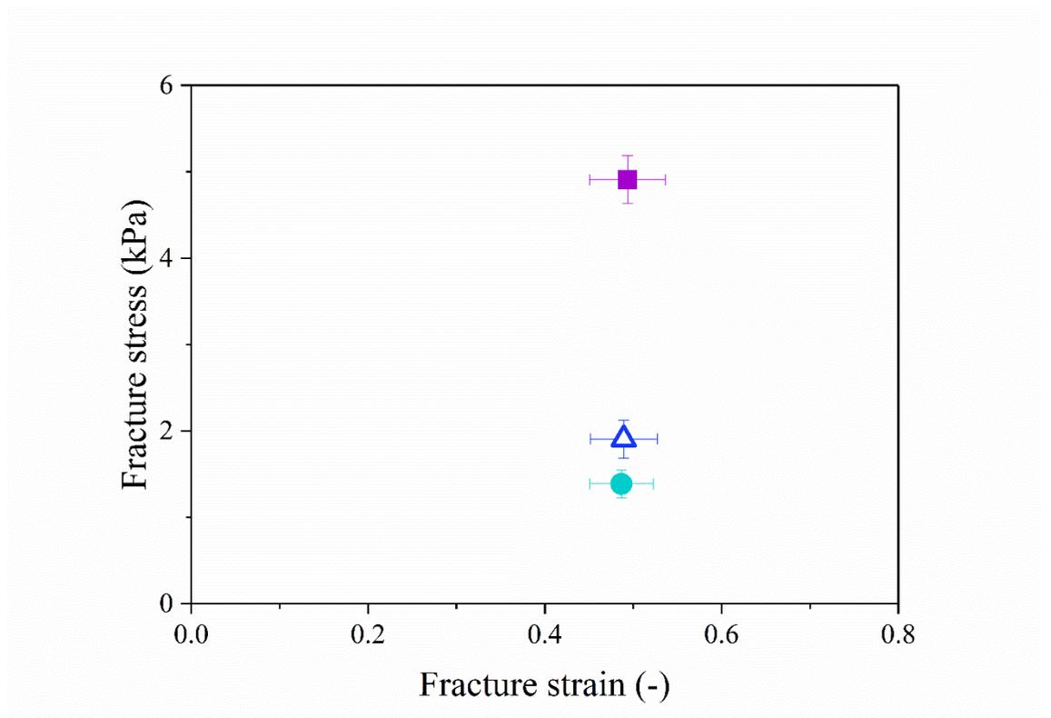
**Figure 3.9.** Mean ( $\pm$  SD) fracture stress and fracture strain curve of puncture tests with Volodkevitch probe of mixed  $\kappa$ C hydrogels of various concentrations and an added layer of CaA beads, with 1.6 $\kappa$ C0.2CaA<sub>300</sub> (●), 1.6 $\kappa$ C0.2CaA<sub>1000</sub> (△), 2.4 $\kappa$ C0.2CaA<sub>300</sub> (■).
