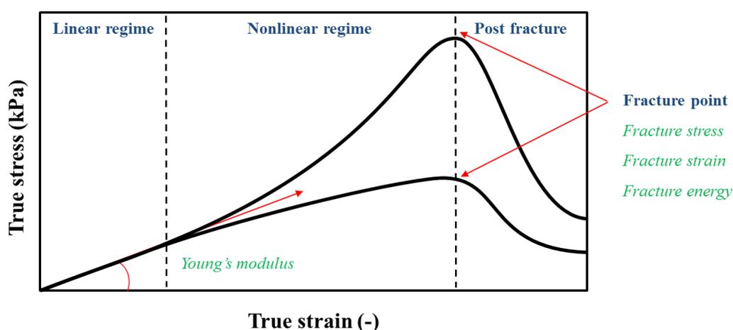
**Figure 1.3. Representation of typical stress strain curve of solid materials under large deformation, explaining the fracture behaviour (Koç *et al.* 2013).**
