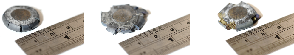
Figure 5.45: Two step deformation compression test samples, the second stage of deformation performed at 1150°C. Performed a strain rates of 0.01\text{s}^{-1} (left) 0.1\text{s}^{-1} (centre) 1\text{s}^{-1} (right).
