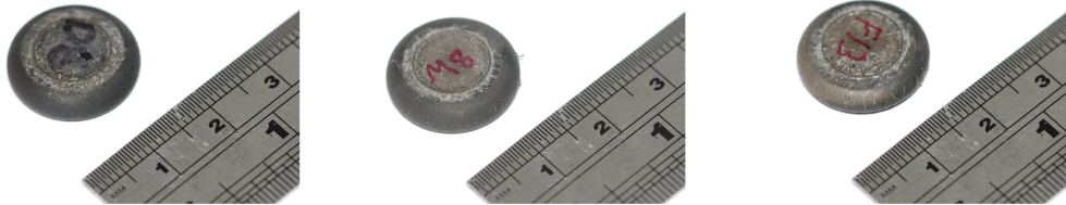
Figure 5.38: Photograph of samples post compression test on the Gleeble 3800 at strain rates of 0.01\text{s}^{-1} (left), 0.1\text{s}^{-1} (centre) and 1\text{s}^{-1} (right). All tests performed at 1100^\circ\text{C} .
