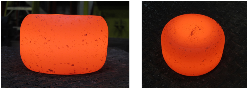
Figure 5.79: Large scale billet after a two hit deformation to a strain of 1.0, performed at 1100°C. Billet showed no cracks after deformation. The billet shown was named 3_2 in Table 5.12.
