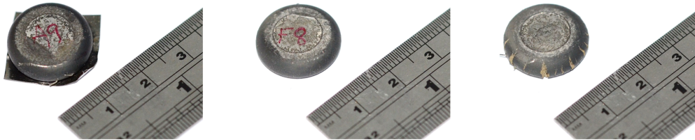
Figure 5.39: Photograph of samples post compression test on the Gleeble 3800 at strain rates of 0.01\text{s}^{-1} (left), 0.1\text{s}^{-1} (centre) and 1\text{s}^{-1} (right). All tests performed at 1125^\circ\text{C} .
