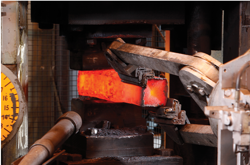
Figure 5.71: Close up image of the dies and work piece using the forging press located at Carpenter Technology Corporation Reading PA. Image Courtesy of Carpenter Technology.
