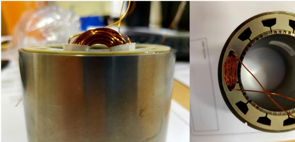
Figure 10.8. PDD single layer phase coil winding
