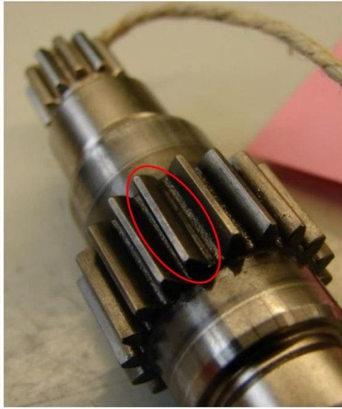
Figure 1.5. Gear wheel with tooth root crack [25]
