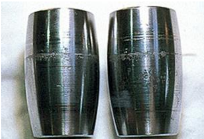
Figure 1.11. Bearing race spalling [30]
