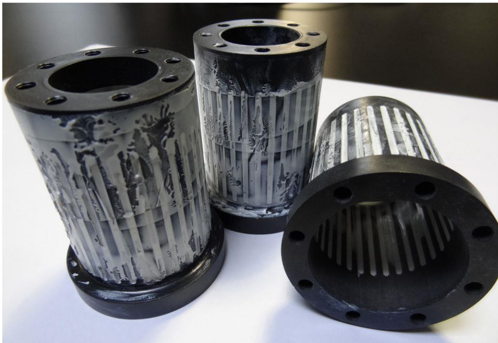
Figure 9.12. Assembled PEEK PPR with pole pieces
