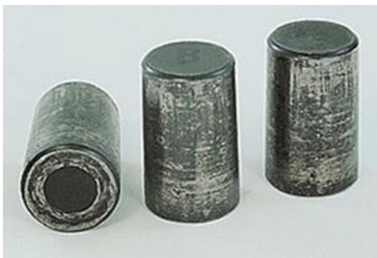
Figure 1.16. Bearing rollers removed from seized bearing [30]
