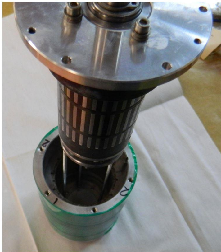
Figure 9.27. Final assembly of magnetic gear prototype
