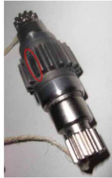
Figure 1.6. Gear wheel with broken tooth [25]
