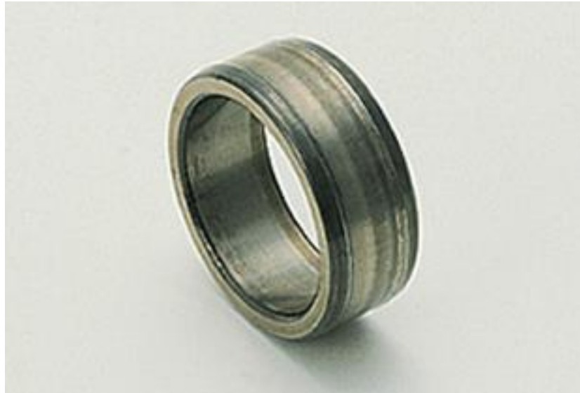
Figure 1.13. Roller bearing wear of inner race [30]
