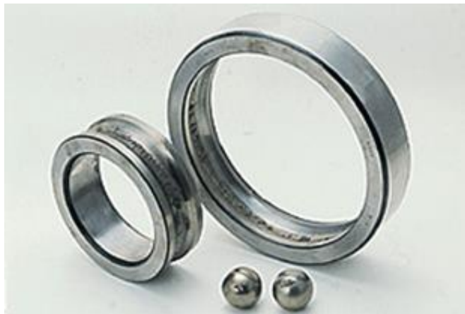
Figure 1.10. Flaking of ball bearings races [30]
