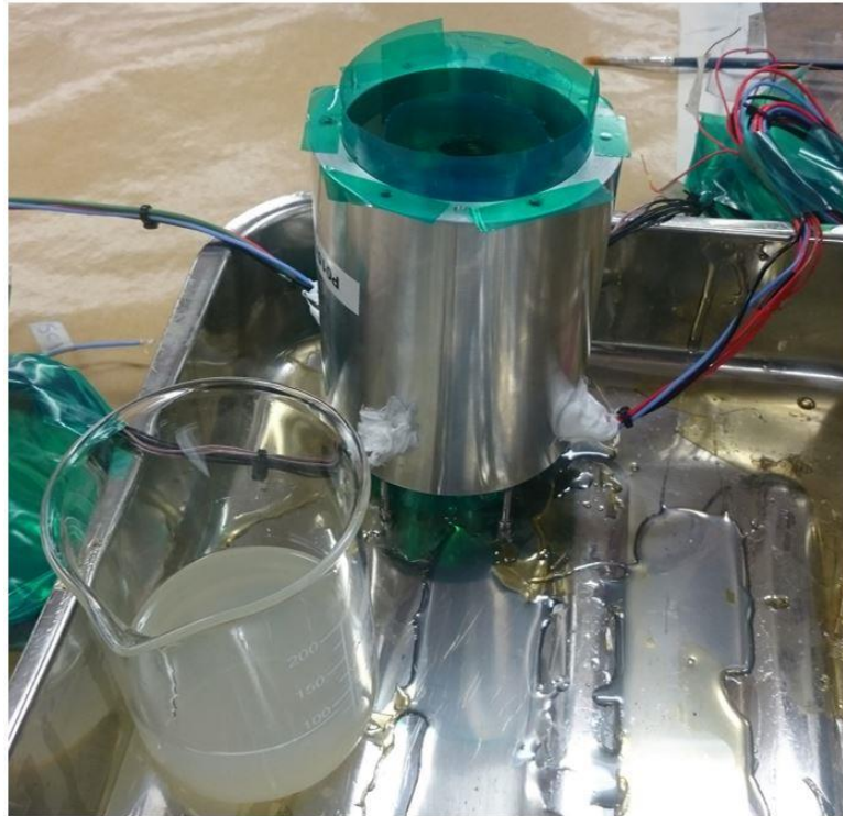
Figure 10.13. PDD stator in case during winding varnishing
