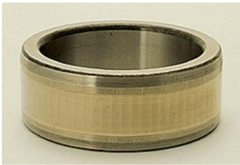
Figure 1.15. Bearing fretting caused by roller elements [30]
