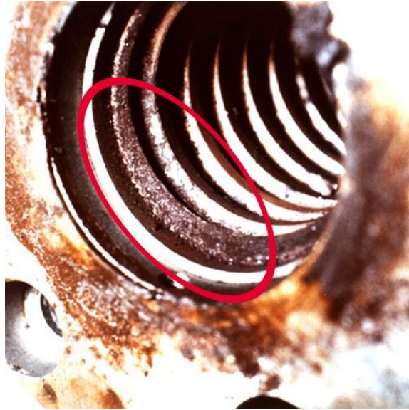
Figure 1.8. Wear of ball screw nut race [28]
