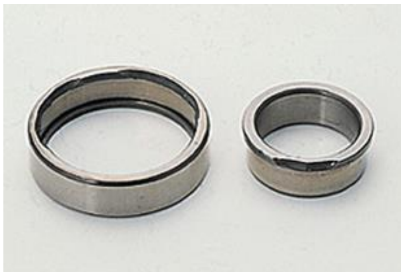
Figure 1.14. Roller bearing chipping of inner and outer guide rings [30]
