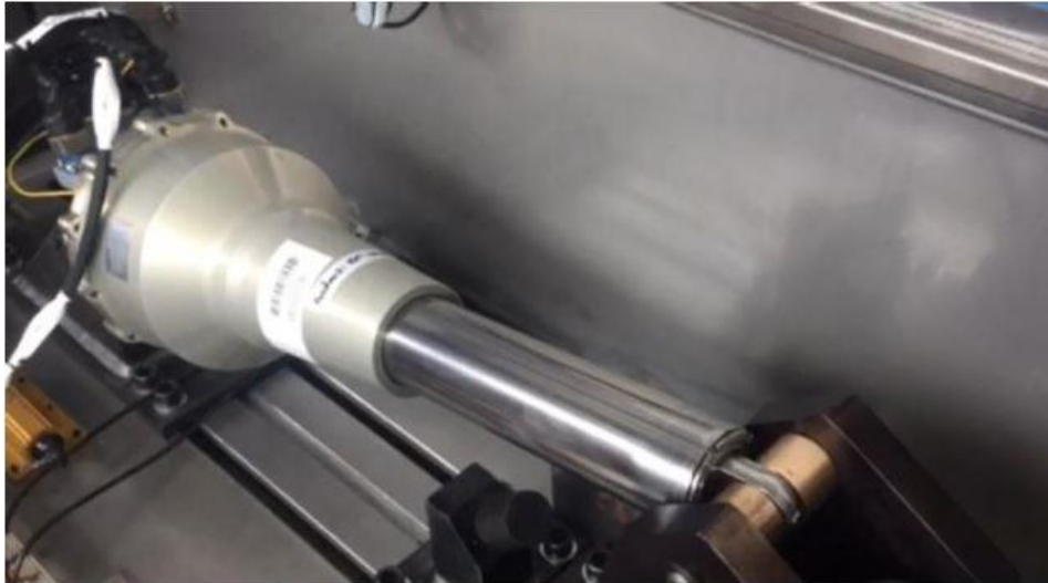
Figure 1.17. EMA extension under normal operating conditions [32]
