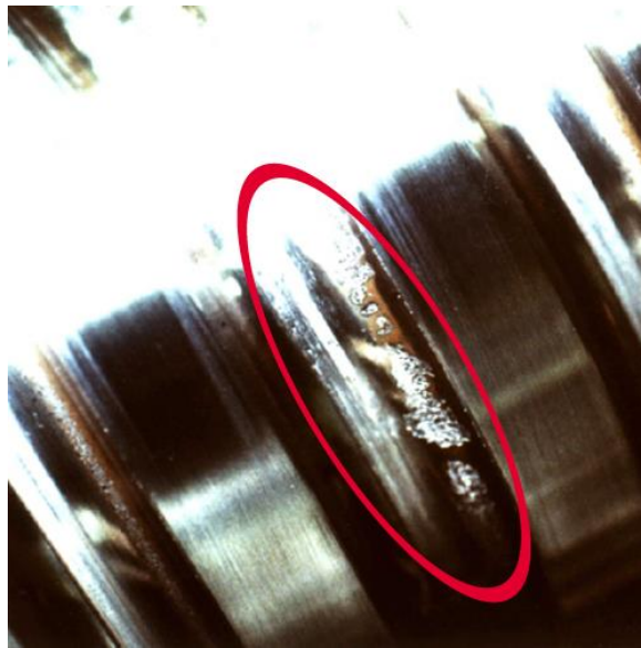
Figure 1.5. Gear wheel with tooth root crack [25]
