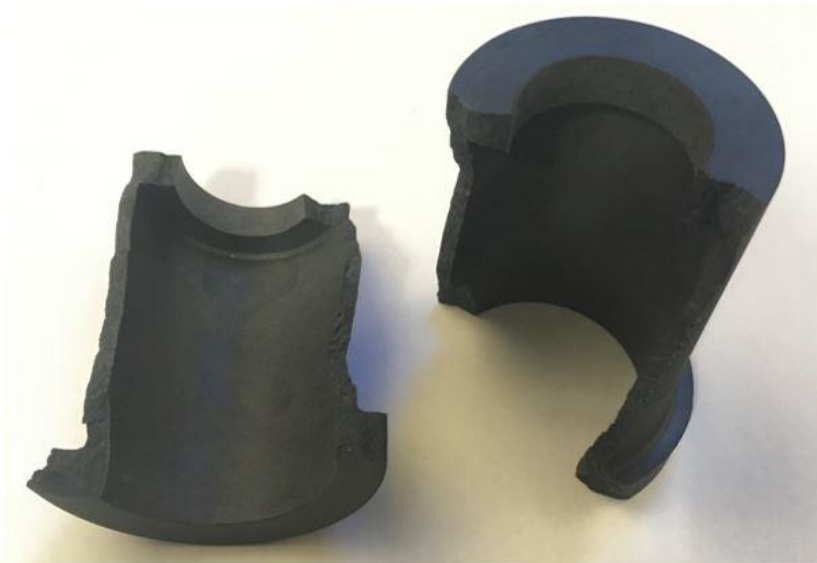
Figure 9.9. PEEK material failure during machining
