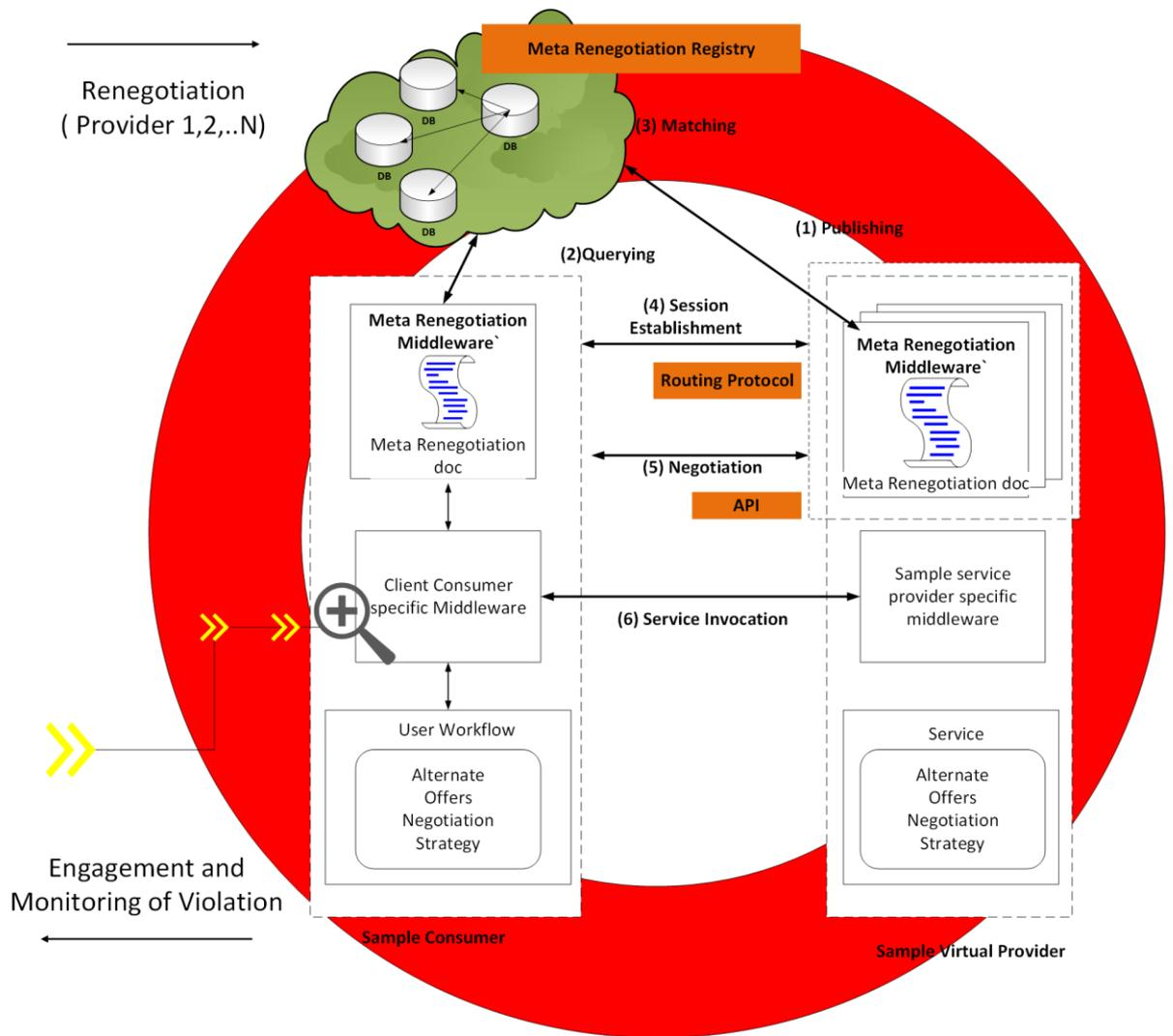
**Figure 3.20** Details of the renegotiation process within the self-adaptive brokerage architecture
