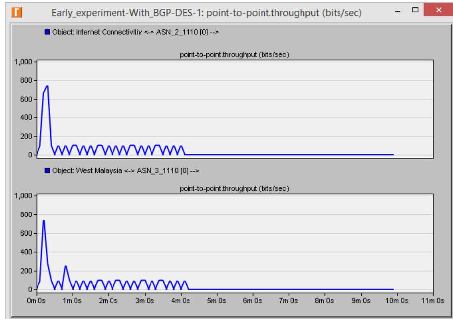
Figure 3.12 Point to point throughput – West Malaysia using BGP
