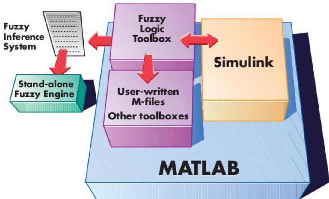
**Figure 3.2** Fuzzy Logic Toolbox within MATLAB
