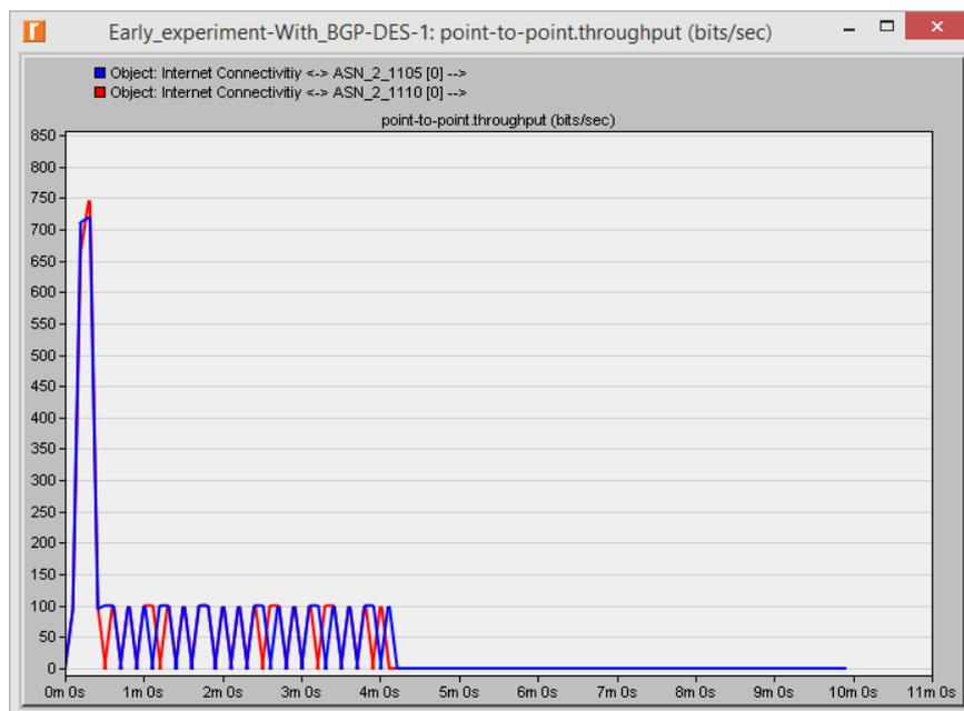
**Figure 3.14** Point to point throughput – West Malaysia using multiple BGP – (B)
