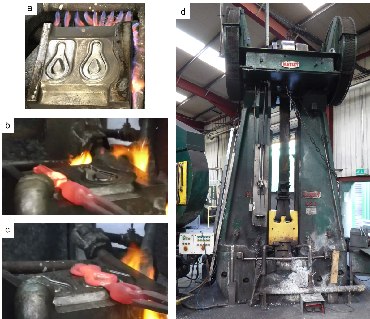
Figure 6.3: Closed-die multi-blow forging of the near-net shaped ‘eye bolt’ at W.H. Tildesley Ltd: (a) starter (left) and finisher (right) dies, (b) forged specimen after second blow on the starter die, (c) forged specimen after tenth blow on the finisher die, and (d) closed-die drop forge
