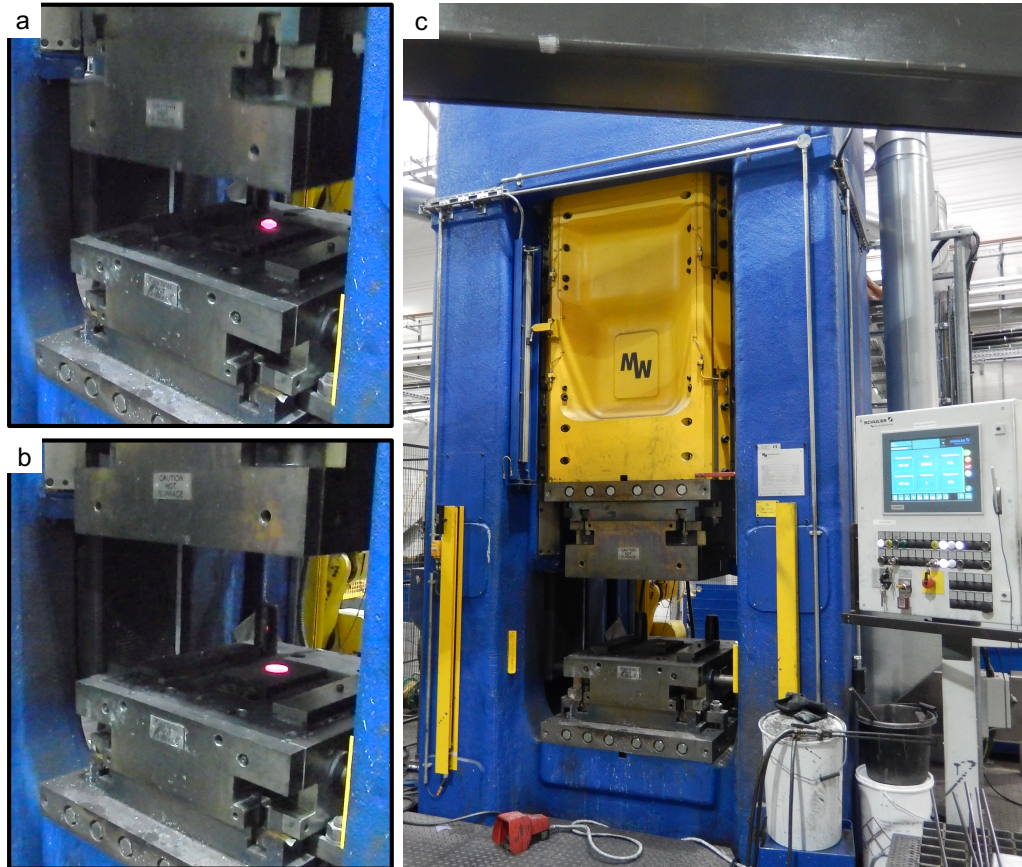
Figure 5.2: Photographs of large-scale forging of the double truncated cones (a) before forging and (b) after forging, and (c) the 2100 t screw press at the Advanced Forming Research Centre (AFRC) which was used for the large-scale forging
