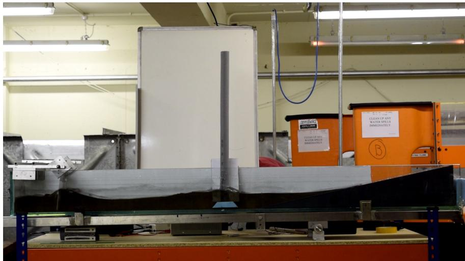
Figure 7.1: The wave tank set-up with a wave-maker (left), beach (right) and a beam.
