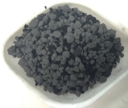
Figure 6.28 Photographic image of black and grey particles collected after first pass in the rotary kiln at 1173 K.
