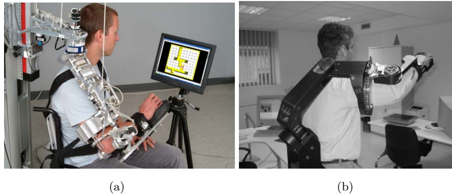
Figure 2.26: A patient training with the ARMin semi-exoskeleton rehabilitation robot (Nef et al. , 2007) (a) and a patient training with the L-Exos (Montagner et al. , 2007) (b).
