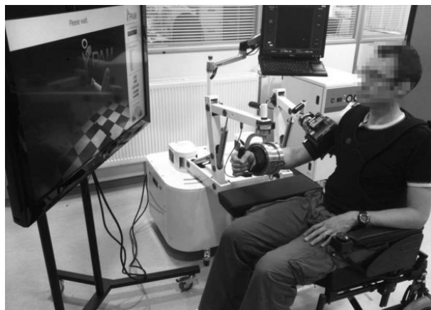
Figure 2.22: The iPAM pneumatically actuated dual robot rehabilitation system. Source: (Jackson et al. , 2013).
