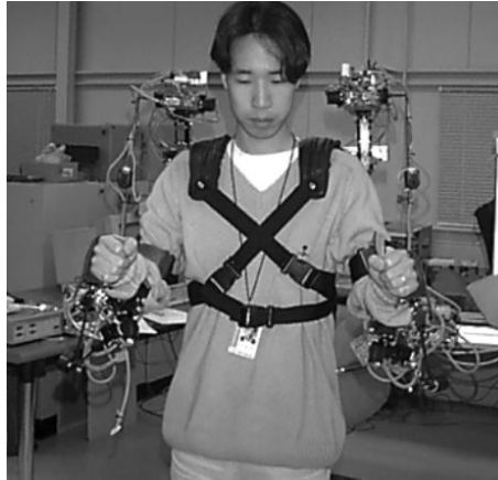
Figure 2.24: The exoskeleton-type master arm developed at KIST worn by a user (Kim et al. , 2005).
