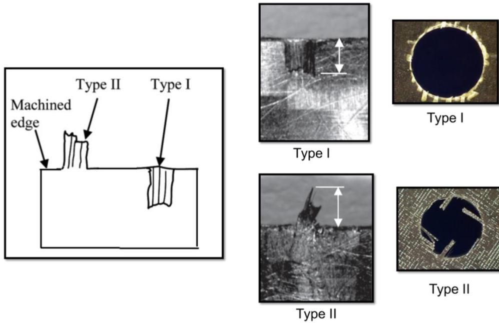
Figure 2-4- Type I and Type II delamination. Adapted from REF [3],[19]
