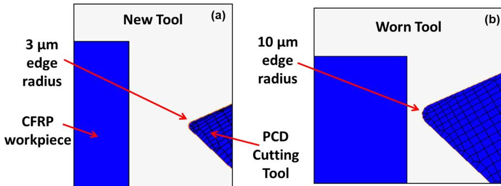
Figure 7-6- Worn and un-worn cutting tool 2D FE mesh:
