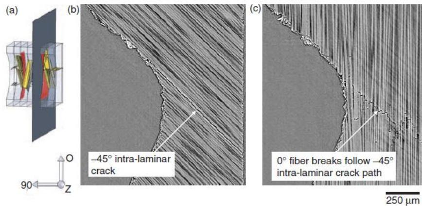
Figure 2-21 - Cross sections taken by SRCT through 45 and 0 degree ply. Showing crack paths through the material [66].
