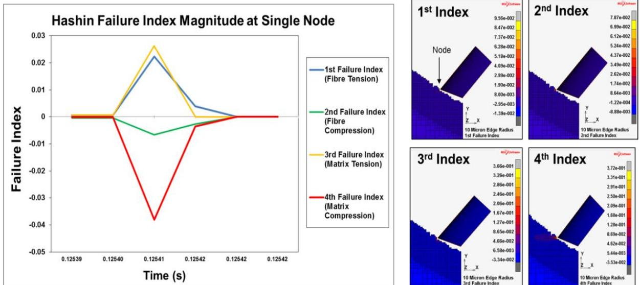
Figure 8-14- Hashin failure index at single node over successive increments leading to element failure. (90 degree fibre orientation, 10  $\mu\text{m}$  edge radius, 800 mm/min Feed and 6000RPM)
