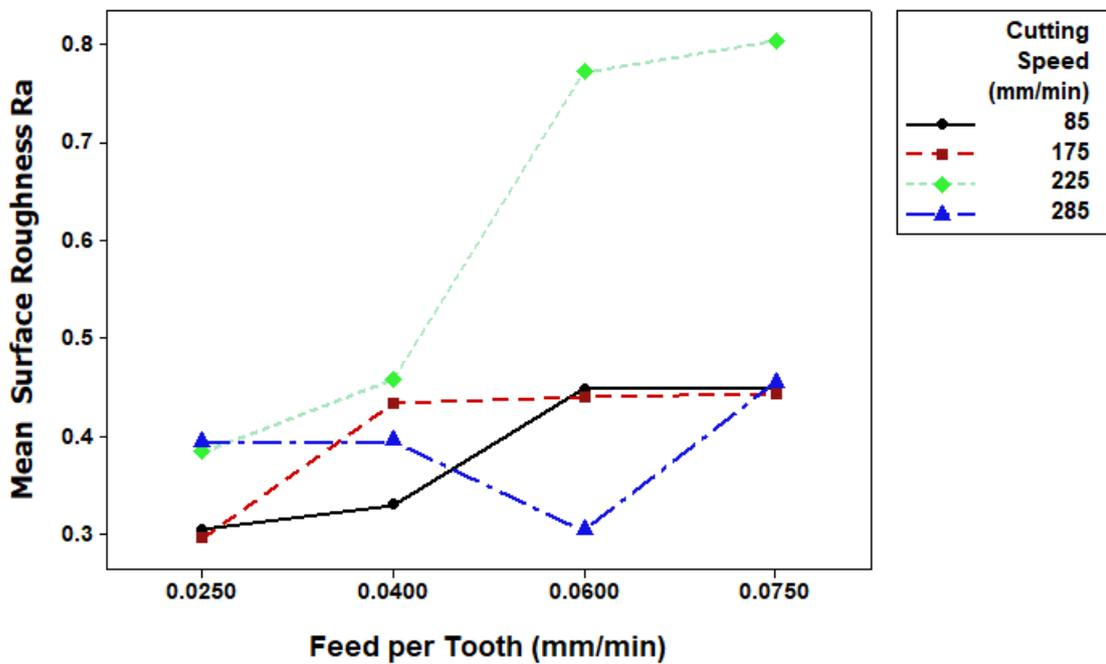
Figure 3-12- Mean  $R_a$  surface roughness for 135 degree fibre orientation, against feed rate grouped at each cutting speed.
