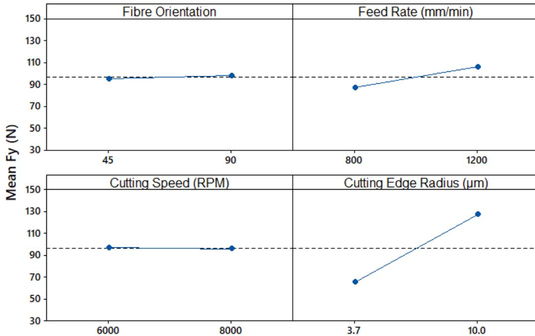
Figure 5-15- Main effects plot for mean  $F_y$  thrust force unidirectional test.
