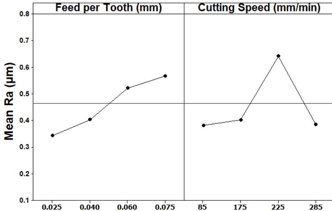
Figure 3-13- Main Effects for mean roughness for 90 degree fibre orientation, against feed rate and each cutting speed. Shown for multidirectional laminate and optical technique.
