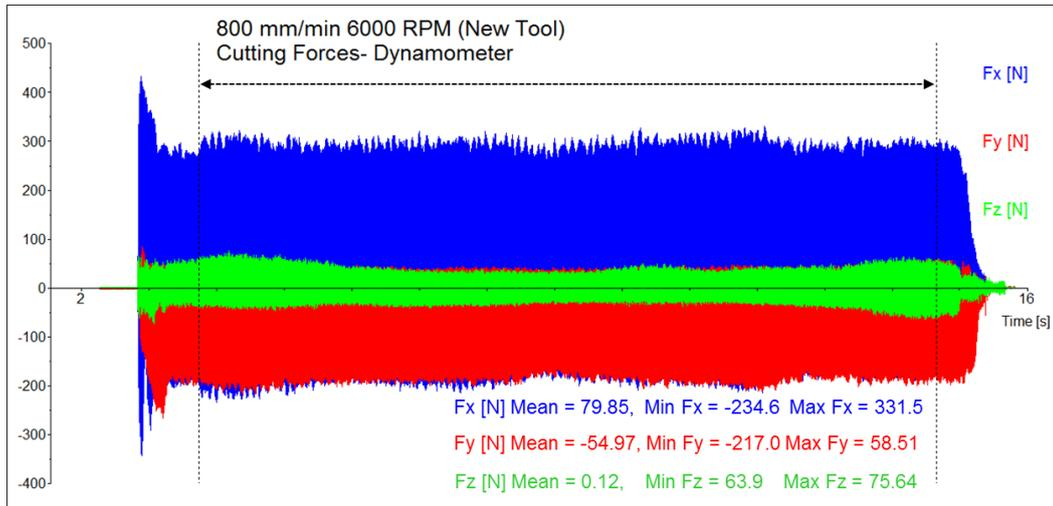
Figure 5-1- Dynamometer output for machining forces at 800 mm/min, 6000 RPM with new tool. Calculation of mean cutting forces.
