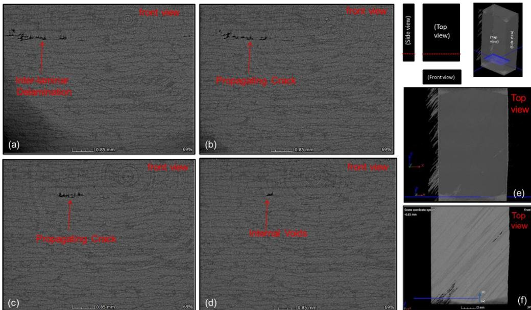
Figure 5-34- CT scans of delamination propagation from machined edge of unidirectional 45 degree fibre orientation laminate.
