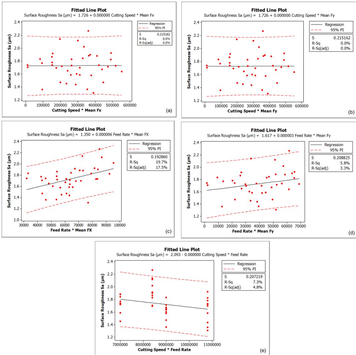
Figure 6-3- Fitted line plot for interaction variables effect on surface roughness, shown with 95 % confidence interval: (a) Cutting speed \* Mean Fx, (b) Cutting Speed \* Mean Fy, (c) Feed Rate \* Mean Fx, (d) Feed Rate \* Mean Fy, (e) Cutting Speed \* Feed Rate.
