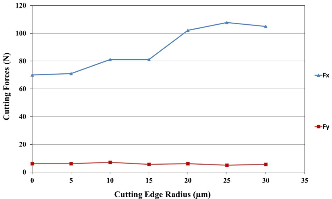
Figure 8-10- Effect of an increasing cutting edge radius on Fx and Fy from FE model. (45 Degree Fibre Orientation, 1200 mm/min & 6000 RPM).
