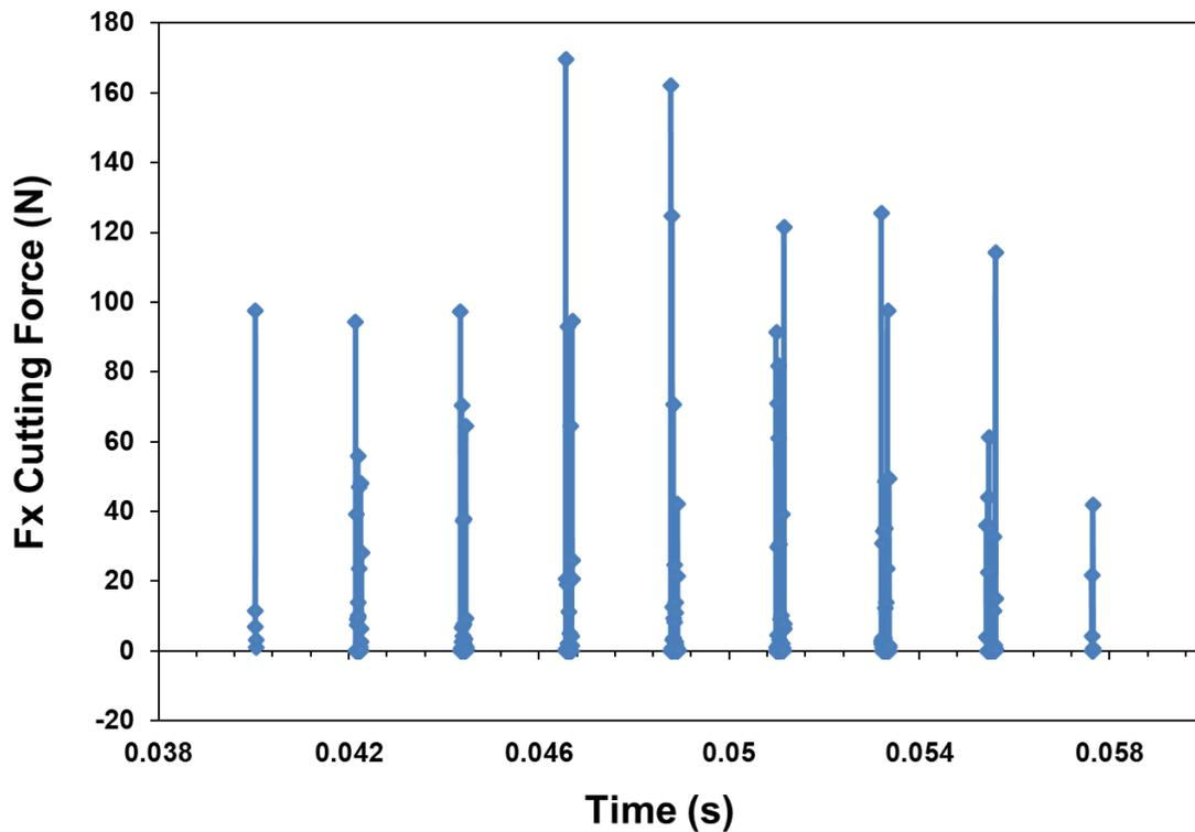
Figure 8-21- 3D FE model cutting forces (Fx). vs Time
