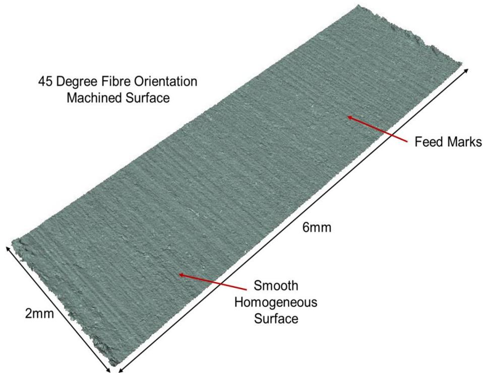
Figure 5-11- Optical surface scan unidirectional laminate. (45 degree fibre orientation, worn tool, 800 mm/min, 6000 RPM).
