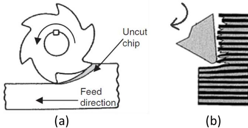
Figure 2-8 – (a) Change in chip dimensions during conventional milling [3], (b) Rotation of the cutting edge will vary against fibre orientation [26].
