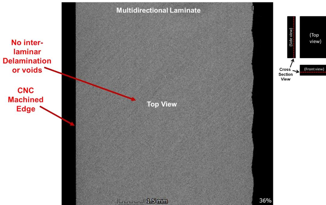
Figure 5-38- Multidirectional laminate- top view showing no internal interlaminar-delamination.
