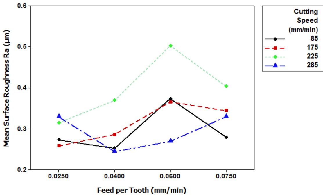
Figure 3-10- Mean  $R_a$  surface roughness for 45 degree fibre orientation, against feed rate grouped by cutting speed.
