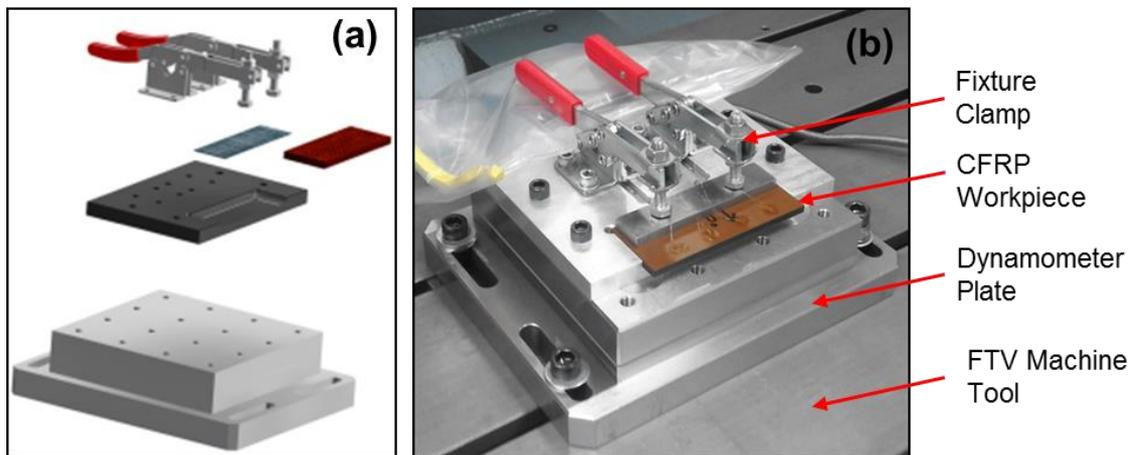
Figure 4-3- Experimental set up
