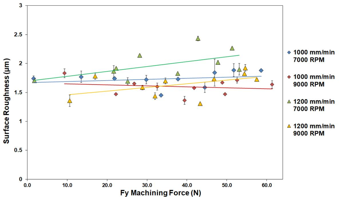
Figure 5-30- Surface roughness ( $S_a$ ) vs  $F_y$  machining force from experiment. Grouped by applied cutting speed and feed rate.
