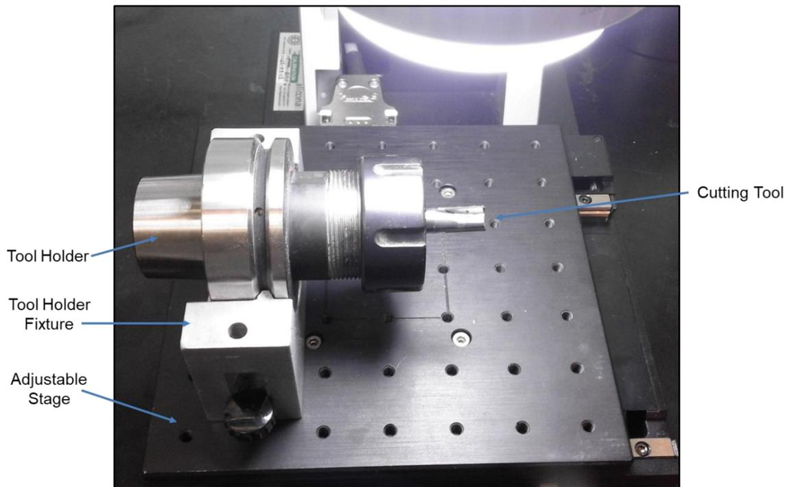
Figure 4-6- Tool holder fixture for CER measurements.
