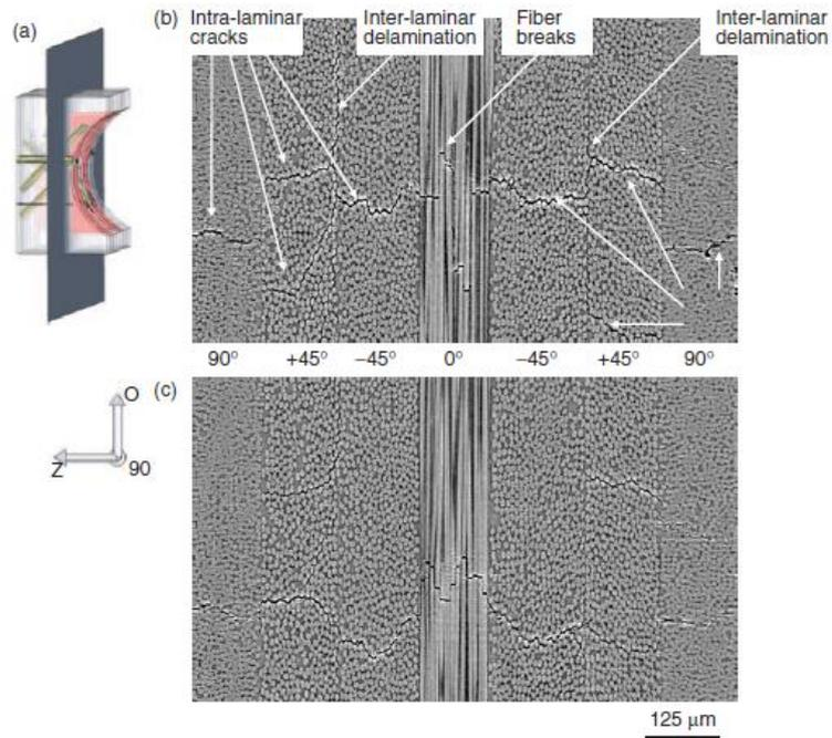
Figure 2-20- Two cross section images taken by SRCT ahead of crack notch. Showing Inter-laminar delamination and intra-laminar cracks [66].
