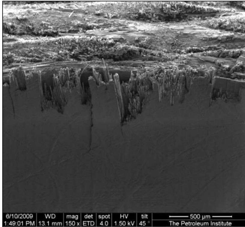
Figure 2-11- SEM image of type I/II delamination on edge machined at extreme cutting conditions [19].
