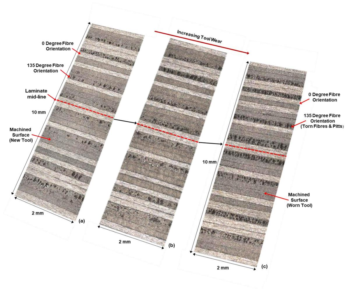
Figure 5-17- Machined Surface Optical scans from focus variation system of multidirectional laminate. . Images show a 3D surface image of the machined surface profile texture at increasing tool wear. The full laminate thickness of 10mm is shown.
