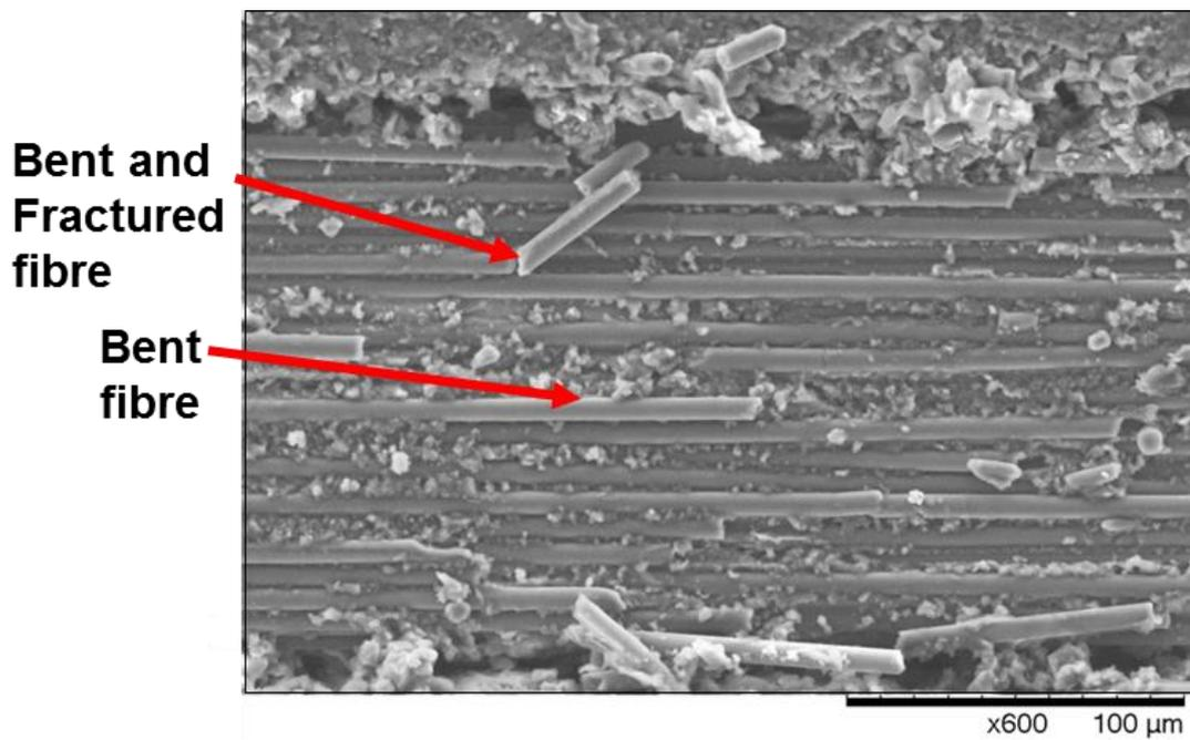
Figure 3-23- A 0 Degree fibre orientation, multidirectional laminate, experimental test 2. (These tests are on multidirectional laminate, SGS tool, Feed 1200 mm/min, 7000RPM)
