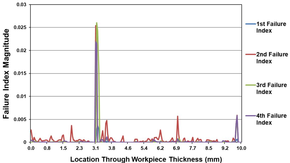
Figure 8-33-Through thickness of 3D model Hashin failure index damage.
