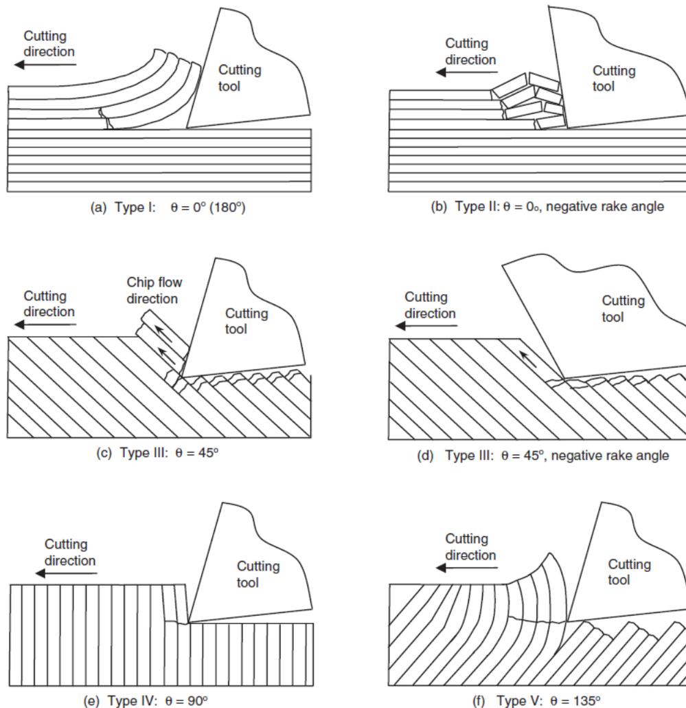
Figure 2-6 - Cutting mechanisms at different fibre orientations. Adapted from REF [3],[21].
