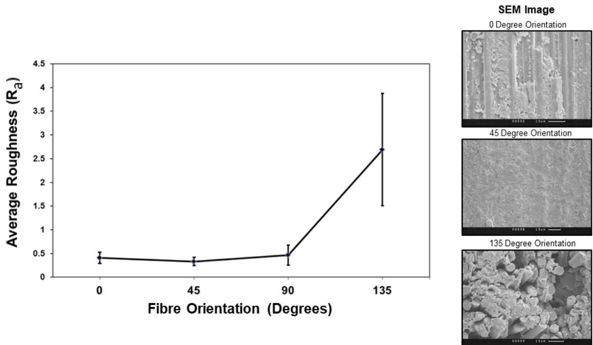
Figure 3-8- Average roughness vs fibre orientation on multidirectional laminate, with error bars shown as standard deviation using optical technique. SEM images of fibre orientation machined surface are shown for reference.
