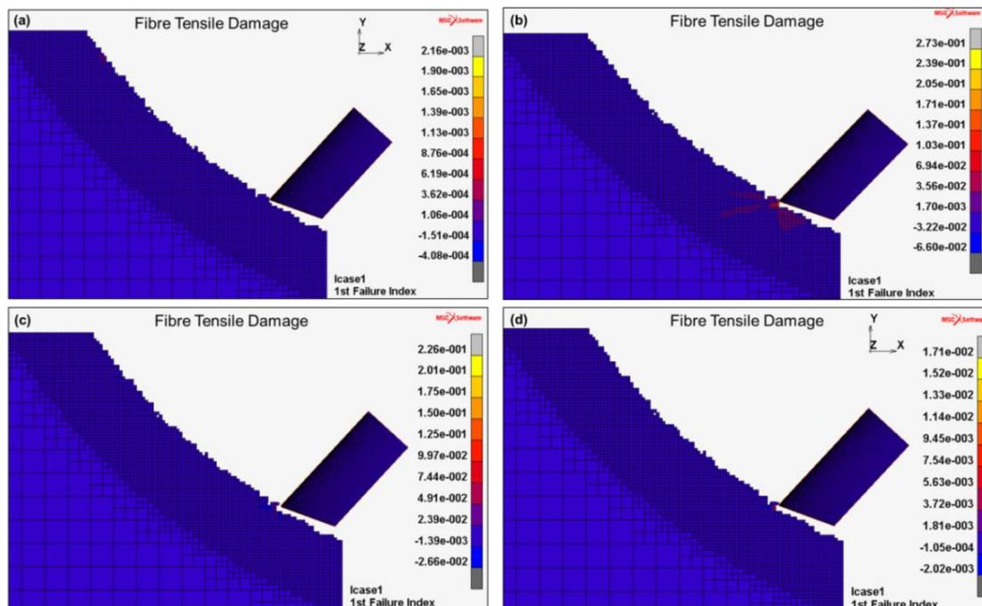
[Figure 8-12](#)- Tensile fibre failure magnitude (1st Failure index), over subsequent increments. (90 degree fibre orientation, 10 $\mu$ m edge radius, 800mm/min Feed and 6000RPM)
