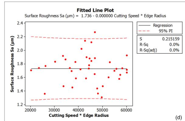
Figure 6-2- Fitted line plot for interaction variables effect on surface roughness, shown with 95 % confidence interval: (a) Mean Fx \* Edge Radius, (b) Mean Fy \* Edge Radius, (c) Feed rate \* Edge Radius, (d) Cutting Speed \* Edge Radius.
