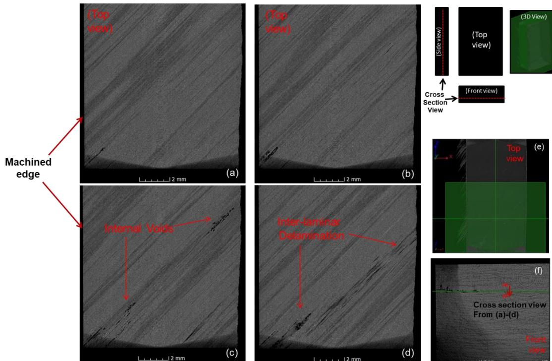
**Figure 5-33- Inter-laminar Delamination propagating through thickness shown from the top view of the unidirectional laminate, machined at 45 degree fibre orientation.**
