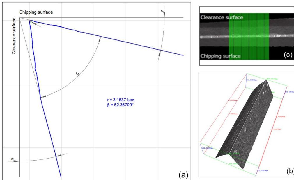
Figure 4-7- Cross section tool cutting edge mean parameters calculation-optical device (new tool).
