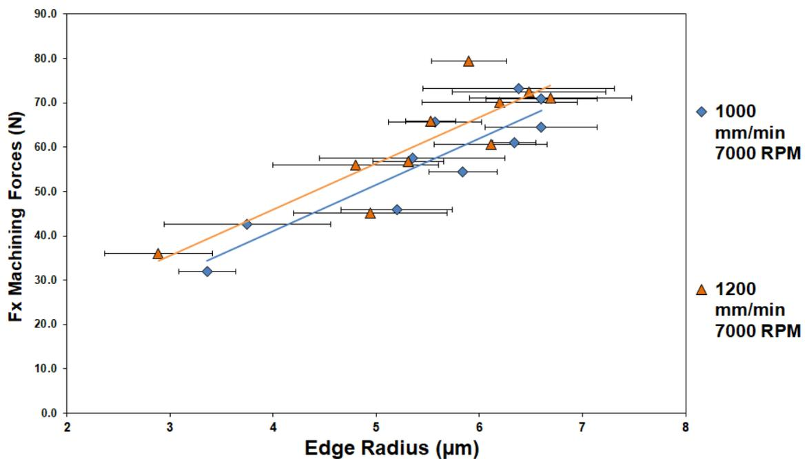
Figure 5-22-  $F_x$  Cutting forces against increasing edge radius at 7000 RPM. The error bars represent standard deviation in the edge radius measurement from 3 cutting edges.
