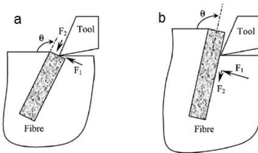
Figure 2-7 - Cutting mechanism at positive fibres orientation at small and large depth of cut. Adapted from REF [18].
