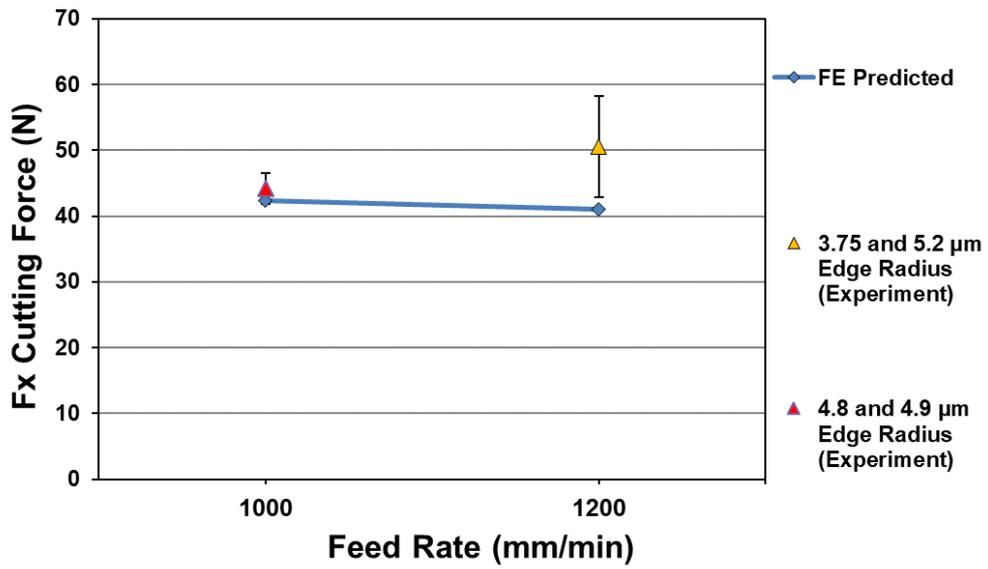
Figure 8-23- Experimental and FE model Fx cutting forces vs increasing feed at 7000 RPM.
