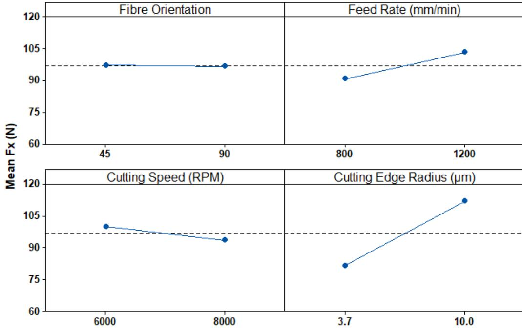
Figure 5-14- Main effects plot for mean Fx cutting force unidirectional test.
