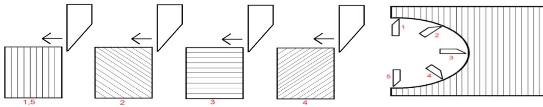
Figure 2-9- Slot milling, cutting tool edge to fibre orientation. Adapted from REF [18].
