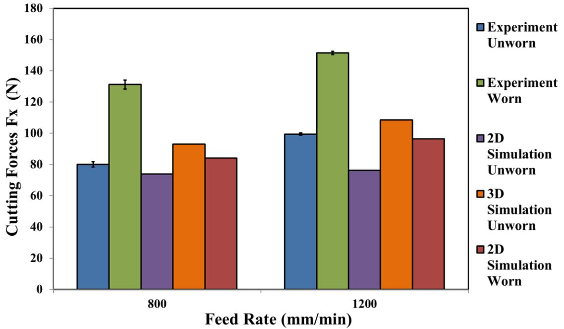
Figure 8-6- Fx cutting forces vs feed rate from experimental and FE for 90 degree fibre orientation at 6000 RPM.
