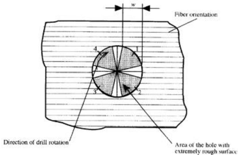
Figure 2-15 - Variation in roughness at different points on hole surface due to fibres orientation [38].
