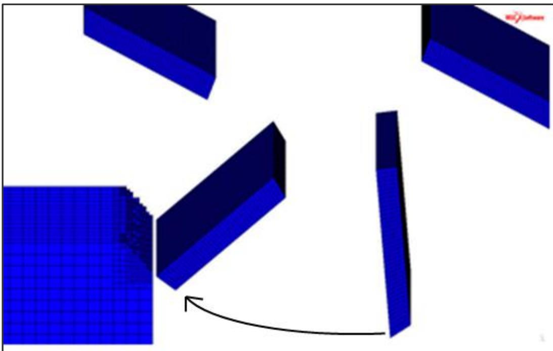
Figure 8-2- 3D Edge trimming simulation with composite elements and advancing adaptive meshing.
