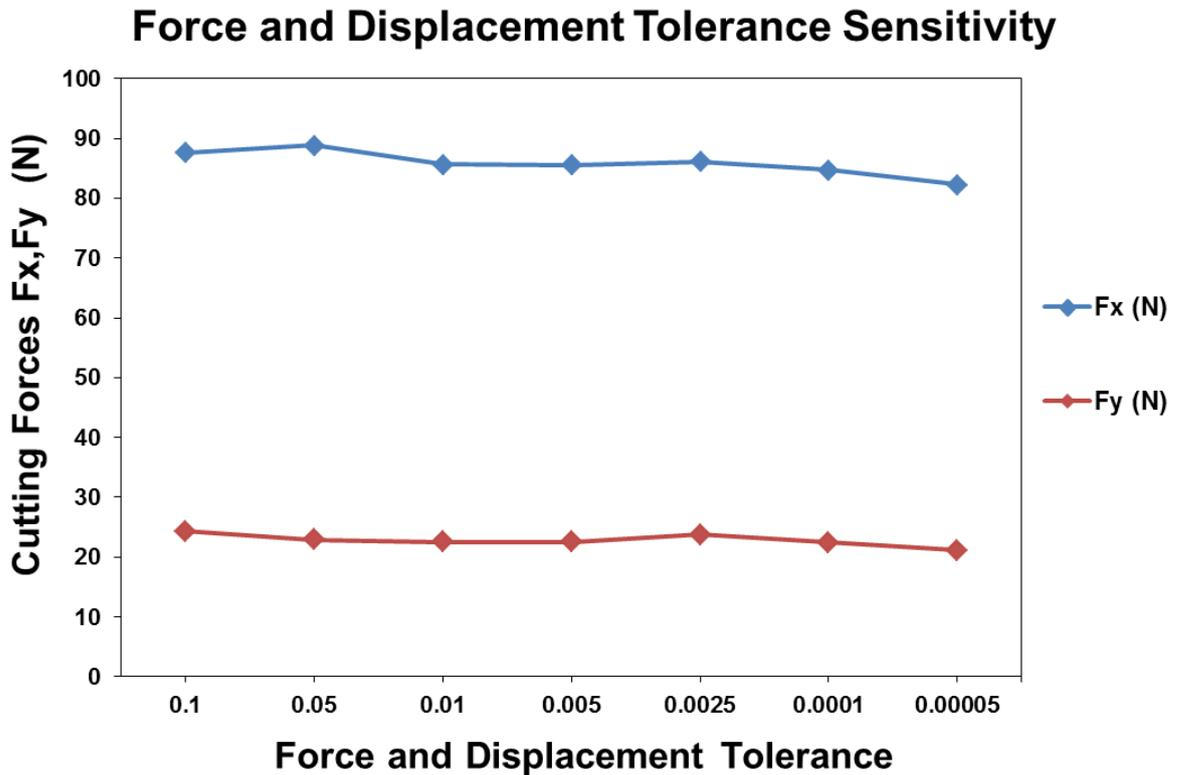
Figure 8-20- A convergence test for force and displacement tolerance sensitivity.
