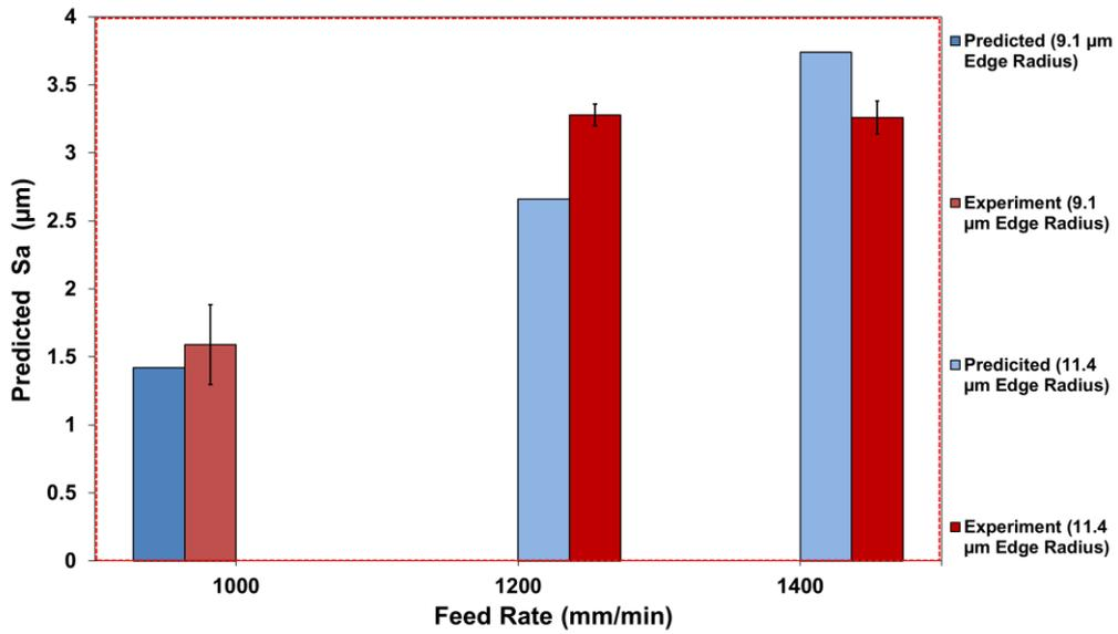
Figure 8-30- Experimental vs predicted  $S_a$  surface roughness at increasing feed rate at constant 11000 RPM. Error bar represents standard deviation between set of test results.
