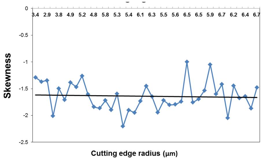
Figure 8-36- The 135 degree fibre orientation, change in skewness vs increasing cutting edge radius.
