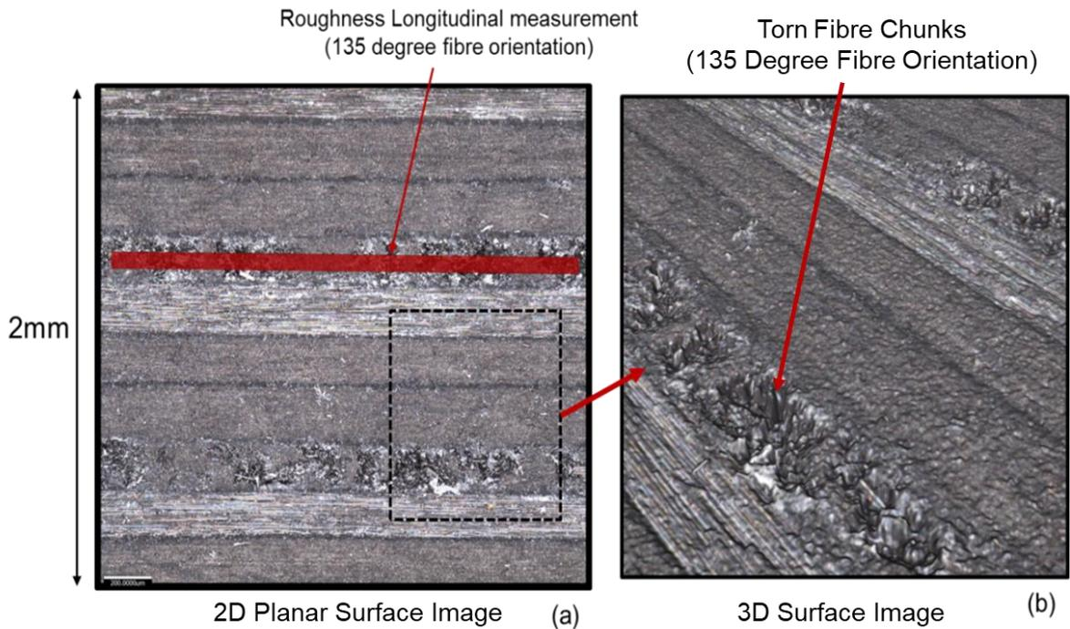
Figure 3-5- Optical focus variation surface scan of machined surface.
