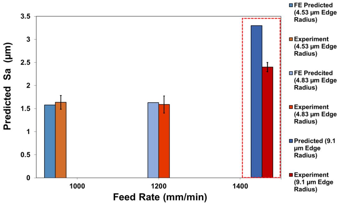
Figure 8-29- Experimental vs predicted  $S_a$  surface roughness at increasing feed rate at constant 9000 RPM. Error bar represents standard deviation between averaged set of test results with a different edge radius.
