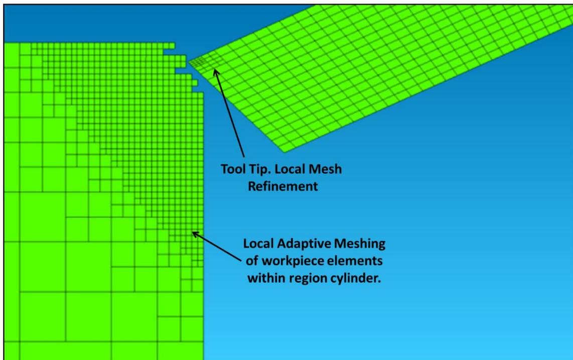
Figure 7-5- Local adaptive re-meshing of workpiece and tool tip.
