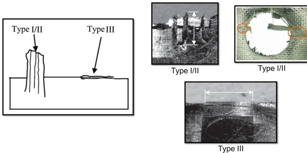
Figure 2-5- Type I/II and Type III delamination. Adapted from REF [3],[19]
