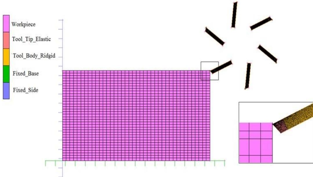
[Figure 7-1- 2D Milling simulation showing tool tip and fixed boundary conditions.](#)
