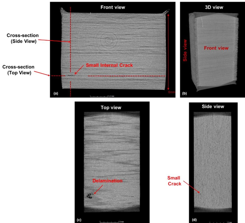
Figure 5-37- CT scans 90 degree fibre orientation, un-machined sample.
