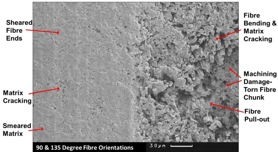
Figure 3-17- SEM image of 90 and 135 degree ply.
