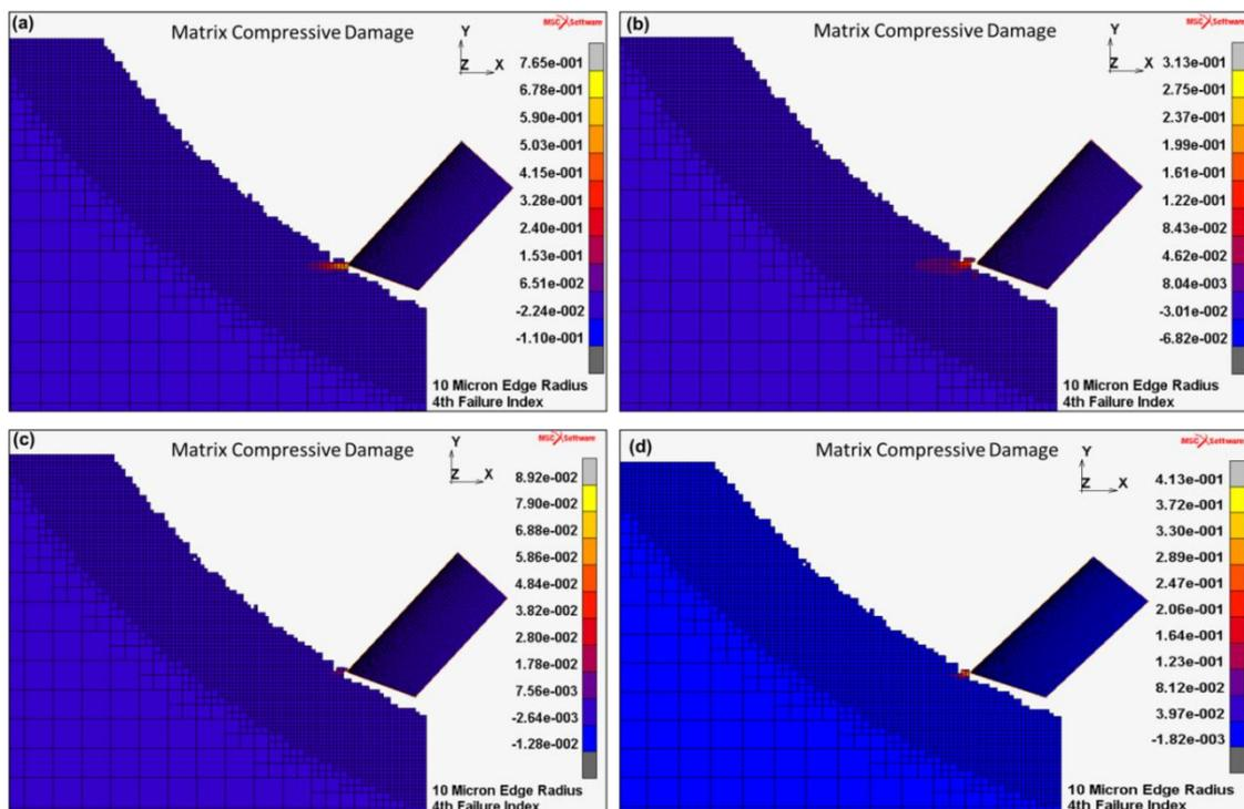
Figure 8-13- Matrix compressive failure magnitude (4th Failure index), over subsequent increments. (90 degree fibre orientation, 10 $\mu$ m edge radius, 800mm/min Feed and 6000RPM)
