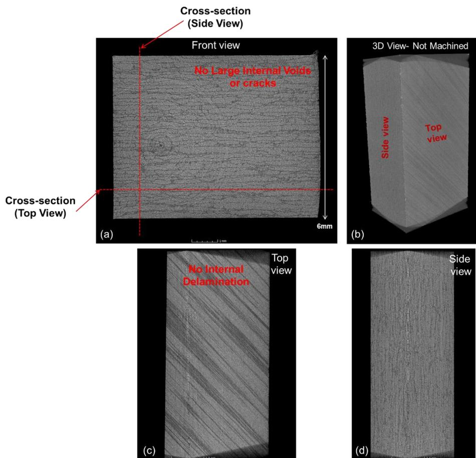
Figure 5-36- CT scans 45 degree orientation, un-machined sample.
