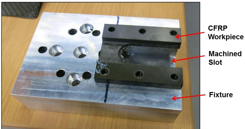
Figure 3-2-Experimental setup of machined slot, workpiece and fixture.
