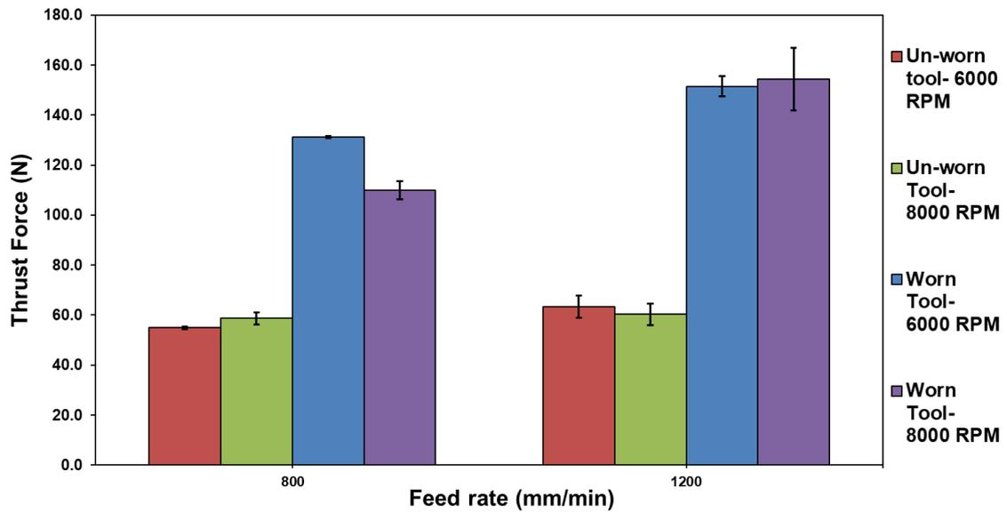
Figure 5-6-  $F_y$  thrust force vs feed rate, with worn and un-worn tool. (90 degree fibre orientation).
