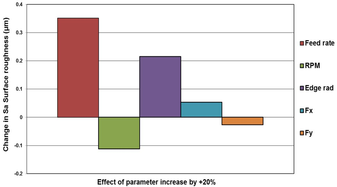
Figure 8-27- Effect of a 20 % increase in process parameters on the  $S_a$  surface roughness.
