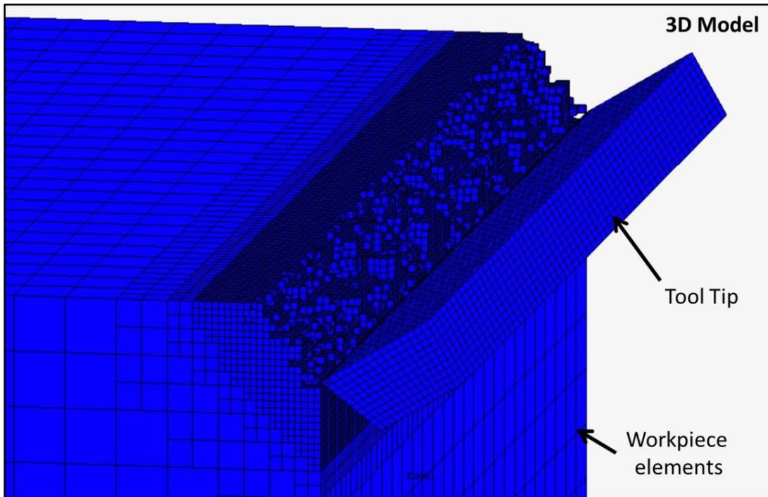
Figure 8-3- 3D Simulation with deactivation of orthotropic composite elements by Hashin damage model.
