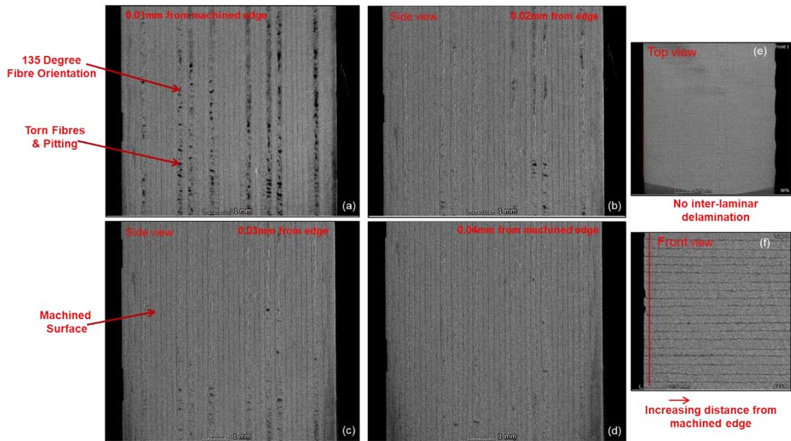
Figure 5-39- Machined surface- CT scans showing damage at progressing distance from the machined edge.
