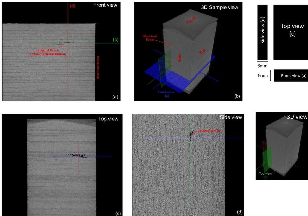
Figure 5-35- 90 degree fibre orientation with internal crack.
