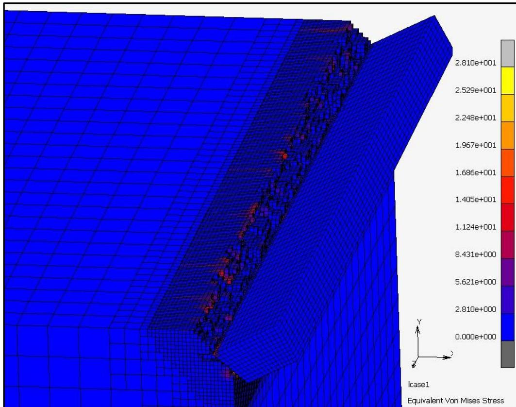
Figure 8-32- Von Mises stress through thickness, 3D FE edge trimming model.
