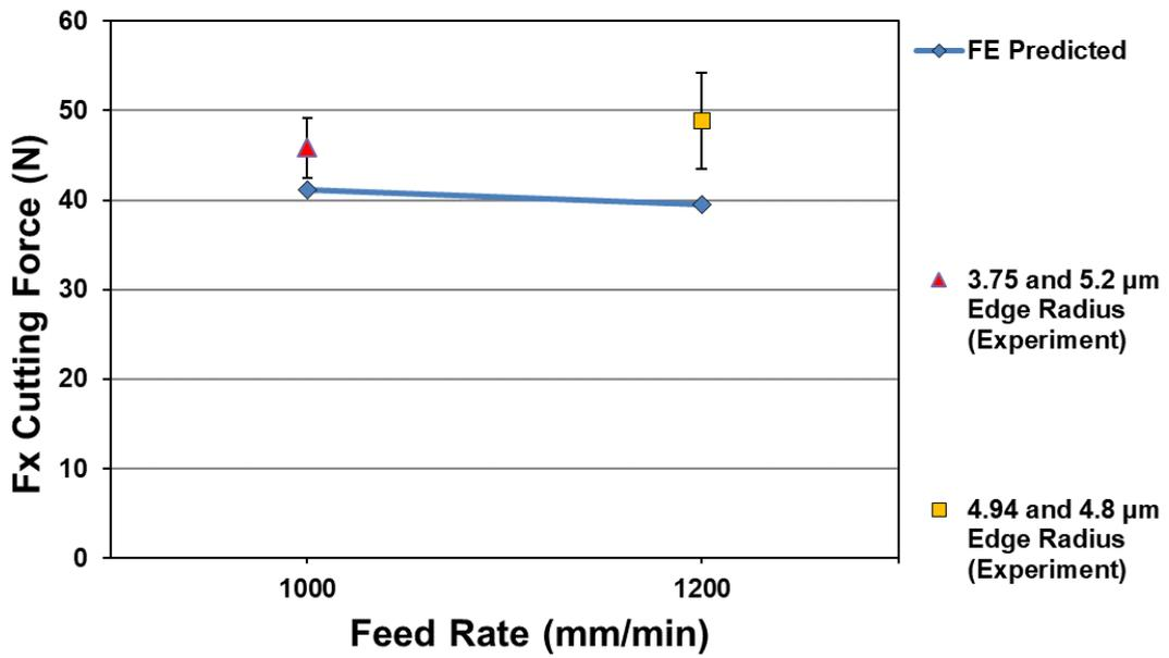
Figure 8-24- Experimental and FE model Fx cutting forces vs increasing feed at 9000 RPM.
