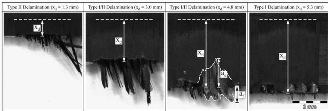
**Figure 2-10- Different delamination on a machined edge of woven composite [29].**
