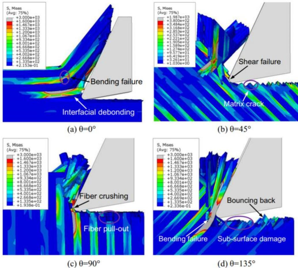
Figure 2-25- Cutting mechanism on different fibre orientations in micro-mechanical orthogonal cutting model. Adapted from REF [75].
