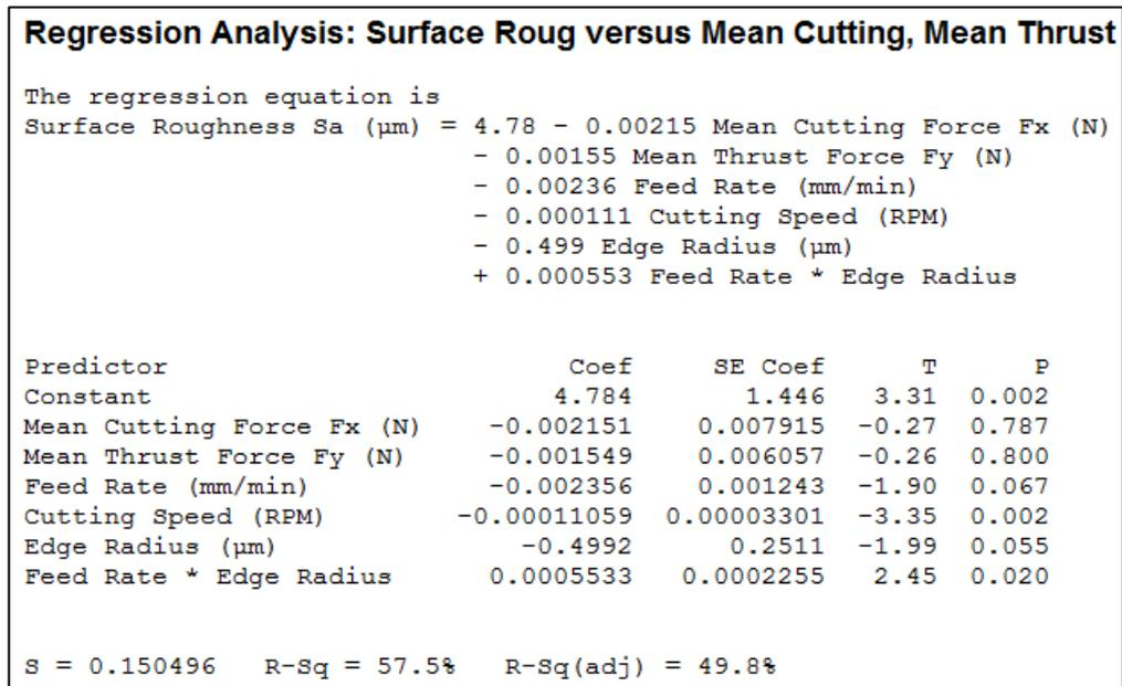
Figure 6-6- Regression model output with additional model predictors.
