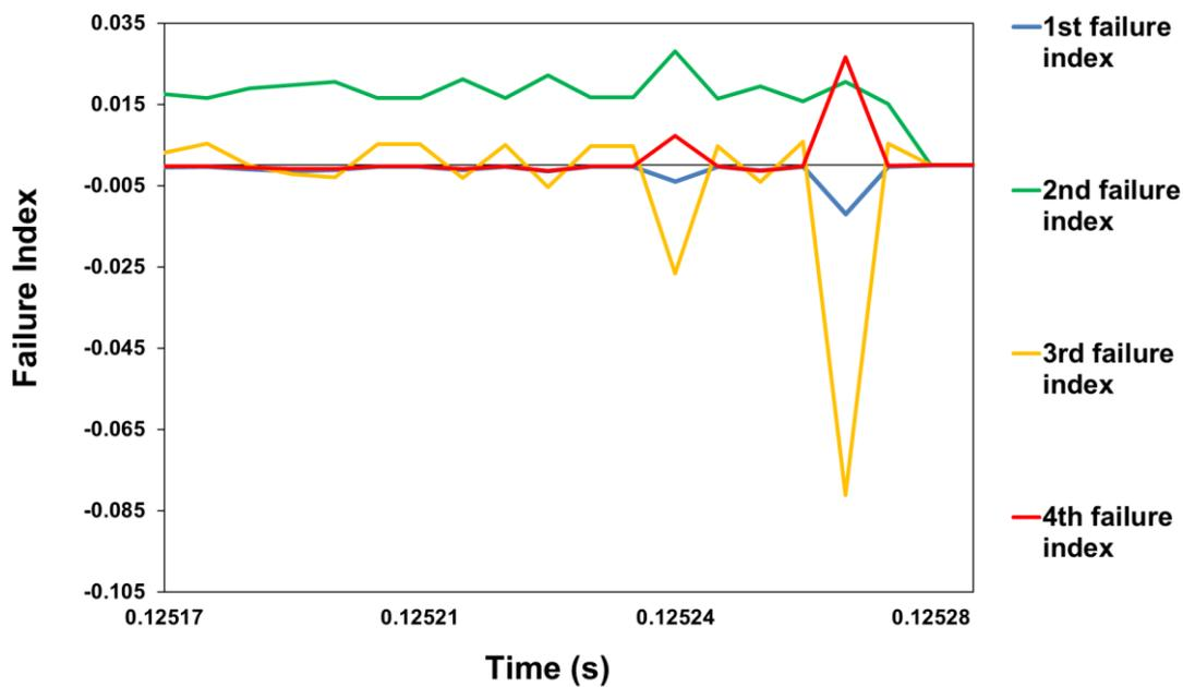
Figure 8-16- FE model- Hashin failure index at single node position over successive increments. (45 degree fibre orientation, 10 $\mu$ m edge radius, 800mm/min Feed and 6000RPM)
