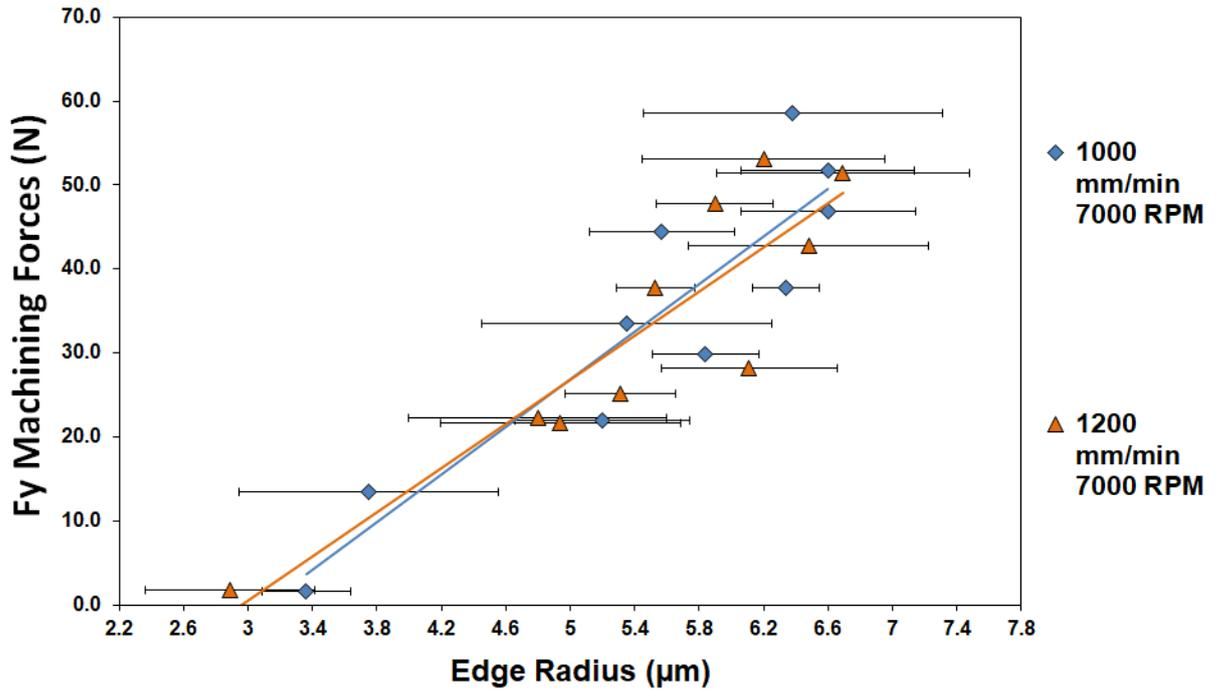
Figure 5-24- Fy Cutting forces against increasing edge radius at 7000 RPM. The error bars (x-axis) represent standard deviation in the edge radius measurement from 3 cutting edges.
