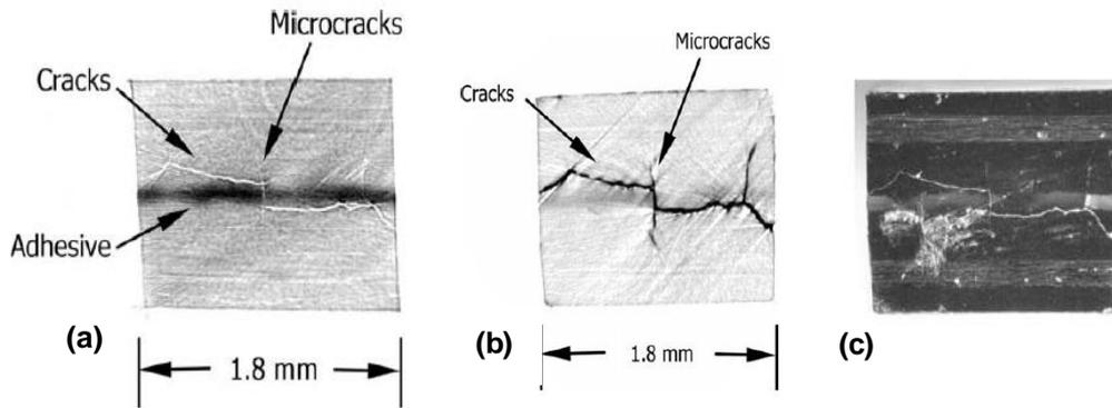
Figure 2-19- Comparison of images taken of a carbon fibre specimen by Micro-CT scan (with and without dye penetrant) and optical microscope.
