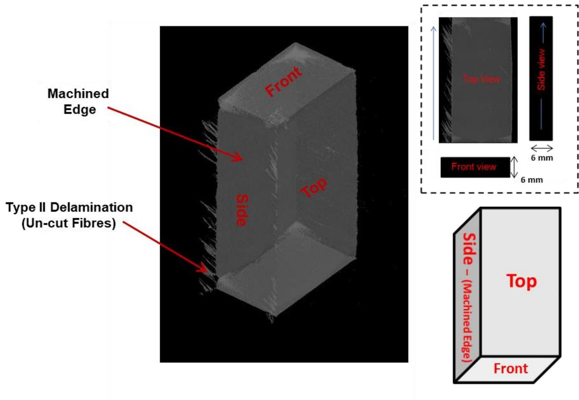
[Figure 5-31](#)- CT scan of machined unidirectional 45 degree fibre orientation, showing planar views.
