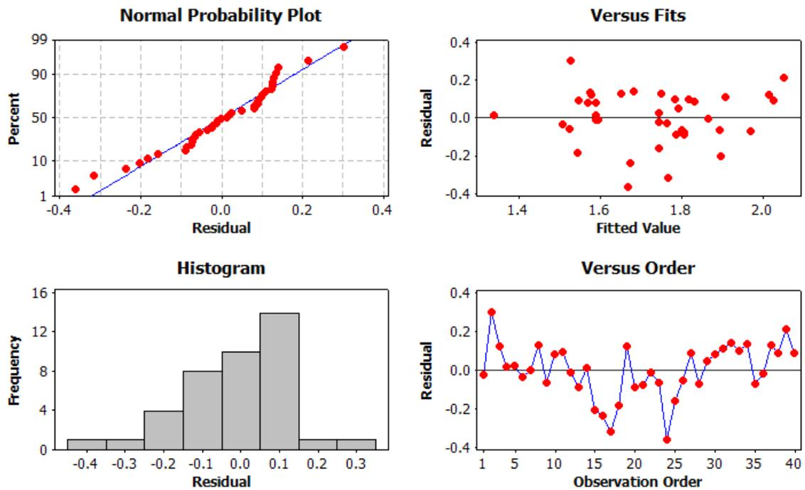
Figure 6-5- Residual plots of  $S_a$  surface roughness for first multiple linear regression model attempt.
