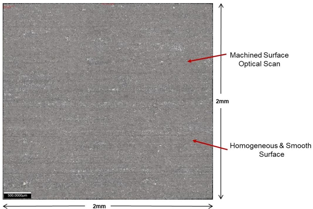
Figure 5-10- 2 x 2mm optical focus variation scan taken from middle of sample. (90 degree fibre orientation, 800 mm/min, 6000 RPM, Worn-tool).
