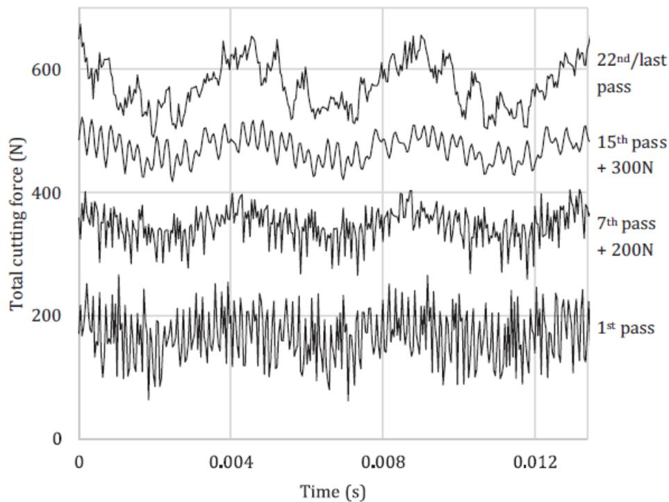
Figure 2-16- The total cutting force at different levels of tool wear, with 3 tool rotations shown [48].
