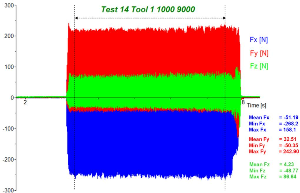
Figure 5-21- Machining forces from multidirectional test dynamometer.
