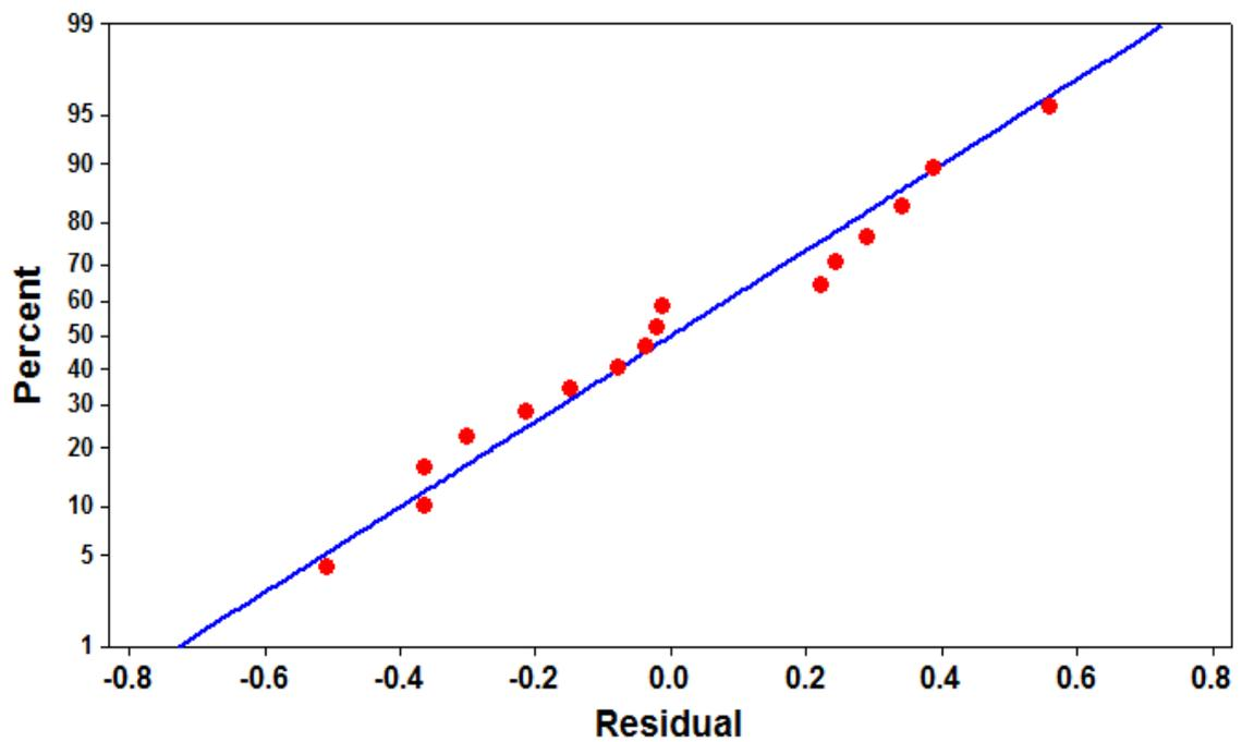
Figure 6-12- Normal probability plot for surface roughness (Sa) response
