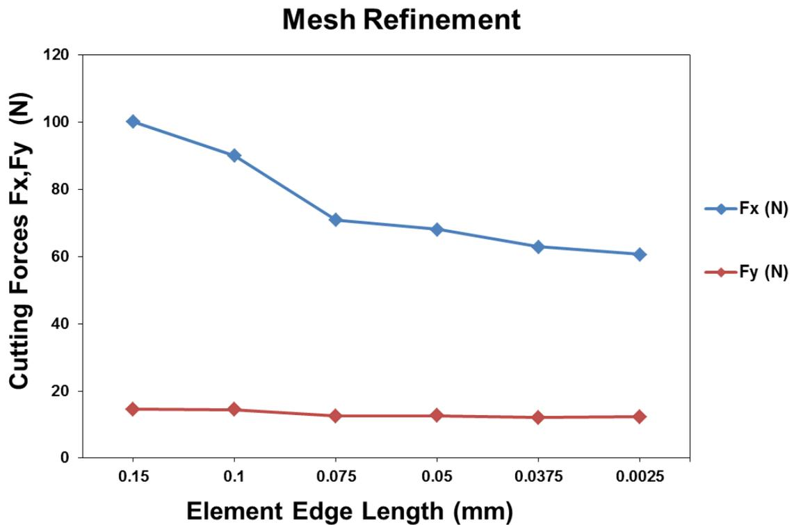
Figure 8-18- Mesh refinement against decreasing element size.
