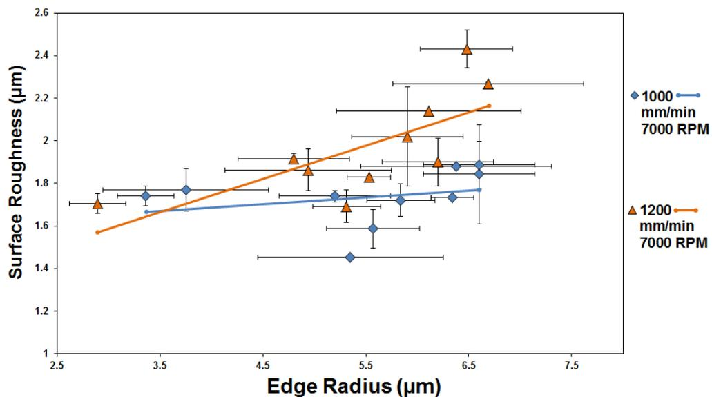
Figure 5-19- Mean  $S_a$  against increasing edge radius, grouped by dependant parameters feed rate and cutting speed at 7000 RPM. The error bars show standard deviation in roughness and edge radius measurement.
