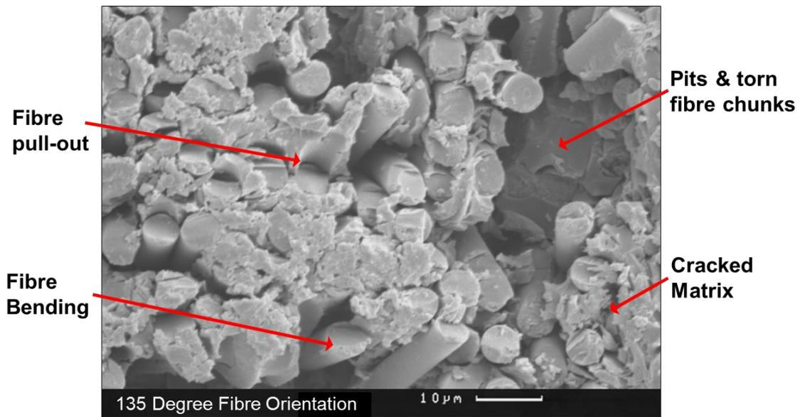
Figure 3-20- The 135 Degree fibre orientation SEM image.
