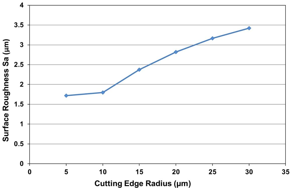
Figure 8-11- The predicted increase in  $S_a$  surface roughness with cutting edge radius.
