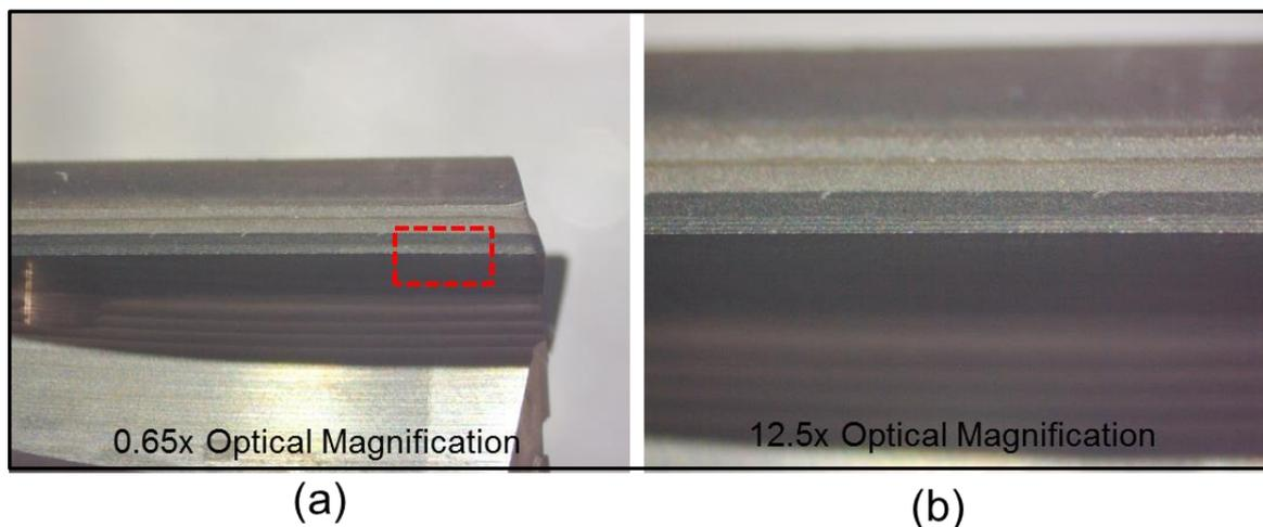
[Figure 5-7- Optical microscope images of new unworn PCD tool.](#)
