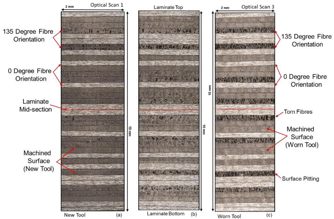
Figure 5-16- Multidirectional optical focus variation scans. Images show a 2D plane image of the machined surface profile texture at increasing tool wear. The full laminate thickness of 10mm is shown.
