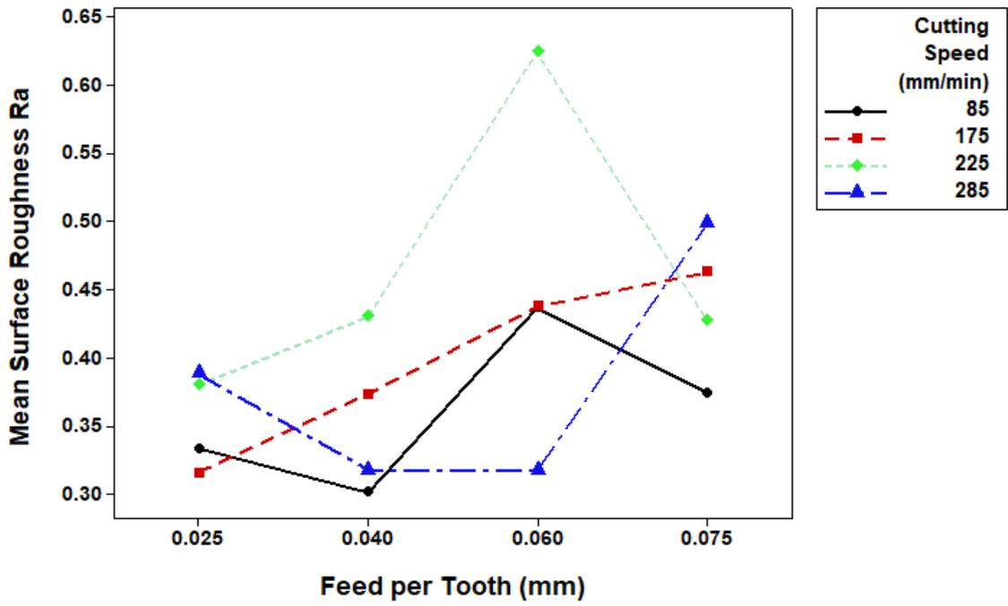
Figure 3-9- Mean  $R_a$  Surface roughness for 0 degree fibre orientation, against feed rate grouped at each cutting speed.
