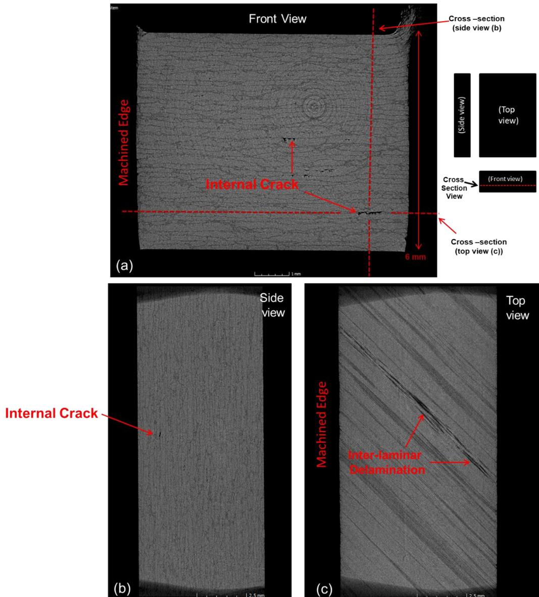
[Figure 5-32- 45 degree fibre orientation with internal crack.](#)
