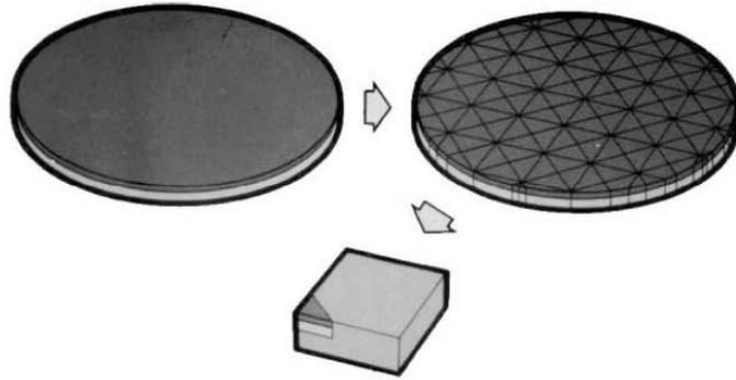
Figure 2-18 – PCD disk which is then cut into segments before brazing onto tool [61].
