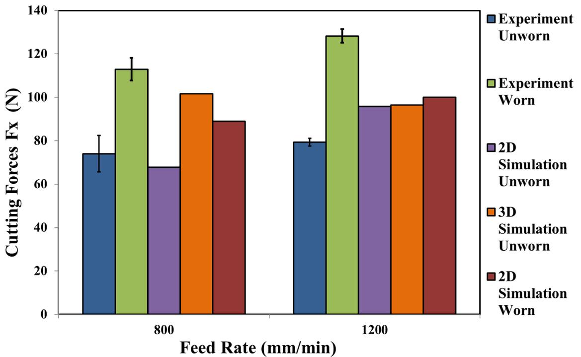
Figure 8-7- Fx cutting forces vs feed rate from experimental and FE for 45 degree fibre orientation at 6000 RPM.
