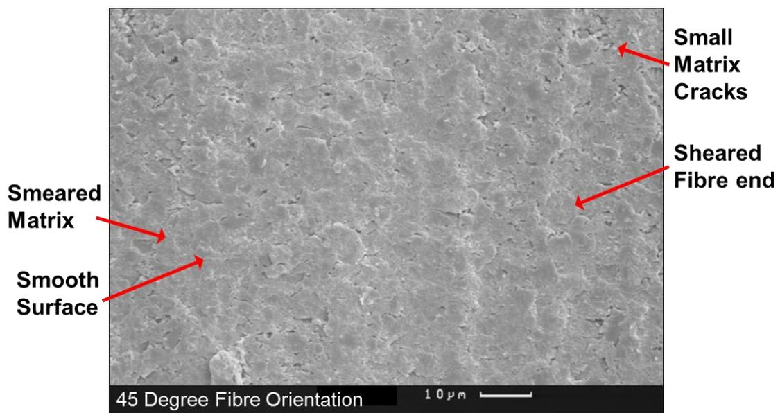
[Figure 3-21- The 45 Degree fibre orientation SEM image.](#)
