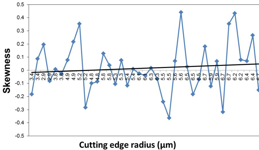
Figure 8-35- The 0 degree fibre orientation, change in skewness vs increasing cutting edge radius.
