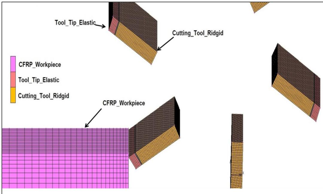
Figure 7-3- 3D Milling simulation with contact bodies.
