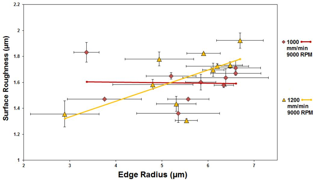
Figure 5-20- Mean  $S_a$  against increasing edge radius, grouped by dependant parameters feed rate and cutting speed at 9000 RPM. The error bars show standard deviation in roughness and edge radius measurement.
