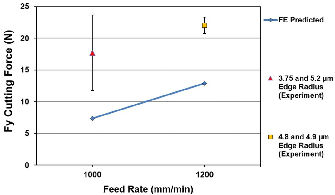
Figure 8-25- Experimental and FE model Fy cutting forces vs increasing feed at 7000 RPM.
