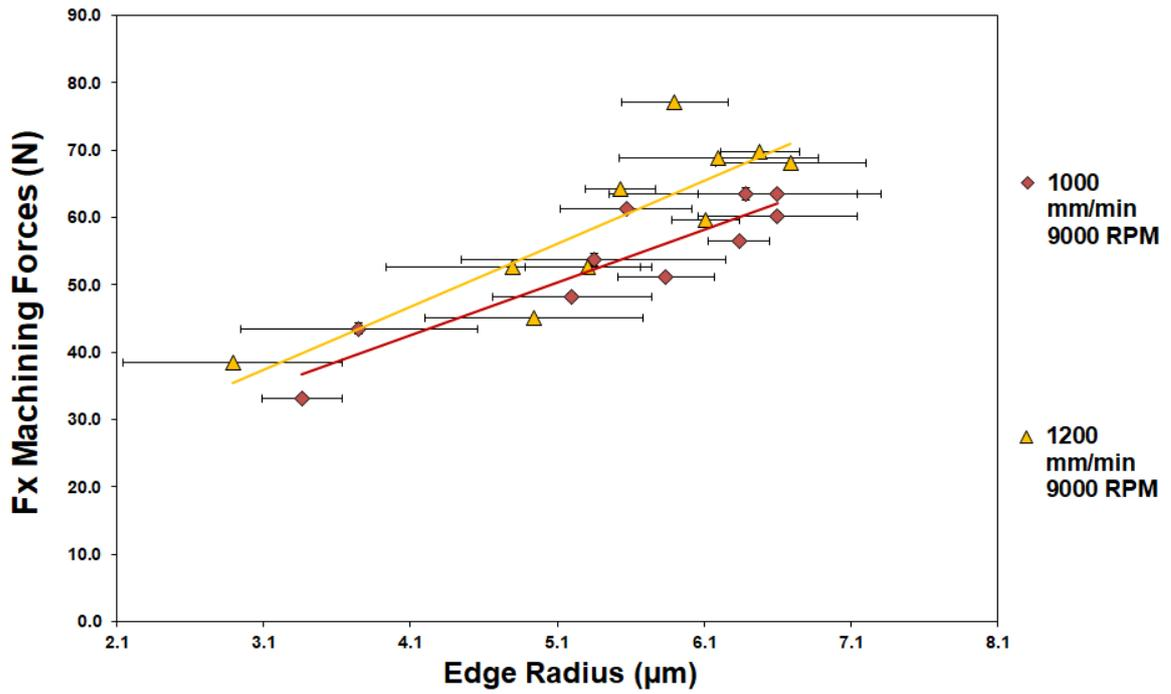
Figure 5-23- Fx Cutting forces against increasing edge radius at 9000 RPM. The error bars represent standard deviation in the edge radius measurement from 3 cutting edges.
