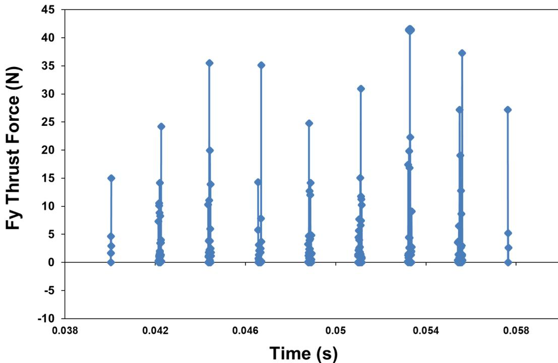
Figure 8-22- 3D FE model thrust forces (Fy) vs time.
