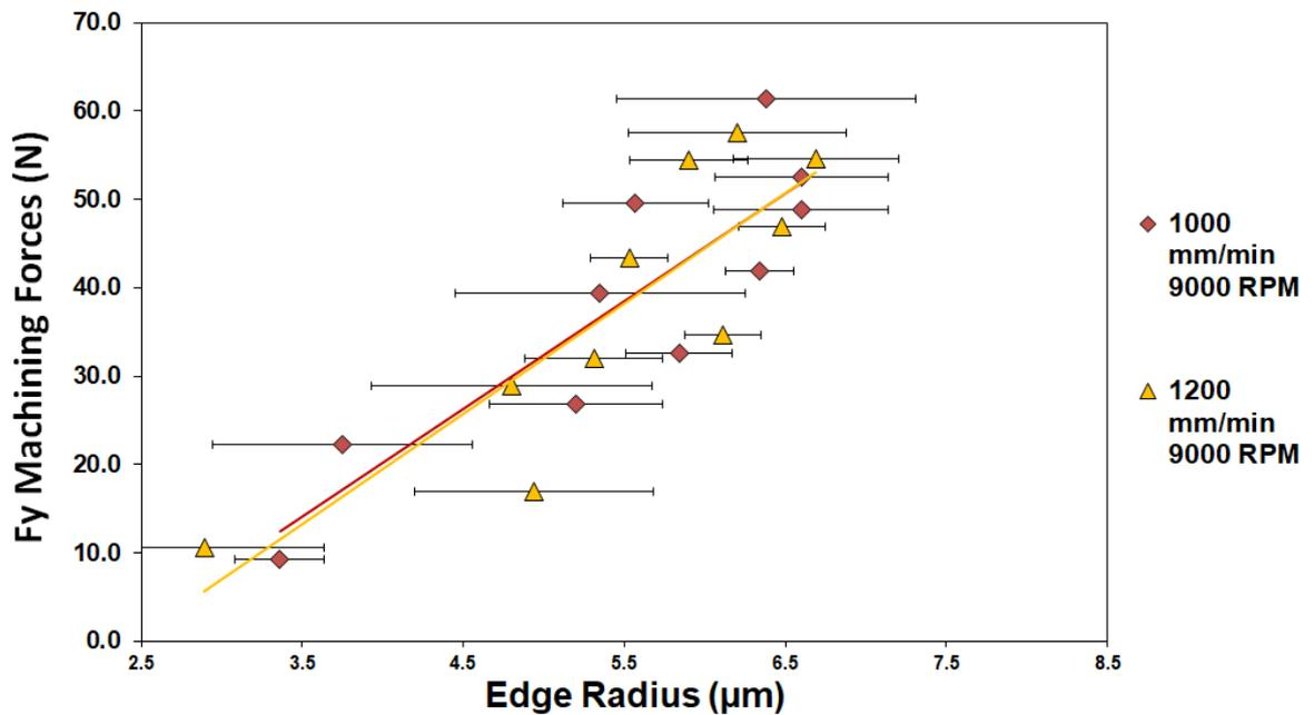
Figure 5-25- Fy Cutting forces against increasing edge radius at 9000 RPM. The error bars represent standard deviation in the edge radius measurement from 3 cutting edges (x-axis).
