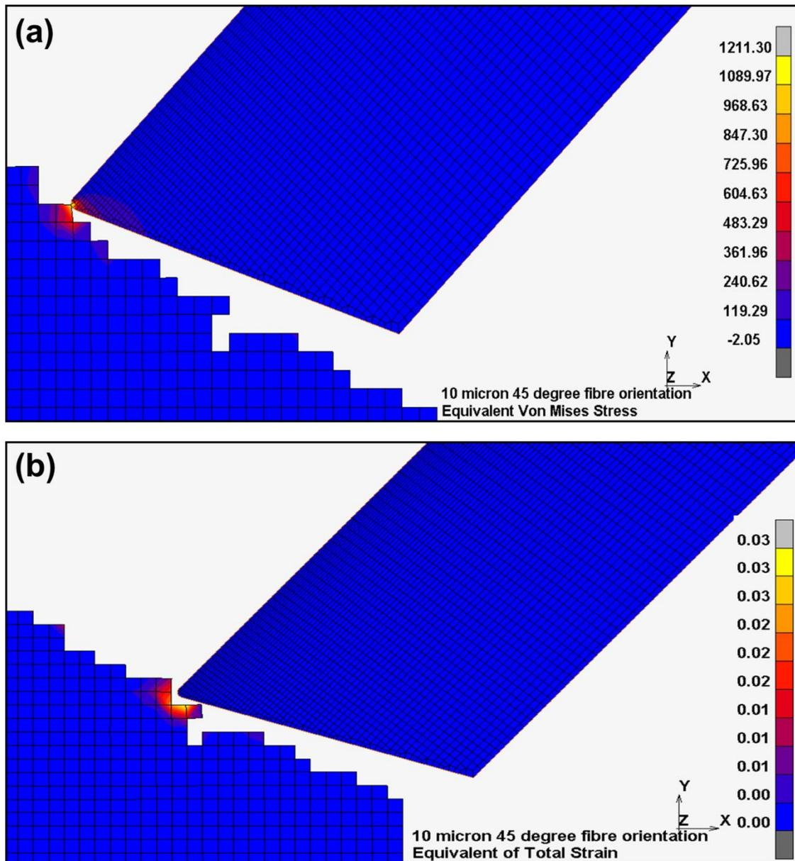
Figure 8-17- (a) Equivalent Von Mises stress,
