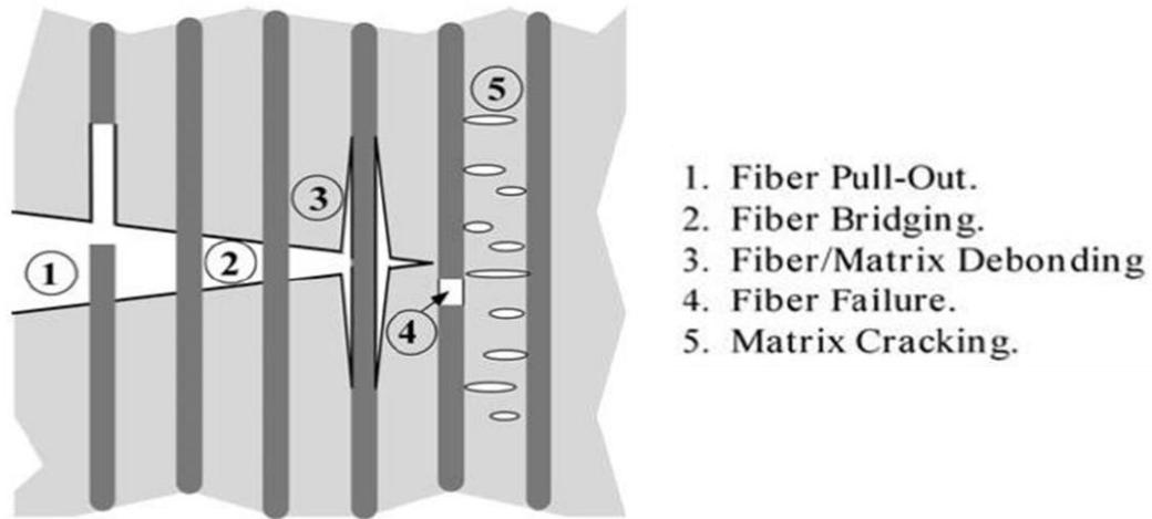
Figure 2-2 - Different failure mechanisms of laminate fibre composites. Adapted from REF [10]
