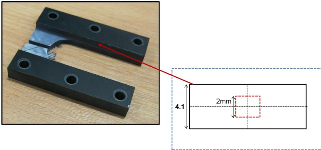
Figure 3-4- Position of optical scans for roughness measurements on sample.
