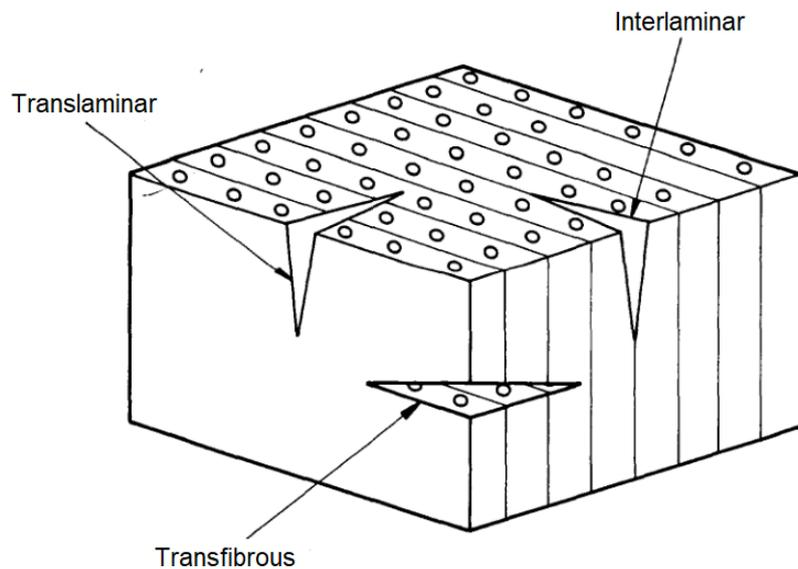
Figure 2-3 - Failure definition types [11].
