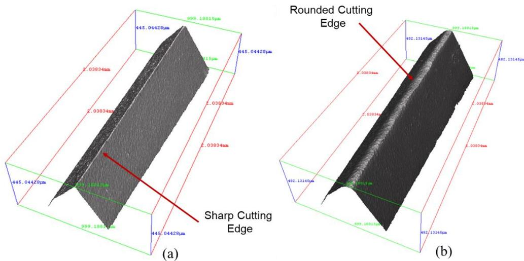
Figure 5-9- Tool cutting edge rounding Alicona scans,
