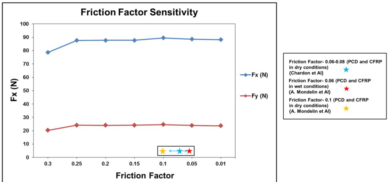
**Figure 8-19- Friction factor sensitivity.**
