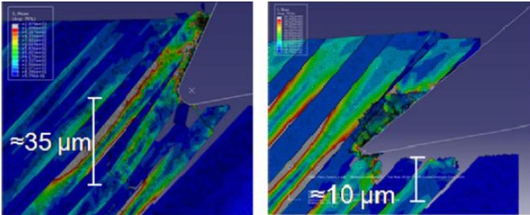
Figure 2-23 - Finite element model of composite machining to simulate use of a new high rake angle tool [71].
