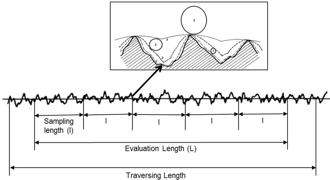
Figure 2-13- Profile evaluation length and sampling length. The stylus radius will dictate the profile vertical and lateral resolution as shown.
