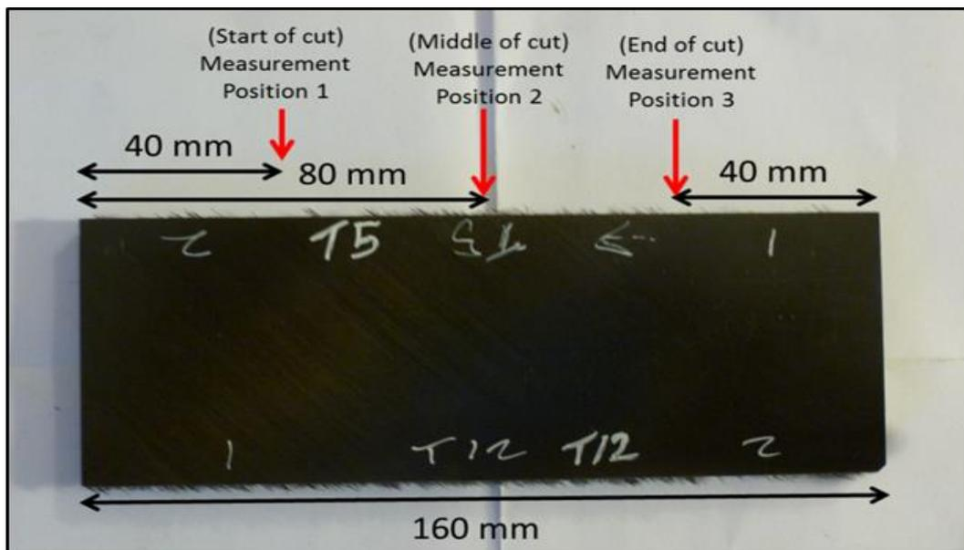
Figure 4-8 – Optical scan positions, (unidirectional sample).
