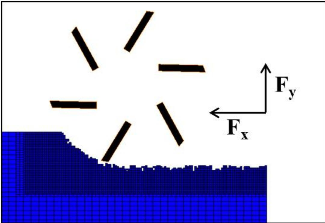
Figure 8-1- 2D edge trimming simulation with composite elements and  $F_x$  and  $F_y$  machining force orientation.
