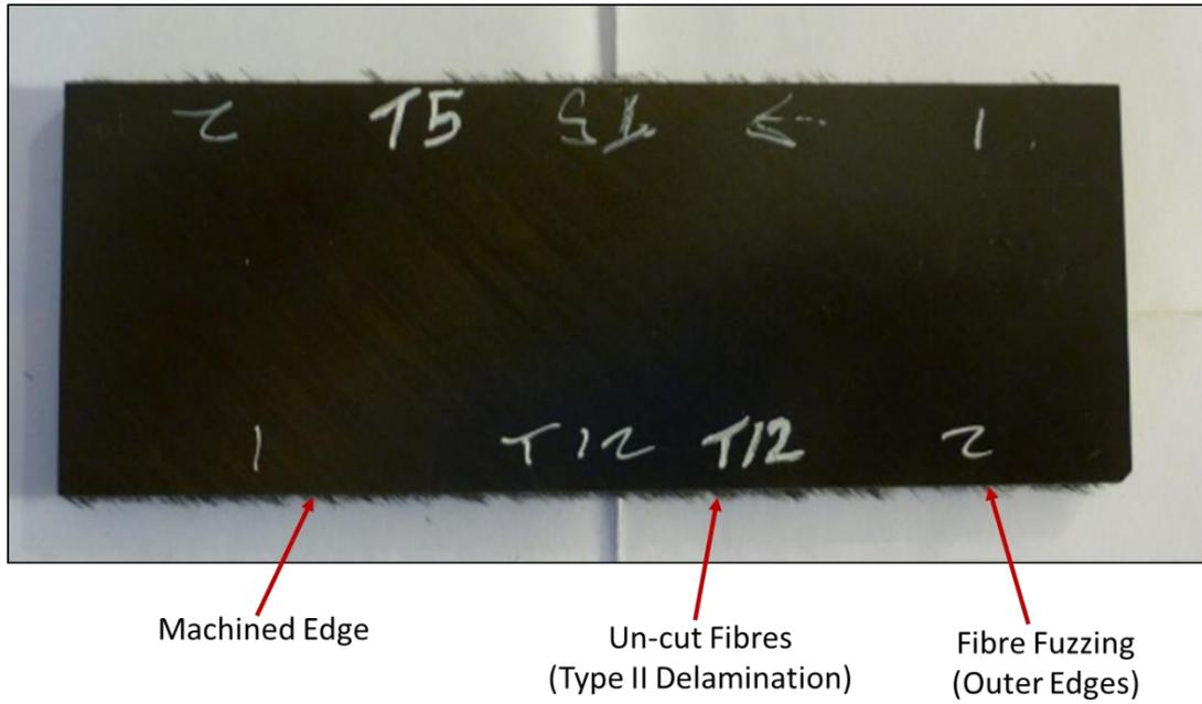
Figure 5-12- Machined unidirectional sample 45 degree orientation showing some un-cut fibres on top and bottom of laminate (worn cutting tool).
