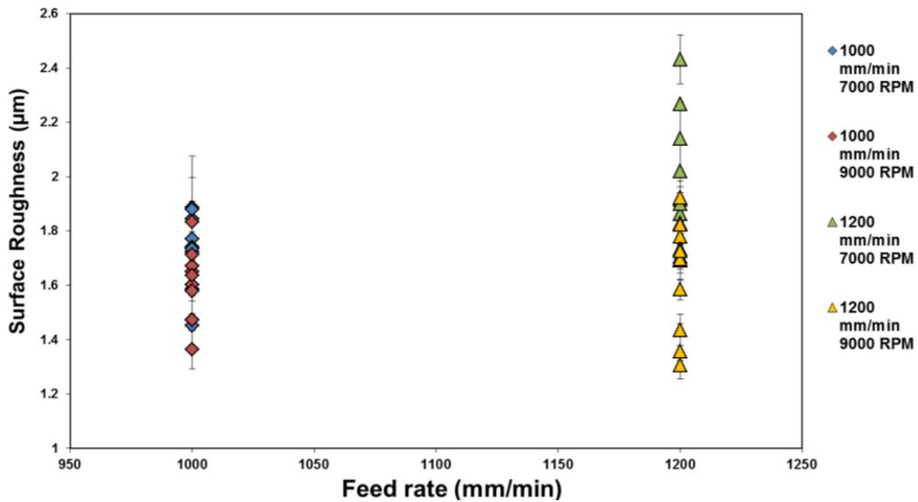
Figure 5-18- Surface roughness ( $S_a$ ) vs feed rate (grouped by applied cutting speed). (Error bars show standard deviation in roughness measurement.)
