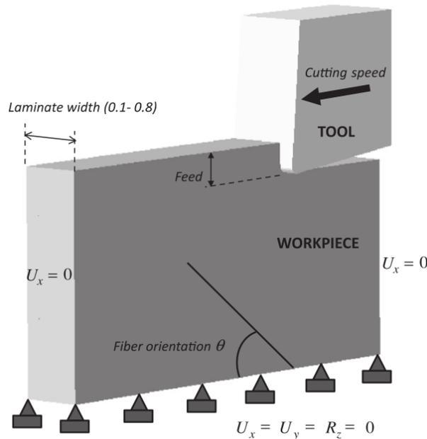
Figure 2-24 – 3D EHM model of orthogonal turning [72].
