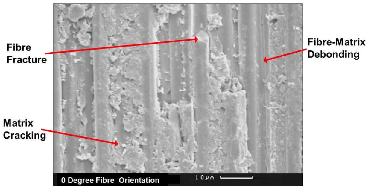
[Figure 3-19- The 0 Degree fibre orientation SEM image.](#)
