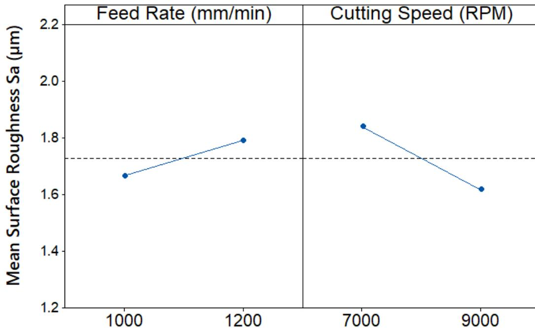
Figure 5-28- Main effects plot for average surface areal roughness parameter  $S_a$ .
