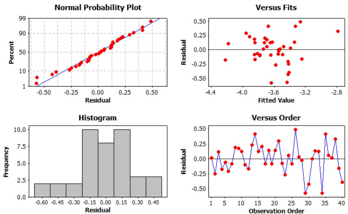
Figure 6-9- Residual plots for skewness, histograms of residuals, normal probability plot and residuals versus run order.
