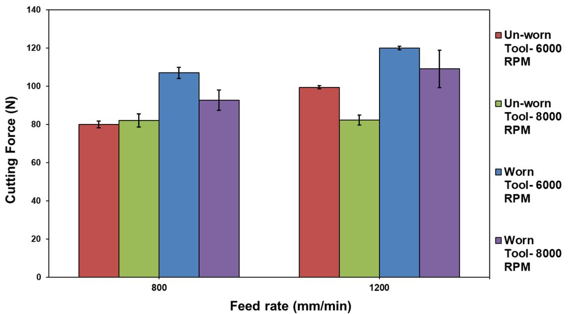
Figure 5-5- Fx cutting force vs feed rate, with worn and un-worn tool. (90 degree fibre orientation).
