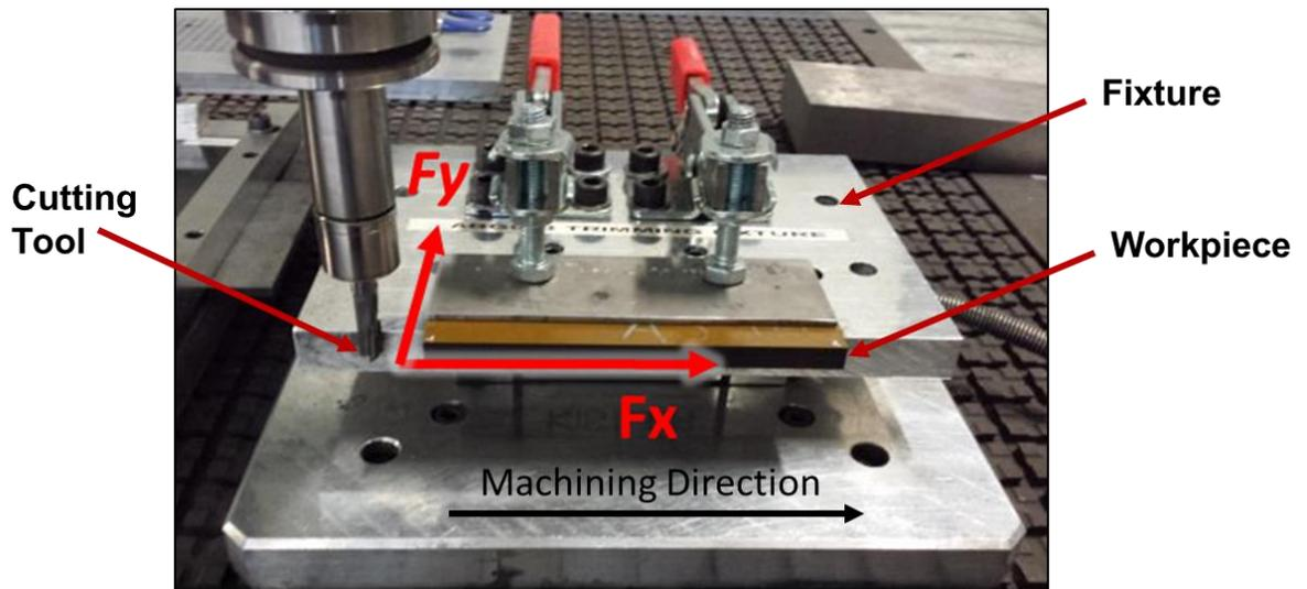
Figure 4-5- Machining forces orientation:  $F_x$  and  $F_y$ .
