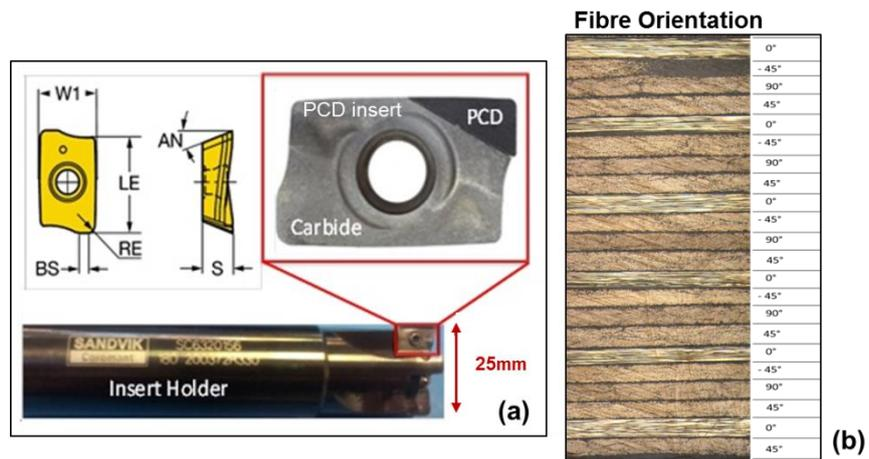
Figure 3-1- (a) PCD insert and 25 mm diameter tool holder,
