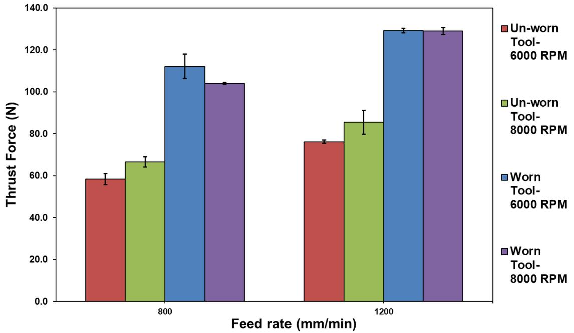
Figure 5-4- Fy thrust force vs feed rate, with worn and un-worn tool. (45 degree fibre orientation).
