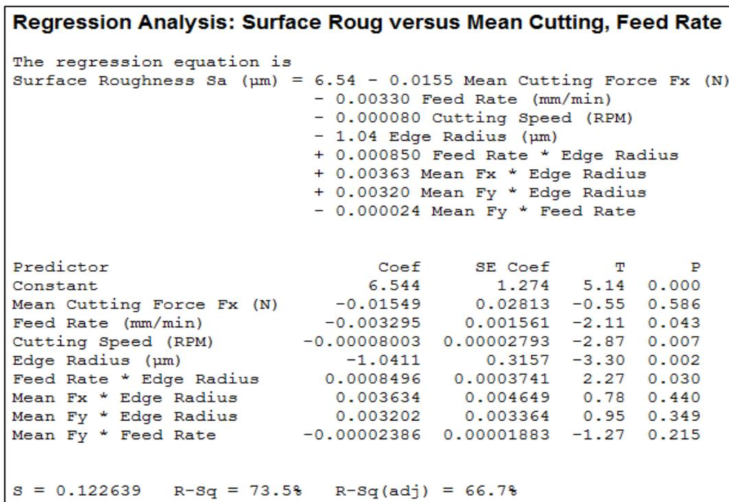
Figure 6-7- Final regression equation output with final predictors and interaction terms included.
