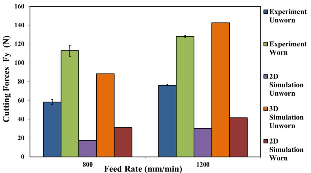
Figure 8-9-  $F_y$  cutting forces vs feed rate from experimental and FE for 45 degree fibre orientation at 6000 RPM.
