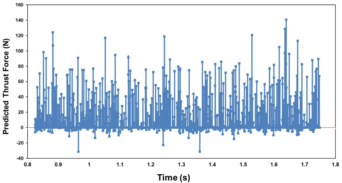
Figure 8-5- Fy thrust force output from FE model.
