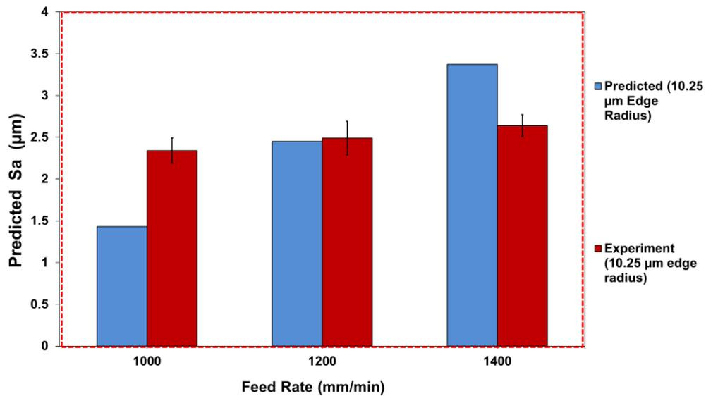
Figure 8-31- Experimental vs predicted  $S_a$  surface roughness at increasing feed rate at constant 11000 RPM, (10.25  $\mu\text{m}$  edge radius). Error bar represents standard deviation between averaged set of test results with a different edge radius.
