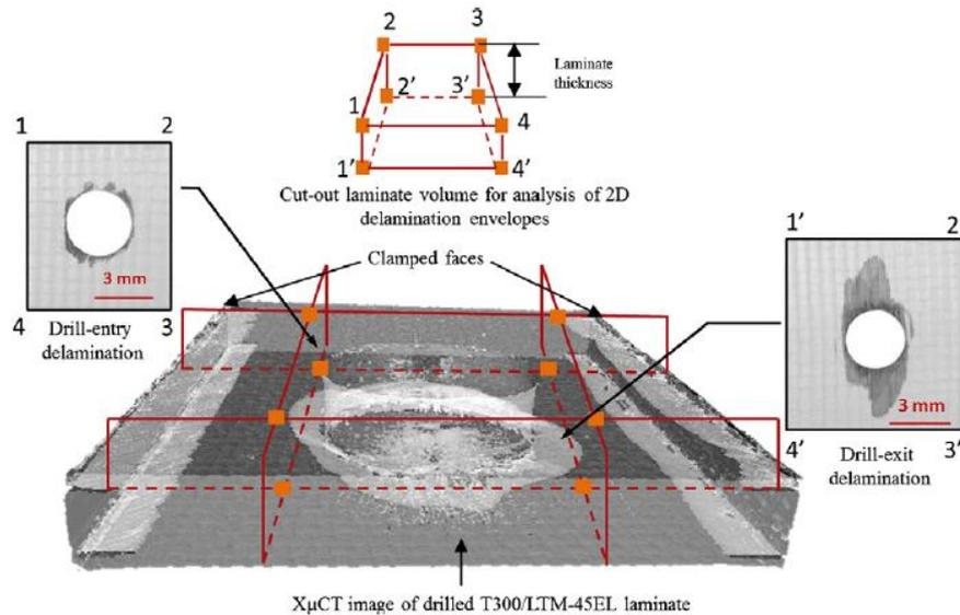
[Figure 2-22 - CT scan of drill entry and exit delamination \[6\].](#)
