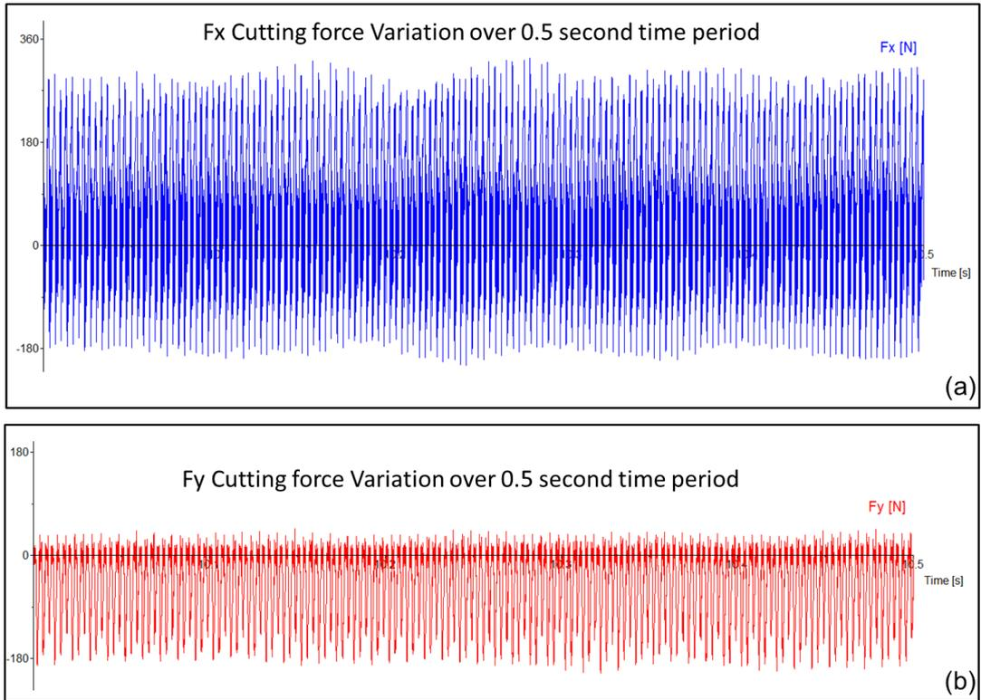
Figure 5-2- Machining force fluctuation over 0.5 seconds of cutting.
