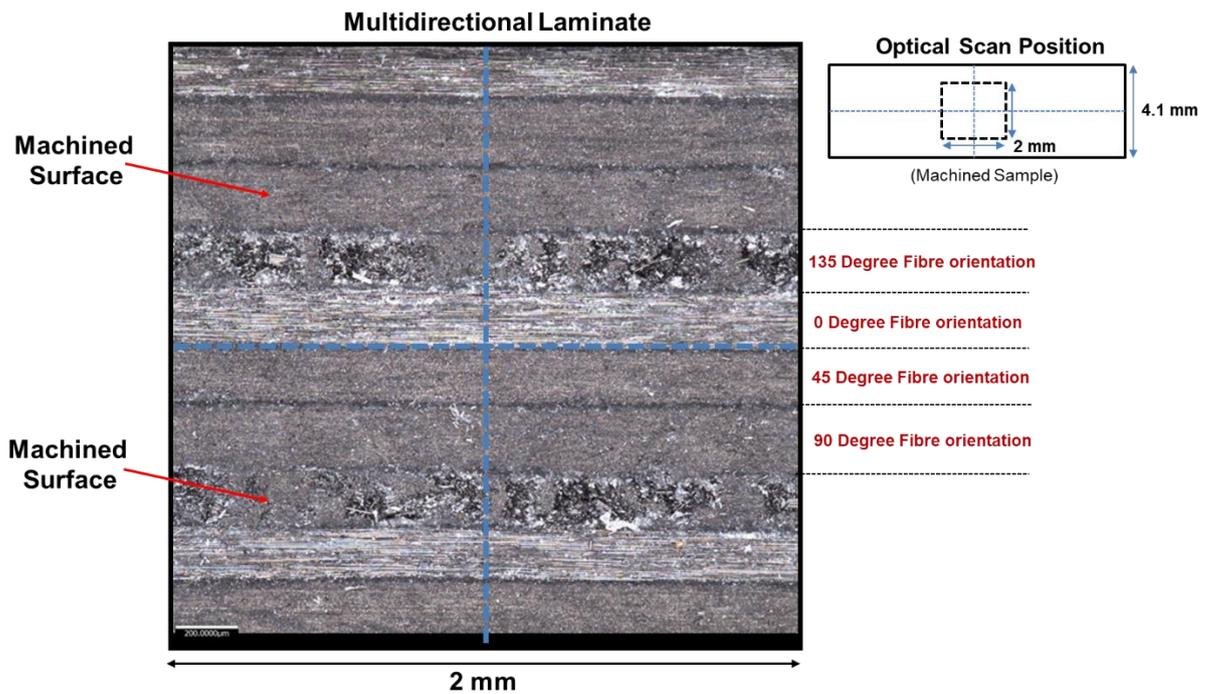
Figure 3-7- Optical surface measurement highlighting different surface damage on each fibre orientation. The image shows the edge machined surface profile.
