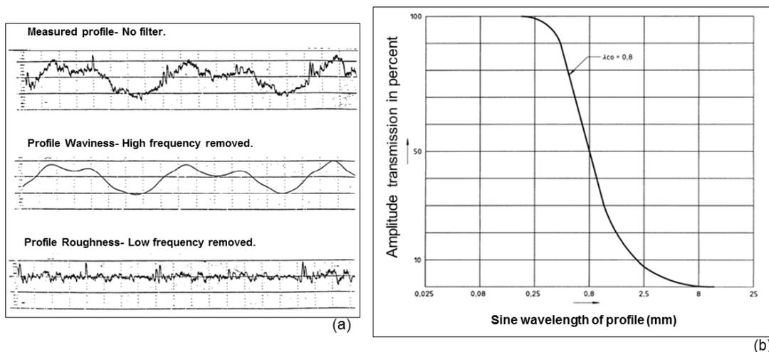
Figure 2-14- Removal of low frequency component in roughness measurement, (a) Measured profile with waviness and roughness shown, (b) Removal of profile waviness.
