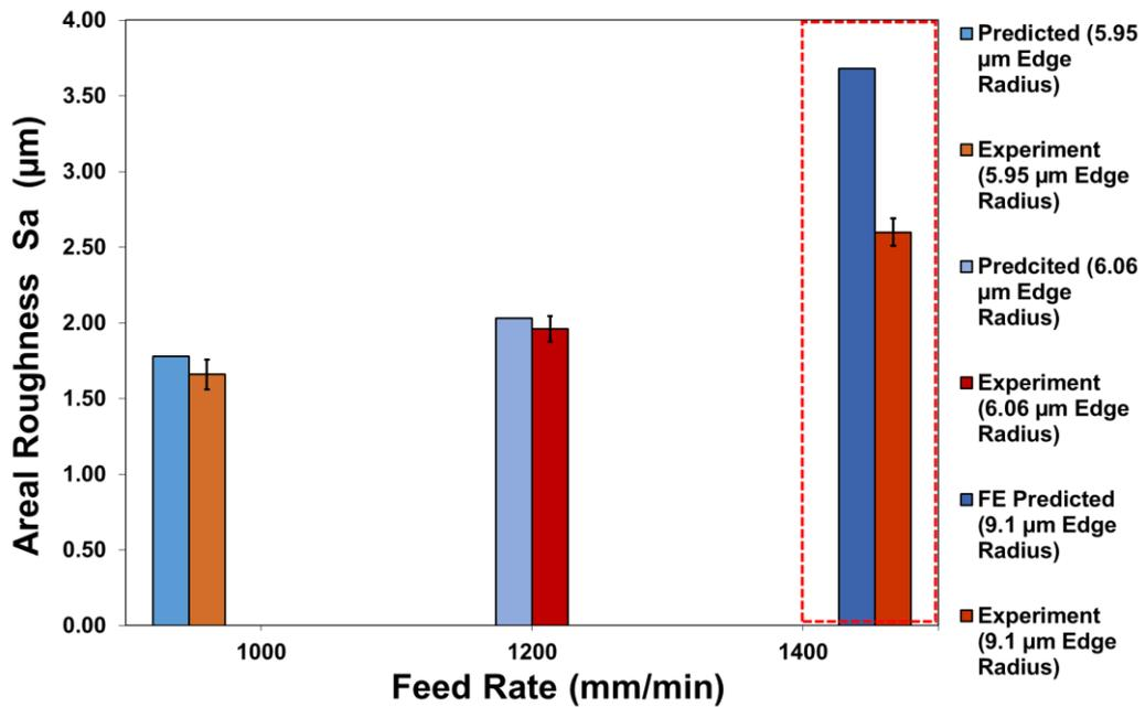
Figure 8-28- Experimental vs FE predicted  $S_a$  surface roughness at increasing feed rate at constant 7000 RPM. Error bar represents standard deviation between averaged set of test results with a different edge radius.
