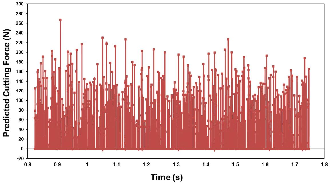
Figure 8-4- Fx cutting force output from FE model.
