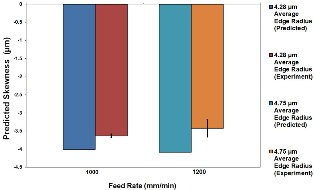
Figure 8-34-Predicted skewness values vs experiment.
