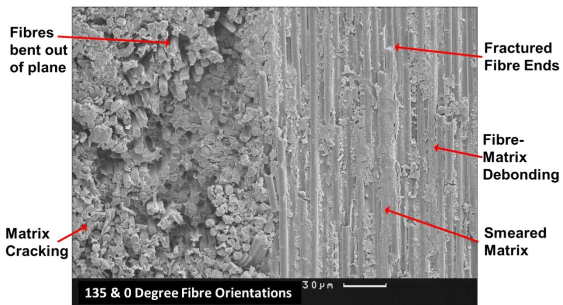
Figure 3-18- SEM image of 135 and 0 degree ply.
