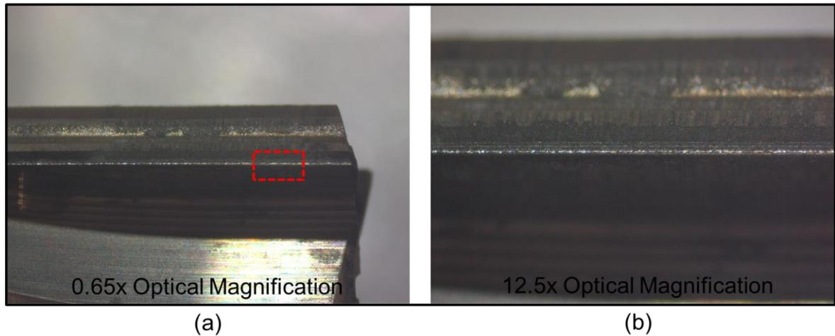
Figure 5-8- Optical microscope images of worn PCD tool.
