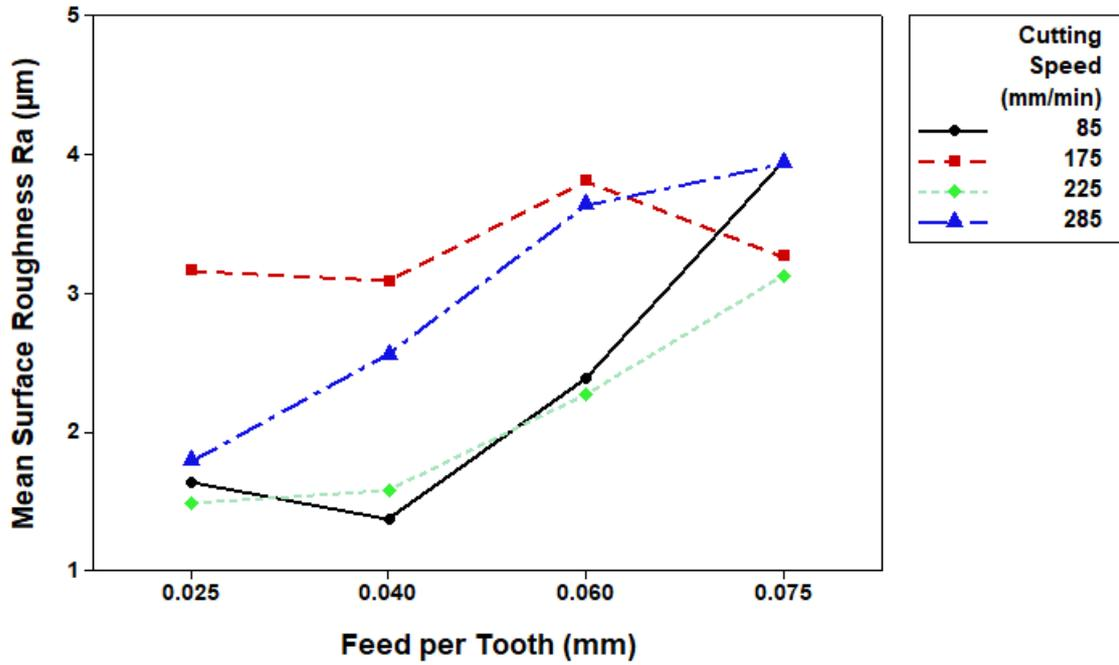
Figure 3-11- Mean  $R_a$  surface roughness for 90 degree fibre orientation, against feed rate grouped at each cutting speed.
