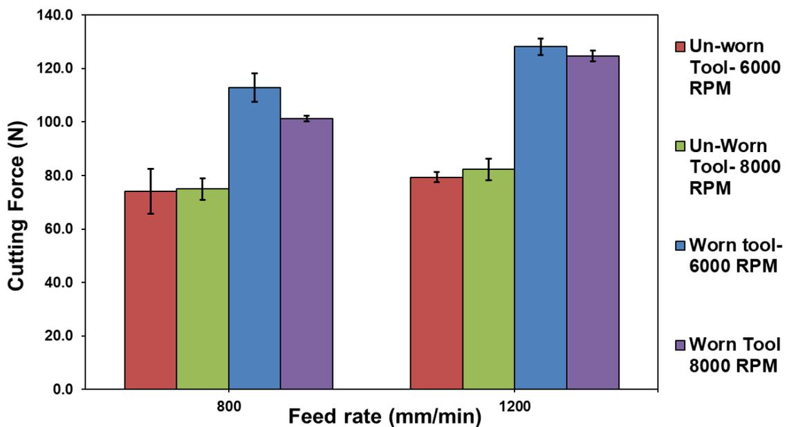
Figure 5-3-  $F_x$  cutting force vs feed rate, with worn and un-worn tool. (45 degree fibre orientation).
