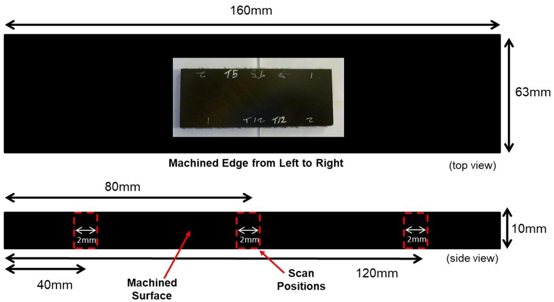
Figure 4-9- Three optical scan positions on sample for roughness calculation, (unidirectional sample).
