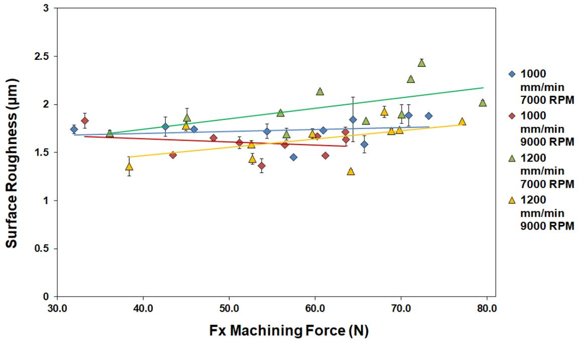
Figure 5-29- Surface roughness ( $S_a$ ) vs  $F_x$  machining force from experiment. Grouped by applied cutting speed and feed rate.
