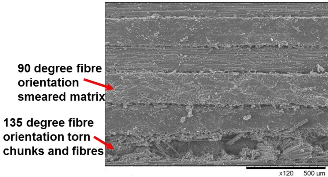
Figure 3-22- Multidirectional laminate, experimental test 2, worn cutting tool.
