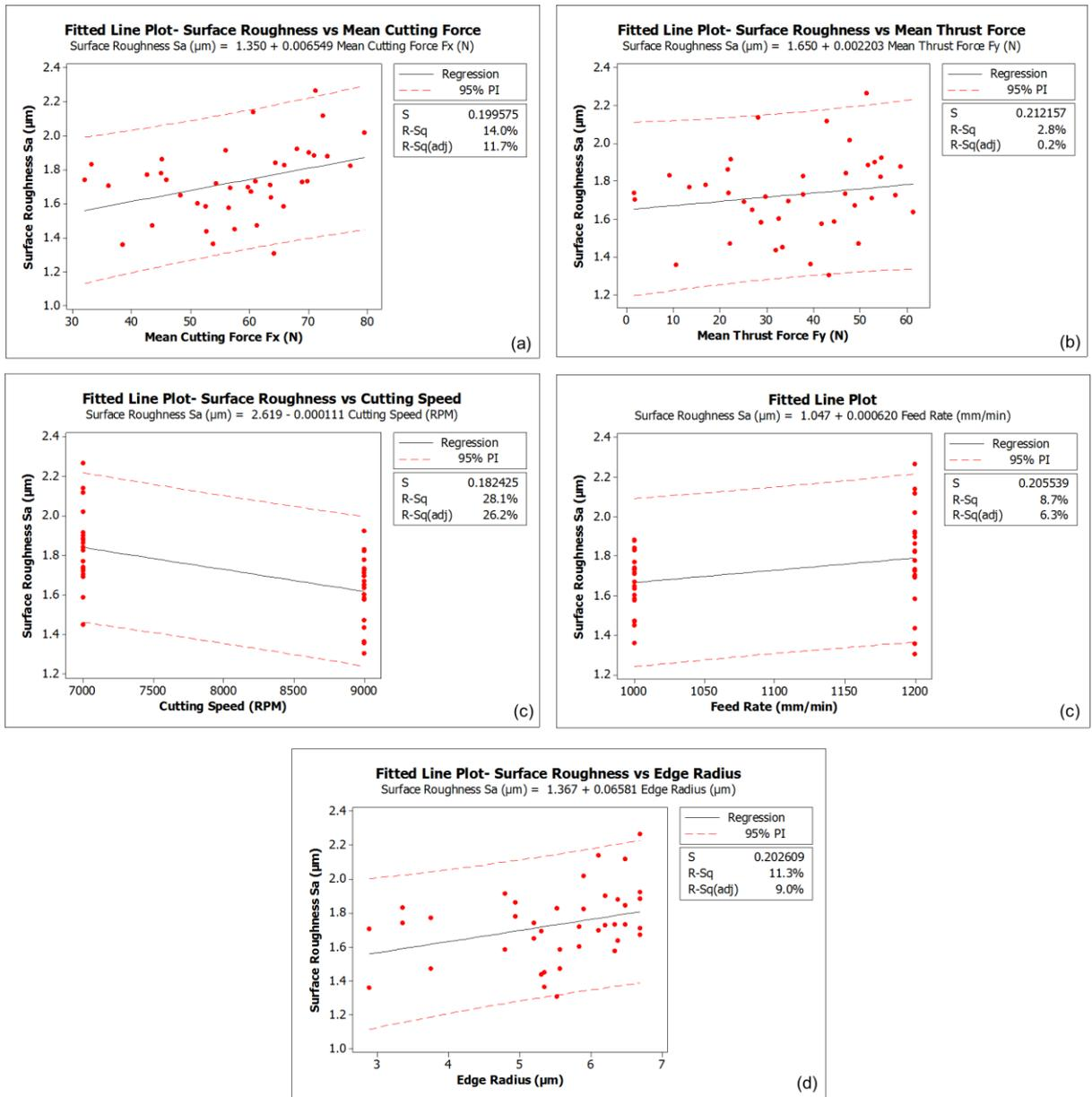
Figure 6-1- Fitted line plot for predictor variables effect on surface roughness, shown with 95 % confidence interval, (a) Mean Fx, (b) Mean Fy, (c) Feed rate, (d) Edge radius.
