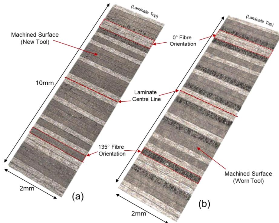
Figure 4-11- Example Alicona optical scans from a CFRP multidirectional laminate:
