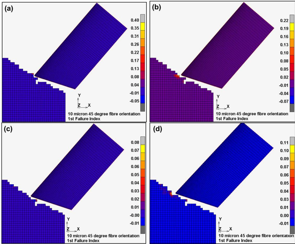
Figure 8-15- Fibre tensile failure magnitude (1st Failure index) in subsequent increments (a)-(d). (45 degree fibre orientation, 10 $\mu$ m edge radius, 800mm/min Feed and 6000RPM)
