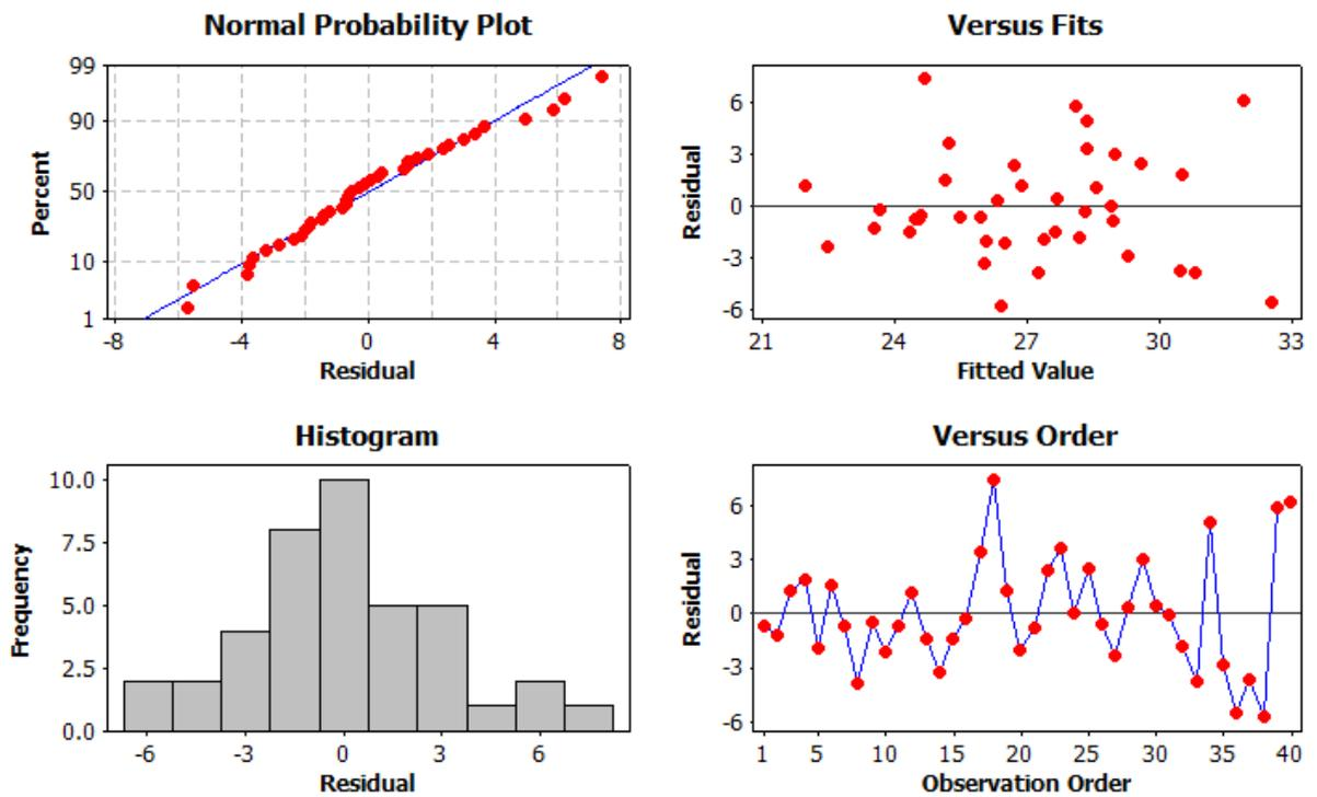
Figure 6-10- Residual plots for kurtosis, histograms of residuals, normal probability plot and residuals versus run order.
