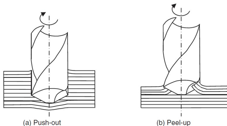
[Figure 2-12- Two types of delamination while drilling composites.](#)
