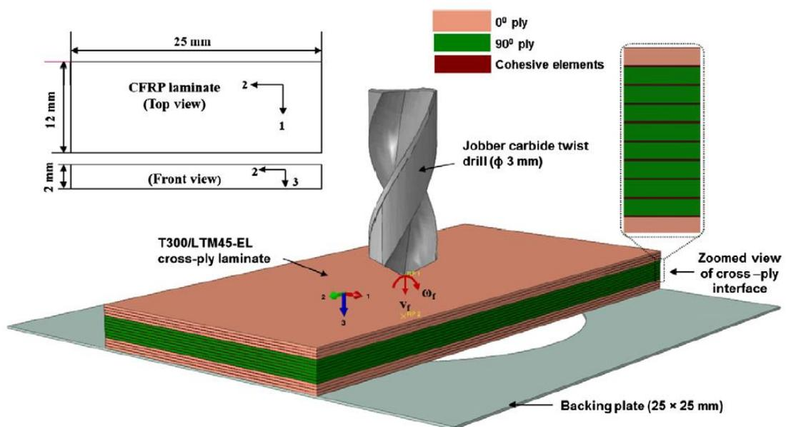
[Figure 2-26- Drilling CFRP laminate 3D model \[6\].](#)
