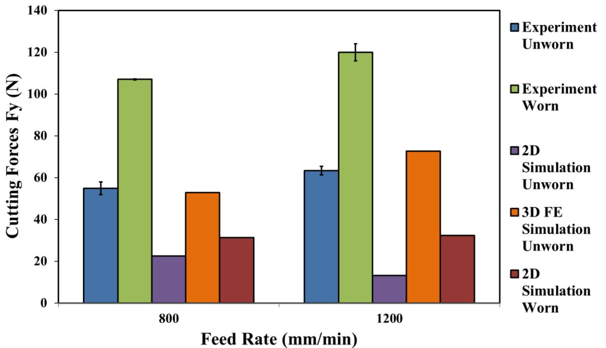
Figure 8-8-  $F_y$  cutting forces vs feed rate from experimental and FE for 90 degree fibre orientation at 6000 RPM.
