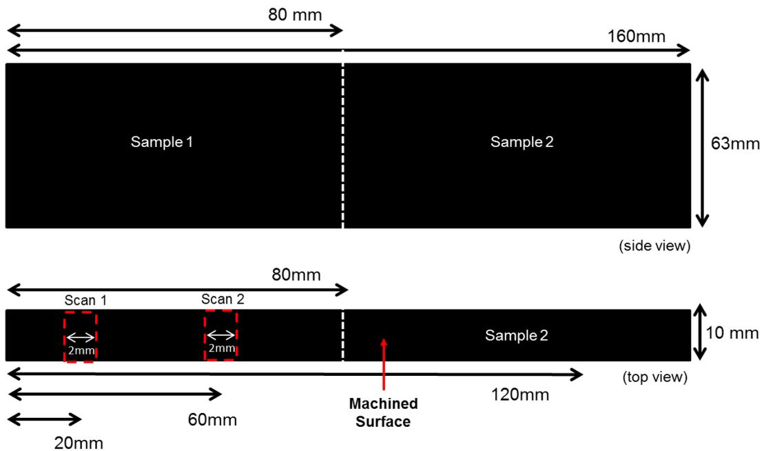
Figure 4-10- Roughness measurement positions, (multidirectional laminate).
