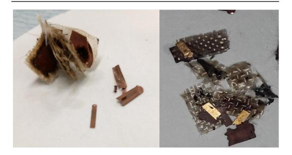
**Figure 48:** A delaminated PCB chips: (left) After 1 hour of microwave-assisted leaching in bmim[HSO<sub>4</sub>]; (right) After 2 hours of microwave-assisted leaching in bmim[HSO<sub>4</sub>] liquid.
