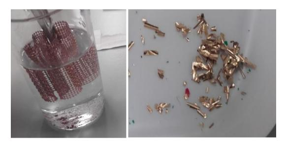
Figure 74: (a) The copper mesh used as cathode, copper-nickel alloy powder dropping off copper mesh into distilled water; (b) some gold flakes collected after Cu-Ni leaching process.
