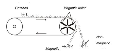
**Figure 8** Magnetic separation technique using a magnetic roller and a rubber belt.
