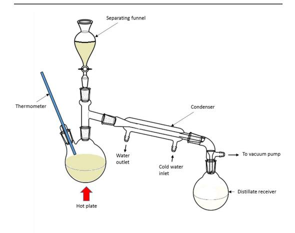
**Figure 29:** Vacuum distillation setup for the regeneration of BmimHSO<sub>4</sub> ionic liquid after delamination reaction process.
