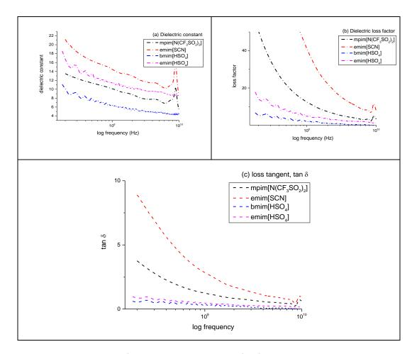
Figure 34: Measured frequency sweep data for four imidazolium-based ionic liquids at room temperature, showing the frequency dependence of microwave absorption and permittivity dispersion. The loss tangent distribution is also shown in fig (c).
