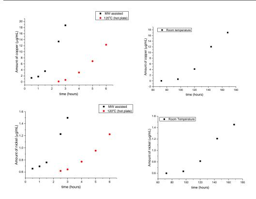
Figure 63: The rates of reaction for leaching of copper and nickel at different conditions: MW environment; heating plates at 120°C and at Room temperature (25°C).
