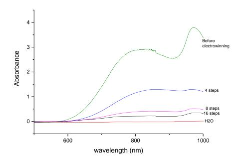
**Figure 69:** UV-Visible spectra of Cu-Ni alloy taken after various steps of electrowinning process. Each electrowinning step lasted 3 minutes at 3V.
