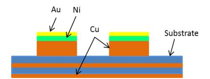
**Figure 43**: A schematic one-sided model structure of the PCB finger showing the epoxy resin substrate; multi-layered surface metal plates of Cu, Ni and Au; and internal plates of Cu embedded in the epoxy resin substrate.
