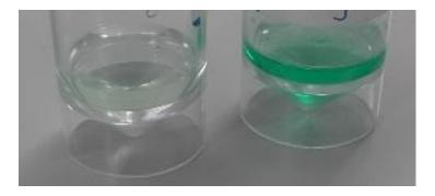
Figure 70: A comparison of electrolytes before and after electrodeposition steps. (left) pale green liquid after 16 electrodeposition steps, each step conducted at 3 V for 3 mins; (right) aqua green liquid before electrodeposition.
