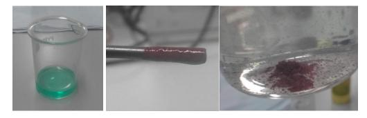
Figure 68: (a) Leachate from Cu-Ni leaching used as electrolyte; (b) Cu-Ni alloy deposited on a graphite electrode after electrodeposition step at 3V for 3mins; (c) Cu-Ni alloy deposits being washed in distilled water.
