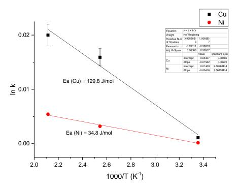
Figure 65: Arrhenius plot used to determine the activation energy for copper and nickel leaching in 1M HCl acid where NH<sub>4</sub>Cl is used as oxidant.
