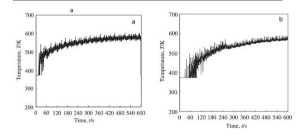
**Figure 13** Change in temperature of sputtered thin film of with a thickness of 34.6 nm during microwave irradiation. b) Change in temperature of evapourated Au film with a thickness of 29.5 nm during microwave irradiation.**[103]**
