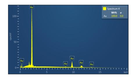
Figure 67: SEM-EDS elemental analysis over an area specified by spectrum
