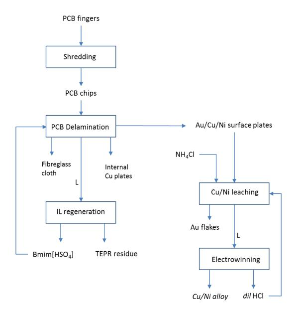
Figure 45: A process flow diagram employed in this study used in the treatment of PCB fingers. It outlines the major separation and recovery steps. Product materials include fibre glass cloth, gold metal flakes, TEPR residue, Cu/Ni alloy.
