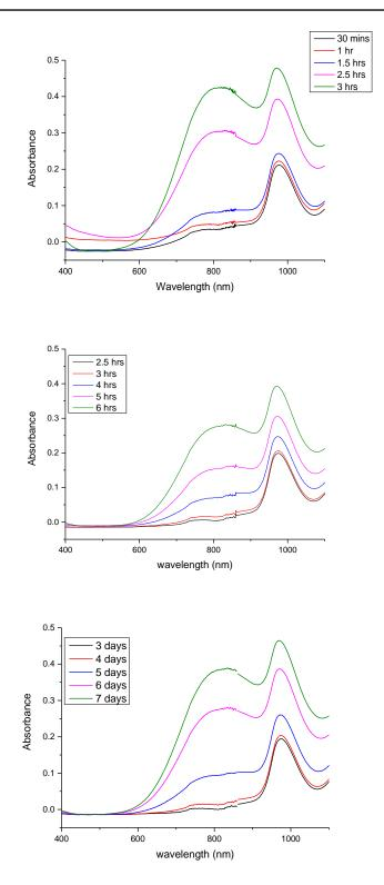
Figure 61: UV-Visible spectra of HCl acid leachate after Cu/Ni dissolution reaction: (a) microwave-assisted leaching; (b) leaching at 120°C; (c) leaching at Room Temperature.
