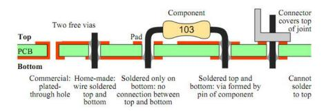
Figure 3: (Top) A multi-layered PCB type showing copper plated holes, copper tracks embedded within polymer substrate and copper surface plates on both faces of the substrate [52]; (bottom) Cross-section of a double-sided printed circuit board showing free vias formed by a plated-through hole and a wire through a non-plated hole soldered top and bottom [53].
