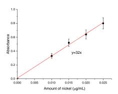
Figure 62: Calibration plots based on Beer-Lambert Law that relates the Absorbance from UV-Visible spectra to the Amount of substance or concentration dissolved (µg/mL).
