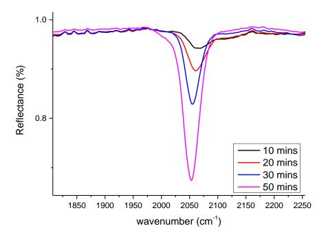
**Figure 55:** Lone peak at 2048, characteristic of CN bond, increases in intensity as resident time of delamination reaction is increased.
