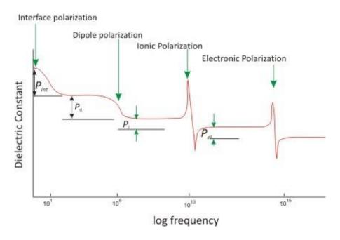
**Figure 36:** Schematic figures between dielectric constant verses frequency showing various mechanisms [146].
