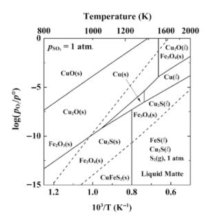
**Figure 9:** Predominance-area diagram system showing principal compounds formed by oxidation of chalcopyrite at various temperatures and oxygen pressures [75].
