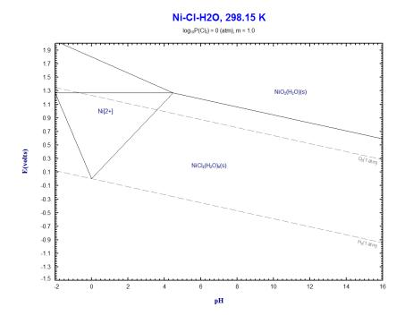
**Figure 60:** Eh-pH diagrams of Ni-Cl-H<sub>2</sub>O system corresponding to eqn. 26.
