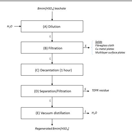
**Figure 51:** A flow chart of bmim[HSO<sub>4</sub>] regeneration process showing the various steps of the process namely; dilution, filtration, decantation, separation/filtration and vacuum distillation.
