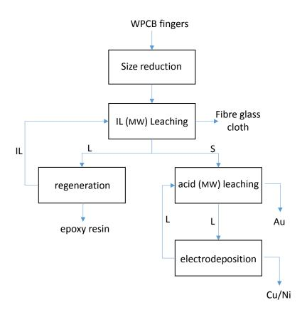
Figure 1: A green and novel route to separating waste PCB fingers.
