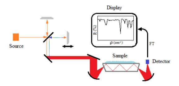
**Figure 20:** Schematic of ATR-FTIR spectrometer showing how the IR beam interacts with the surface of the sample without penetrating into it [132].
