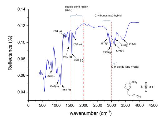
**Figure 30:** Fourier Transform Infre-red (FTIR) spectra for Bmim[HSO<sub>4</sub>]. (a) S=O stretching (b) antisymmetric SO<sub>2</sub> stretching (c) SOH bending.
