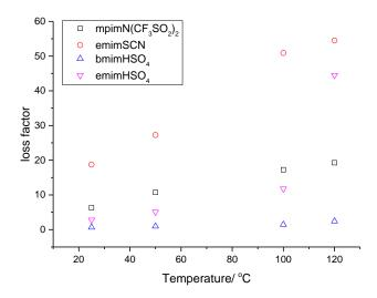
Figure 37: Effect of temperature on the dielectric properties of the measured ionic liquids at 2.45 GHz frequency; (top) dielectric constant against temperature, (bottom) dielectric loss factor against temperature.
