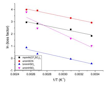
**Figure 38:** Arrhenius plots of the dielectric properties of the imidazolium-based ionic liquids measured at 2.45 GHz.
