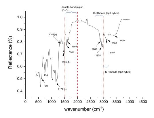
Figure 33: Fourier Transform Infre-red (FTIR) spectra for emim[HSO<sub>4</sub>]: (a) S=O stretching; (b) antisymmetric SO<sub>2</sub> stretching; (c) SOH bending.
