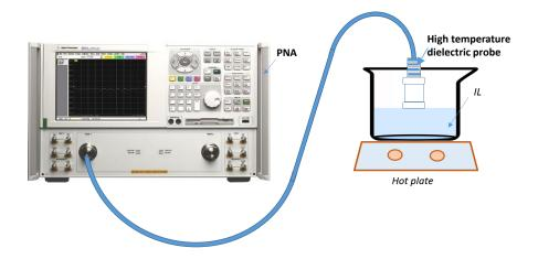
**Figure 27:** PNA frequency sweep mode of measurement; A hot plate is used to vary the temperatures (25, 50, 100 and 125 °C) of the ILs as the measurement is conducted. The probe just touches the surface of the liquid.
