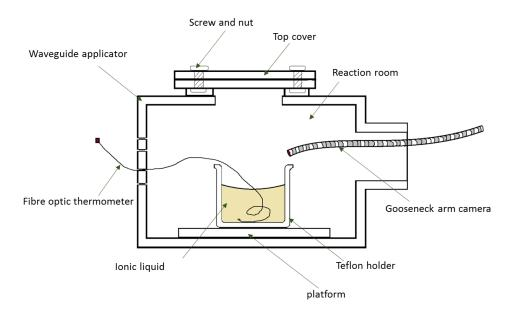
Figure 26: Microwave applicator setup showing the Teflon holder.
