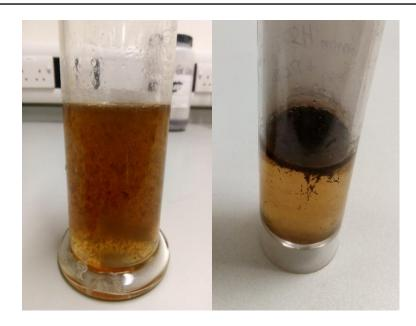
**Figure 49:** H<sub>2</sub>O diluted Bmim[HSO<sub>4</sub>] leachate after delamination process: (left) leachate after sieving out the surface plates, internal plates and fibreglass cloth reinforcement; (right) decanted leachate after sitting for 1 hour.
