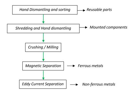
**Figure 7** The pre-processing of e-waste to separate the metal and non-metal fractions
