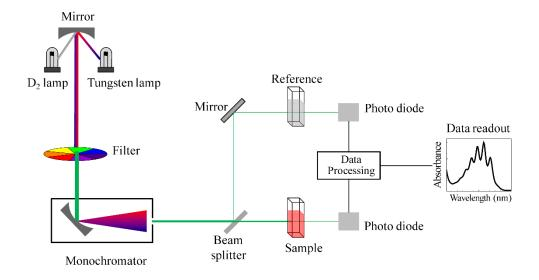
**Figure 22:** Schematic of UV-visible spectrometer showing the working principle [134].
