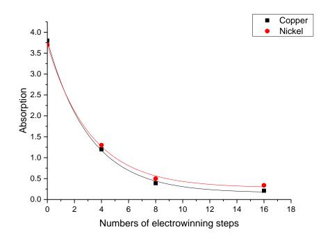
**Figure 71:** A decreasing concentration of copper and nickel after electrowinning steps.
