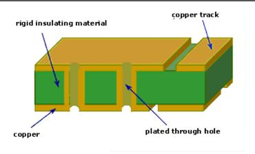
**Figure 2** A single-sided (top) and a double sided (bottom) PCB board types showing copper through holes and plating either or one side of the polymer substrate or on both sides [52].
