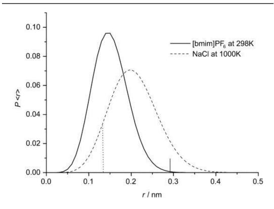
Figure 18: Probability distribution for holes in [bmim]PF<sub>6</sub> at 298 K and NaCl at 1000 K. Vertical lines show the average ionic radius of the ions.
