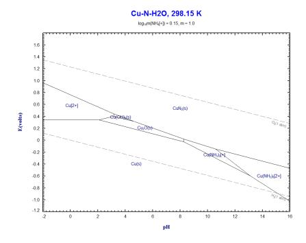
**Figure 59:** Eh-pH diagrams of Cu-N-H<sub>2</sub>O system corresponding to eqn. 25.
