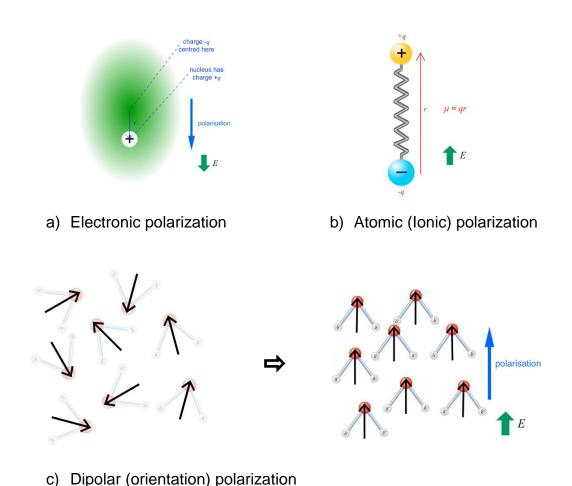
Figure 35 Schematic of mechanisms of polarization
