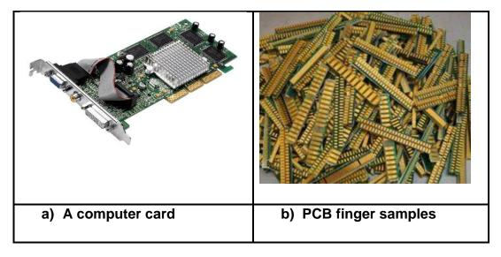
**Figure 19** (a) A typical computer PCB card; (b) PCB fingers ripped off from several computer cards.
