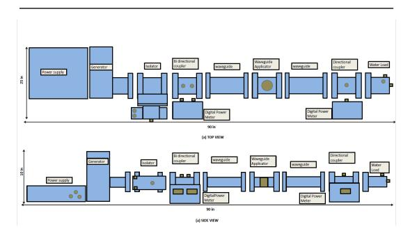
Figure 24: 1.8 KW microwave heating equipment block diagram
