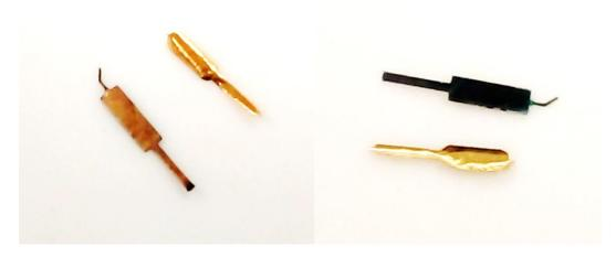
Figure 58: A comparison between a rigid multi-layered surface plate before leaching and a gold flake after leaching reaction: (a) a top view of the surface plate compared to a gold flake; (b) a bottom view of the surface plate compared to a gold flake after leaching away copper and nickel layers.
