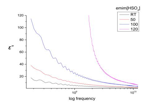
**Figure 75** A temperature-dependant frequency sweep reading of microwave properties at an isotherm, maintained at (25, 50, 100 and 125°C) by using a hot plate. Both the microwave dielectric constant and loss factor increase as temperature is increased
