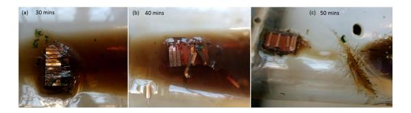
**Figure 47:** Dissolution of FR4 epoxy resin and detachment of surface metal plates of PCB fingers in bmim[HSO<sub>4</sub>] liquid after (a) 30 minutes; (b) 40 minutes; (c) 50 minutes.
