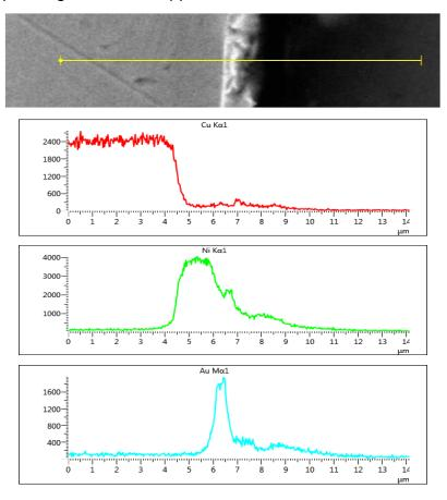
Figure 42: Line scan across a surface metal plate of the PCB finger showing three plated layers of metal; Copper, Nickel and Gold.
