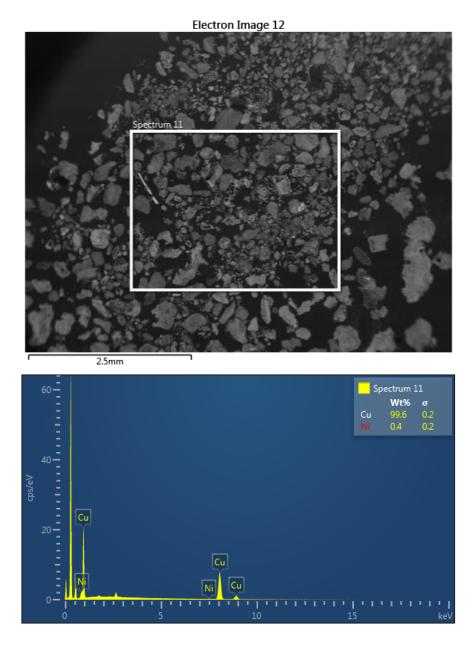
**Figure 73:** SEM-EDS elemental analysis of copper-nickel powder obtained from electrowinning technique. An alloy of 99 wt% Cu and 0.4 wt% Ni was discovered.
