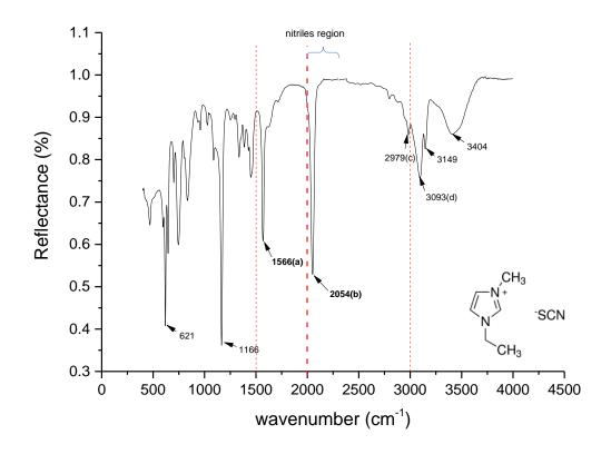
**Figure 32:** Fourier Transform Infre-red (FTIR) spectra for Bmim[HSO<sub>4</sub>]. (a) C=C stretching vibrations (b) SCN group stretching (c) C-H stretching from imidazole ring.
