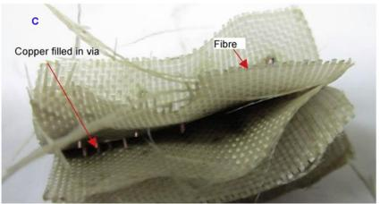
Figure 17 Photograph of waste PCB treated by the emim[BF<sub>4</sub>] at 260°C after 20 min [119].
