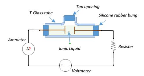
**Figure 23:** A T-glass tube with electrical circuit used to measure the electrical conductivity of the ionic liquids
