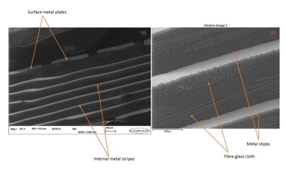
**Figure 39:** a) cross-sectional image of a PCB finger indicating the surface metal plates and the internal metal plates. b) A zoomed-in image of the polymer substrate of a PCB finger showing the fibre glass reinforcement and internal metal stripes.
