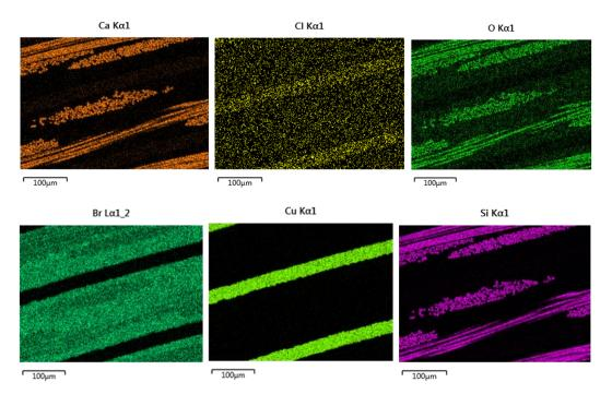
Figure 41: Mapping of surface elements from Figure 39b obtained by EDS analysis.
