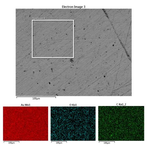
**Figure 66:** A SEM-EDS elemental mapping of the recovered gold metal from waste computer PCB fingers.
