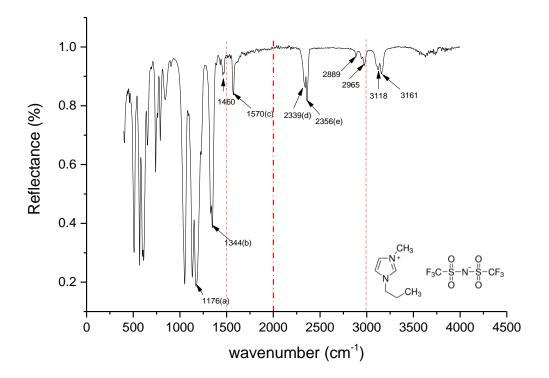
**Figure 31:** Fourier Transform Infre-red (FTIR) spectra for  $Mpim[(CF_3CF_2SO_2)_2N]$ . (a) S=O stretching, (e) C=C stretching vibrations Compare all these spectra with the literature data
