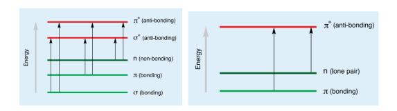
**Figure 21:** (a) The possible electronic transitions that light might cause, (b) electronic excitation following absorption of light, for which very high energy radiation (in the vacuum ultraviolet, <200 nm) is required.
