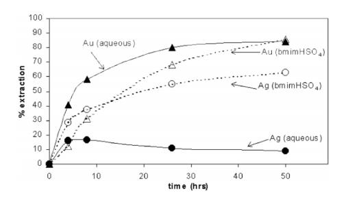
**Figure 15** Comparative leaching of gold and silver from ore using aqueous H₂SO₄ or bmim⁺HSO₄⁻ in the presence of Fe(III) and thiourea **[41]**.
