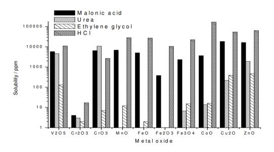
**Figure 14:** Graph showing the solubility of a range of d-block metal oxides dissolved in three different DESs, compared to HCl [118].
