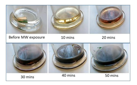
**Figure 46:** Bmim[HSO<sub>4</sub>] liquid changes colour as it dissolves TEPR substrate over time in a 200W, 2.45GHz microwave environment.
