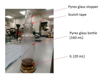
**Figure 28:** *MW-assisted leaching setup for the leaching of epoxy resin from WPCB chips using bmimHSO<sub>4</sub> ionic liquid.*
