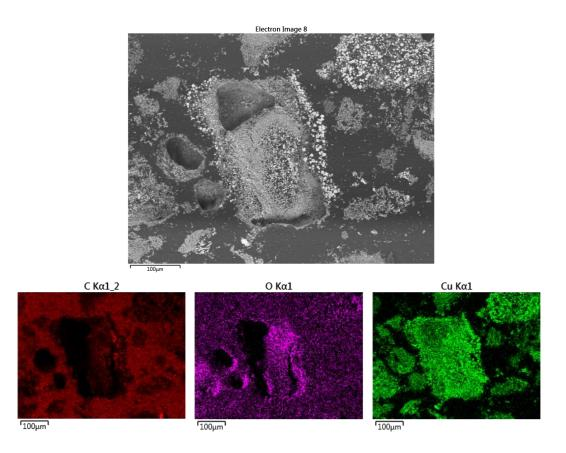
**Figure 72:** SEM-EDS elemental mapping of copper powder obtained after electrowinning technique
