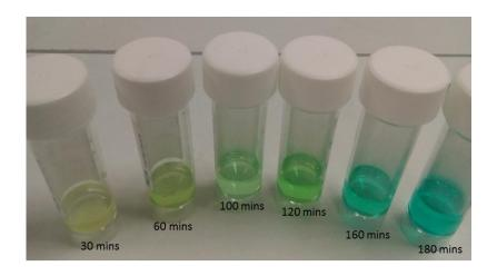
Figure 57: Change of colour of 1.0 M HCI / NH<sub>4</sub>CI leachate solvent during microwave-assisted leaching of copper and nickel. Aqua green colour was achieved at the end of reaction after 3 hours.
