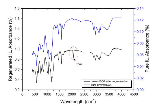
**Figure 52:** An FTIR spectra comparing pure bmim[HSO<sub>4</sub>] to a regenerated bmim[HSO<sub>4</sub>] liquid after delamination process. A new peak at 2048 cm<sup>-1</sup> present in the regenerated IL spectrum shows the presence of CN bond characteristic of the diamine hardener found in the TEPR substrate.
