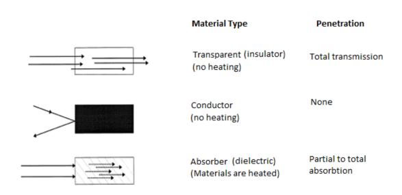
Figure 10 Interaction of microwave with materials [49]
