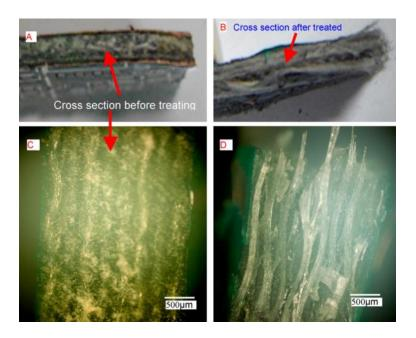
**Figure 16** Photograph (A) and metallographic photograph (C) of cross section untreated WPCBs as well as photograph (B) and metallographic photograph (D) of cross section the WPCBs treated by the emim[BF<sub>4</sub>] at 240°C after 30 min **[119]**.
