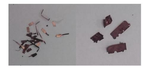
**Figure 56:** (*left*) *multi* – *layered surface plates* (*Au, Ni, Cu*) found on the surface of the TEPR substrate, right) internal copper plates embedded in the TEPR substrate.
