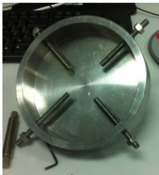
Figure 3-12: Stainless steel rig used on the Instron machine to create a flat platform for the perspex holder to be secured to.
