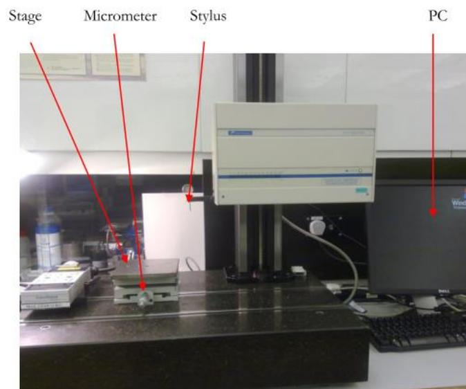
Figure 4-13: Talysurf PGI800 used to measure surface roughness of silicon replicas of cartilage specimens (Russell, 2010).
