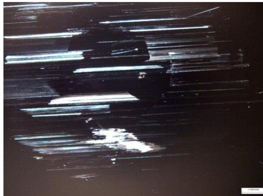
Figure 4-29: Material transfer onto metal plates in post testing condition.
