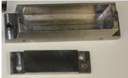
Figure 4-9: A photograph of CoCr plate and bath (Russell, 2010) used for cartilage on metal configurations.
