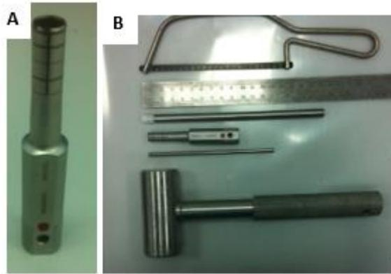
Figure 2-4: Pin removal tools included three separate instruments; A) 8.5mm diameter corer tool; B) Summary of all tools used during pin extraction, from bottom up – hammer, 4 mm diameter rod, corer tool, 8 mm diameter stainless steel rod, ruler and small saw for removing excess bones attached.
