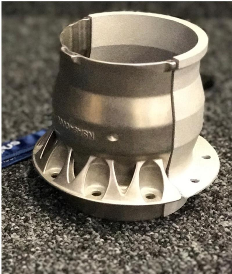
Figure 20 - A400M Bulkhead Seals - Original (right) and design for AM (left)
