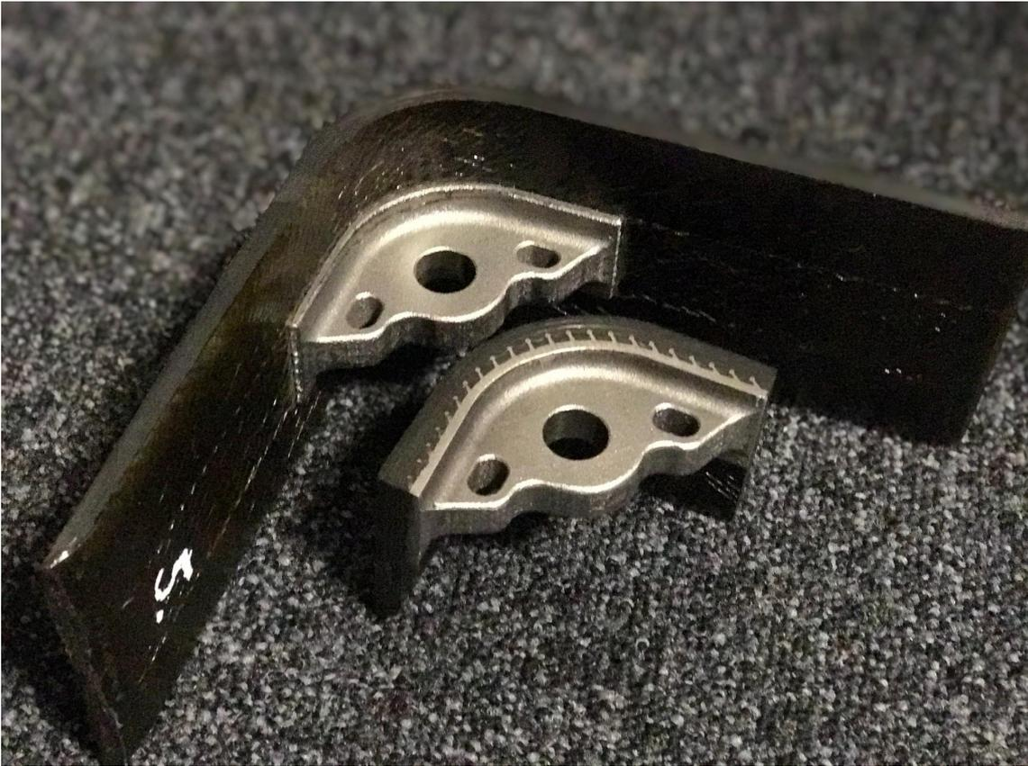
**Figure 14 - HYPER pins embedded into CFRP leading edge wing skins**
