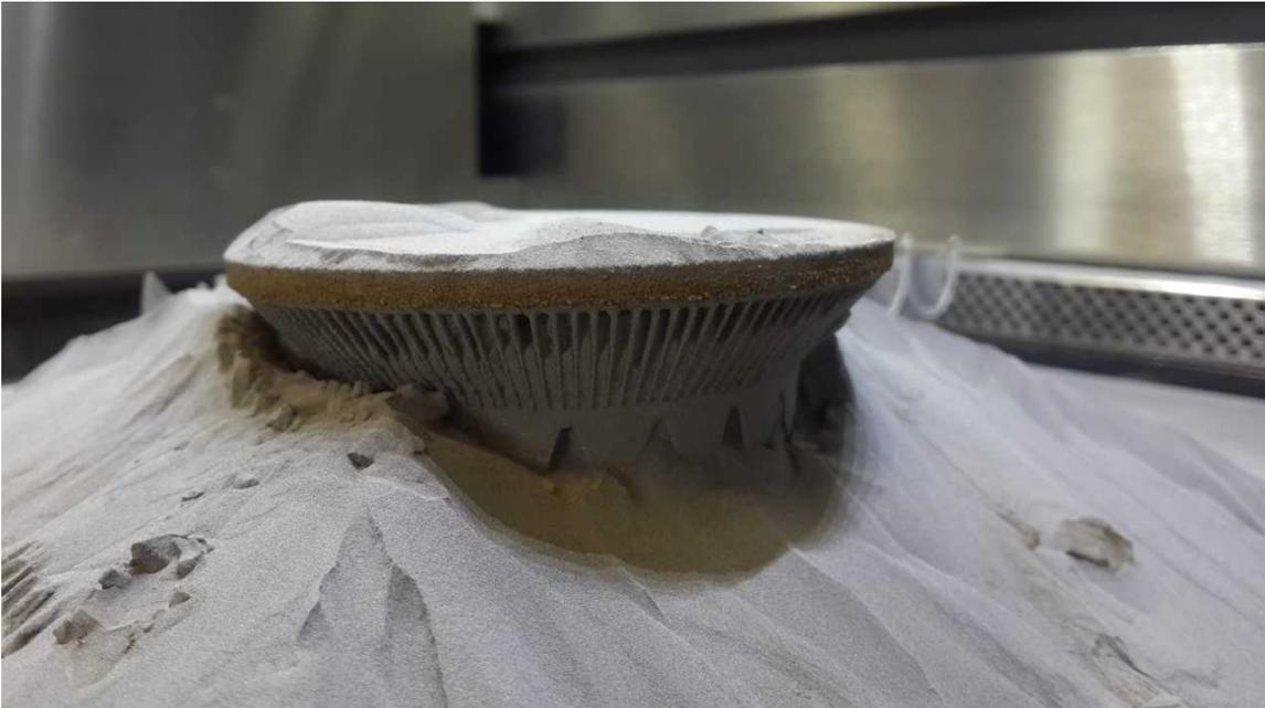
**Figure 16 - Overheating of the deposit caused by a combination of inadequate thermal dissipation and fast scan and recoating strategies**
