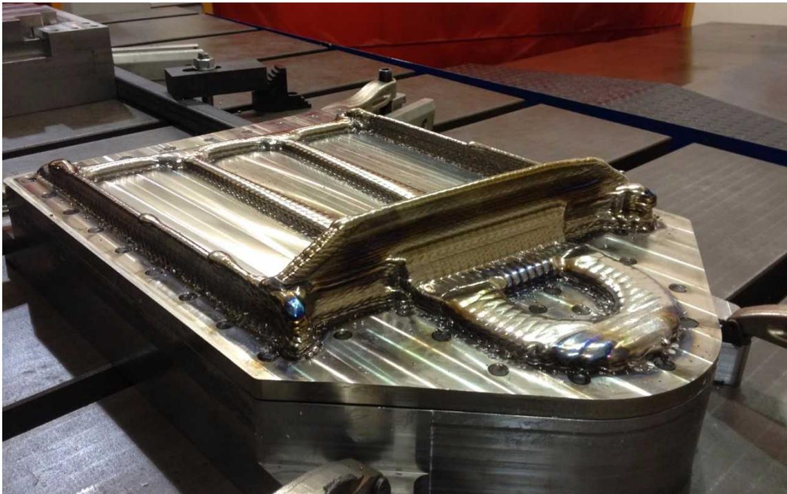
**Figure 8 - Similar component stress, relieved on its own build plate and tooling - now almost completely flat**
