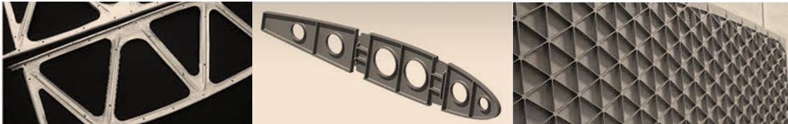
**Figure 24 – Aircraft rib development in-line with loading and performance requirements and the development of better analytical techniques**
