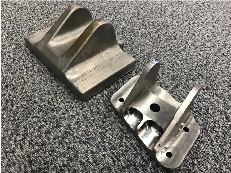
**Figure 2 - Near-net shape forging (top) and the machined part extracted from the forging (bottom)**
