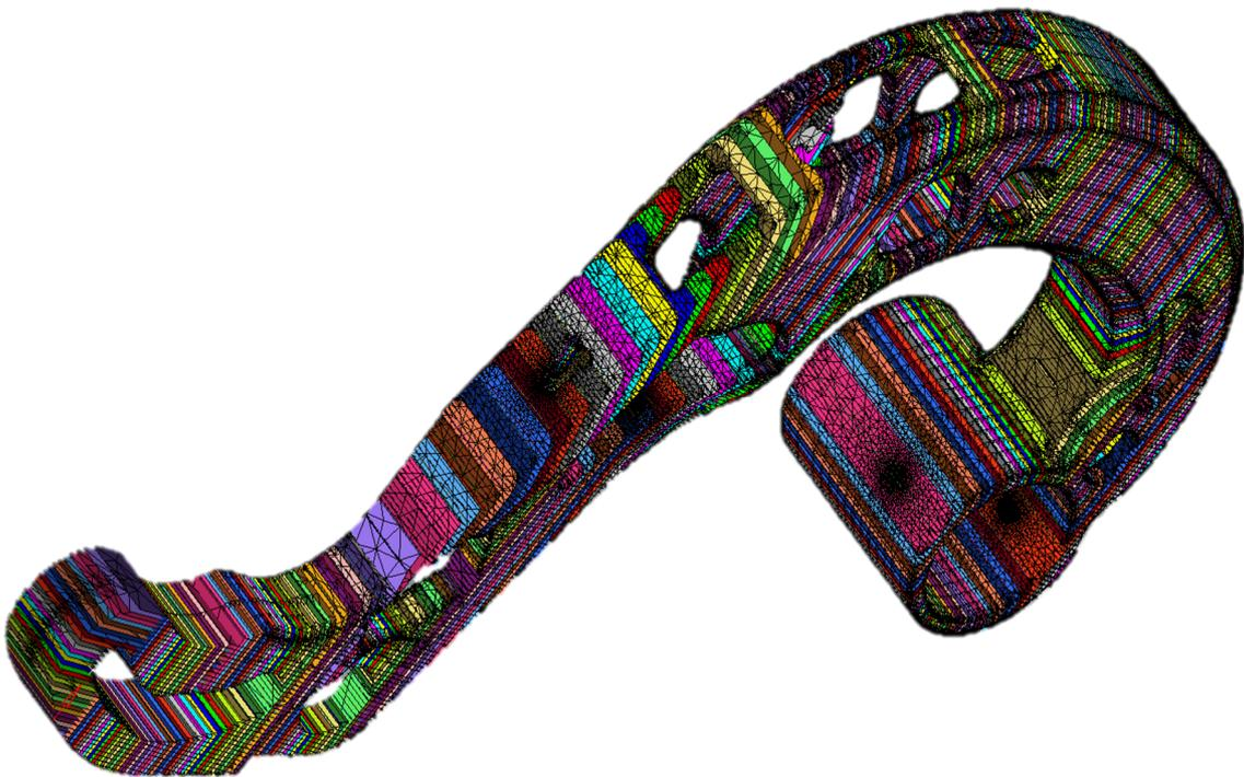
**Figure 5 - A coarse representation of a 3D CAD part sliced into 2D planar profiles.**
