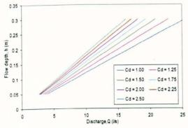
Figure 8-7 Flow depth predictions using different  $C_d$  (using James et al., 2004 equation)
