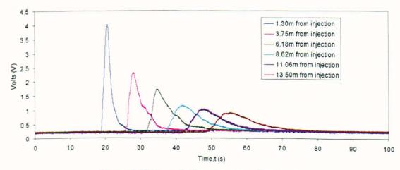
Figure 5-22 Example Raw data from fluorometers
