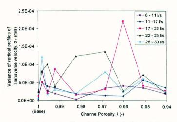
Figure 7-48 Variance of transverse profiles of velocity with channel porosity in growing Carex
