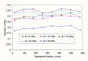
Figure 7-20 Transverse profile of primary velocities (Base Case)
