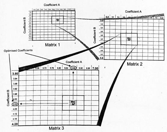
Figure 2-16 Three matrix optimisation procedure (adapted from Dennis, 2000)
