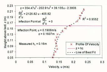
Figure 7-44 Determination of inflection point in vertical profile of velocity (Week 7 Carex, Q = 29.5l/s)
