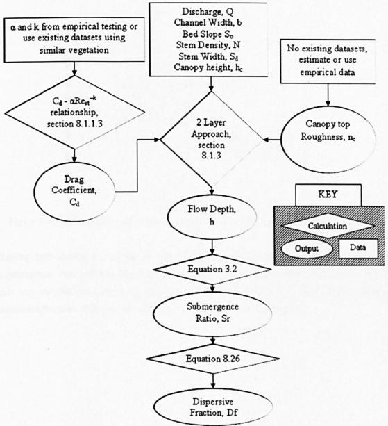
Figure 8-45 Methodology for predicting dispersive fraction in submerged vegetated flow
