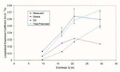
Figure 8-37 Prediction of dispersion coefficient from Murphy et al. (2007) (Equation 8-20) compared to measured values in 5.5cm cropped Carex case.
