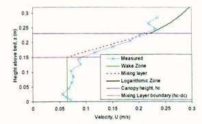
Figure 8-33 Measured and predicted vertical profile of velocity (Cropped to 25cm)
