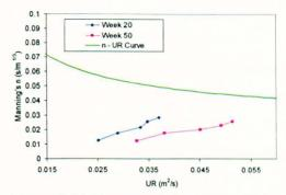
Figure 8-22 Comparison between n-UR curve and measured Carex data
