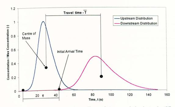
Figure 2-15 Downstream concentration profile at each time step calculated using the ADZ model and two coefficients ( $\tau$  and  $\overline{T}$ )
