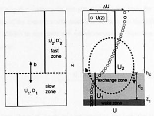
Figure 3-5 2-Zone model applied to submerged vegetated flow (adapted from Murphy, 2007)
