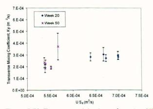
Figure 7-79 Transverse mixing in reeds against US<sub>d</sub>
