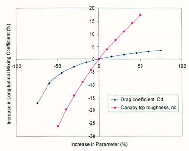
Figure 8-46 Effect of different parameters on dispersive fraction prediction using Equation 8-26
