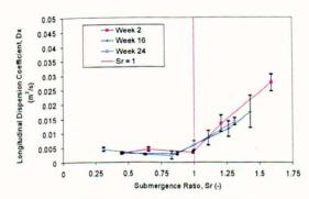
Figure 7-98 ADE dispersion coefficient in growing Carex with submergence ratio
