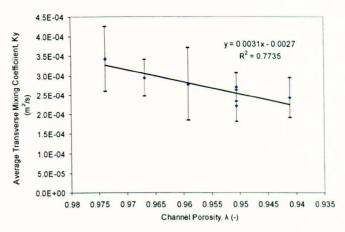
Figure 7-83 Average transverse mixing coefficient against channel porosity
