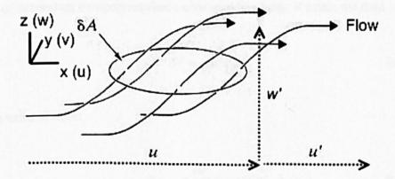
Figure 2-5 Reynolds Stress model (adapted from Chadwick and Morfett, 1994)
