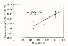
Figure 7-75 Transverse mixing in the base case against flow depth
