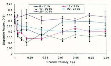
Figure 7-103 Dispersive fraction in growing Carex with channel porosity
