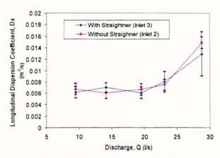
Figure 6-43 Dispersion coefficient in Carex with and without flow straightner
