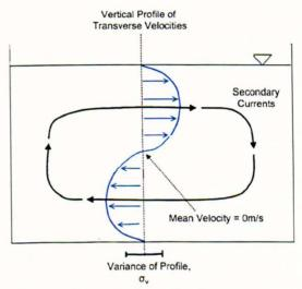
Figure 5-18 Mean and variance of a vertical profile of transverse velocities (theoretical case)
