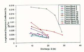
Figure 7-108 Dispersion coefficient against discharge in emergent Carex and reeds
