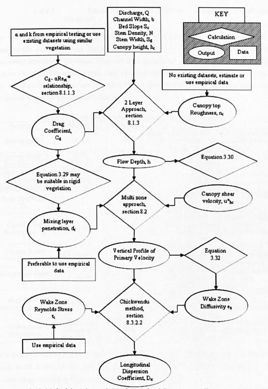
Figure 8-43 Methodology for predicting longitudinal dispersion coefficient in submerged vegetation
