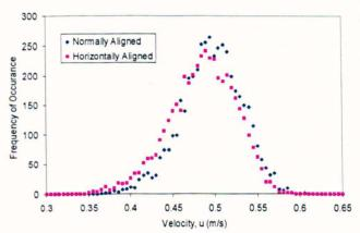
Figure 5-12 Histogram of results from normally aligned and horizontally aligned ADV probe
