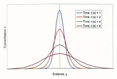
Figure 2-12 Tracer concentration along y axis with time
