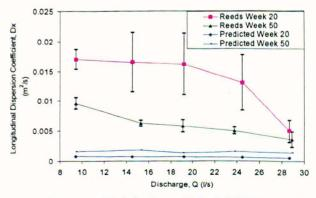
Figure 8-35 Comparison between Lightbody and Nepf (2006) model and measured values of longitudinal dispersion coefficient
