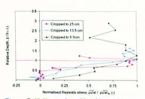
Figure 7-67 Vertical profile of Reynolds stress in growing Carex (Q = 29.5l/s)
