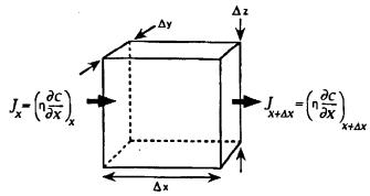
Figure 2-10 Diffusive flux into and out of a small fluid element (adapted from Rutherford 1994)
