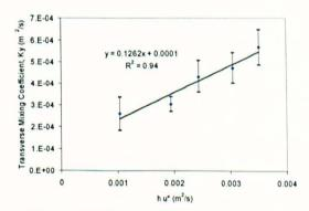
Figure 7-76 Transverse mixing in the base case against hu\*
