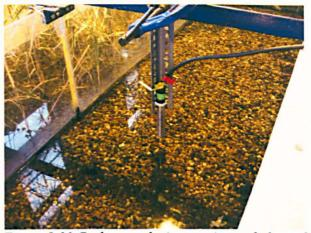
Figure 5-20 Cyclops probe in experimental channel
