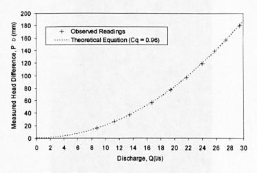
Figure 5-6 Channel pump calibration curve
