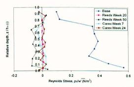
Figure 7-66 Comparison of vertical profile of Reynolds stress in different emergent testing cases ( $Q \approx 20l/s$ )
