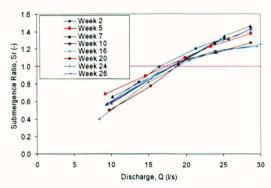
Figure 7-10 Discharge and submergence ratio through Carex
