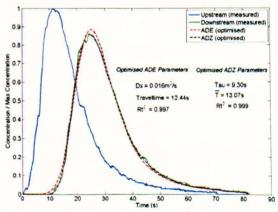
Figure 6-47 Example trace in base conditions (Reach 2, Q= 9.19l/s)
