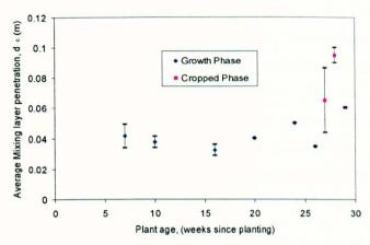
Figure 7-71 Average mixing layer penetration into canopy for each vegetated case
