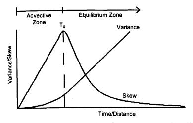
Figure 2-11 Fickian model of changing properties of a concentration profile (Shucksmith et al., 2007).
