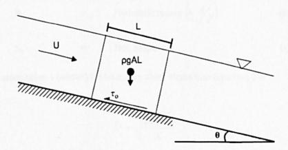
Figure 2-3 Force diagram in uniform flow conditions.
