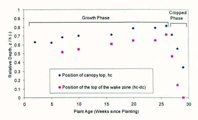
Figure 7-74 Proportion of flow inside the canopy and inside the wake zone for Carex tests conducted at maximum discharge (≈29.5l/s)
