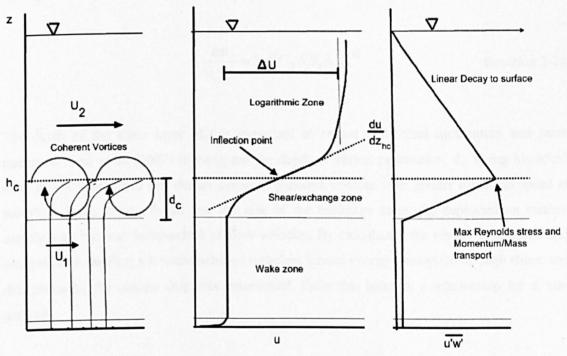
Figure 3-4 Conceptual representation of the mixing layer analogy in submerged vegetated flows
