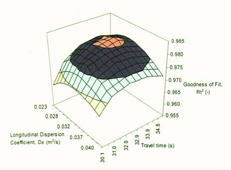
Figure 5-37 Example of how ADE parameters affect the goodness of fit (Rt<sup>2</sup>)
