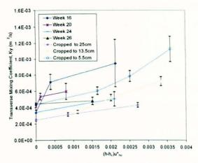
Figure 7-86 Transverse mixing in submerged Carex against (h-h<sub>c</sub>)u\*<sub>hc</sub>
