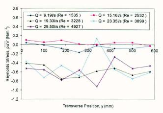
Figure 7-49 Transverse Profile of Reynolds Stress (Base Case)
