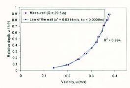
Figure 7-21 Vertical profile of primary velocities (Base Case)
