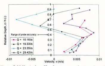
Figure 7-23 Vertical profile of transverse velocities (Base Case)
