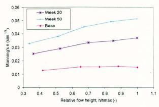
Figure 7-12 Manning's n with flow depth in reeds
