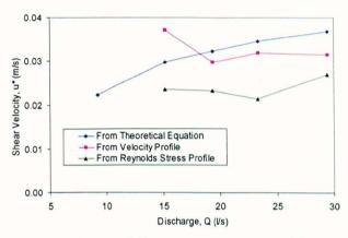
Figure 7-64 Comparison between different measurements of shear velocity (Base Case)
