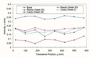
Figure 7-41 Comparison of transverse profiles of primary velocities in different vegetated cases  $(Q \approx 29.5 l/s)$
