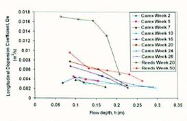
Figure 7-109 Dispersion coefficient against depth in emergent Carex and reeds
