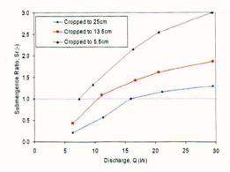
Figure 7-11 Discharge and submergence ratio through cropped Carex
