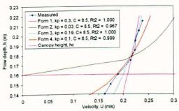
Figure 8-26 Measured and predicted velocity profile above canopy (Week 7 Growth Phase)
