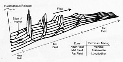
Figure 2-6 Mixing Zones (adapted from Jobson, 1997)
