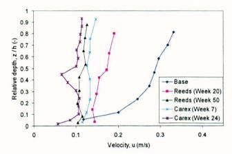
Figure 7-42 Comparison of vertical profile of primary velocities in different emergent vegetated cases ( $Q \approx 20l/s$ )
