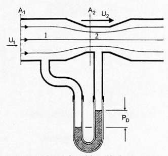
Figure 5-5 Venturi Meter (adapted from Chadwick and Morfett, 1994)
