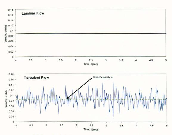
Figure 2-2 Example of velocity measurements in laminar and turbulent flow
