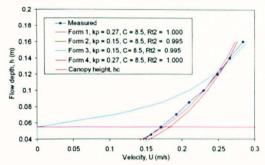
Figure 8-29 Measured and predicted velocity profile above canopy (Cropped to 5.5cm)
