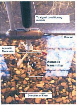
Figure 5-9 ADV Probe in the experimental channel
