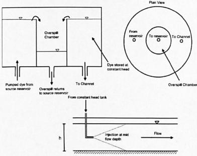
Figure 5-38 Constant injection system schematic
