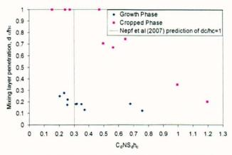
Figure 8-30 Mixing layer depth with  $C_dNS_dh_c$
