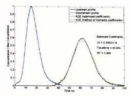
Figure 6-42 Example trace in Carex (With straightner)
