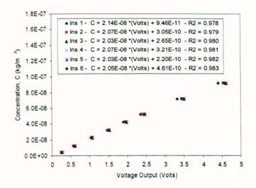
Figure 5-19 Example of six Cyclops-7 fluorometer probe calibration relationships
