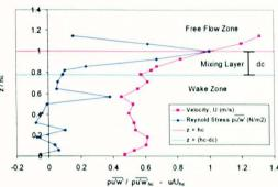
Figure 7-69 Flow Structure in Week 7 Carex Q = 29.5l/s
