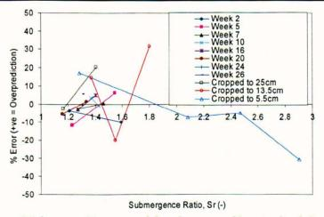
Figure 8-39 error (%) between N-zone model and measured longitudinal dispersion coefficient
