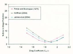
Figure 8-10 Error in flow depth predictions using different  $C_d$  (Week 50 Reeds)
