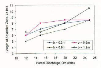
Figure 6-6 Measured length of the advective zone in the experimental channel.
