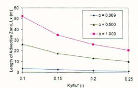
Figure 6-1 Effect of width on advective zone length. Q/b = 30l/sm,  $K_y = 0.13hu*$
