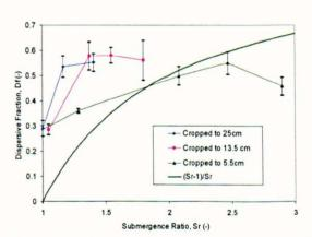
Figure 8-40 Measured and predicted values of dispersive fraction in the growth phase
