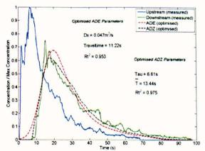
Figure 6-75 Example trace in cropped to 13.5cm Carex (Reach 2, Q= 29.5l/s, submerged conditions)
