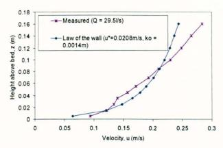
Figure 8-34 Measured and predicted velocity profile above canopy (Cropped to 5.5cm)
