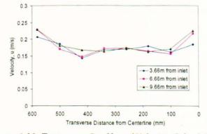
Figure 6-29 Transverse Profiles of Velocity (Inlet 3-Reeds)
