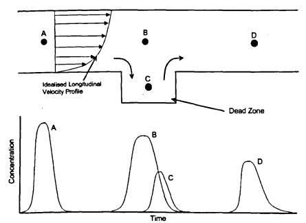
Figure 2-9 Dead Zones in Natural Channels (adapted from Rutherford 1994)
