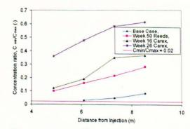
Figure 6-22  $C_{min}/C_{max}$  ratio against distance for different vegetated conditions (Q = 8-10l/s)
