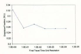
Figure 5-30 Effect of final grid resolution on optimised dispersion coefficient
