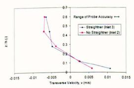
Figure 6-32 Vertical Profile of Transverse Velocities (Reeds)
