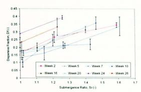
Figure 7-118 Submergence ratio and dispersive fraction (submerged conditions)
