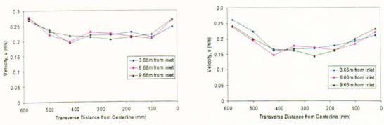
Figure 6-27 Transverse Profiles of Velocity (Inlet 1-Reeds)
