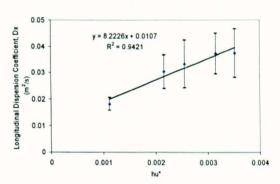
Figure 7-90 Dispersion coefficient in the base case against flow depth
