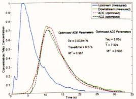
Figure 6-48 Example trace in base conditions (Reach 1, Q = 29.5l/s)
