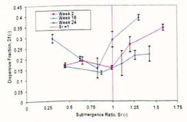
Figure 7-101 Dispersive fraction in growing Carex with submergence ratio
