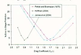
Figure 8-12 Error in flow depth predictions using different  $C_d$  (Week 26 Carex)
