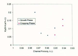
Figure 7-89 Normalised ((h-h<sub>o</sub>) $u^*_{ho}$ ) transverse mixing with porosity
