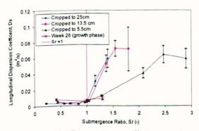
Figure 7-104 Dispersion coefficient against submergence ratio in cropped Carex
