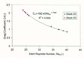
Figure 8-15  $C_d$ -  $Re_{st}$  relationship though Carex ( $C_d$  from Equation 8-5)
