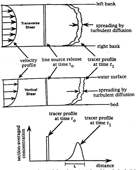
Figure 2-8 Transverse and vertical shear dispersion (adapted from Rutherford, 1994)
