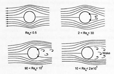
Figure 3-1 Wake formation with increasing stem Reynolds number (from Douglas et al., 2005)
