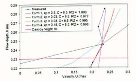
Figure 8-28 Measured and predicted velocity profile above canopy (Cropped to 25cm)
