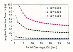
Figure 6-3 Effect of discharge on advective zone length. b = 0.3m,  $K_v = 0.13hu^*$ .
