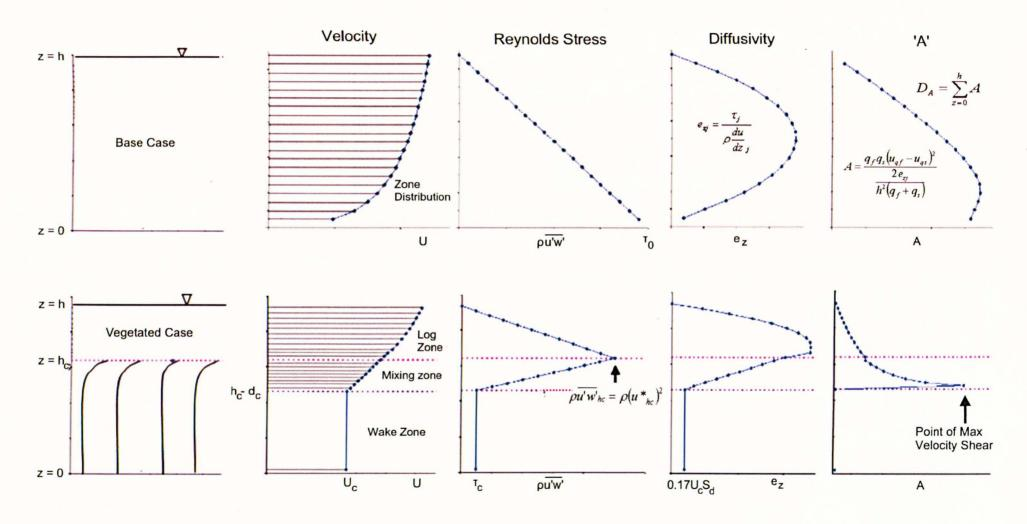
Figure 8-38 N-Zone Chickwendu model applied to plane shear flow and flow through submerged vegetation
