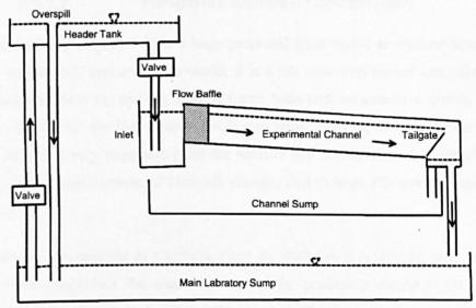
Figure 5-1 Initial Laboratory schematic
