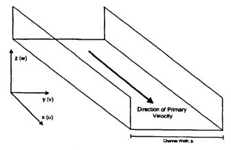
Figure 2-4 Cartesian axes and velocity components relative to an open channel
