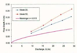
Figure 7-6 Stage discharge through reeds
