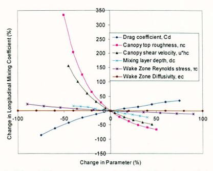
Figure 8-44 Effect of different parameters on longitudinal dispersion coefficient prediction using the methodology outlined in Figure 8-43
