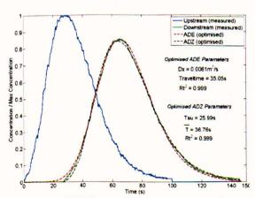
Figure 6-74 Example trace in cropped to 13.5cm Carex (Reach 2, Q= 6.32l/s, emergent conditions)
