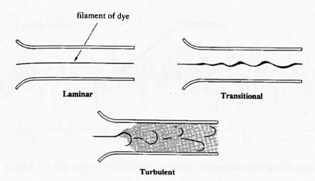
Figure 2-1 Filament of dye in laminar, transitional and turbulent flow (Chadwick and Morfett, 1994).
