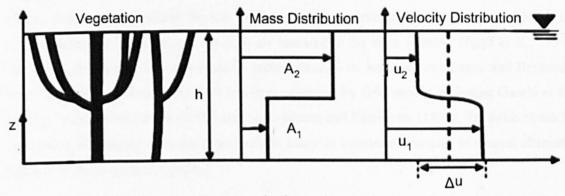
Figure 3-3 Relationship between mass and velocity distribution through emergent vegetation (adapted from Lightbody and Nepf, 2006)
