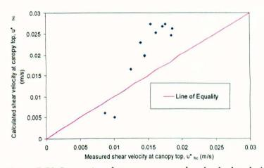
Figure 7-73 Comparison between measured and calculated u\*hc
