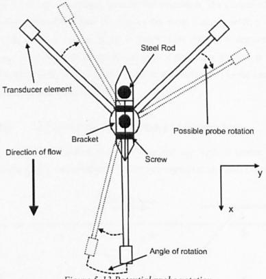
Figure 5-13 Potential probe rotation
