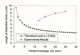
Figure 6-7 Theoretical and Experimental Trend. Q/b = 25l/sm,  $K_y = 0.13hu^*$ ,  $\alpha = 0.069$ .
