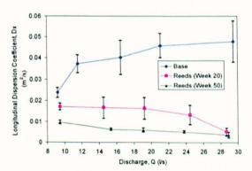
Figure 7-94 Dispersion coefficient in reeds against flow depth
