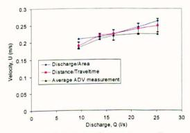
Figure 7-8 Velocity Comparison – Carex (Week 2, submerged at 21.331/s and 25.221/s)
