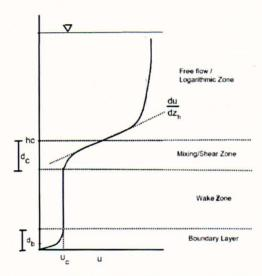
Figure 8-25 Conceptual Model of Vertical Profile of Primary Velocity through Submerged Vegetation
