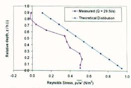
Figure 7-51 Reynolds Stress compared to theory (Base case, Q=29.5l/s)
