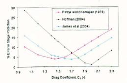
Figure 8-11 Error in flow depth predictions using different  $C_d$  (Week 2 Carex)
