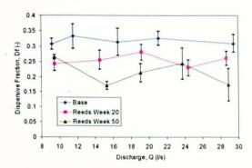
Figure 7-97 Dispersive fraction in reeds against discharge
