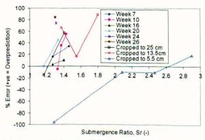
Figure 8-36 error (%) between Murphy (2007) model and measured values of longitudinal dispersion coefficient
