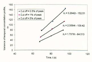
Figure 5-29 Example of how the growth of variance with time is dependent on levels of cut off.
