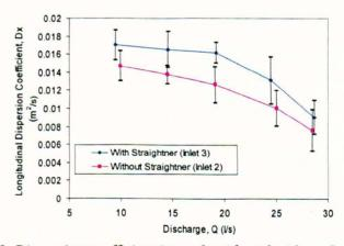
Figure 6-38 Dispersion coefficient in reeds with and without flow straightner
