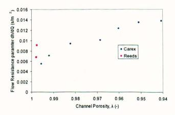
Figure 7-14 Changing flow resistance with porosity
