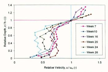
Figure 7-43 Vertical profile of primary velocities in growth phase Carex (Q = 29.5l/s)
