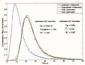
Figure 6-46 Example trace in base conditions (Reach 1, Q= 9.19l/s)
