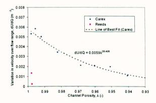
Figure 7-15 Change in velocity over discharge with channel porosity
