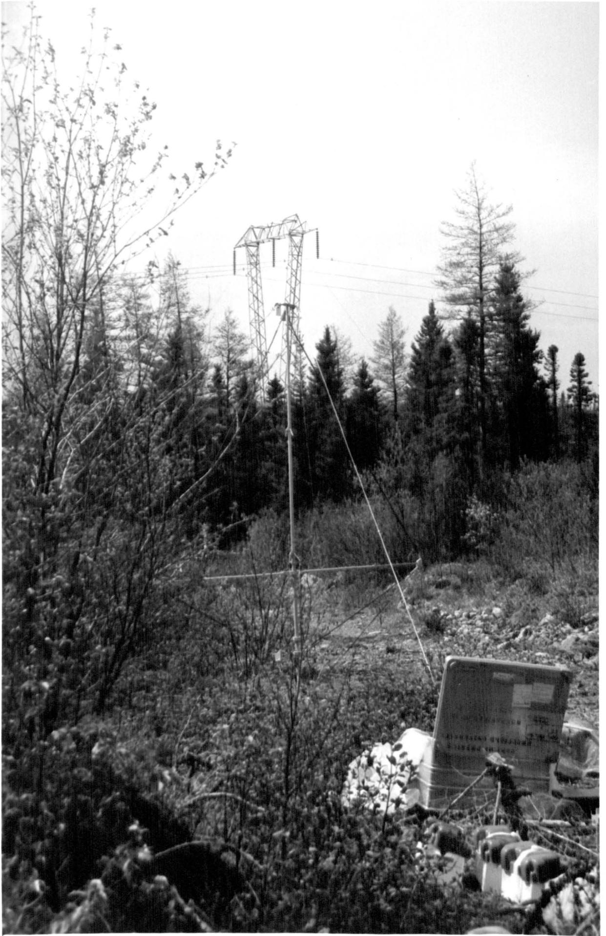
Figure 4.7 . Photograph of the Buchans power line with the loop aerial used at the fixed station.
