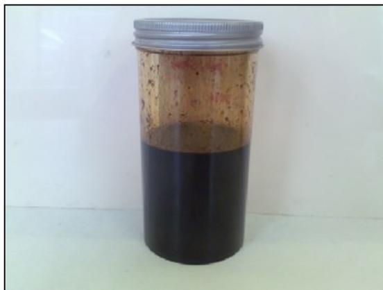
**Figure 7-10:** Liquid obtained from pyrolysis of oil palm stone at 500°C.
