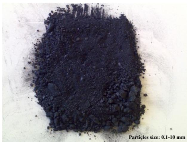
**Figure 7-8:** Char obtained from pyrolysis of PKC at 500°C.
