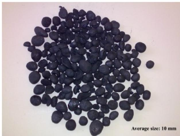
**Figure 7-6:** Char obtained from pyrolysis of OPS at 500°C.
