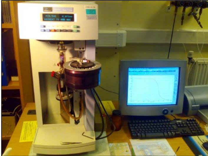
Figure 4-21: Thermogravimetric analyser.
