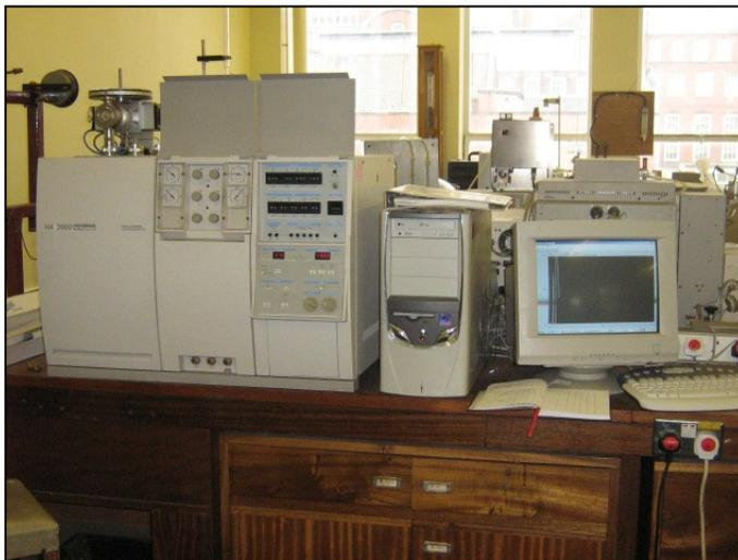
**Figure 4-20:** NA 2000 N-Protein elemental analyser.
