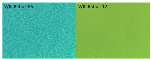
Figure 2.36: Nomarski image of two samples to show improved surface quality with a reduction in the V/III ratio used for the capping layer growth.
