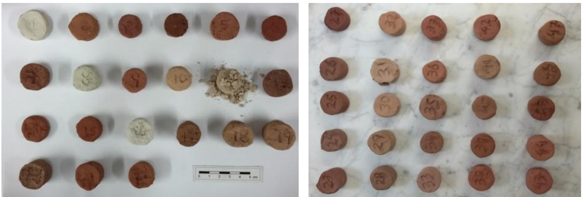
Figure 5.9: The experimental briquettes after the first firing at 700°C.
