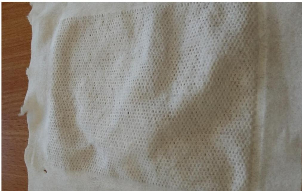
*Figure 6.29: Resulting fabric from compression at 12 tons for the duration of 30 min*
