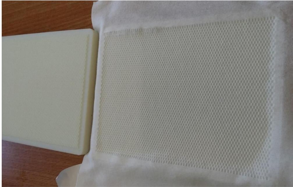
*Figure 6.30: Resulting fabric from compression at 5 tons for the duration of 30 min*
