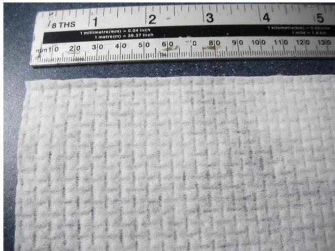
Figure 6.14: Prototype fabric with corrugation
