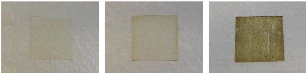
*Figure 6.6: Macroscopic images of the BM smudge for the nominal thicknesses of 123  $\mu\text{m}$  (left), 200  $\mu\text{m}$  (middle) and 450  $\mu\text{m}$  (right)*
