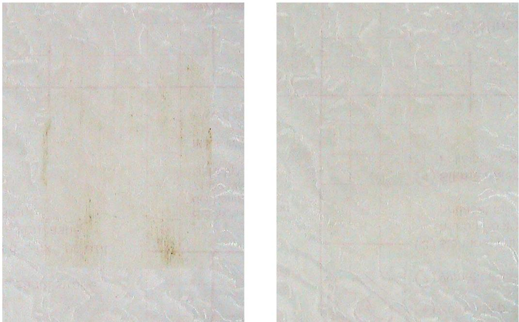
*Figure 6.9: Macroscopic images of the dry-wiped skin mimic surface (left) and the wet-wiped skin mimic surfac (lotion loading 440%) (right)*
