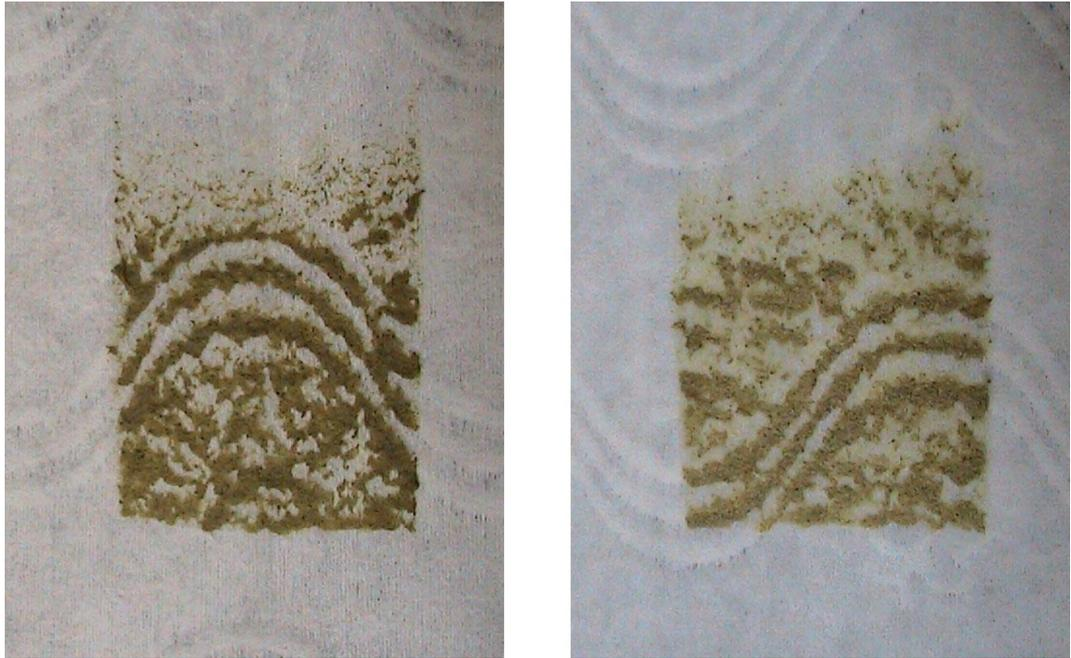
*Figure 6.8: Macroscopic images of the contaminated dry wipe surface (left) and the contaminated wet wipe surface (lotion loading 440%) (right).*
