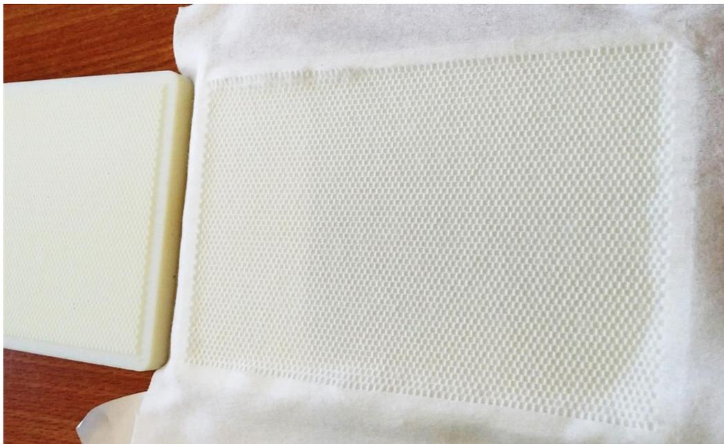
*Figure 6.31: Resulting fabric from compression at  $50 \text{ kg/cm}^2$  for the duration of 30 min*
