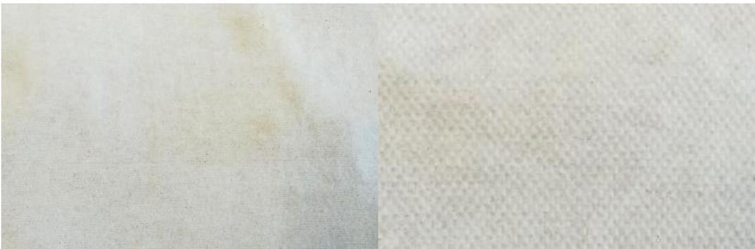
*Figure 6.36: On the left, third wipe of the plain plain hydroentangled fabric. On the right, third wipe of the new structured hydroentangled fabric*
