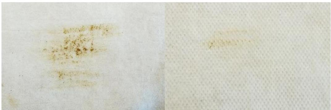
*Figure 6.35: On the left, second wipe of the plain plain hydroentangled fabric. On the right, second wipe of the new structured hydroentangled fabric*
