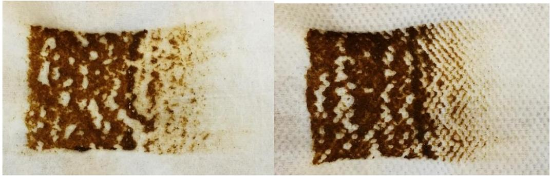
*Figure 6.34: On the left, first wipe of the plain plain hydroentangled fabric. On the right, first wipe of the new structured hydroentangled fabric*
