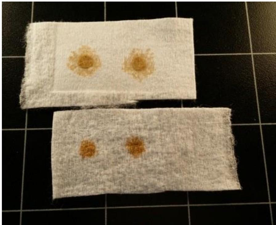
*Figure 4.13: Spread of BM slurry in 90.2% low porosity fabric (top) and 95.6% high porosity fabric (bottom) showing heterogeneous phase separation in the low porosity fabric*
