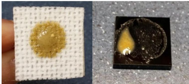
*Figure 4.59: An example of how the specimens appear after the z-direction BM slurry absorption experiment. Left: fabric specimen with a smudge of slurry picked up after contact. Right: plastic plate with residual slurry after contact.*
