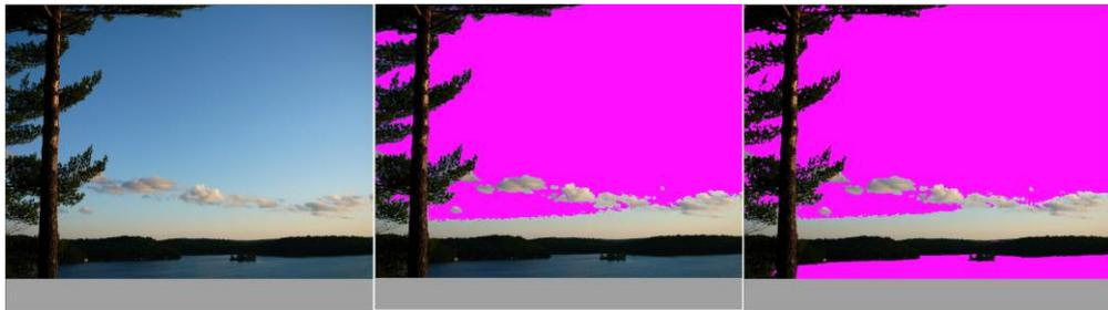
**Fig. 7.2.2-4** A comparison of blue sky detection by an ellipse model and by an ellipsoid model: original (left), detection using an ellipsoid model with 95% coverage rate (centre), and detection using an ellipse model with 95% coverage rate (right).
