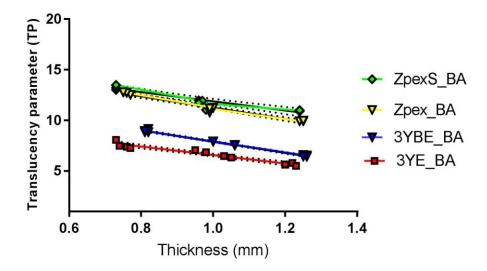
Figure 5-2 Plot of the thickness against translucency parameter (TP) of all groups before aging. All groups can be clearly seen showing a linear relationship, however there are some outliers which can affect the strength of the linearity of the relationship.
