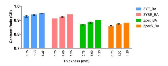
Figure 5-5 Effect of thickness on Contrast Ratio(CR). The bar chart showing clearly the significant difference in the Contrast ratio (CR) for different thickness for each material.
