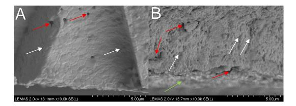
Figure 4-15 SEM images of the fractured surface of Zpex before (A) and after(B)Aging. Hackles indicated by white arrows, pores indicated by red arrows, green arrow indicates area of transformation.
