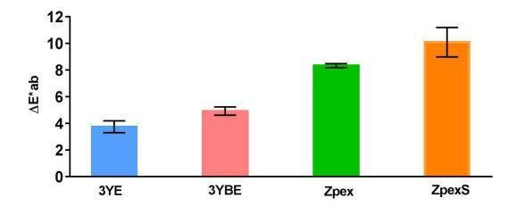
Figure 5-15  $\Delta E^*ab$  Mean +SD of 1.00 mm thickness of all tested groups.
