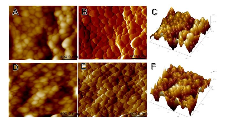
Figure 4-22 AFM for 3YE before and After aging. (a) height sensor BA (b) amplitude view BA (c) 3D view BA (d,e,f After aging).
