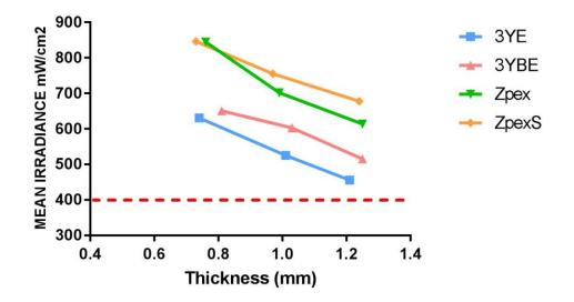
Figure 5-22 Mean light irradiance for all tested materials after aging at various thicknesses. Red line indicates minimum amount of light irradiance required to initiate polymerization.
