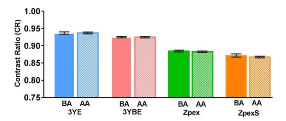
**Figure 5-9 Effect of aging on Contrast ratio (CR).** The bar chart showing there is no significant changes in the CR of all groups.
