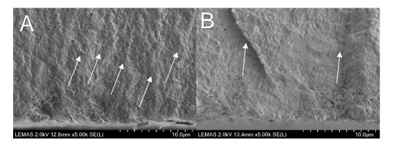
Figure 4-14 SEM images of the fractured surface of 3YBE before (A) and after (B)Aging. Hackles indicated by white arrows.
