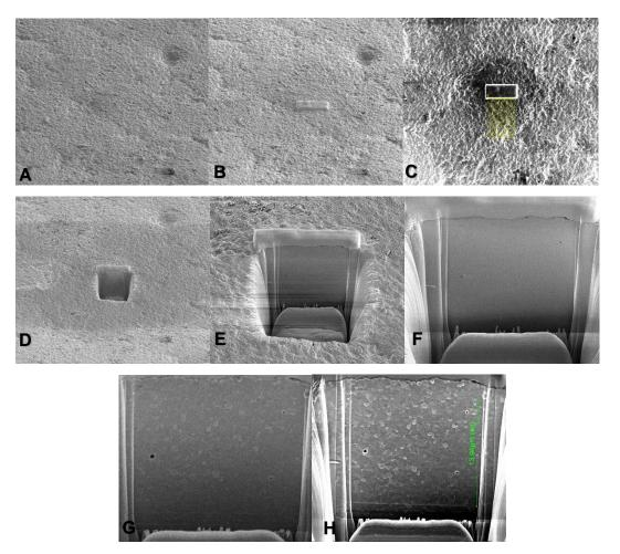
Figure 3-6 Stages of FIB-SEM sample preparation and Imaging (A) Determination of area of interest (B) Platinum layer deposition (C) Area to be milled (D) Bulk removal (E) Bulk removal of depth (F) Cleaning cross section (G) first Ion Beam Image (H) Ion beam immersion image to improve resolution.
