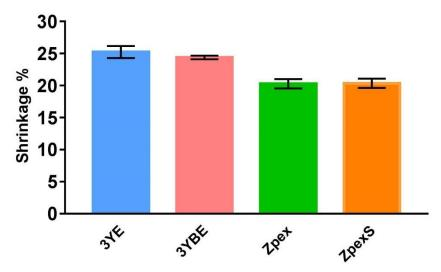
Figure 4-1 Percentage Shrinkage of all materials after sintering.
