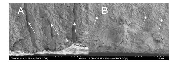
Figure 4-13 SEM images of the fractured surface of 3YE before (A) and after (B)Aging. Hackles indicated by white arrows.
