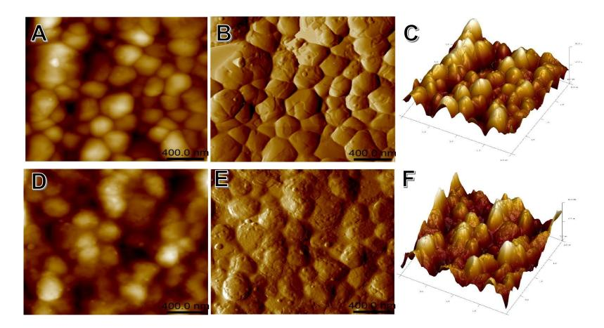
Figure 4-24 AFM for Zpex before and After aging. (a) height sensor BA (b) amplitude view BA (c) 3D view BA (d,e,f After aging).
