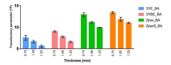
Figure 5-1 Effect of thickness on Translucency Parameter (TP). The bar chart showing clearly the significant difference in the TP for different thickness for each material.
