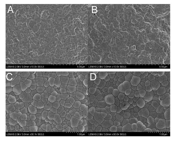
Figure 4-10 SEM images showing the surface topography of 3YBE.
