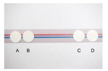
Figure 5-20 Difference in colour before and after aging. (A,B) 3YBE before and after aging,(C,D) Zpex before and after aging.
