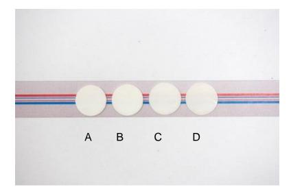
Figure 5-10 The difference in the translucency, 0.75mm thickness. (A) 3YE (B) 3YBE (C) Zpex (D) ZpexS.
