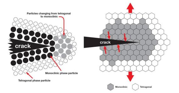
Figure 2-3 schematic representation of crack induced transformation. © Glidewell Laboratories.
