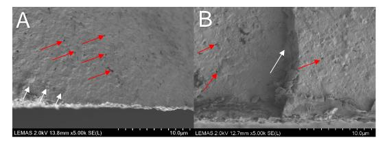
Figure 4-16 SEM images of the fractured surface of ZpexS before (A) and after(B)Aging. Hackles indicated by white arrows, pores indicated by red arrows.
