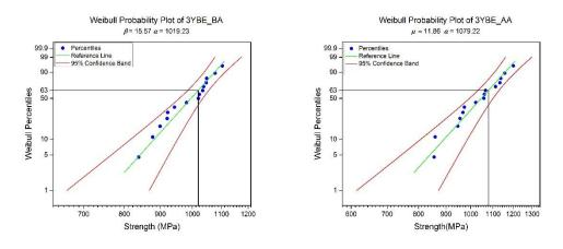
Figure 4-4 Weibull probability plot for BFS data of 3YBE\_BA and 3YBE\_AA. BFS values represented by the blue circles plotted against Weibull percentiles. Characteristic strength (α) was calculated as the load where 63% of samples failed. Upper and lower 95% CI bounds are represented by the red line.
