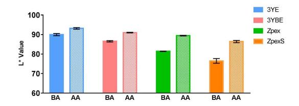
Figure 5-16 L\* mean values+ SD before and after aging.
