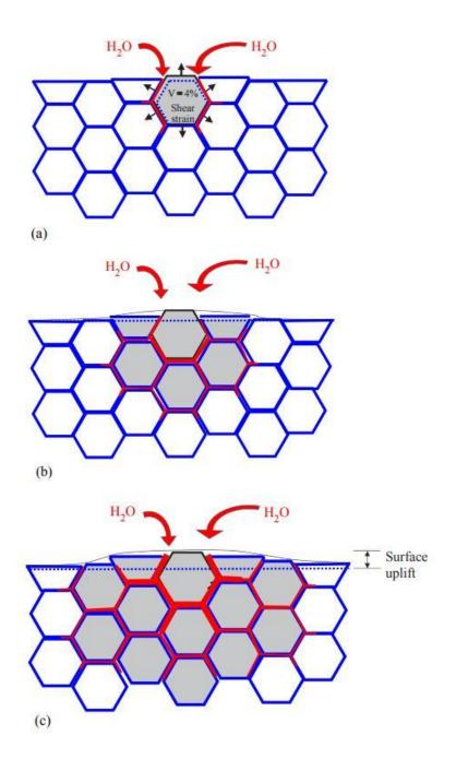
**Figure 2-2 Schematic representation of aging process.** (a) Nucleation on a particular grain (b) Growth of the transformed zone (c) Transformed grains are grey. Red path represents the penetration of water due to micro cracking around the transformed grains (Chevalier, 2006).
