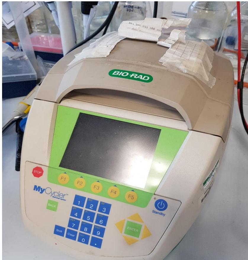
Figure 2.5: MyCycler thermal cycler (Bio-Rad).
