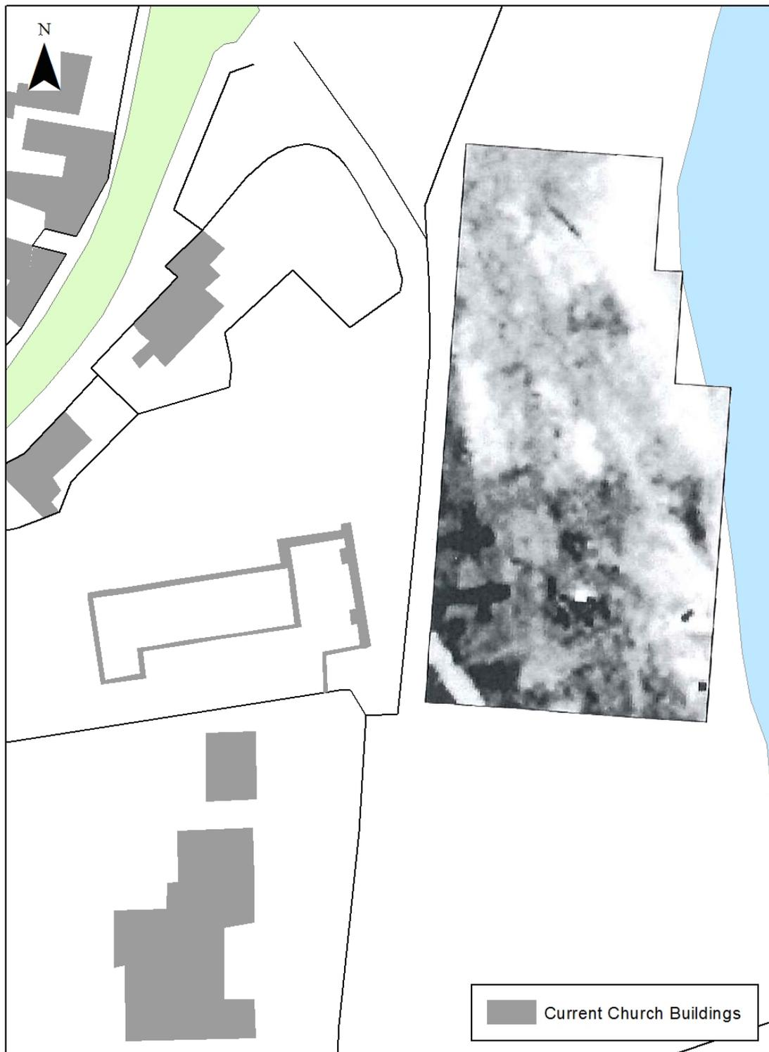
Figure 49 – Geophysical resistivity survey to the east of Old Malton church
