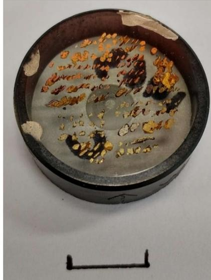
**Figure 6-8:** An example of 25mm gold particle mount. Polishing was conducted until the interior of the gold grains was revealed.
