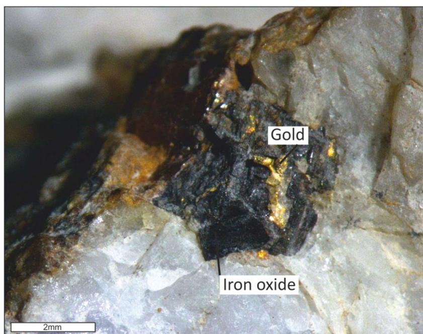
**Figure 6-3:** Visible gold collected from Buckland Zone (BZ07).
