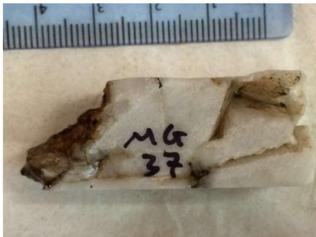
**Figure 6-11:** An example of a sample that has been cut to a chip ready for mounting and polishing.
