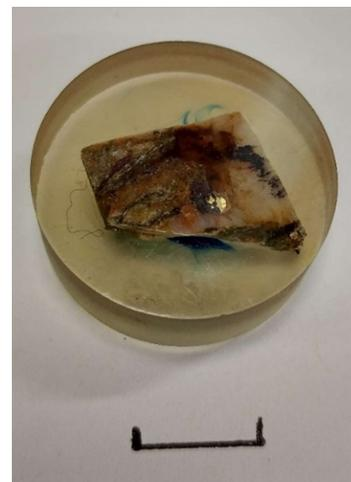
**Figure 6-10:** An example of visible gold mounted in 30mm block that has been polished.
