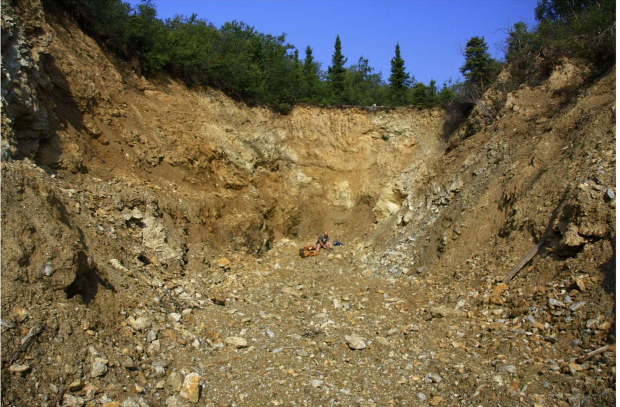
**Figure 7-2:** Boulder Lode mine cut excavated to reveal bedrock and veining.
