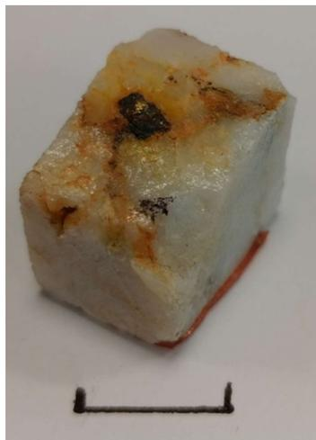
**Figure 6-9:** Visible gold from vein cut down to chip prior to mounting in mould and resin.
