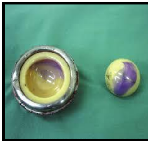
Figure 2.13.Stripe wear in third generation alumina[140].
