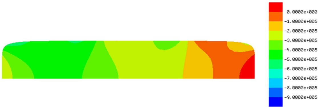
Fig. 4-53 Contour plot of the H-field along the magnetization direction of the PM at rated current operation of the NdFeB SPM machine capable of withstanding demagnetization due to fault.
