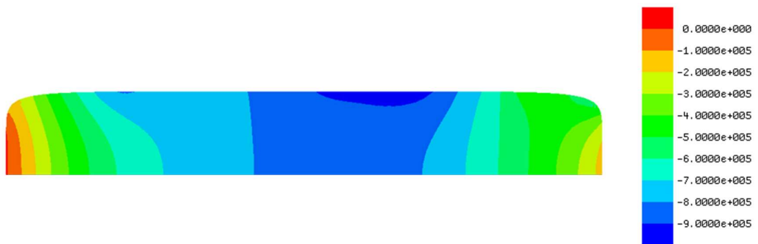
Fig. 4-37 Contour plot of the H-field along the magnetization direction of the PM when H_{min} occurs during the fault transient of the minimum cost NdFeB SPM machine.
