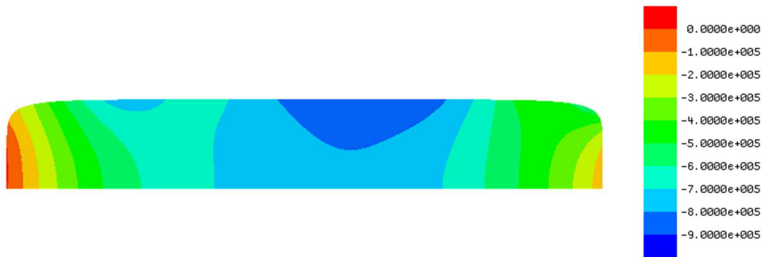
Fig. 4-54 Contour plot of the H-field along the magnetization direction of the PM when H_{min} occurs during the fault transient of the NdFeB SPM machine capable of withstanding demagnetization due to fault.
