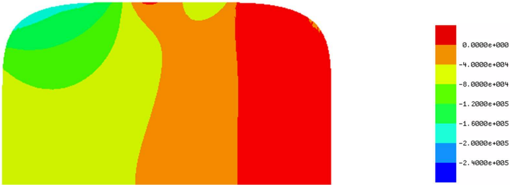
Fig. 4-67 Contour plot of the H-field along the magnetization direction of the PM at rated current operation of the ferrite SPM machine capable of withstanding demagnetization due to fault.
