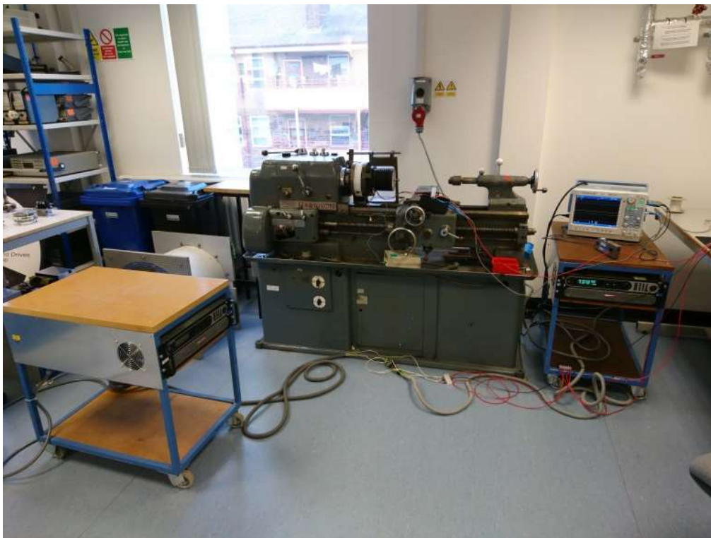
Fig. 5-58 Experimental setup part 2: Lathe, two power supplies and connections.
