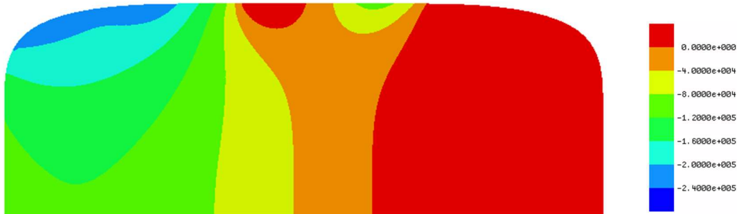
Fig. 4-45 Contour plot of the H-field along the magnetization direction of the PM at rated current operation of the minimum cost ferrite SPM machine.
