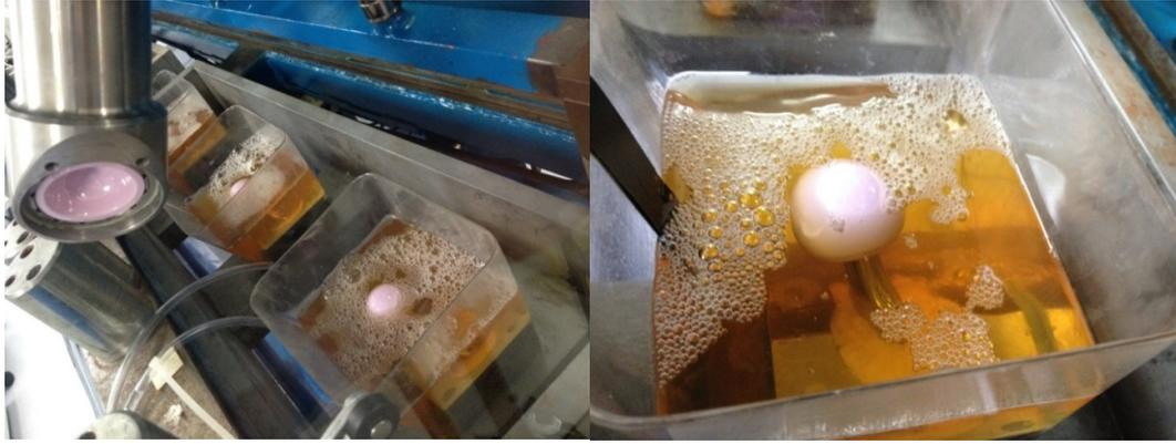
Figure 2-11. Leeds Hip Simulator with lubricant serum applied on the stations
