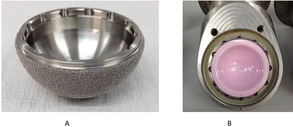
Figure 2-3. PINNACLE® shell (A) and, ceramic liner inserter in the cup fixture (B).
