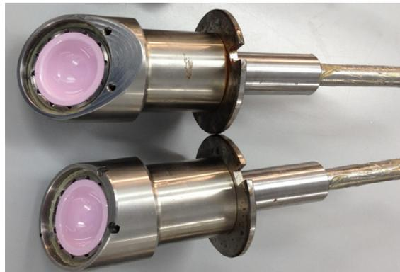
Figure 2-4. Two designs of cup the fixtures, top is 65° and bottom is 45° inclination angle.
