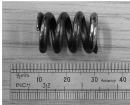
Figure 2-9. Photograph of a spring used in these studies to illustrating geometrical-end finish.
