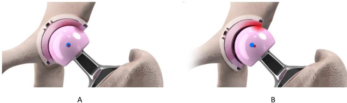
Figure 6-1. Schematic demonstrating a higher dynamic separation under the same translational mismatch for a low (A) and high (B) cup inclination angle.
