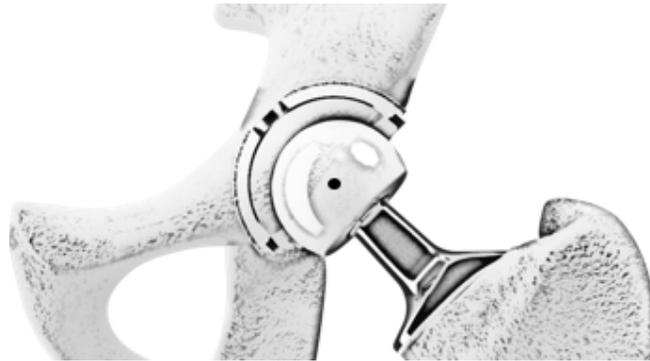
Figure 3-1. Schematic of the acetabular cup and femoral head conforming to each other at the hip joint centre set by the cup position.
