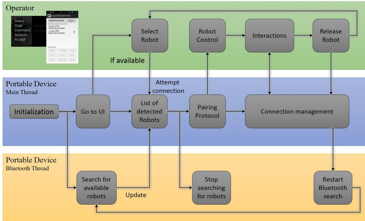
Fig. 3.3 User interface software architecture representation.
