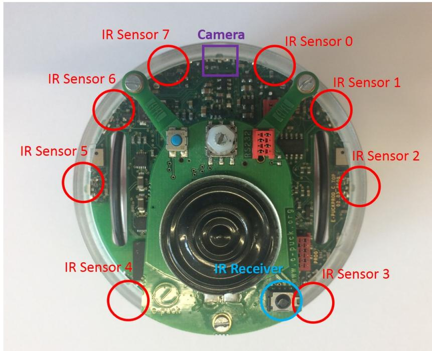
Fig. 3.2 A picture of the real epuck taken from the top. In it, the location of every IR proximity sensor, the IR receiver and the color camera are marked.
