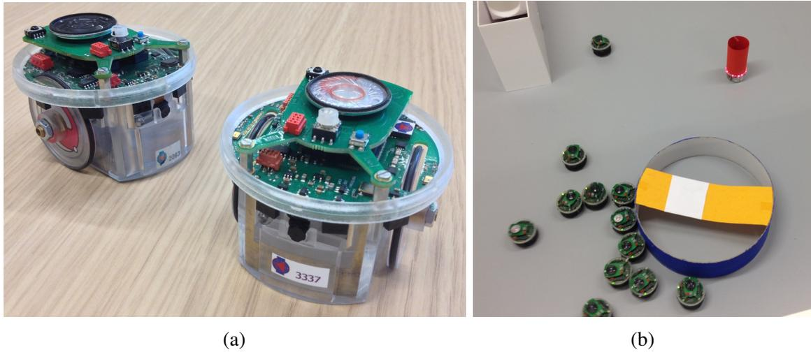
Fig. 3.1 (a) The real e-puck robot. (b) A group of e-puck robots pushing the object towards the (red robot) dynamic goal.
