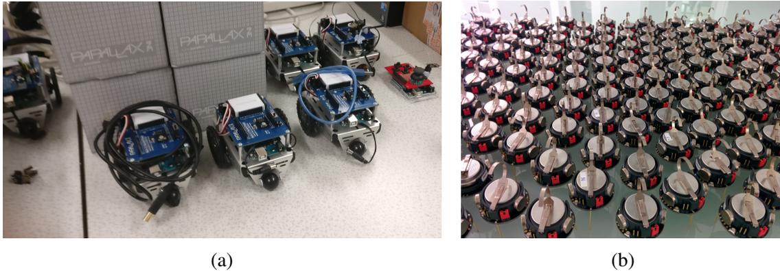
Fig. 2.3 a) A small group of Boe-Bot robots that will work as a swarm. b) A group of Kilobot robots belonging to the 900 robots swarm from The University of Sheffield.
