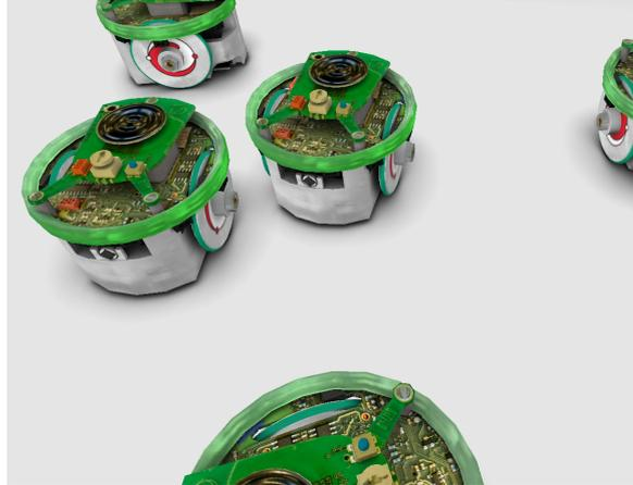
Fig. 4.1 The e-puck miniature mobile robot in the simulation.
