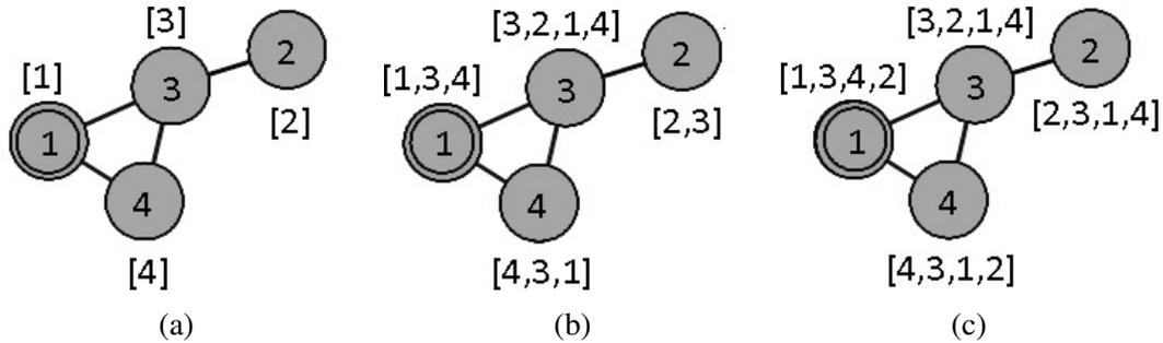
Fig. B.1 Example of robots counting (lines denote pairs of robots within communication range). (a) Initially, only their own ID is in the list. (b) The robots include the IDs received by their neighbors. (c) After a further iteration, each robot contains everyone's IDs in their list. Note that perfect communication is assumed. In practice, the e-pucks may be unable to receive multiple messages simultaneously.
