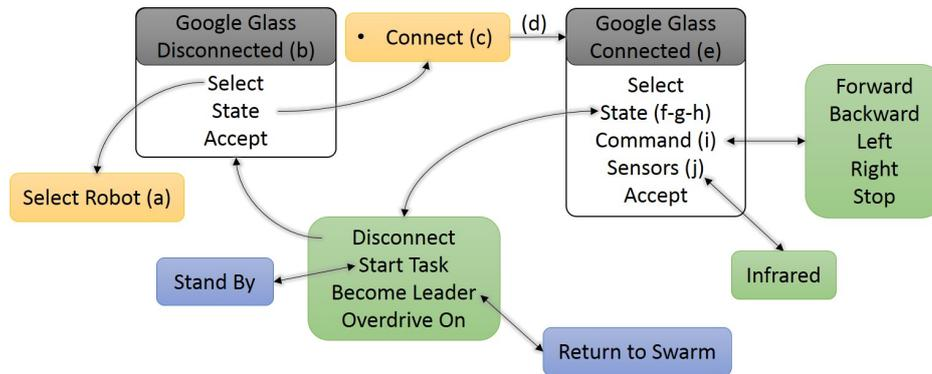
Fig. 3.10 Diagram explaining the architecture of the Google Glass software. The letters next to the instructions and arrows make reference to the screenshots presented in Fig. 3.9.
