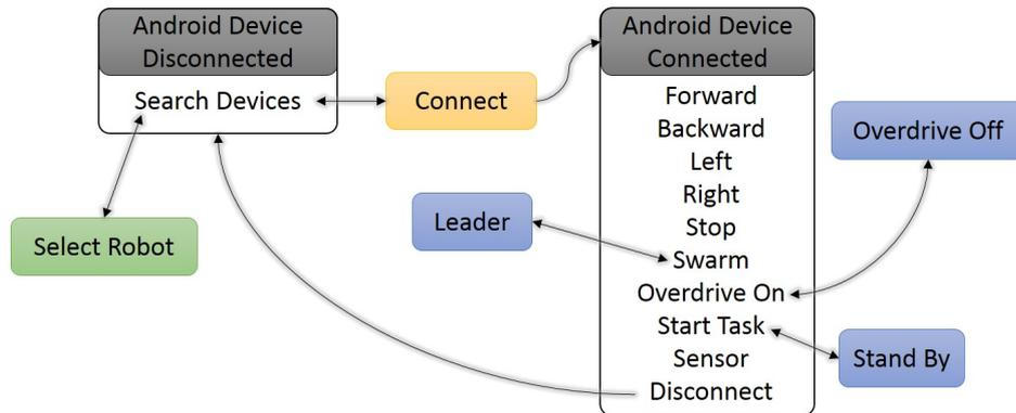
Fig. 3.6 Diagram of the architecture of the Android mobile device software.
