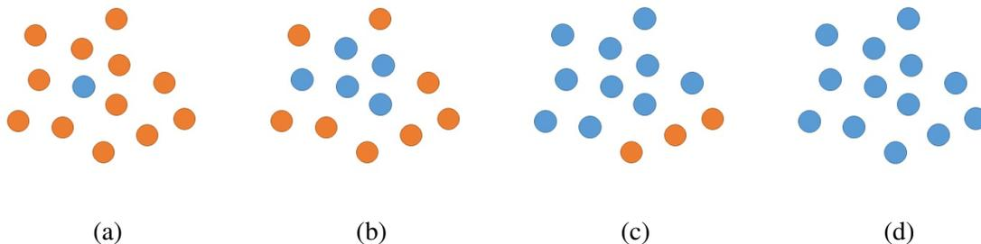
Fig. 4.4 The gossip algorithm relays a command to the nearest neighbours. a) The leader robot receives a new command from the operator. b) It relays it to the nearby robots. c) The nearby robots relay the message to their locally connected robots. d) Finally all robots have relayed the message to all the locally connected robots.
