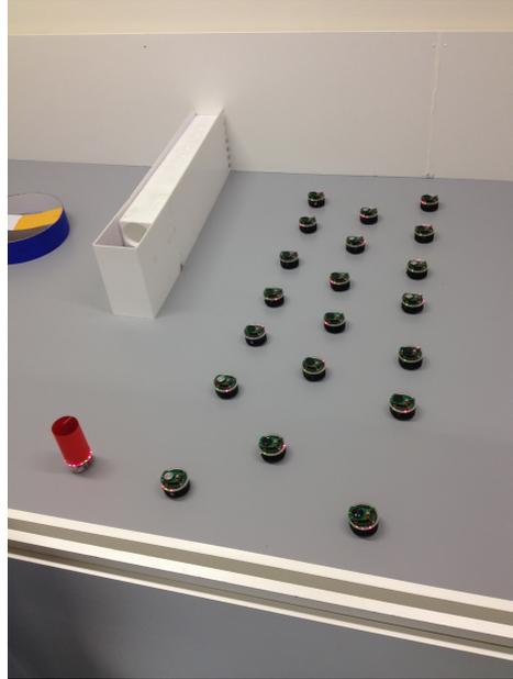
Fig. 3.11 Initial positions of the swarm robots, the leader robot and the object for every trial.
