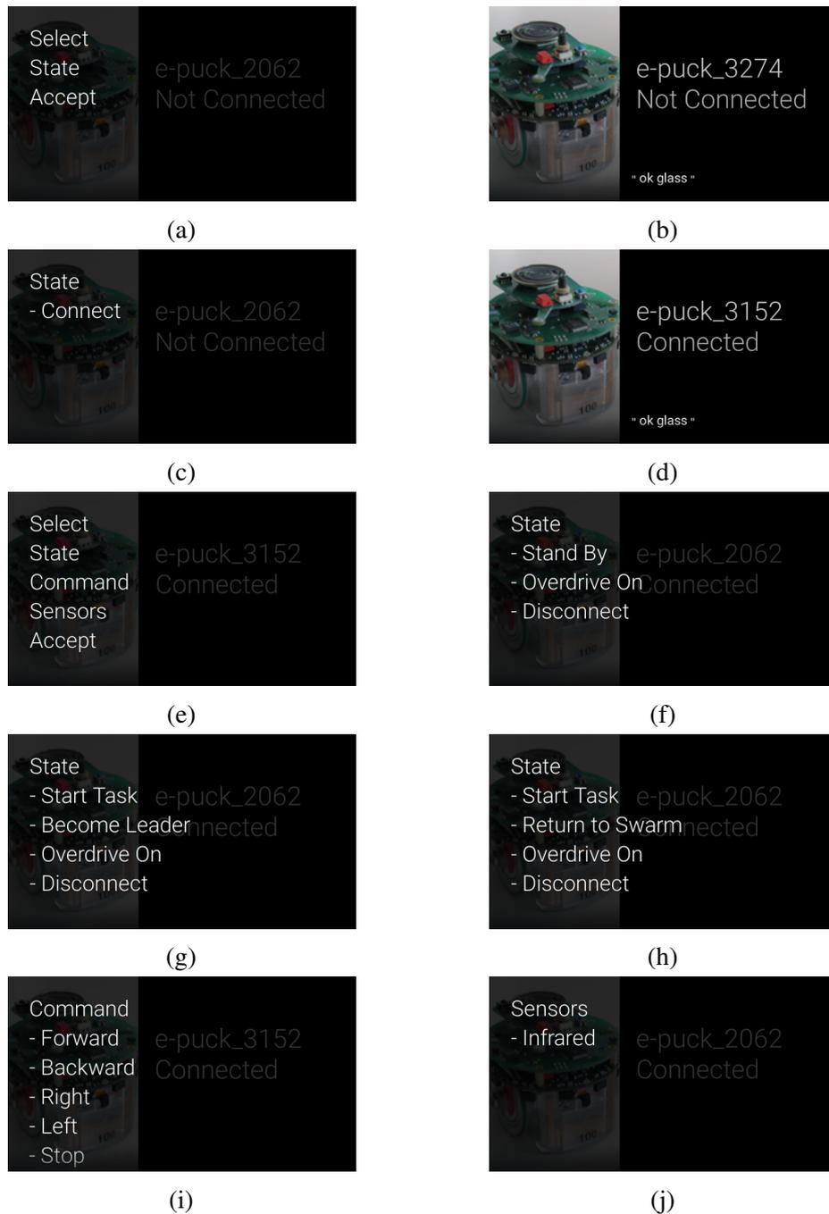
Fig. 3.9 Snapshots taken from the Google Glass interface: a) Disconnected “Main” menu. b) Disconnected Selection list. c) Disconnected “State” menu. d) Connected list. e) Connected “Main” menu f) Connected “State” menu while active. g) Connected “State” menu during “Stand-By” as swarm unit. h) Connected “State” menu menu during “Stand-By” as leader. i) “Commands” menu. j) “Sensor” menu .
