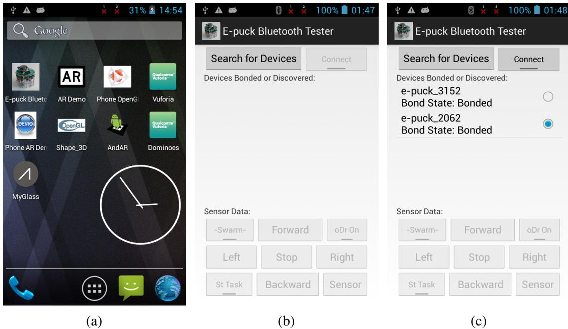
Fig. 3.5 Snapshots taken from the Android phone interface. a) The portable device main menu. b) The portable device when it starts searching for available e-puck robots. c) The portable device when it has already found some e-puck robots.
