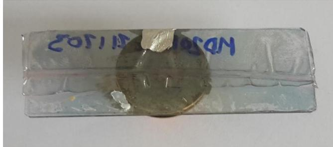
Figure 4.23: An acetate replica mounted on a glass microscope slide prepared for SEM observation
