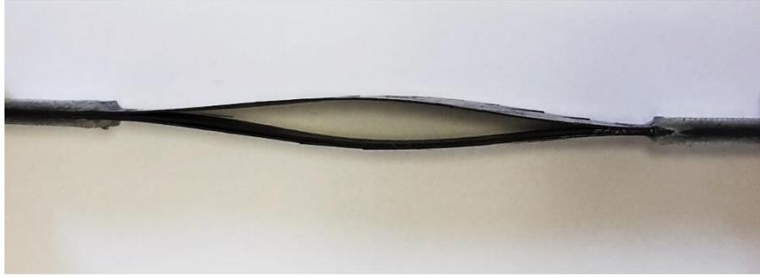
Figure 5.30 Example of a fatigued tensile specimen cycled to  $1 \times 10^6$  cycles. Compressive force was applied to the ends of the specimen by hand in order to open and emphasize the delamination.
