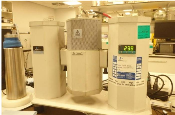
Figure 3.20: PerkinElmer DMA 8000
