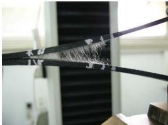
Figure 2.23: Electro-spun Nylon-6,6 fibre interleaf under mode I loading [85]
