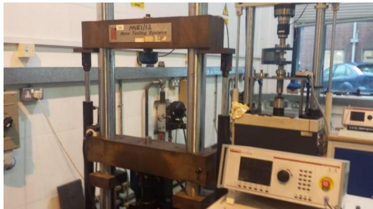
Figure 4.15: Nene 12.5kN servo-hydraulic test machine, and MOOG SmarTEST ONE controller
