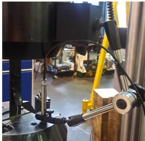
Figure 4.21: LVDT setup used to measure grip separation in tensile tests
