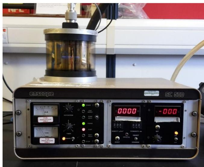
Figure 6.1: Emscope SC 500 gold vapour deposition machine
