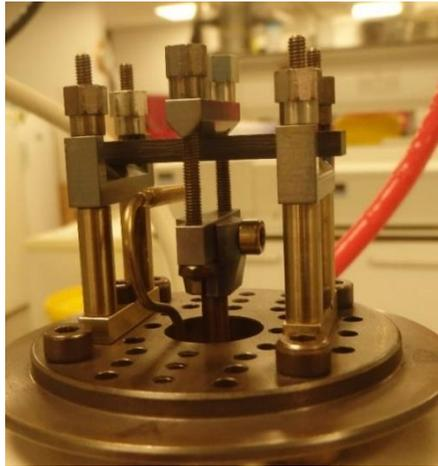
Figure 3.21: A sample mounted in the three point bend test configuration. The mechanical actuator is attached to the central loading point.
