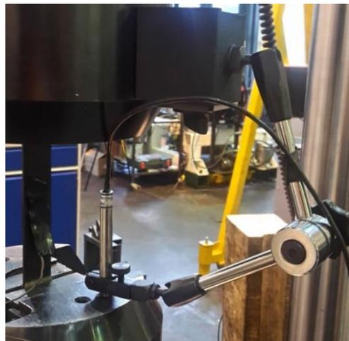
Figure 4.21: LVDT setup used to measure grip separation in tensile tests
