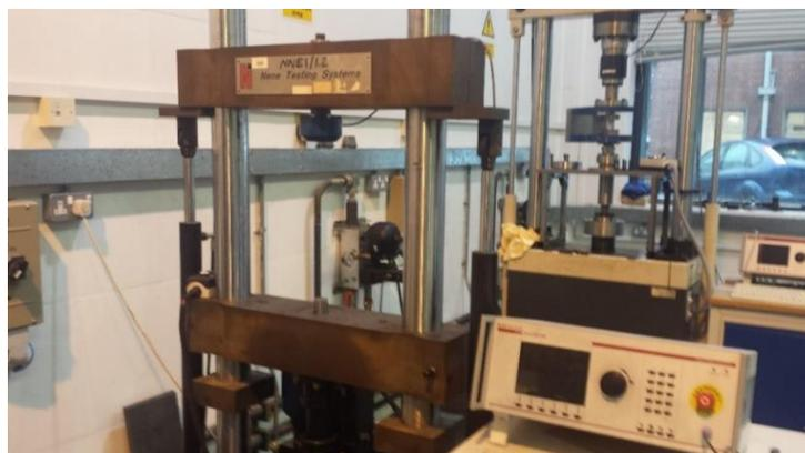
Figure 4.15: Nene 12.5kN servo-hydraulic test machine, and MOOG SmarTEST ONE controller
