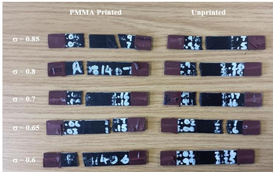
Figure 5.10: Randomly selected samples of ranging stress factors that failed in cyclic loading. In all cases, fracture occurred at the loading points.
