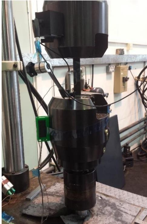
Figure 4.25: Tensile sample in situ in the Mayes 100kN servo-hydraulic test frame
