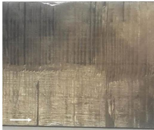
Figure 6.27 Photograph of a (gold coated) delamination surface (0° horizontal fibre orientation). Transverse crack lines are clearly visible. Delamination fronts propagated outwards from these cracks, driven forward by free edge stresses.
