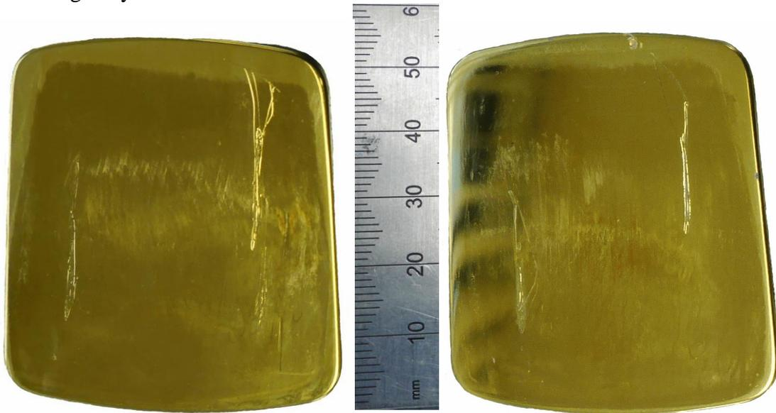
Figure 3.12 Scratched surfaces from wear track analysis
