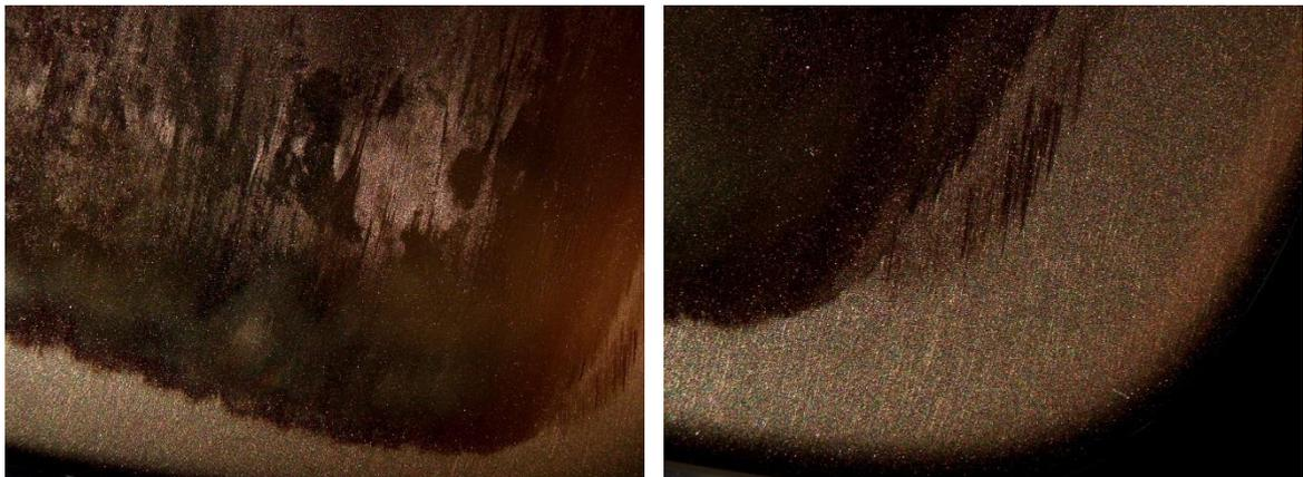
Figure 3.10 Optical microscope images of the worn insert footprint compared to unworn tibial edges
