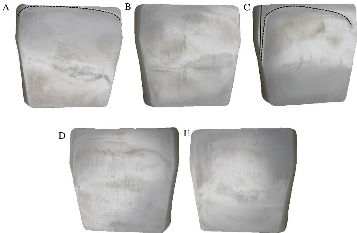
Figure 3.13 Photos of the superior insert surfaces at the end of 12Mc with edge loaded areas highlighted
