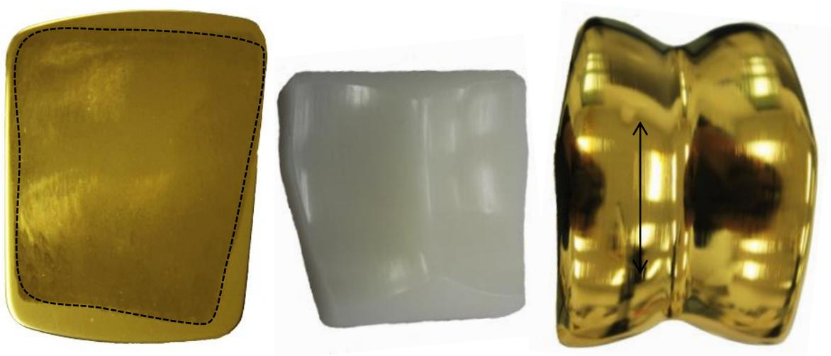
Figure 3.8 Typical component surfaces after 4Mc with insert imprint on tibial component and unidirectional scratches on the talar component
