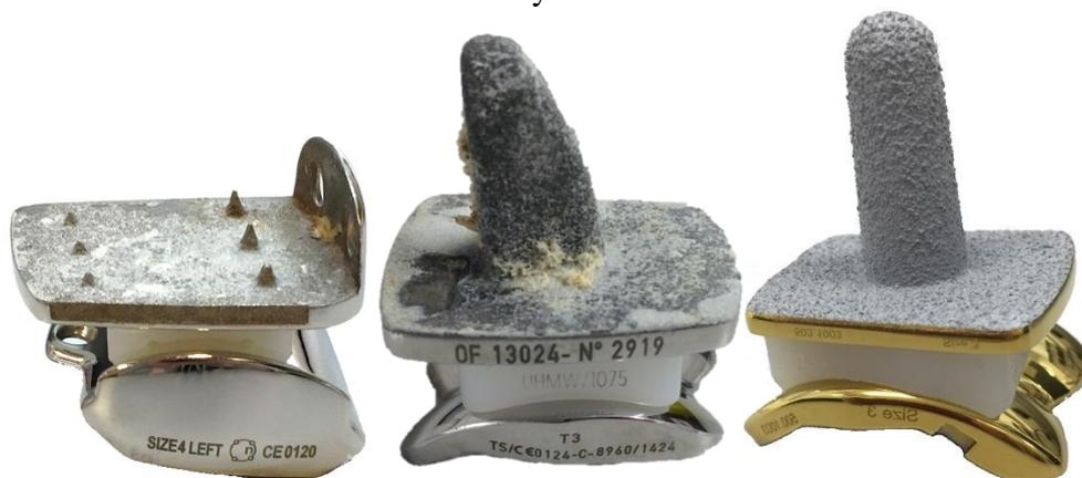
Figure 6.23 Retrieval Hingtegra and AES TARs compared to simulator Zenith components
