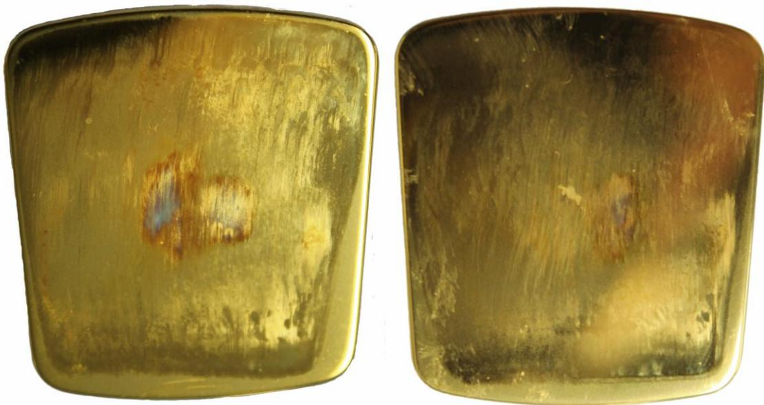
Figure 3.4: Two tibial components which experienced visual coating damage
