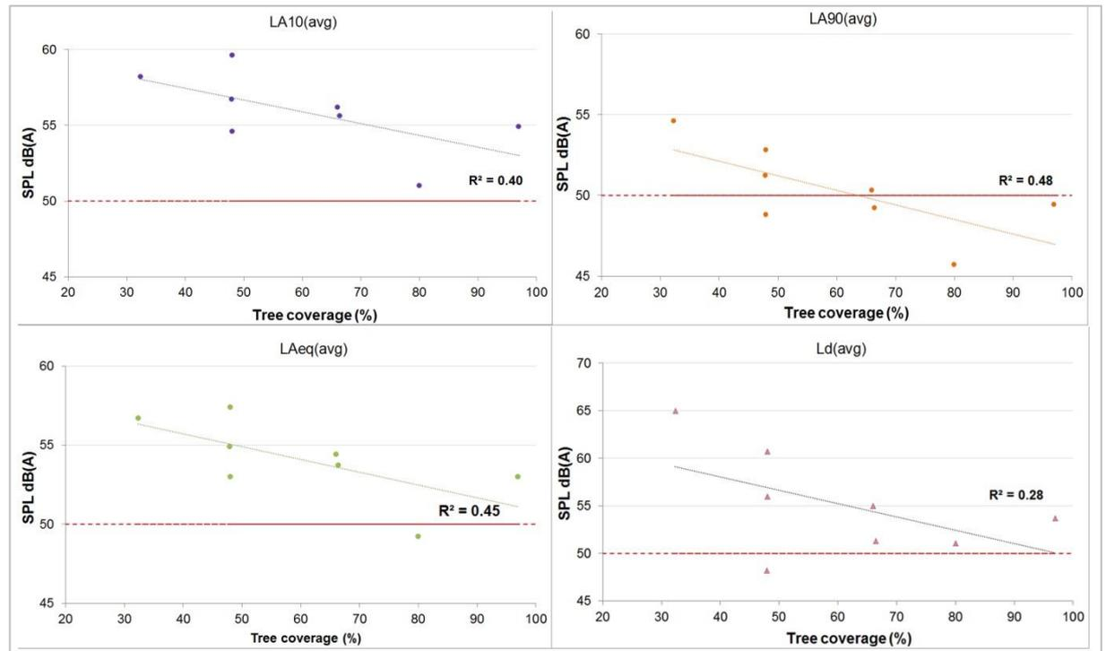
**Fig.6.12.** Correlations between tree coverage and  $L_{A10}$ ,  $L_{A90}$ ,  $L_{Aeq}$  and  $L_d$  with the respective  $R^2$  values. A cut-off line has been added at 50 dB(A) in order to facilitate the comparison among the noise indicators.  $L_{d(avg)}$  refers to simulated noise levels, while the other acoustic indicators refer to measured values in the parks.
