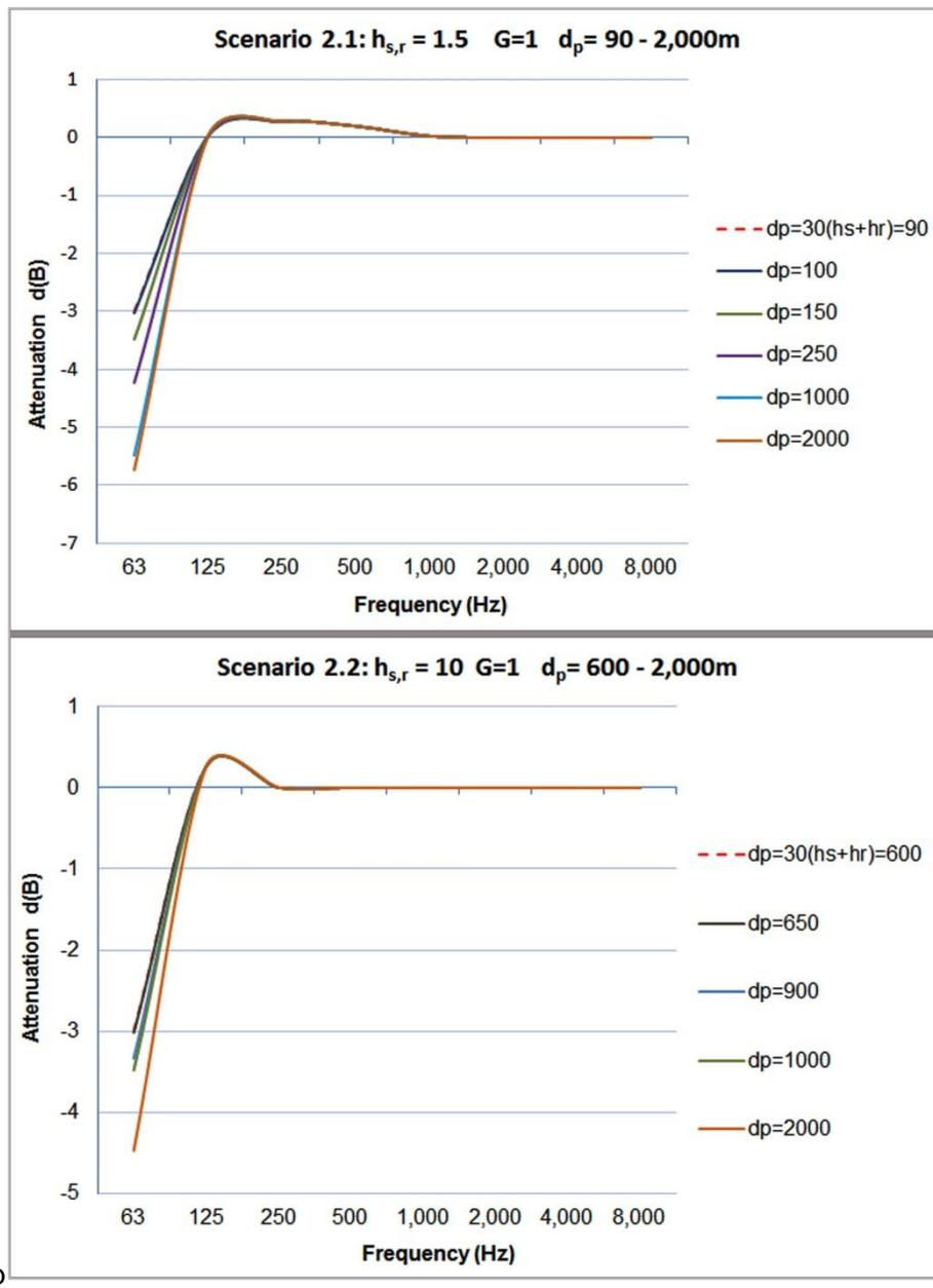
**Fig.3.4.** Scenario 2: Ground attenuation per octave band for  $G=1$ ,  $d_p=1.5-2,000\text{m}$  and (a)  $h_{s,r}=1.5\text{m}$ , (b)  $h_{s,r}=10\text{m}$
