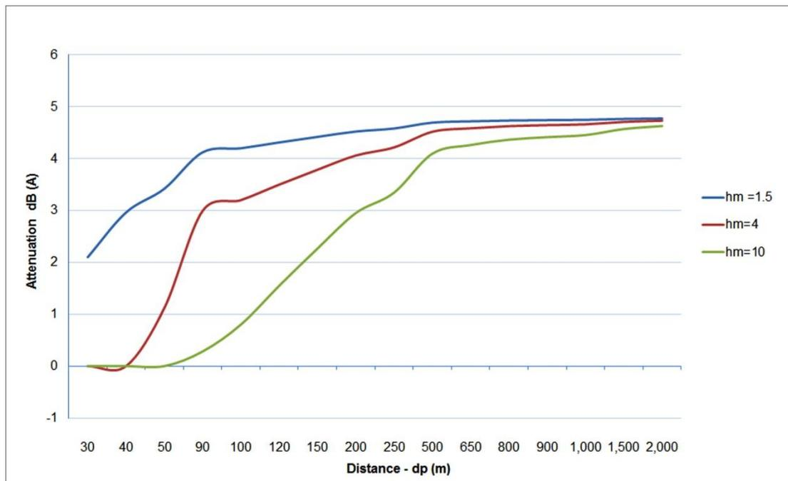
Fig.3.5. Attenuation in receiver's position with different height ( $h_m$ ) scenarios.
