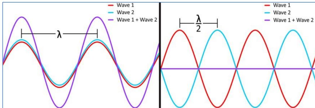
**Fig.2.1.** Example of positive interference (left) and negative (right) with the subsequent changes in the wave length. Source: <http://angstromengineering.com/thin-film-u/introduction-optical-coatings/>
