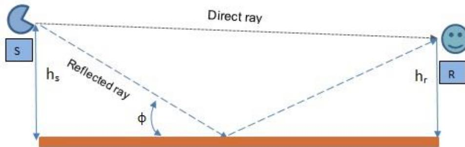
**Fig.3.1.** Reflected and direct ray in outdoor sound propagation between source (S) and receiver (R)
