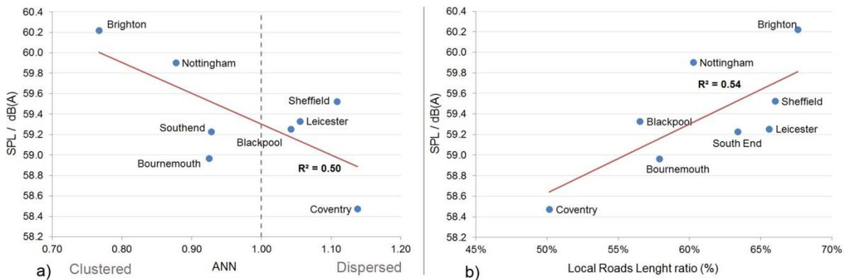
**Fig.5.6.** Statistically significant variables interacting with noise levels in the macro-scale: (a) Negative effect of the ANN ( $R^2= .50$ ), (b) Positive effect of the Local Roads Length ratio ( $R^2 = .54$ ).
