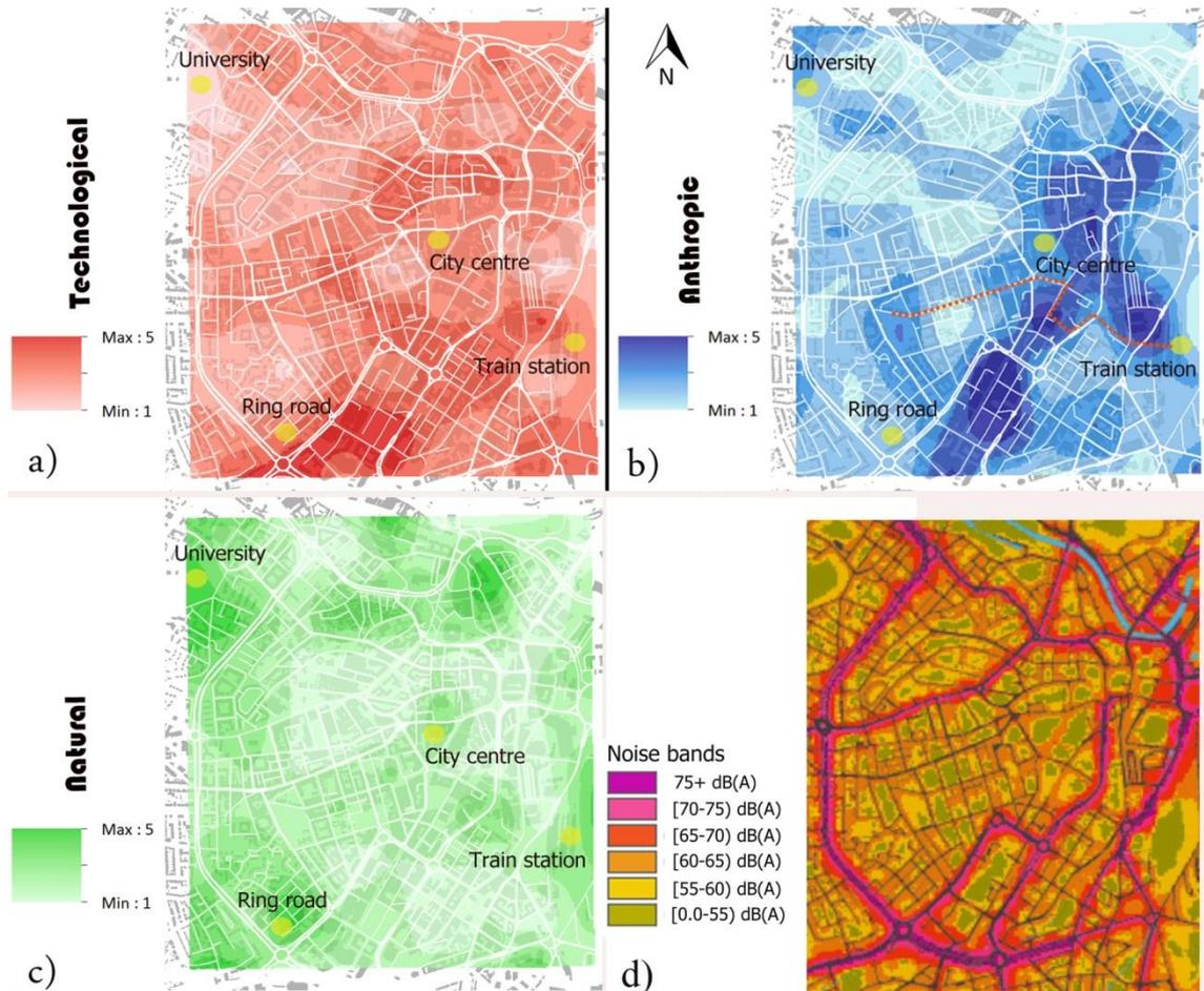
**Fig.8.6.** Spatial variability of the audible sound sources (technological, anthropic, natural) in comparison with the corresponding noise map for the area from the first round of noise mapping.
