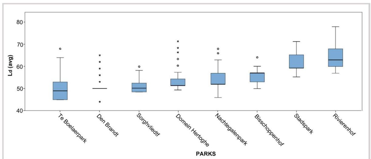
**Fig. 6.8.** Box and whisker plots representing the simulated noise levels within the borders of the eight parks sorted in an ascending form for  $L_{d(avg)}$ .
