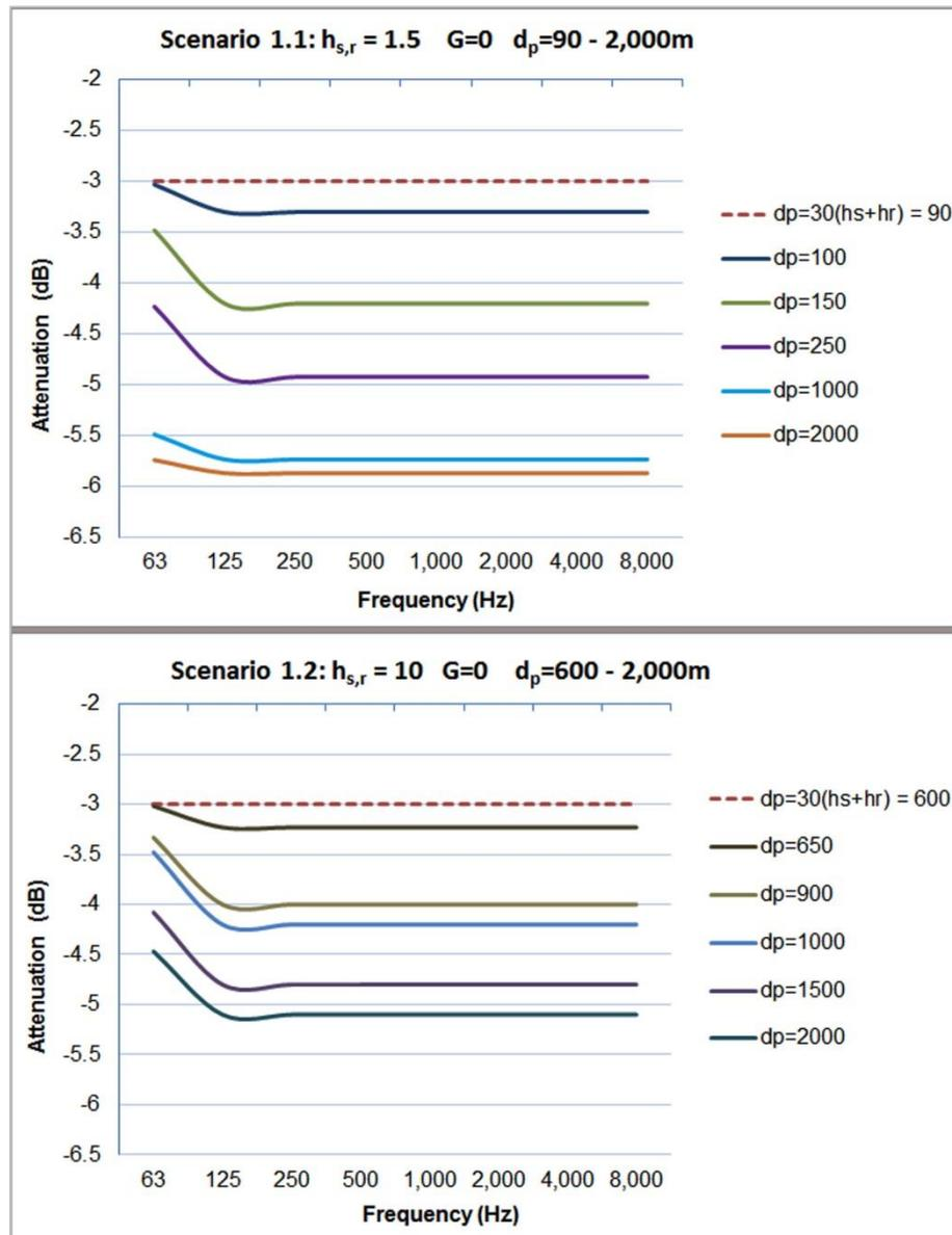
**Fig.3.3.** Scenario 1: Ground attenuation per octave band for  $G=0$ ,  $d_p=1.5\text{-}2,000\text{m}$  and (a)  $h_{s,r}=1.5\text{m}$ , (b)  $h_{s,r}=10\text{m}$
