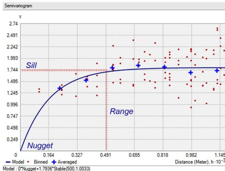
**Fig.8.3.** Typical example of semivariogram with the basic components of nugget, range and sill. The red dots represent groups of points (bins) within the lag distance.
