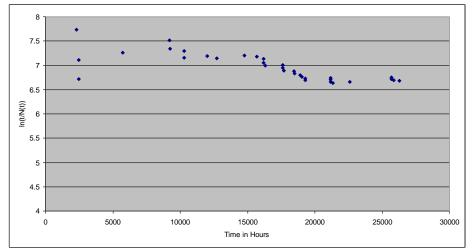
Figure 34: Cumulative Failure Rate against *t* on a log-linear Paper for Failures of Resource D Site 1.
