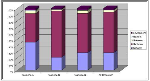
Figure 9: Breakdown of Downtime into Root Causes for Resources from Site 2.
