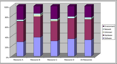
Figure 8: Breakdown of Downtime into Root Causes for Resources from Site 1.
