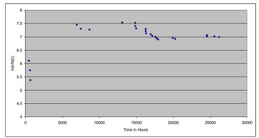
Figure 31: Cumulative Failure Rate against t on a log-linear Paper for Failures of Resource A Site 1.
