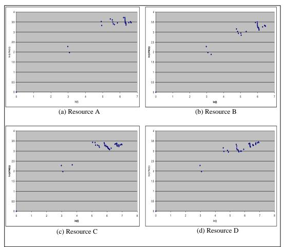
Figure 91: The Duane Plot for Resources Repairs time, Site 1.
