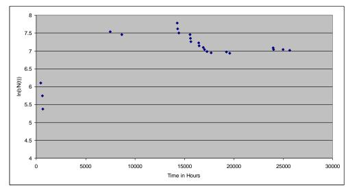
Figure 32: Cumulative Failure Rate against *t* on a log-linear Paper for Failures of Resource B Site 1.
