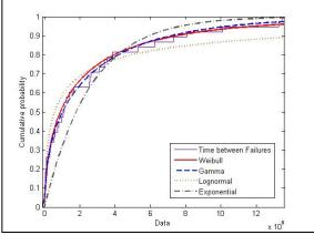
Figure 23: Time between Failures for Resource C Site 2.
