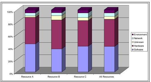
Figure 7: Breakdown of Failures into Root Causes for Resources from Site 2.
