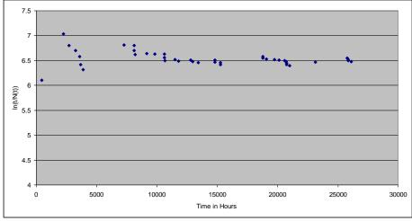
Figure 36: Cumulative Failure Rate against *t* on a log-linear Paper for Failures of Resource B Site 2.
