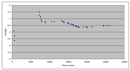
Figure 33: Cumulative Failure Rate against *t* on a log-linear Paper for Failures of Resource C Site 1.
