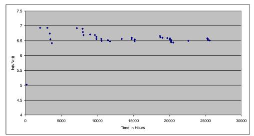
Figure 37: Cumulative Failure Rate against t on a log-linear Paper for Failures of Resource C Site 2.
