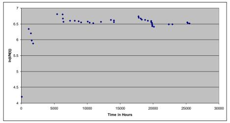
Figure 35: Cumulative Failure Rate against t on a log-linear Paper for Failures of Resource A Site 2.
