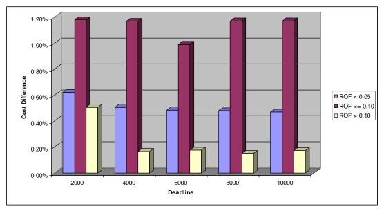
Figure 82: Percentage Difference between DRFC Execution Cost and Optimal Cost Experiment 8.
