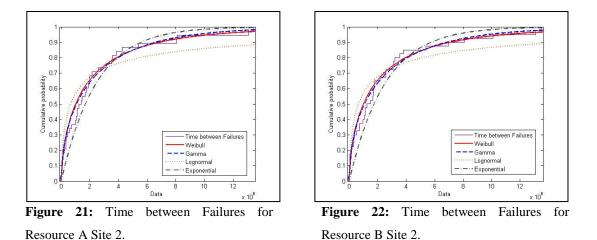
In Resource A, the distribution between failures is well modelled by a Weibull or Gamma distribution. Both distributions create an equally good visual fit and the same negative log-likelihood.
