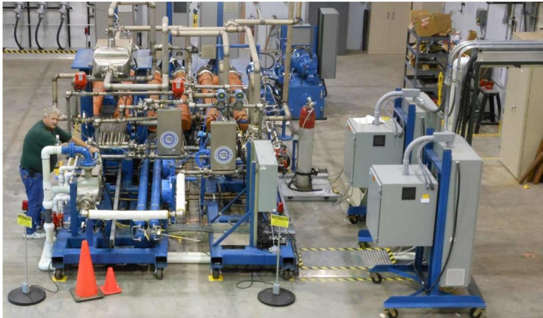
Figure 2-12 S-CO<sub>2</sub> split flow recompression CBC test assembly at SNL (Courtesy of SNL)
