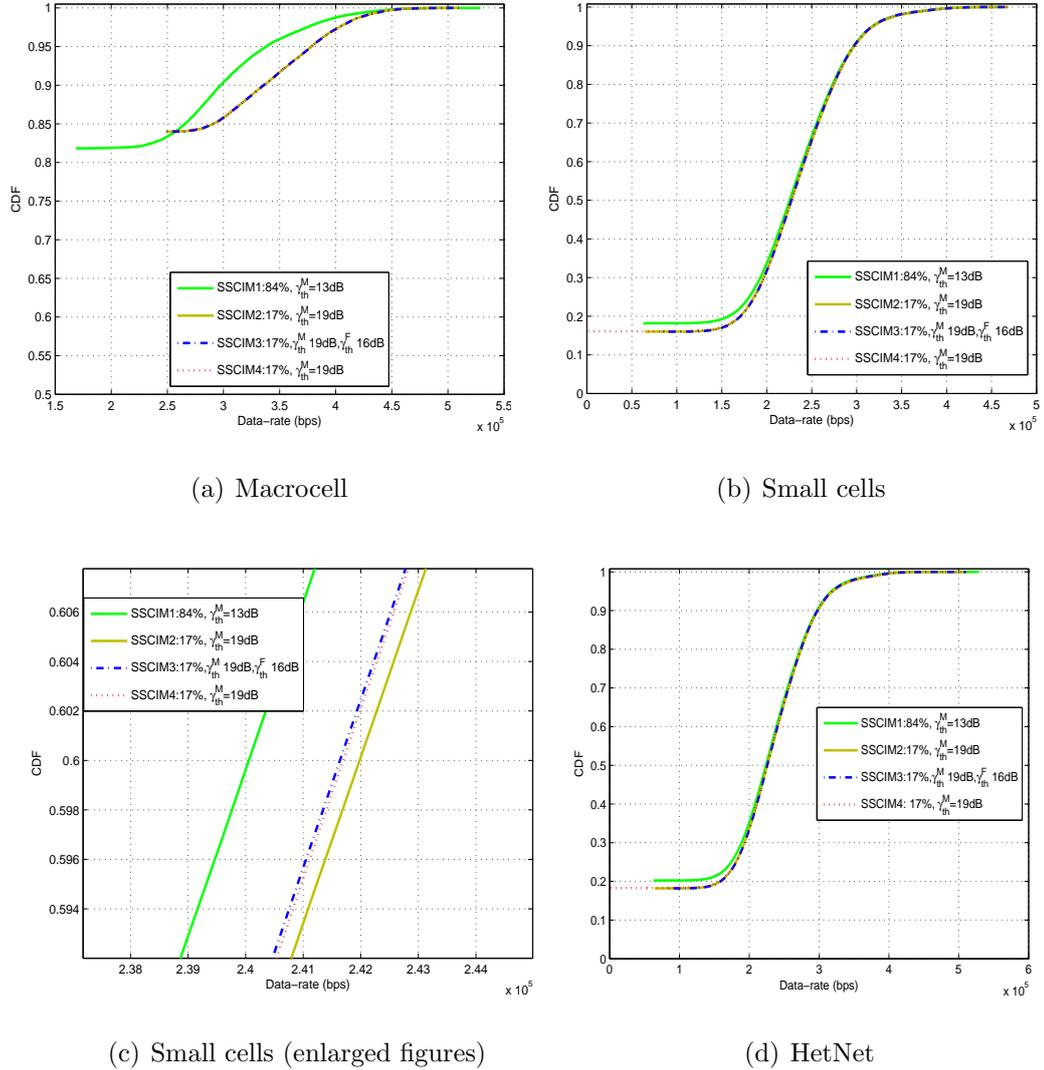
**Figure 5.3:** Cumulative distribution function of user data-rate for SSCIM.
