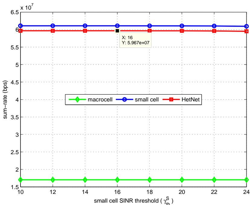
**Figure 5.1:** Average capacity per symbol period of SSCIM3:  $\varphi_M$  17%,  $\gamma_{th}^M$  19dB.
