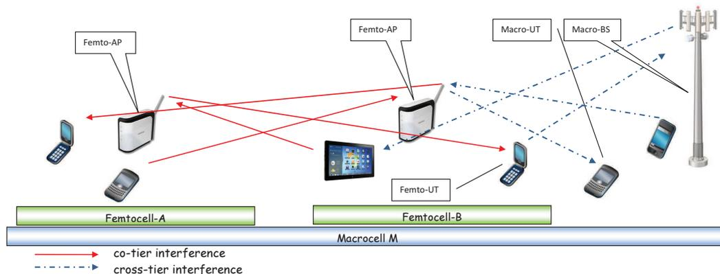
Figure 3.2: Co-/ cross-tier interference in heterogeneous cellular networks
