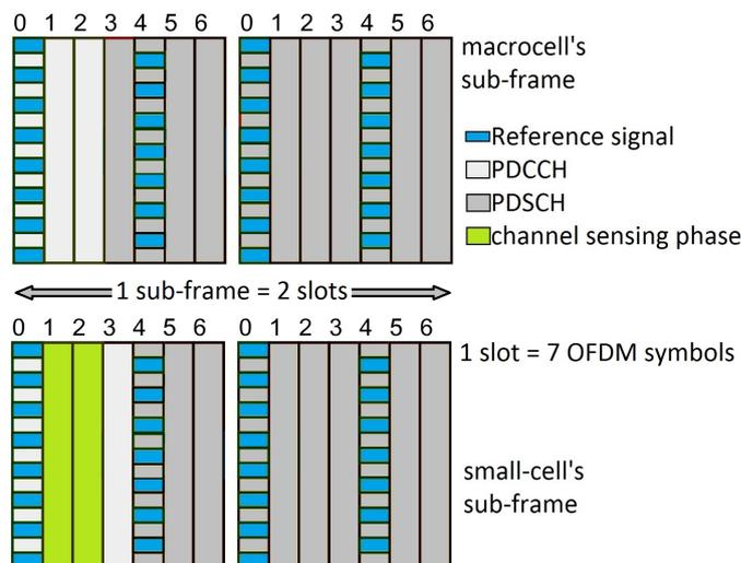
**Figure C.3:** The model of sub-frames in HetNet used in simulation
