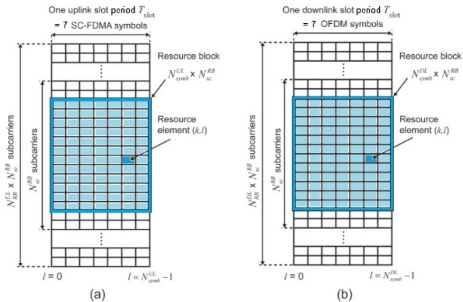
**Figure C.2:** Resource blocks of 3GPP-LTE for (a) uplink and (b) downlink; adapted from Rumney (2013)
