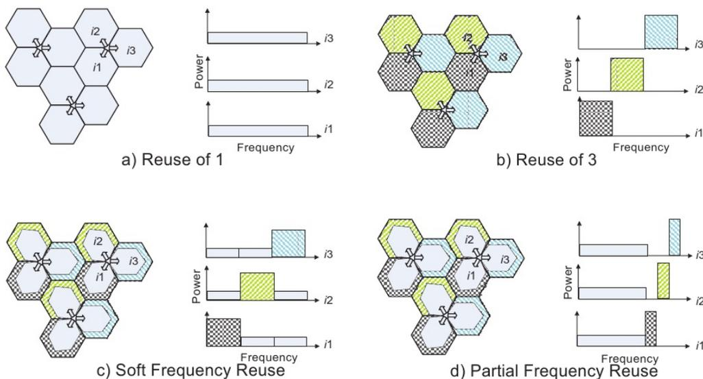
**Figure 3.4:** Spectrum splitting and reuse methods adapted from [Rahman and Yanikomeroglu \(2010\)](#)
