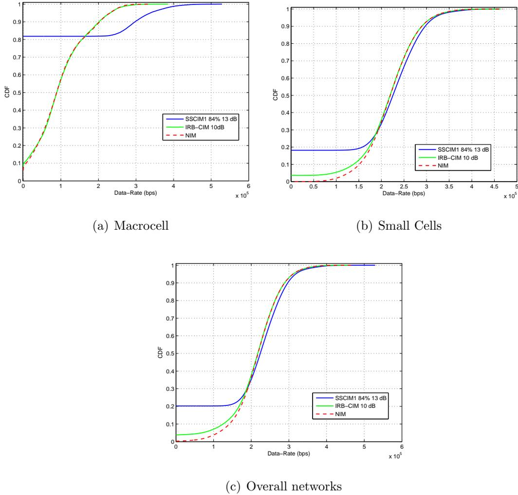
**Figure 4.6:** Distribution function of data-rate for different schemes.
