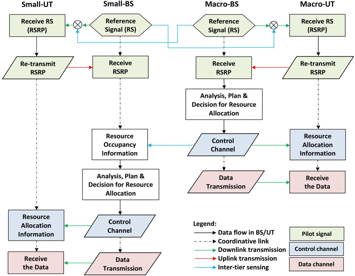
**Figure 4.2:** Downlink signalling procedure for the even slot of each subframe
