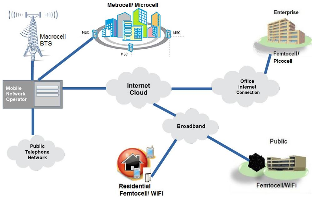
**Figure 2.1:** Small cells as an integral part of modern mobile networks
