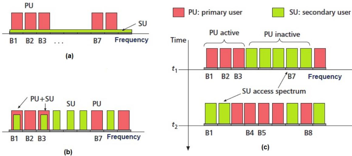
**Figure 3.6:** Dynamic spectrum access models in cognitive radio: (a) Underlay, (b) Overlay, (c) Interweave; adapted from [Song et al. \(2012\)](#).
