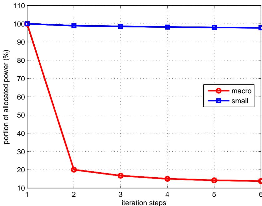
**Figure 6.5:** The average portion of the allocated power over the maximum power of each cell when using sOSPA 4 dB (outdoor, 75 m, 6 UTs for each cell).
