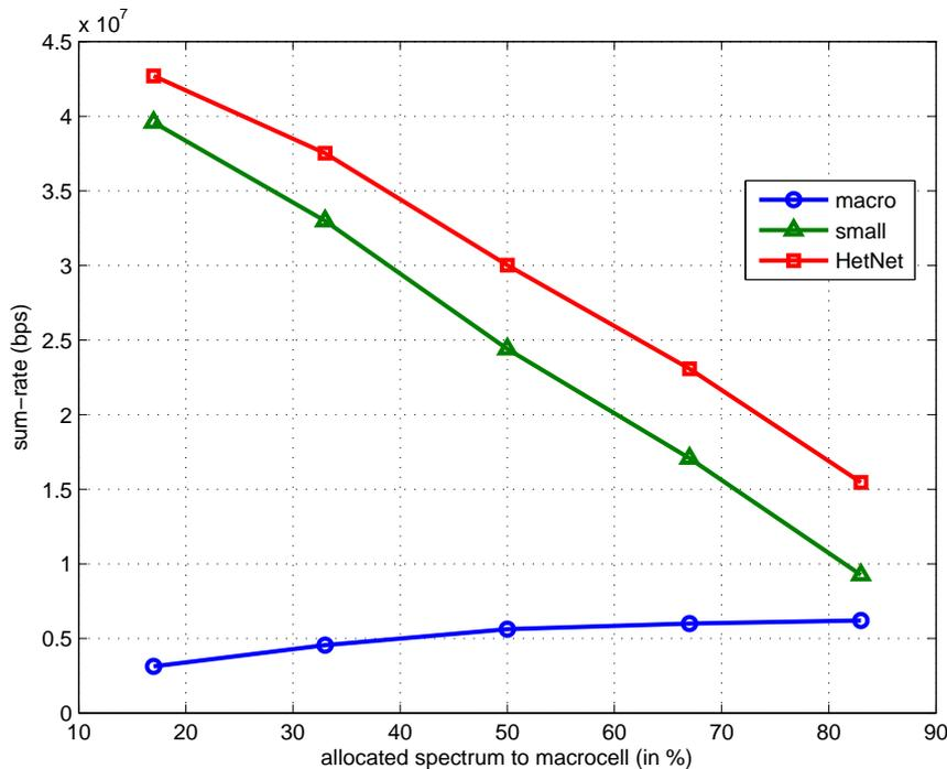
**Figure 6.2:** Average sum rate of each cell using the SSA method with  $d_{MS0}$  75 m (outdoor), 6 UTs per cell, and portions of the macrocell's spectrum.
