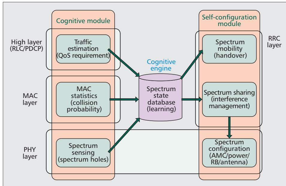
**Figure 2.5:** Cognitive small cell functional architecture ©2013 IEEE (Huang et al., 2013).
