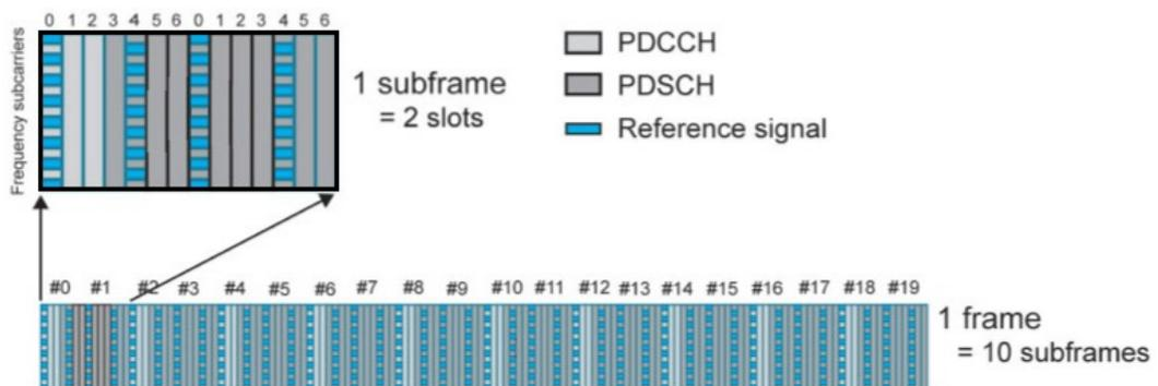
**Figure C.1:** The simplified LTE frame structure used in simulation
