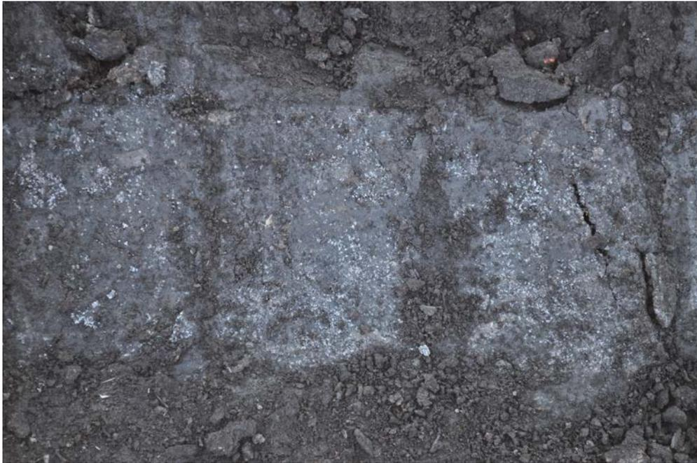
Figure A1.15. Heavy crystal formation on the top of the soil of the wetland unit after 11 months.
