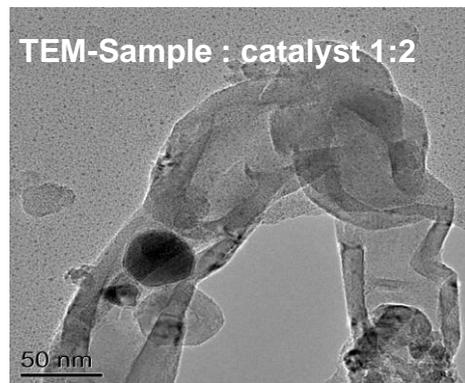
**Figure 4-19 SEM and TEM images of reacted catalysts from the pyrolysis-catalysis of waste tyres at different tyre:catalyst ratios (1:0.5; 1:1; 1:2) with no water and 900°C .**
