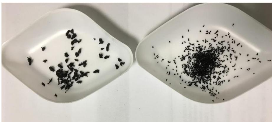
Figure 3-1 Waste truck (left) and car tyres (right) samples
