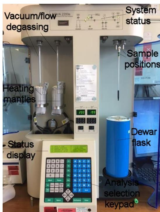
Figure 3-10 NOVA 2200e instrument used to characterize the porous properties of catalysts.
