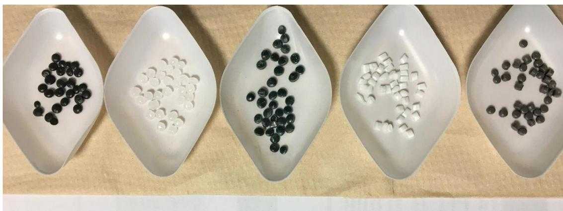
**Figure 3-2 Plastic samples (From left to right: HDPE, LDPE, PS, PET and PP).**
