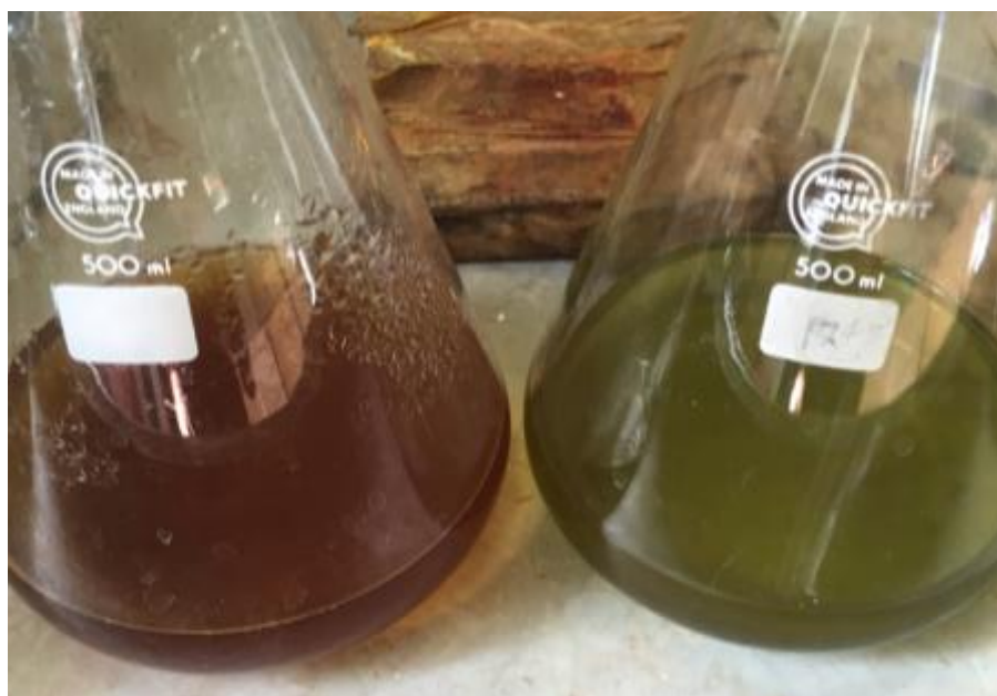
Figure 3.9. Extracts of golden rod with water as a solvent (left) and ethanol as solvent (right).
