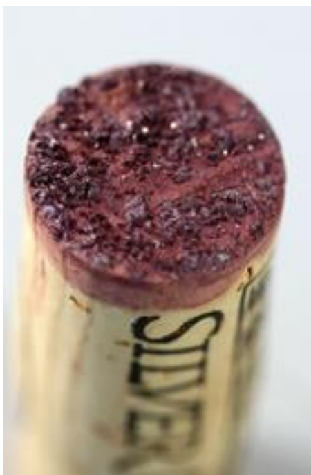
Figure 1.9. Crystals of potassium tartrate formed on the inside of a wine cork.
