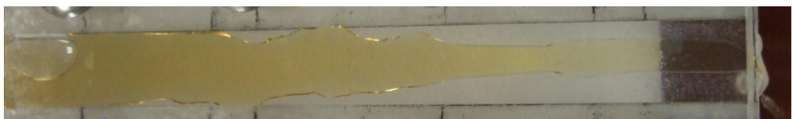
**Figure 4.3: Sporadic wetting of the oil phase with the cell cleaned and prefilled with the aqueous phase**
