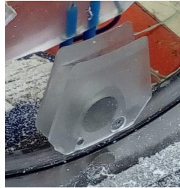
Figure 7.2 (left): AEI Calibration grid detail (inset: support)
