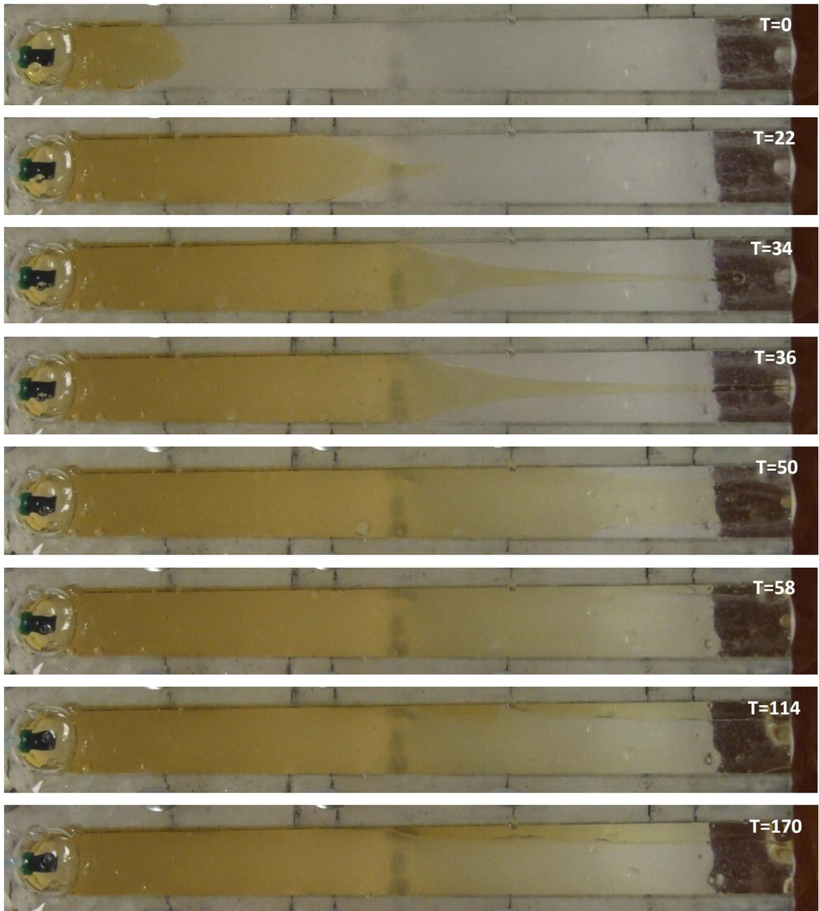
Figure 4.6: Evolution of the channel flow profile for the aqueous-prefilled case, viewed from above.
