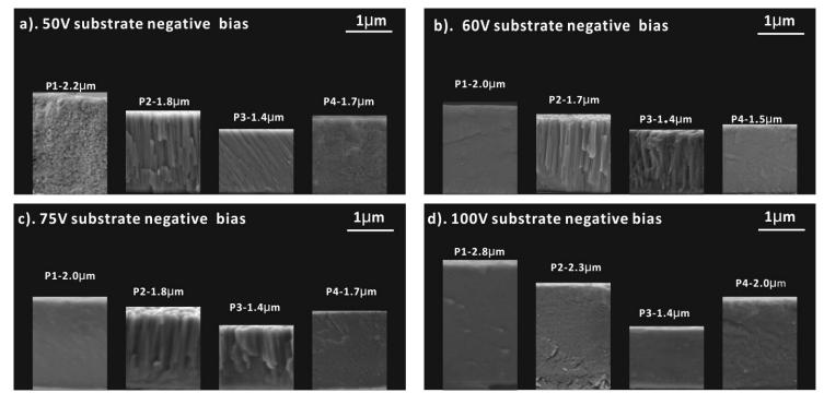
Figure 5.4: Fractured cross-sectional morphologies of AlCuMoMgZrB layers deposited at: (a) 50 V; (b) 60 V; (c) 75 V; (d)100 V substrate negative bias
