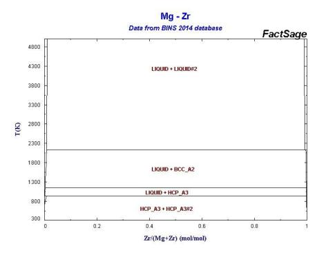
Figure 8.1 Mg-Zr binary phase diagram
