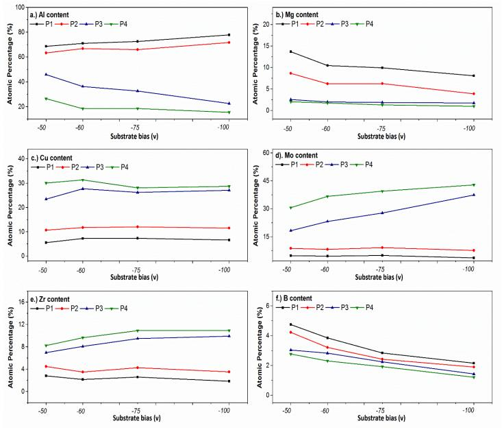
Figure 5.1 Elemental compositions varying with substrate negative bias; (a) Al; (b) Mg; (c) Mo; (d) Cu; (e) Zr; (f) B
