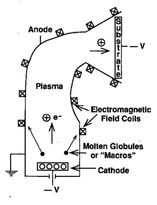
Figure 3.1 The Curved Configuration of Magnetically Filtered Cathodic Arc Evaporation System [61]
