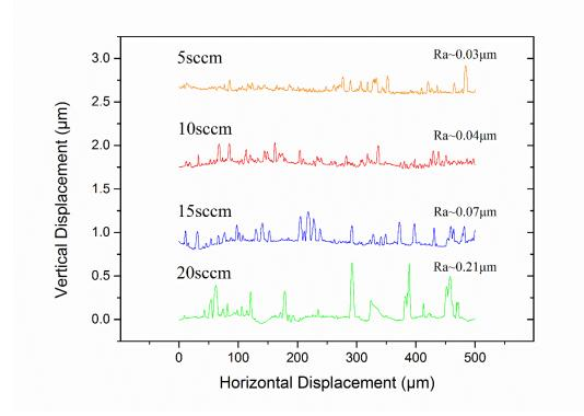
Figure 7.7 Two-dimensional surface profilometry of AlCuMoMgZrB(N) coatings
