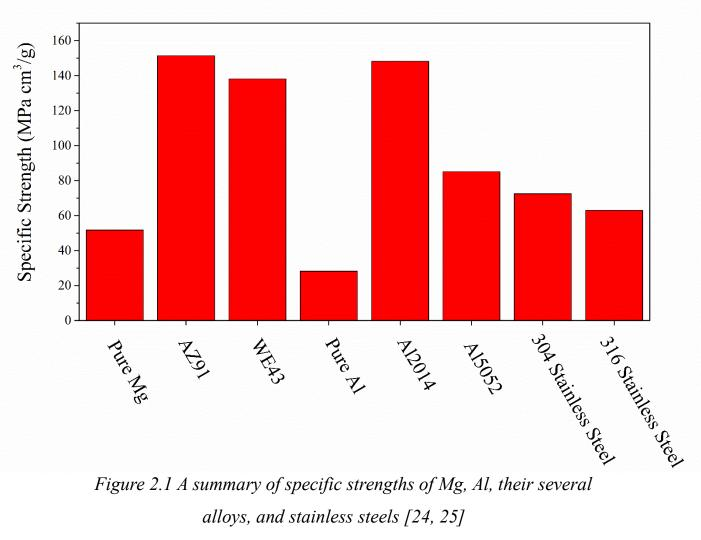
Figure 2.1 A summary of specific strengths of Mg, Al, their several alloys, and stainless steels [24, 25]
