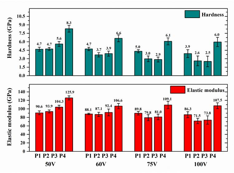
Figure 6.1 Hardness and elastic modulus of AlCuMoMgZrB layers H and E of WE43 substrate were detected as 56.2 GPa and 1.4 GPa, respectively
