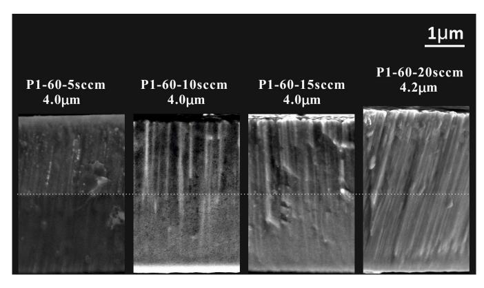
Figure 7.5 Fracture cross-sectional morphologies of AlCuMoMgZrB(N) coatings
