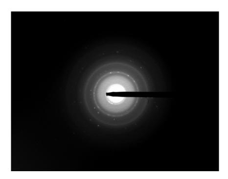
Figure 7.4 SAED pattern images of P1-60-15sccm coating
