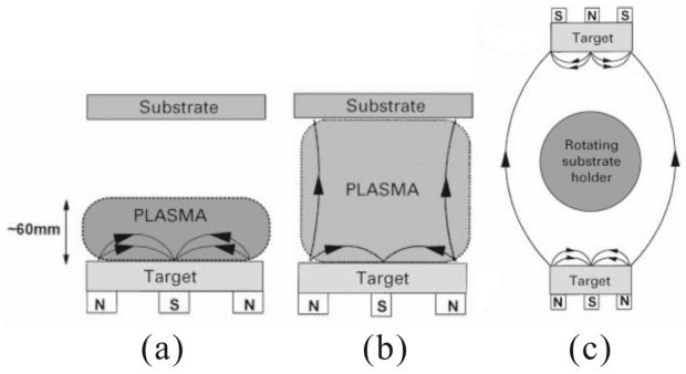
Figure 3.2 Different configurations of magnetron sputtering (a) Balanced magnetron; (b) Unbalanced magnetron (c) Closed-field configuration [106]:
