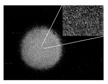
Figure 4.8 SEM image of 3B abrasive wear mode in WE43 Mg alloy
