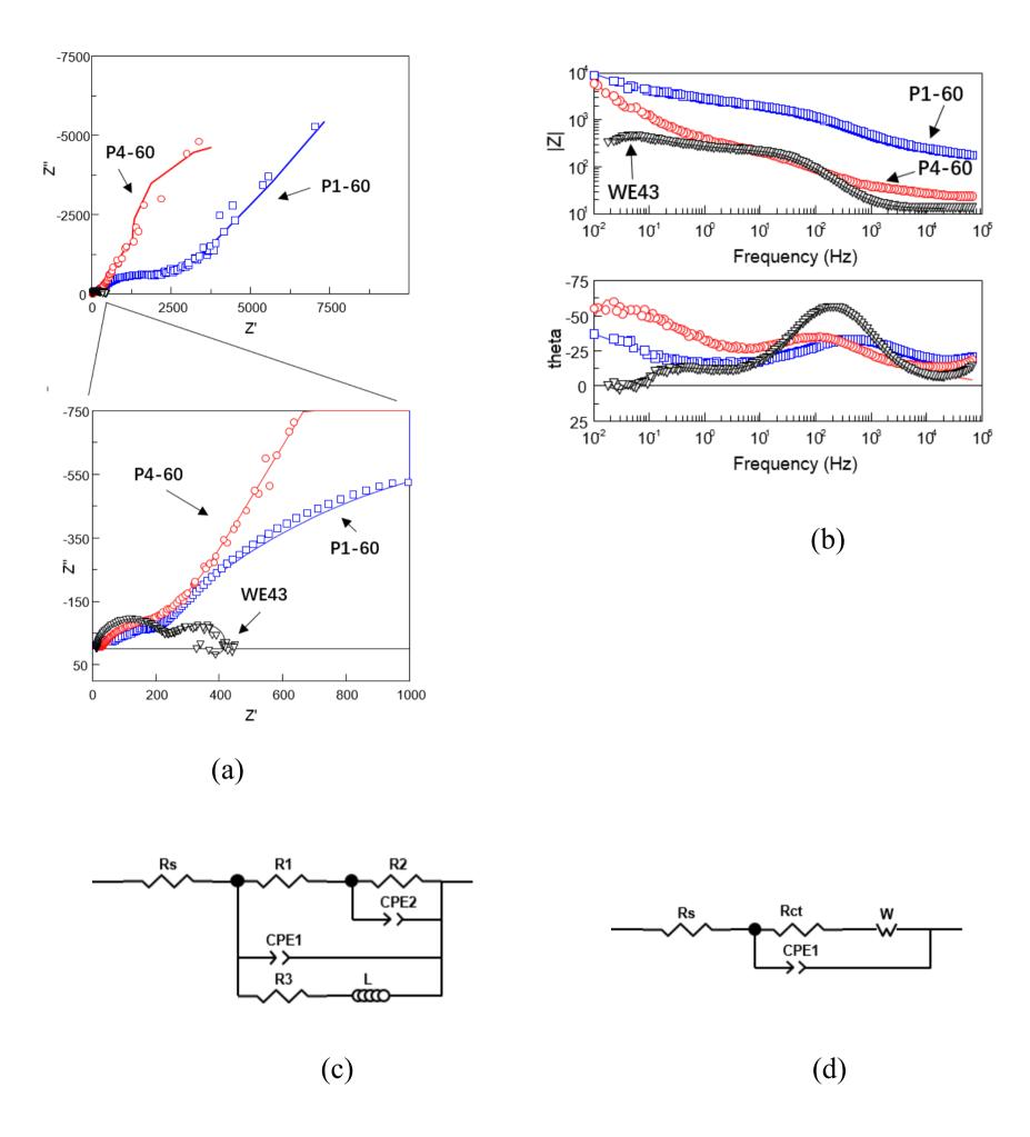
Figure 6.7 EIS analysis of P1-60 and P4-60 layers and WE43 substrate: (a) Complex plot,(b) Bode plots, (c) equivalent circuit for WE43 substrate and (d) equivalent circuit for P1-
