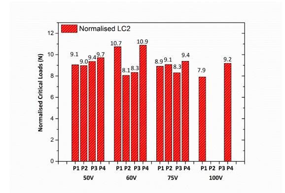
Figure 6.4: Normalised L<sub>C2</sub> of AlCuMoMgZrB layers
