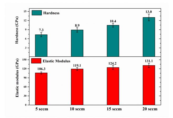
Figure 7.8 Hardness and elastic modulus of AlCuMoMgZrB(N) coatings
