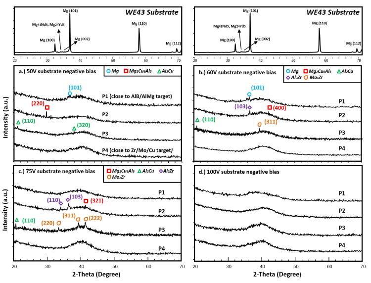
Figure 5.3 XRD patterns of WE43 substrate and AlCuMoMgZrB layers deposited at: (a) 50 V; (b) 60 V; (c) 75 V; (d)100 V substrate negative bias
