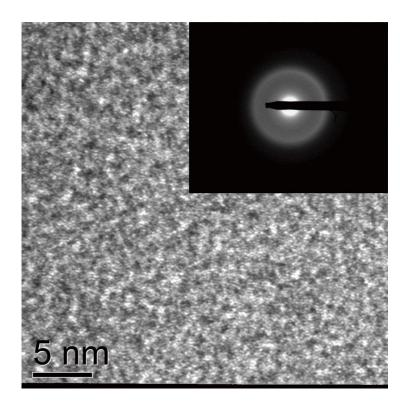
Figure 6.9 HRTEM and SAED pattern images of cross section foil of P1-60 layer
