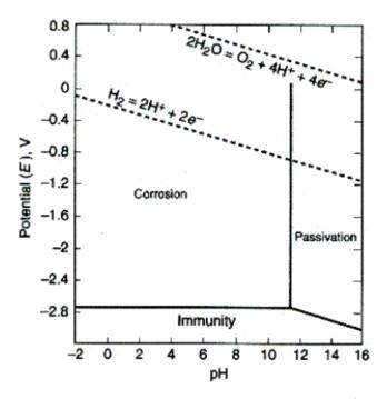
Figure 2.2 Pourbaix diagram of magnesium at 25 C water [27]
