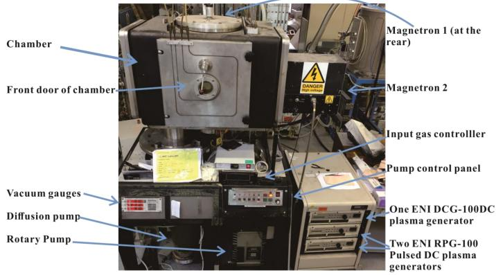
Figure 4.2 The Nordiko unbalanced magnetron sputtering
