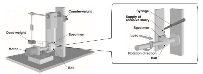
Figure 4.7 Schematic diagram of the "fixed-ball" micro-abrasion apparatus and its operating details [145]
