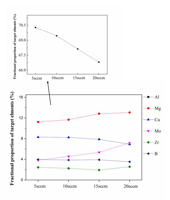
Figure 7.1 Fractional proportion of Al, Mg, Cu, Mo, Zr and B elements in each as-deposited coating excluding N
