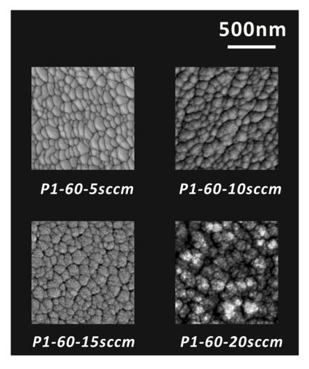
Figure 7.6 Surface morphologies of AlCuMoMgZrB(N) coatings
