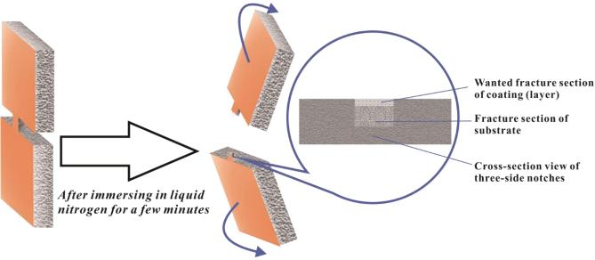
Figure 4.5 Schematic of preparing fracture sections
