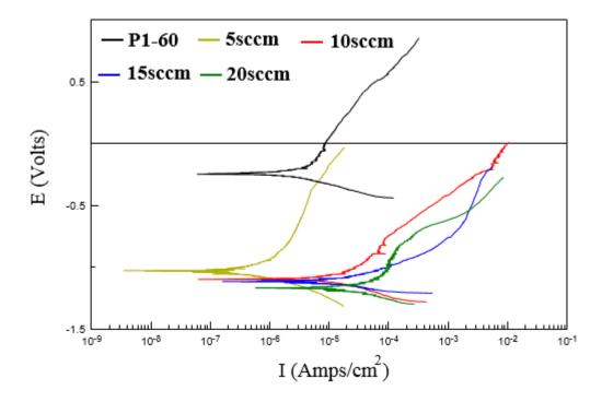
Figure 7.11 Potentiodynamic polarisation curves of AlCuMoMgZrB(N) coatings and the P1-60 base layer (ie. '0 sccm').
