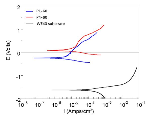
Figure 6.8 Potentiodynamic polarisation curves of WE43 substrate, P1-60 and P4-60 layers
