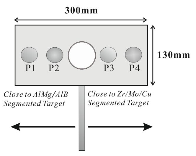
Figure 4.1 Plan-view of substrate holder prior to deposition
