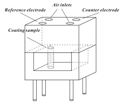
Figure 4.9 A schematic diagram showing the plane three-electrode cell
