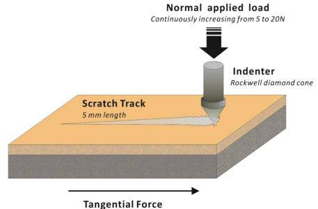
Figure 4.6 Schematic view of scratch-adhesion tester arrangement
