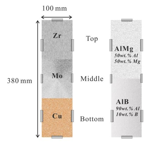
Figure 4.3 Schematic drawing of segmented targets
