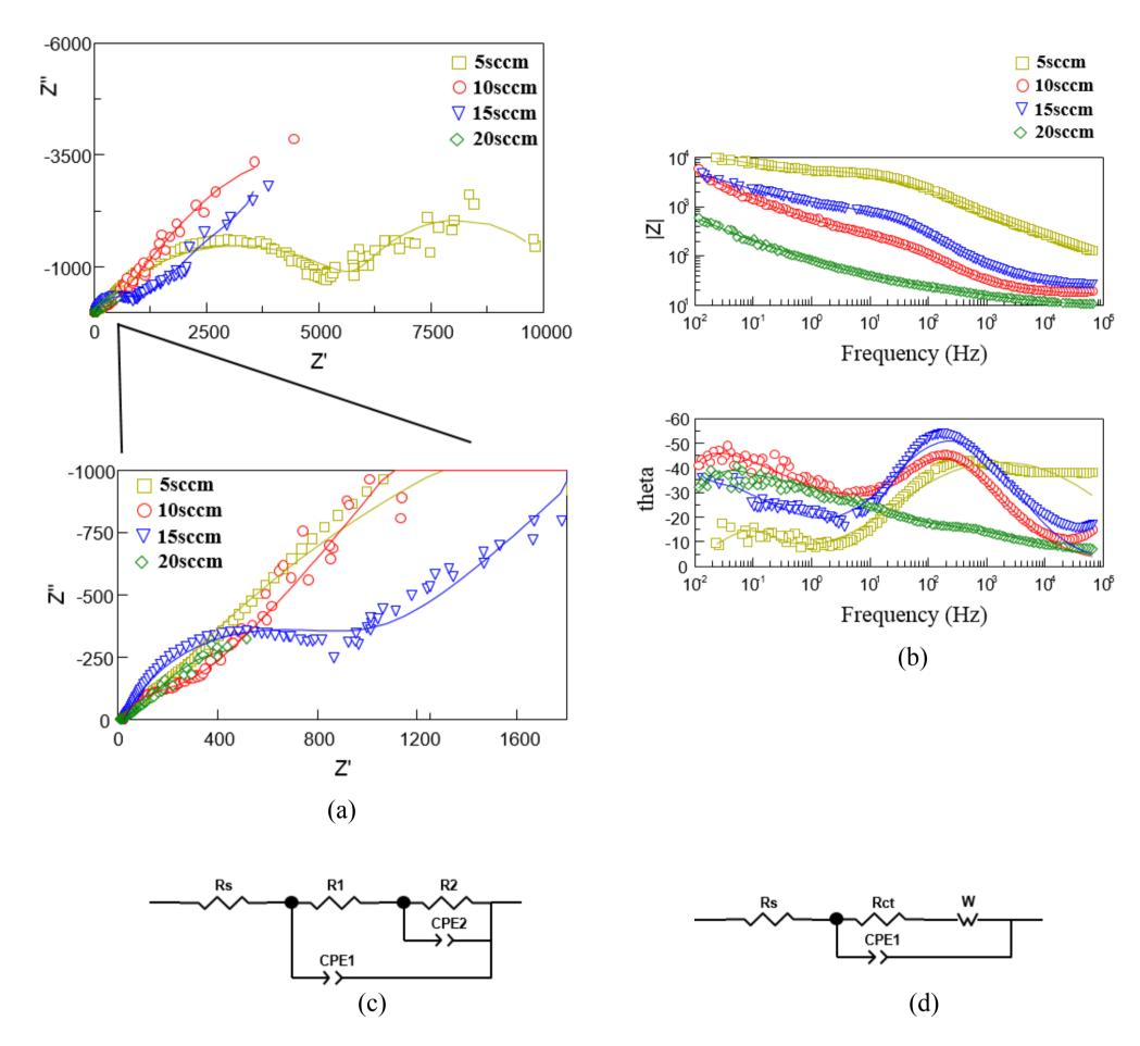
Figure 7.10 EIS analysis of AlCuMoMgZrB(N) coatings: (a) Complex plot, (b) Bode plots, (c) equivalent circuit for P1-60-5sccm coating and (d) equivalent circuit for P1-60-10sccm, P1-60-15sccm and P1-60-20sccm coatings
