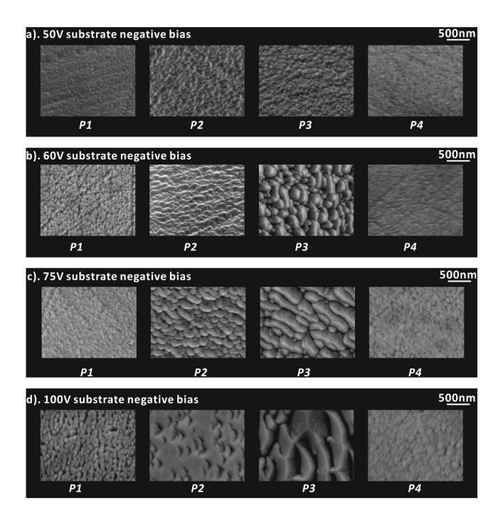
Figure 5.5 Surface morphologies of AlCuMoMgZrB layers deposited at: (a) 50 V; (b) 60 V; (c) 75 V; (d)100 V substrate negative bias
