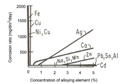
Figure 2.3 Effect of alloying elements on corrosion rate of magnesium in 3% NaCl solution at room temperature [31]
